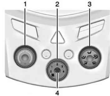
Climate Control System with Heater Only
