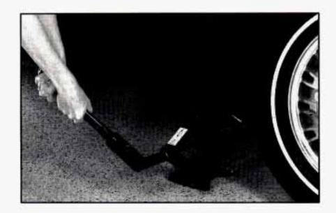
8. Lower the vehicle by turning the jack handle to the left. Lower the jack completely.
