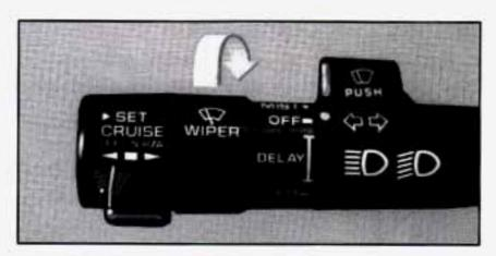
WIPER: Turn the band on the turn signal lever to control the wipers.
