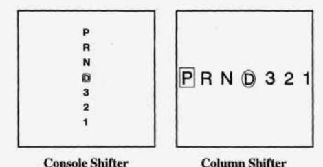
PARK (P): This position locks the front wheels. It's the best position to use when you start the engine because your vehicle can't move easily.
