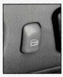
Press the power door lock to lock or unlock all the doors at once. The rear power door locks provide a lock only function as a convenience feature. For safety reasons, they will not unlock the doors.
