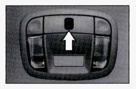
The control switch only works when the ignition is on or when the Retained Accessory Power (RAP) is active. Press the switch rearward and release to express-open the glass panel and sunshade. The sunshade can also be opened by hand. If you want to stop the roof in a partially opened position, press the switch in either direction. Press and release the switch again to open it fully.
