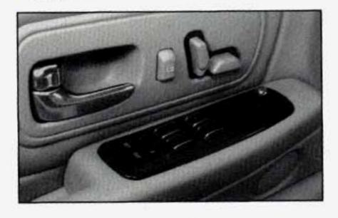
The power seat controls, located on the front doors, move and adjust the angle of the seat.
