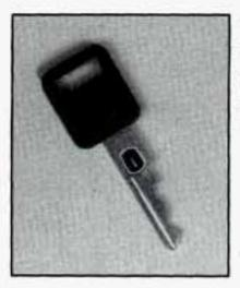
The square key is for the ignition only. It has a resistor pellet which is part of the vehicle's PASS-Key®II system.
