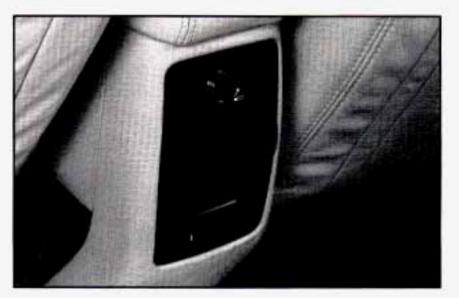
The direction of airflow to the rear seats can be adjusted if you have the optional full console (DeVille Concours Only). Move the fan lever to adjust the blower speed from LO to HI. Move the vent lever to direct the airflow.
