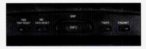
INFO RESET: Pressing this button will reset the MPG AVG, GAL FUEL USED, AVG MPH and OIL LIFE LEFT. Pressing INFO RESET when a non-resettable display appears will cause a "recall" mode to occur. When this happens, all Driver Information Center (DIC) warning messages that have been displayed since the ignition key was turned to RUN will redisplay. If no messages were displayed, a MONITORED SYSTEMS OK message will appear.
