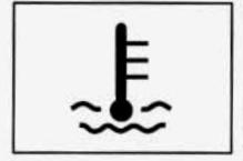
This light tells you that your engine has overheated. You should stop your vehicle and turn the engine off as soon as possible. A warning chime should also sound if this light comes on.
