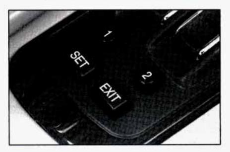
Automatic seat and mirror movement will occur if the Remote Keyless Entry (RKE) transmitter is used to enter the vehicle. The number on the back of the transmitter corresponds to the 1 or 2 seat and mirror position.
