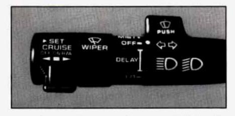
With cruise control, you can maintain a speed of about 25 mph (40 km/h) or more without keeping your foot on the accelerator. This can help on long trips. Cruise control does not work at speeds below 25 mph (40 km/h).
