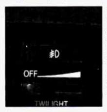
Use the fog lamps for better vision in foggy or misty conditions. When you press the fog lamp button, a small indicator light will tell you that the fog lamps and the parking lamps are on. Press the button again to turn them off.
