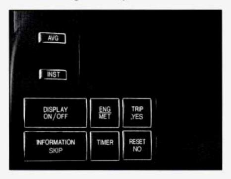
DISPLAY ON/OFF: Pressing this button will turn off the Driver Information Center (DIC), Electronic Climate Control (ECC), fuel data center, the fuel gage, trip odometer and odometer. While the displays are off, pressing the INFORMATION button will only turn on the DIC. If the TRIP button is pressed or the fuel level falls below 4 gallons (15.2 L), all of the displays will come back on.
