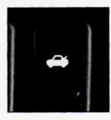
To use this feature, your vehicle must be in PARK (P) and the valet lockout button must be off. Press the trunk release button, located on the headlamp control panel on the left side of the instrument panel, to open the trunk.
