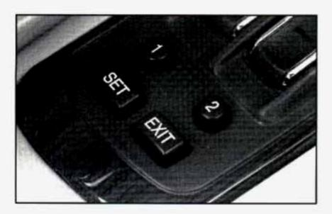
To begin programming, adjust the driver's seat (including lumbar adjustments) and both outside mirrors to a comfortable position and then press the SET button. Within five seconds, press button "1."
