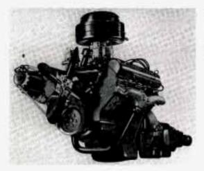
1949 Overhead Valve High Compression V8 Engine
