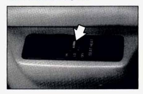
The control is located on the outboard side of each front seat. Move the SEAT HEAT control to either LO or HI to turn on the heating elements in the seat. The LO setting warms the seatback and cushion until the seat approximates body temperature. The HI setting heats the seat to a slightly higher temperature. A telltale light in the control reminds you that the heating system is in use. The heated seats can only be used when the ignition is turned on.
