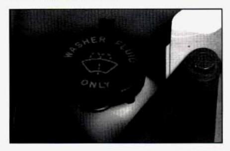
The windshield washer fluid reservoir is located next to the air cleaner on the driver's side of the engine.
