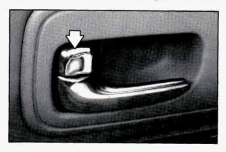
Rotate the manual lock lever forward to lock the door from the inside. To unlock the door, rotate the lever rearward.
