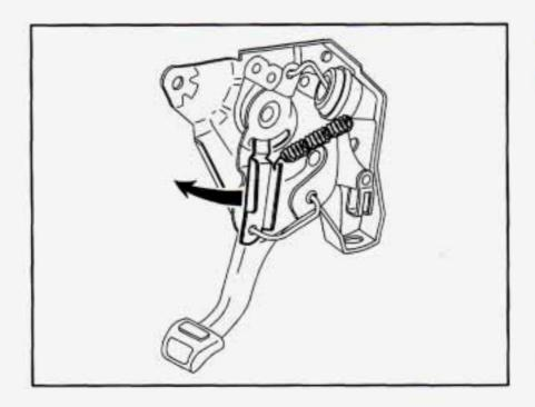
Before releasing the manual parking brake, be sure to put the vehicle in PARK (P) and turn the ignition to OFF.
