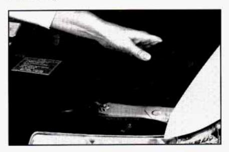
To access the headlamps, lift the cover as shown.
