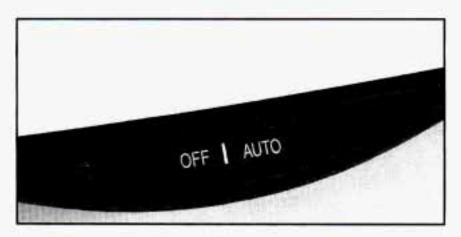
To turn on the automatic dimming feature, press AUTO. To turn off automatic dimming, press OFF. The green indicator light will be illuminated when this feature is active.
