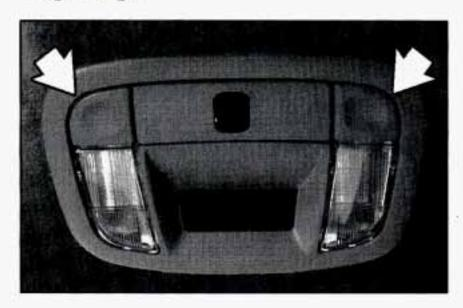
These lamps are located in the front overhead panel.
