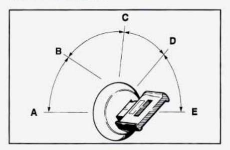
With the ignition key in the ignition switch, you can turn the switch to five different positions.
