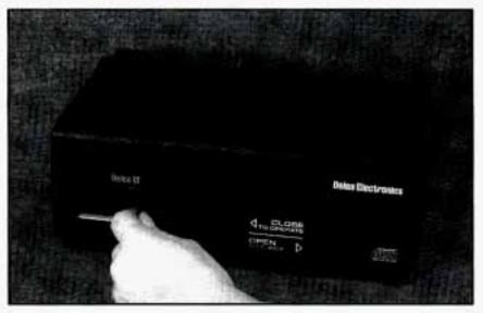
Once you have loaded the discs in the magazine, slide open the door of the compact disc (CD) changer. Push the magazine into the changer in the direction of the arrow marked on top of the magazine. Close the door by sliding it all the way to the left.
