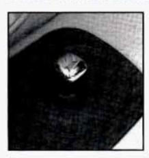
The control on the driver's door armrest operates both outside rearview mirrors. Rotate the control knob to choose the right or left mirror. To adjust the mirror, push the control knob in the direction you want the mirror to go. Adjust each mirror so you can see the side of your vehicle and the area behind your vehicle.
