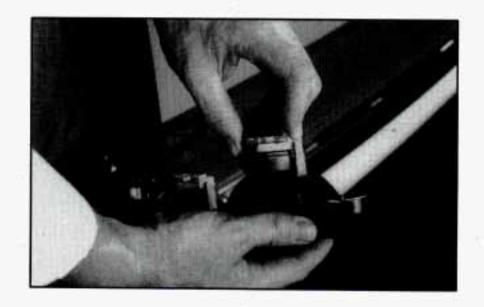
Press the bulb socket housing lever and rotate the socket to the left to remove it.
