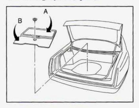
If equipped, the trunk storage system can be used to organize many different items inside the trunk. The cover (A) is located on top of the spare tire cover (B).
