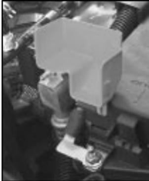
5. Lift and move the red positive (+) terminal cover away from the relay center.
