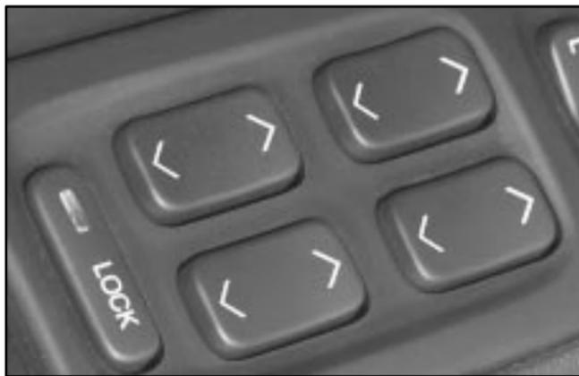
The power window controls are located on the armrest near each window. Press the up or down arrows on the controls to raise or lower windows.
