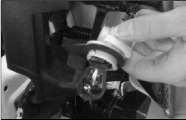
3. Remove the turn signal lamp housing socket and replace the bulb.
