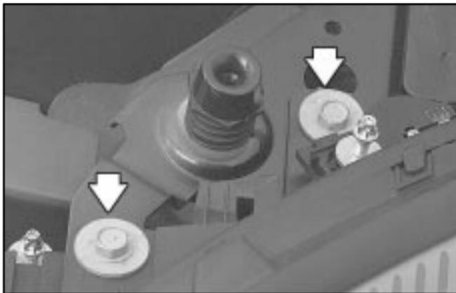
2. Remove the two bolts at the top of the headlamp assembly.
