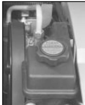
The power steering fluid reservoir is located between the fuse block relay center and the engine on the passenger's side of the vehicle.
