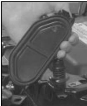
5. Remove the bulb socket dust cover and set aside.
