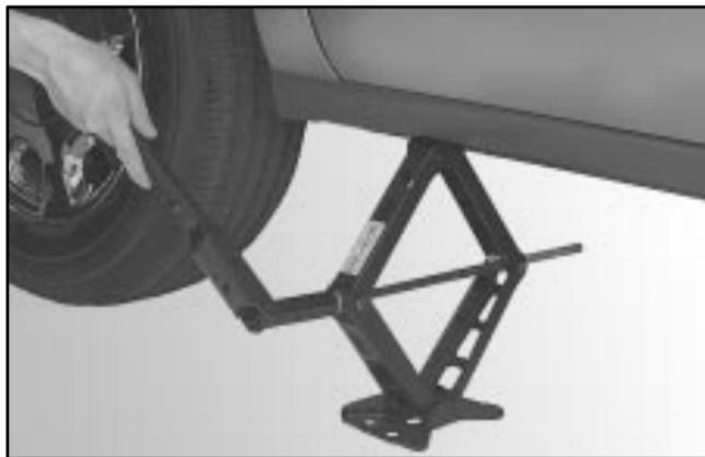
6. Raise the vehicle by turning the jack handle clockwise. Raise the vehicle far enough off the ground for the spare tire to fit under the vehicle.
