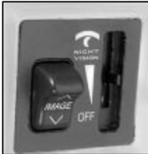
The controls are located to the left of and below the steering wheel. They are used to adjust the brightness and location of the image. Adjust the IMAGE control so the image is as low as possible while remaining visible.
