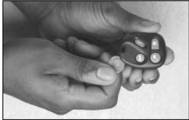
1. Use the round end of the door key or a coin to pry open the transmitter.
