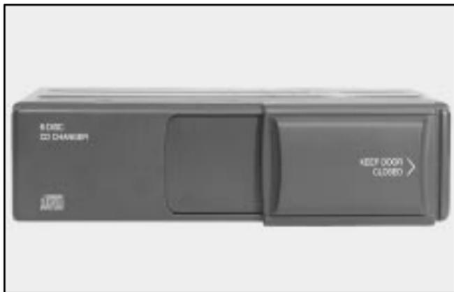
You must first load the magazine with discs before you can play a compact disc. Each of the 6 trays holds one disc. Load the trays from bottom to top, placing a disc in the tray label side up. If you load a disc label side down, the disc will not play and an error will occur. Repeat this procedure for loading up to 6 discs in the magazine.
