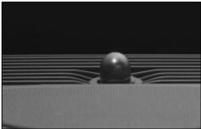
The sensor monitors the sun's solar radiation and is located on top of the instrument panel near the windshield. The ECC panel uses this information to automatically make the necessary temperature and airflow adjustments to maintain your comfort.
