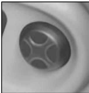
If your vehicle has this feature, the driver's and passenger's seatback lumbar support can be adjusted four ways by moving the single switch located on the side of the seat.
