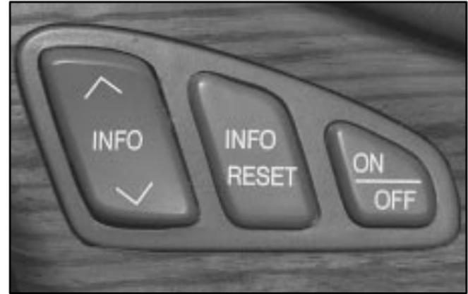
**INFO:** Pressing this button up or down will display the MILES RANGE (Analog Cluster), MPG AVG, MPG INST, GAL FUEL USED, AVG MPH, TIMER, BATTERY VOLTS, RPM TACHOMETER (Digital Cluster), ENGINE OIL LIFE, TRANS FLUID LIFE, PHONE (If Equipped), FEATURE PROGRAMMING and Blank Display.
