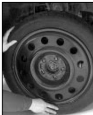
9. Place the spare tire on the wheel-mounting surface.
