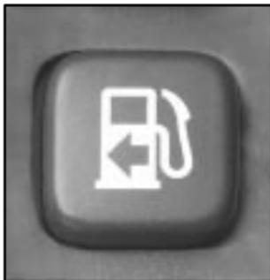
The fuel door release button is located to the left of the steering wheel next to the headlamp knob.
