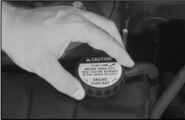
1. You can remove the coolant surge tank pressure cap when the cooling system, including the coolant surge tank pressure cap and upper radiator hose, is no longer hot. Turn the pressure cap slowly counterclockwise (left) until it first stops. (Don't press down while turning the pressure cap.)
