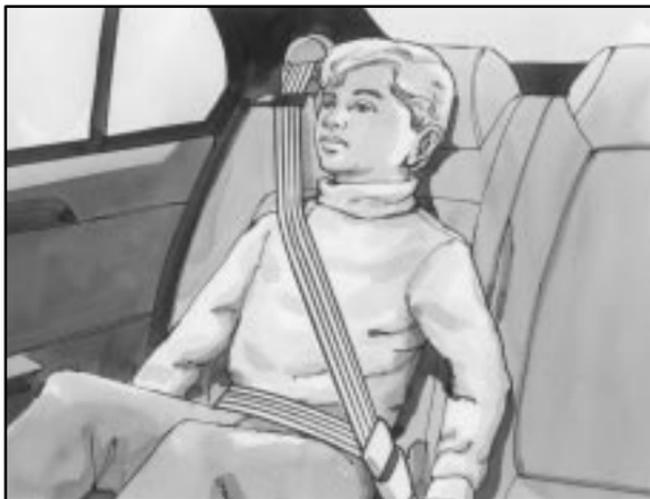
4. Buckle, position and release the safety belt as described in “Rear Seat Passenger Positions” earlier in this section. Make sure that the shoulder belt crosses the shoulder.
