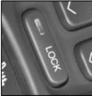
Pressing this button down will disable the rear window controls and cause the button to light, indicating that the feature is in use. To restore power to the rear windows, press the button again.
