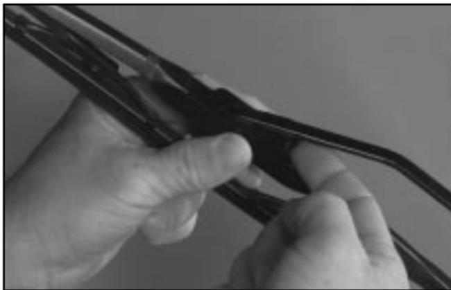
2. Tip the blade up almost to a “T” position and push down on the tab to release the wiper blade assembly.
