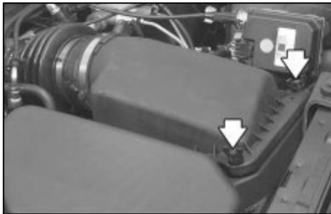
1. Loosen both wing nuts on the top of the air cleaner assembly.
