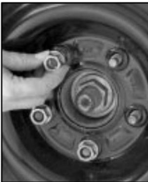
10. Replace the wheel nuts with the rounded end of the nuts toward the wheel. Tighten each nut by hand until the wheel is held against the hub.
