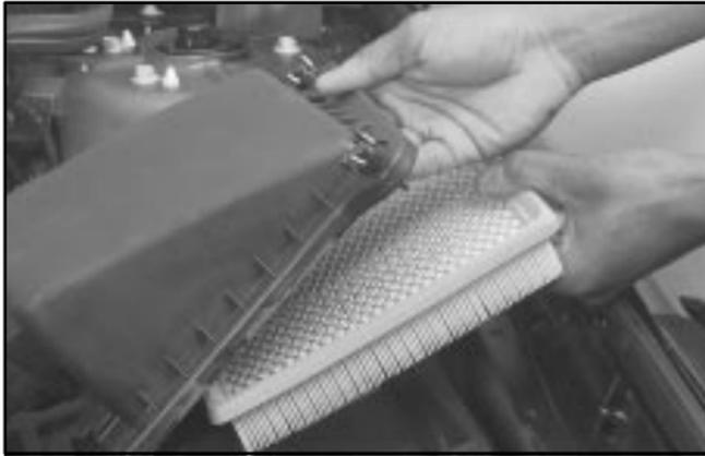
3. Remove the air filter element and any loose debris that may be found laying in the air cleaner base.
