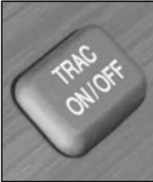
To turn the system off, press the button located on the center console. (For vehicles with a column shifter, the button is located at the end of the shift lever.)
