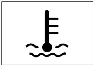
This light tells you that your engine has overheated. You should stop your vehicle and turn the engine off as soon as possible. A warning chime should also sound if this light comes on.
