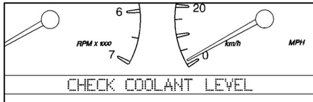
If the CHECK COOLANT LEVEL message comes on and stays on, it means you're low on engine coolant.
