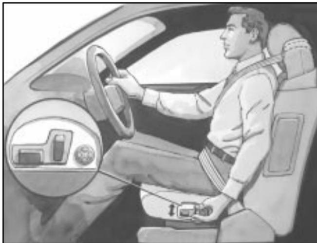
To move it down, press down on the power seat recline control and move the height adjuster to the desired position. You can move the adjuster up just by pushing up on the power seat recline control. After you move the adjuster to where you want it, try to move it down without pushing the power seat recline control to make sure it has locked into position.
