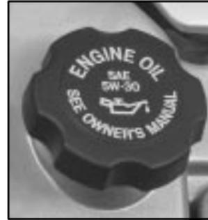
The oil fill cap is located behind the radiator on the passenger's side of the engine. Turn the cap counterclockwise to remove it.
