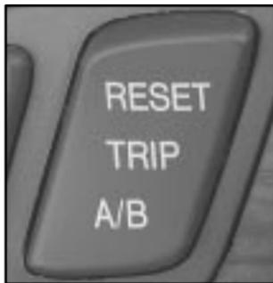
Press this button, to tell how far you've traveled since you last set the trip odometer back to zero.
