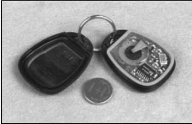
3. Replace the battery. Insert the new battery as the instructions under the cover indicate.
