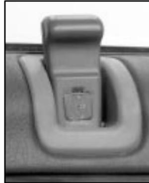
Push down on the manual lock button to lock the door from the inside. To unlock the door, pull up on the button.
