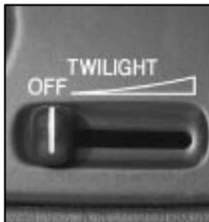
This control is next to the headlamp knob. It automatically switches the lamps on and off by sensing how dark it is outside.
