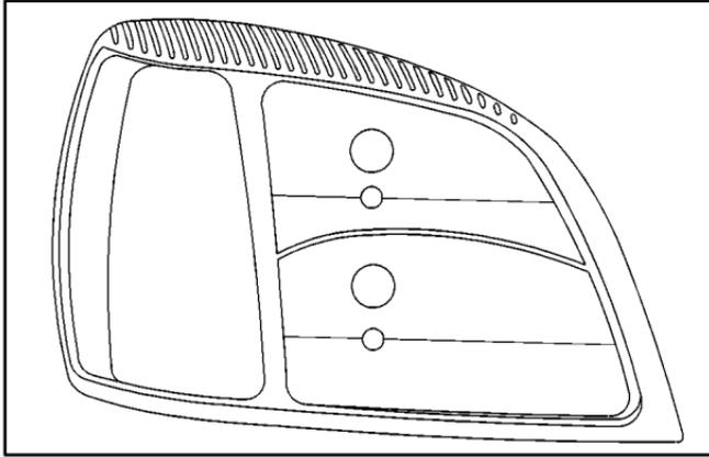
2. Measure the distance from the ground to the aim dot on each lamp; if left low beam, subtract two inches. Record this distance.
