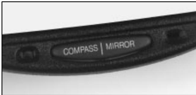
The right side of the button, located at the bottom of the mirror, turns the electrochromic mirror on and off. To turn on the automatic dimming feature, press **MIRROR**. To turn off automatic dimming, press **MIRROR** again. The green indicator light will be illuminated when this feature is active.
