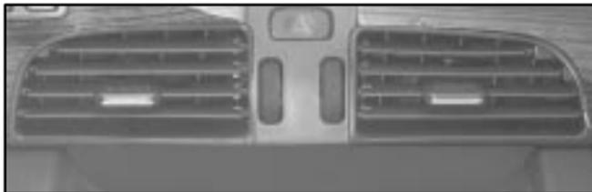
The front outlets are located in the center and at each side of the instrument panel. You can adjust the direction of airflow by moving the center control levers or you can stop the airflow by moving the lever located on each side of the outlets downward.
