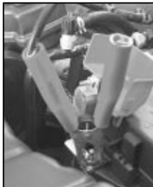
7. Connect the red positive (+) cable to the remote positive (+) terminal of your vehicle.
