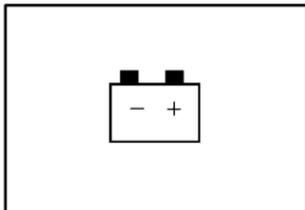
When you turn the key to ON, this light will come on briefly to show that the generator and battery charging systems are working.
