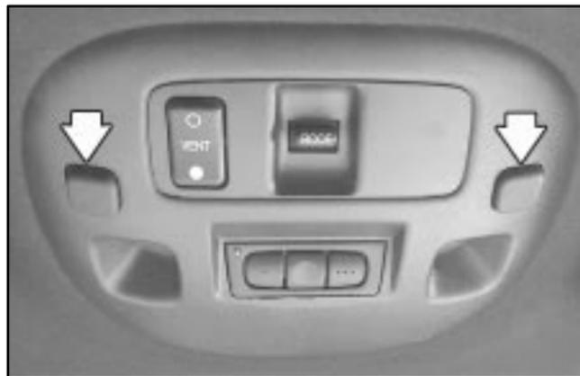
These lamps are located in the front overhead console. Press the button to turn them on. Press it again to turn them off.
