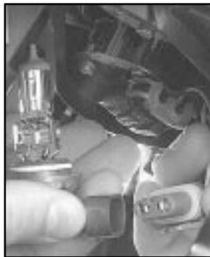
7. Disconnect the bulb from the socket by pulling out the bulb.
