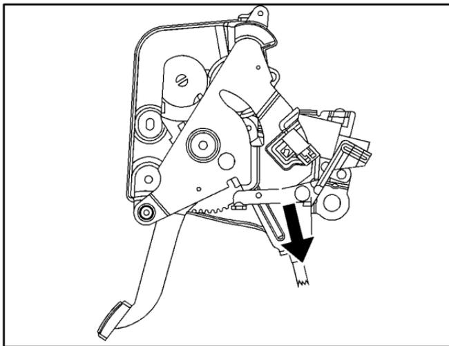
Reach under the driver's side of the instrument panel and pull on the manual release lever, which is located above the parking brake pedal. If the parking brake does not release, you should either drive to the nearest service station or have your vehicle towed.
