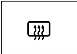
The lines you see on the rear window warm the glass. Press this button to turn on the rear defogger. With it, the rear window and both outside rearview mirrors are heated.
