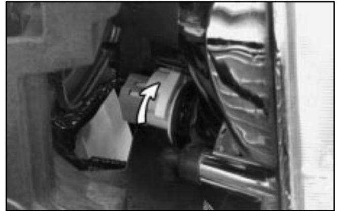
2. Press the tab down and turn the housing socket clockwise to unlock the socket from the lamp housing.
