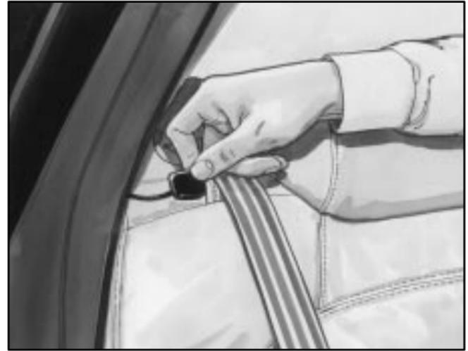
1. Remove the guide from its storage pocket on the top of the seatback.
