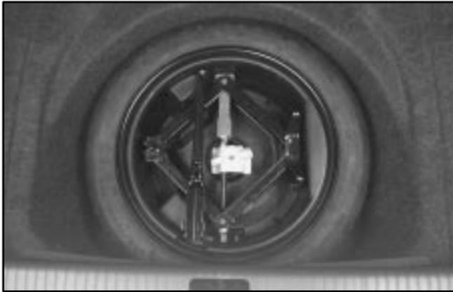
3. Unscrew the wing nuts to remove the container that holds the wrench and jack.
