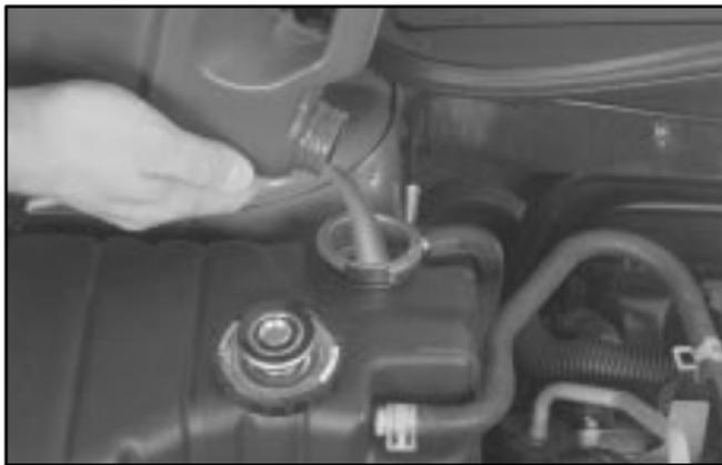
The surge tank is located on the passenger's side of the engine.
