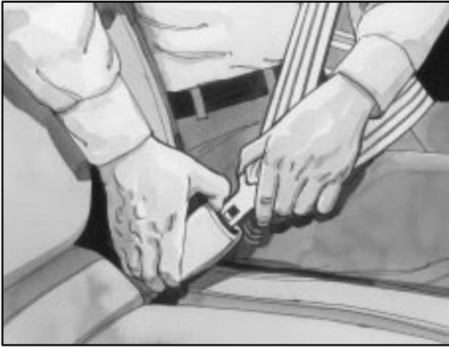
To unlash the belt, just push the button on the buckle. The belt should go back out of the way.
