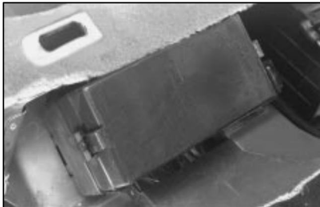
The rear BEC is located under the rear seat on the driver's side. The rear seat cushion must be removed to access the BEC. See "Removing the Rear Seat Cushion" in the Index.
