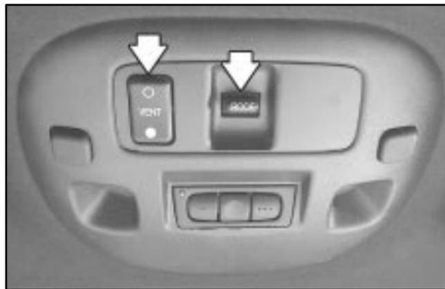
The two control switches to operate the sunroof are located on the overhead console and include VENT, open and close.
