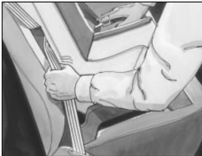
6. To tighten the belt, feed the lap belt back into the retractor while you push down on the child restraint. You may find it helpful to use your knee to push down on the child restraint as you tighten the belt.
