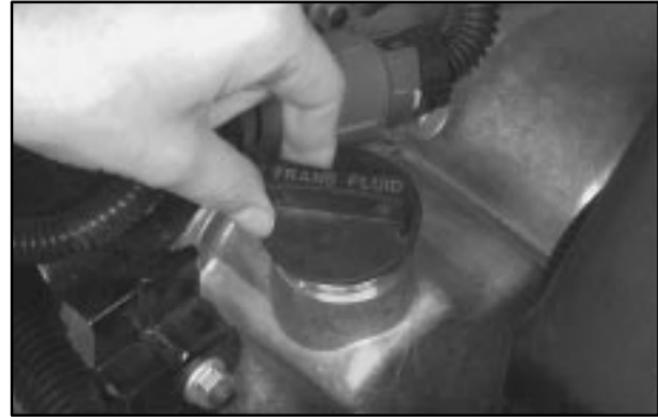
1. The transaxle fluid cap is located next to the radiator hose and below the air cleaner assembly on the driver's side of the engine. Remove the air cleaner assembly so you can reach the transaxle fluid cap. Turn the transaxle fluid cap counterclockwise to remove. Pull out the dipstick and wipe it with a clean rag or paper towel.
