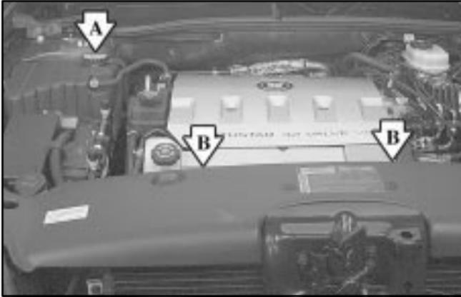
A. Coolant Surge Tank with Pressure Cap
