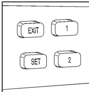
The controls for these features are located on the driver's door panel, and are used to program and recall previous settings.
