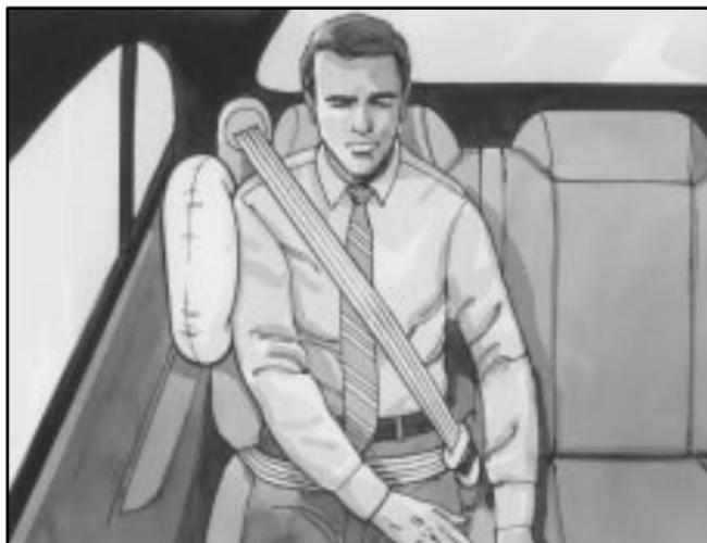
The side impact air bags for the rear seat outboard passenger positions are in the sides of the rear seatback closest to the doors.
