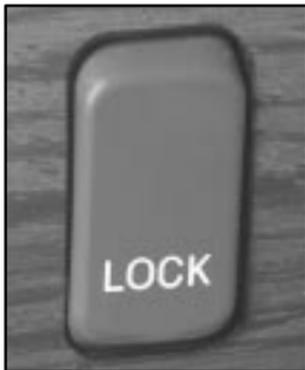
Press the power door lock button to lock or unlock all the doors at once. The power door lock buttons located on the rear doors can lock all the doors at once, but cannot unlock the doors.
