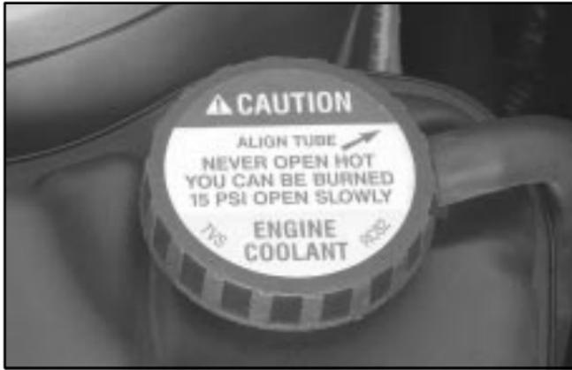
5. Then replace the pressure cap. Be sure the arrows on the pressure cap line up like this.
