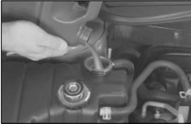
3. Then fill the coolant surge tank with the proper mixture, to the base of the filler neck.
