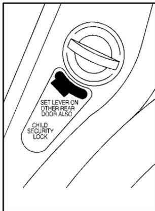
Your vehicle is equipped with rear door security locks that help prevent passengers from opening the rear doors of your vehicle from the inside.
