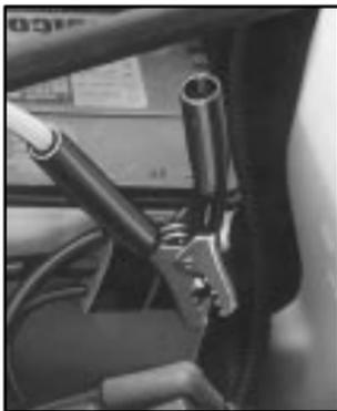
9. Now connect the black negative (-) cable to the good battery's negative (-) terminal.
