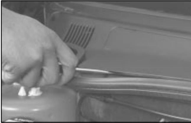
1. To access the passenger compartment air filter, insert the flat tip of a screwdriver into the outer edge of the cover and gently pry the cover up.
