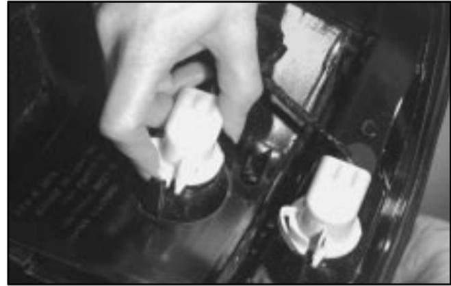
7. Press the bulb socket tab and turn the socket counterclockwise to remove it. To remove the bulb, grasp the socket firmly and pull the bulb out.
