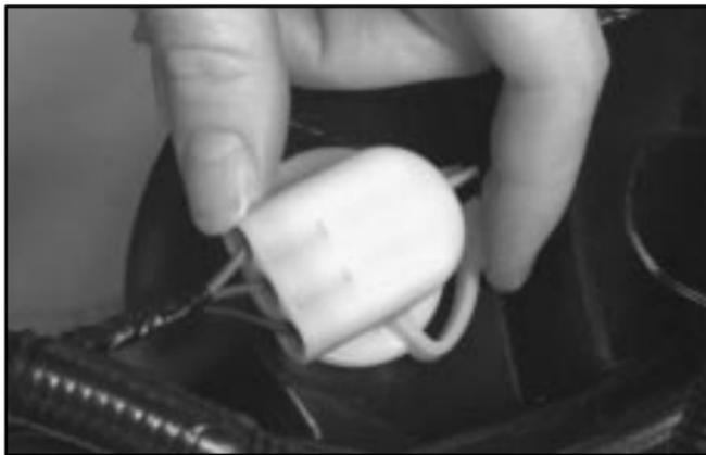
2. Press the bulb socket tab and turn the bulb socket counterclockwise to unlock the socket from the lamp housing.
