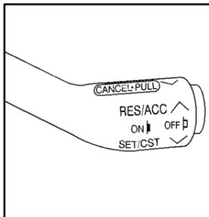
The cruise control lever is located on the lower right side of the steering column.
