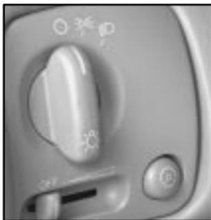
The control located on the left side of the instrument panel operates these lamp systems:
