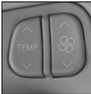
Some heating and cooling controls can be adjusted at the steering wheel. Other touch controls operate some audio controls. See “Audio Steering Wheel Controls” in the Index.
