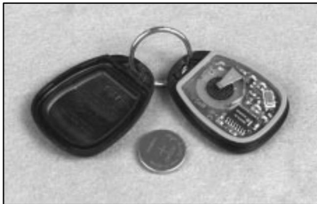
2. Once the transmitter is separated, use a pencil (or a similar object) to remove the old battery. Do not use a metal object.
