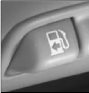
The fuel door release button is located on the left side of the instrument panel below the lamp controls.
