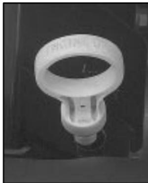
The engine oil dipstick is located directly behind the radiator. The yellow handle says ENGINE OIL on it.
