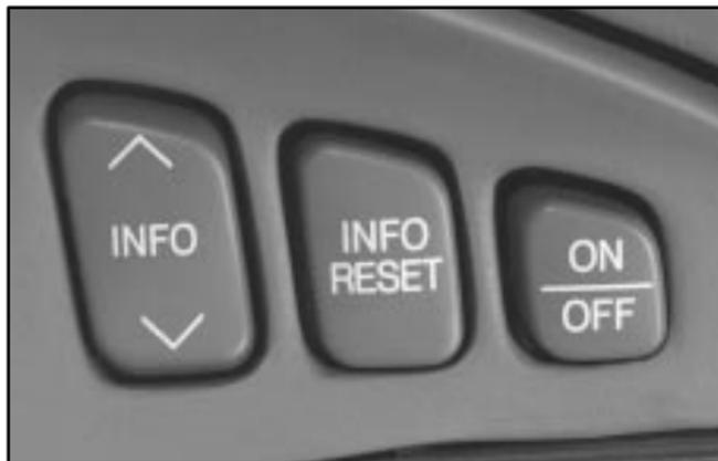
**INFO:** Pressing this button up or down will display the OUTSIDE TEMP, MILES RANGE, MPG AVG, MPG INST, GAL FUEL USED, AVG MPH, TIMER, BATTERY VOLTS OK, ENGINE OIL LIFE, TRANS FLUID LIFE, PHONE (If Equipped) and FEATURE PROGRAMMING.
