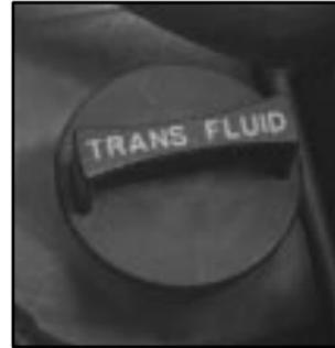
The transaxle fluid cap is located next to the radiator hose and below the air cleaner assembly on the driver's side of the engine.
