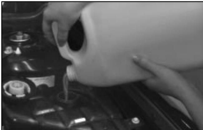
The engine coolant surge tank is located on the driver's side of the engine.
