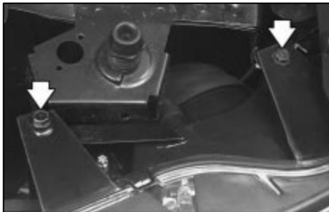
2. Remove the two bolts fastening the headlamp to the headlamp mounting bracket.
