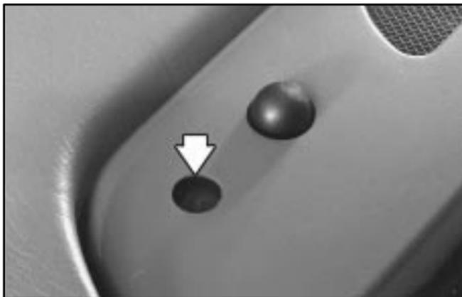
The light sensor for the Daytime Running Lamps (DRL) and the Twilight Sentinel is located on the driver's side of the front defogger grille. If you cover the sensor, it will read "dark" and the lamps will come on.
