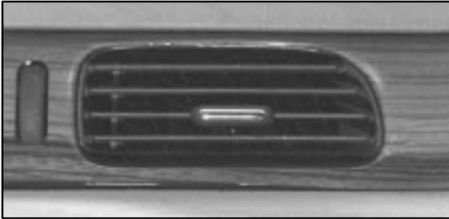
The front outlets are located in the center and at each side of the instrument panel. You can adjust the direction of airflow by moving the center control levers or you can stop the airflow by moving the control dial located on each outlet downward.
