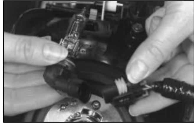
7. After removing the wiring harness connector from the headlamp bulb socket, replace the bulb assembly. Reconnect it to the wiring harness and reinstall the headlamp bulb assembly back into the headlamp housing.
