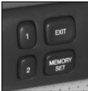
The controls for these features are located on the driver's door panel, and are used to program and recall memory settings.
