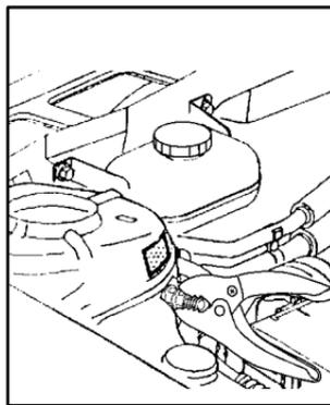
11. Attach the cable at least 18 inches (46 cm) away from the dead battery, but not near engine parts that move.
