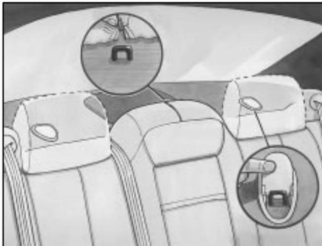
The top strap anchor for the center rear seating position is located at the top of the seat. In order to get to this bracket, you'll have to unzip the seat cover.
