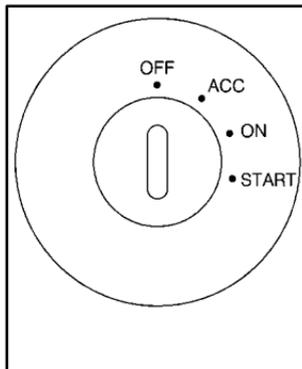
**OFF:** This position lets you turn off the engine and remove the key. This position also locks the steering wheel and transaxle.
