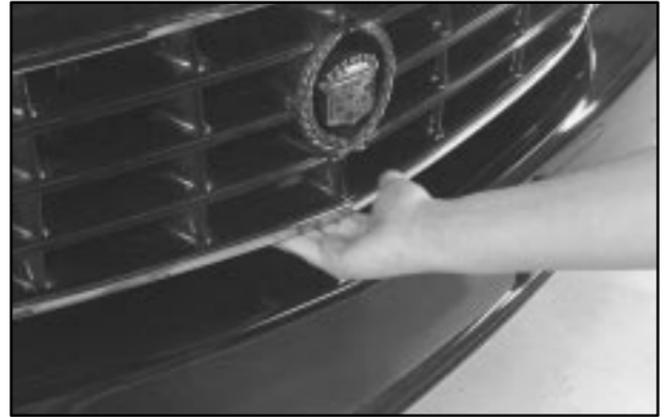
Then go to the front of the vehicle and find the secondary hood release which is located below the front grille. Move the release lever to the left as you raise the hood.
