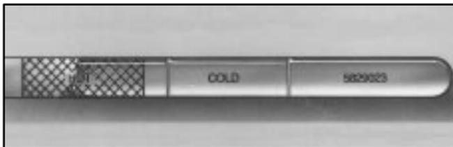
4. Check both sides of the dipstick, and read the lower level. The fluid level must be in the cross-hatched area.
