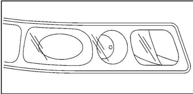
2. Measure the distance from the ground to the aim dot on each lamp. Record this distance.
