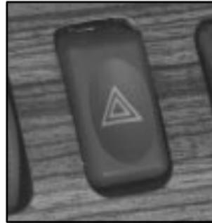
The hazard warning button is located in the center of the instrument panel, between the two air vents. Press the button in to make the front and rear turn signal lamps flash on and off.
