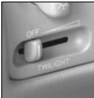
This control is located below the exterior lamps control knob. It automatically turns the lamps on and off by sensing how dark it is outside.
