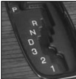
2. Move the shift lever into PARK (P) by pushing the lever all the way toward the front of your vehicle.
