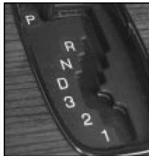
**PARK (P):** This locks the front wheels. It's the best position to use when you start the engine because your vehicle can't move easily.
