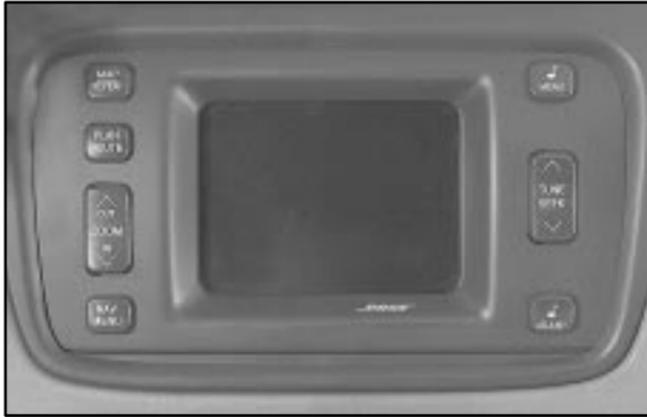
This display screen is located in the center of the instrument panel. There are eight “hard” buttons and a touch sensitive screen.
