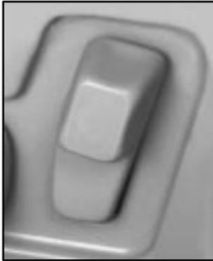
The switches to move your head restraints are located on the outboard side of each front seat.
