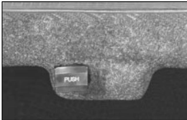
The rear seat pass-through release button is located in the trunk. To release the pass-through door, press the PUSH button located in the center of the trunk panel.
