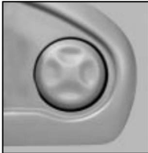
The adaptive seat control is located on the outboard side of each front seat. Use the power seat control first to get the proper position.
