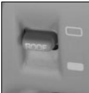
Press and hold the ROOF switch rearward to the first position to open the glass panel and sunshade. The sunshade can also be opened or closed by hand. To close the glass panel, press and hold the ROOF switch forward.
