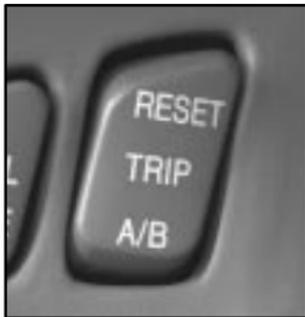
By pressing the bottom of this button, you can tell how many miles you have traveled on either your Trip A or Trip B odometer since you last set the odometer back to zero.
