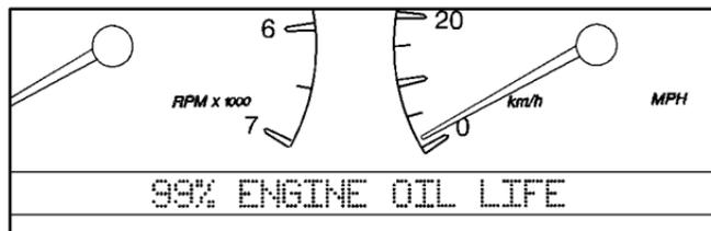
This feature lets you know when to change the engine oil. It's based on the engine oil temperatures and your driving patterns. To see the display, press the INFO button several times until ENGINE OIL LIFE appears. If you see 99% ENGINE OIL LIFE, 99 percent of your current oil life remains.
