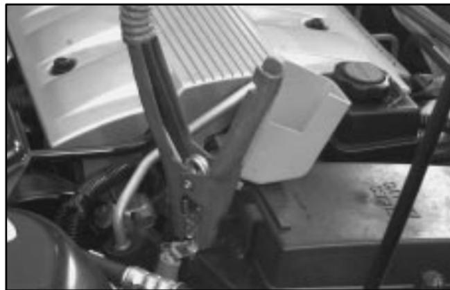
8. Connect the red positive (+) cable to the remote positive (+) terminal of the vehicle with the dead battery.
