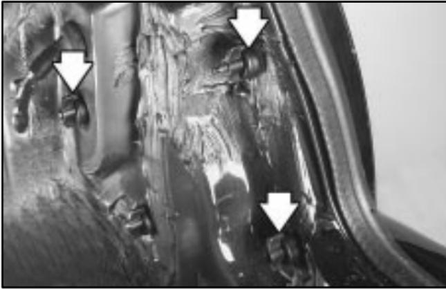
5. Remove the three wing nuts that fasten the taillamp to the body.
