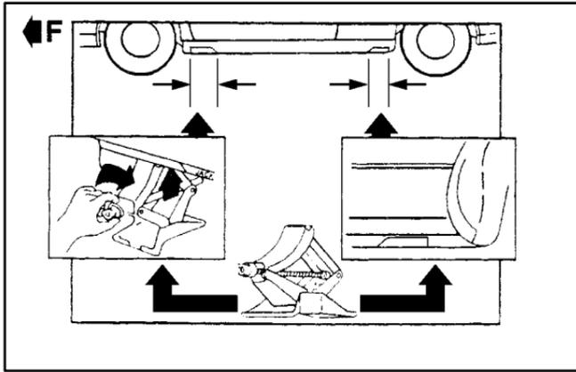
2. Find the jacking location from the diagrams above and corresponding cutouts in the plastic molding.
