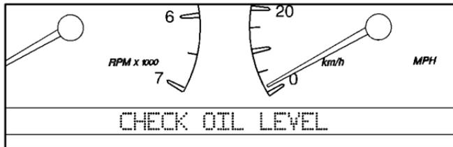
A CHECK OIL LEVEL message will appear when the engine oil is approximately 1 quart (1L) low. If the message is displayed, check the dipstick level and add oil as needed.
