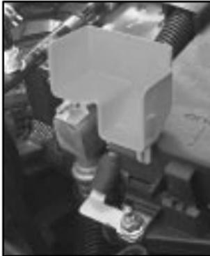
6. Start by lifting and moving the red positive (+) remote terminal cover away from the relay center.
