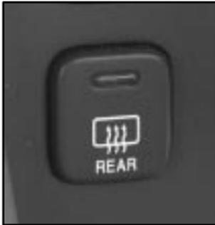
The grid lines you see on the rear window warm the glass. Press this button to turn on the rear defogger.
