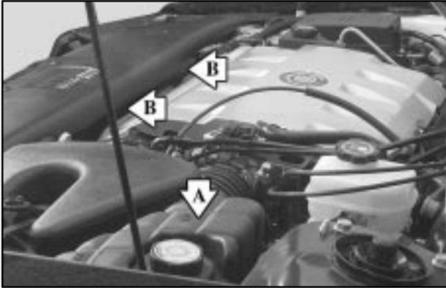
A. Coolant Surge Tank with Pressure Cap
