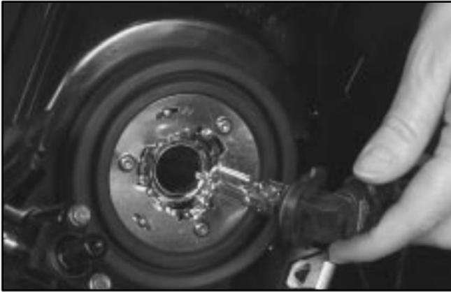
6. Remove the headlamp bulb socket.
