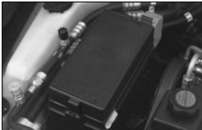
The front Bussed Electrical Center (BEC) is located in the front of the engine compartment between the windshield washer fluid reservoir and the power steering fluid reservoir (on the passenger's side). Lift the cover to gain access.
