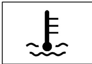
This light tells you that the engine has overheated. You should stop the car and turn the engine off as soon as possible.
