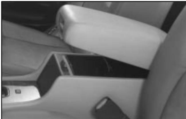
The center console comes with a storage tray, a storage compartment for CDs or tapes, a dual cupholder that unfolds, a coinholder, an optional phone and an armrest. The cupholder can be opened by pressing on the surface panel located in front of the armrest and unfolding it. Close the lid to secure.
