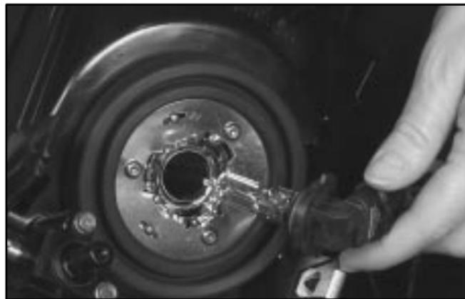
6. Remove the headlamp bulb socket.
