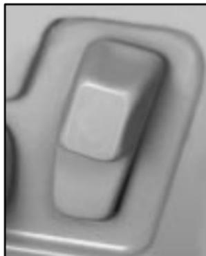
The reclining front seatback controls are located on the outboard side of each front seat.
