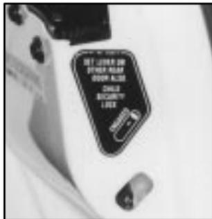
Your vehicle is equipped with rear door security locks that help prevent passengers from opening the rear doors of your vehicle from the inside. The locks are located on the inside edge of each rear door.
