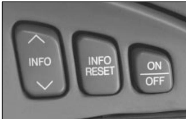
**INFO:** Pressing this button up or down will display the OUTSIDE TEMP, MILES RANGE, MPG AVG, MPG INST, GAL FUEL USED, AVG MPH, TIMER, BATTERY VOLTS, ENGINE OIL LIFE, TRANS FLUID LIFE, PHONE (Option) and FEATURE PROGRAMMING.
