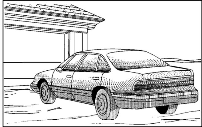
4. Turn on the low beam headlamps and place a piece of cardboard or equivalent in front of the headlamp not being aimed. This should allow the beam cut-off of the headlamp being aimed to be seen on the flat surface.
