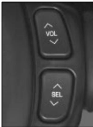
Some audio controls can be adjusted at the steering wheel. They include the following:
