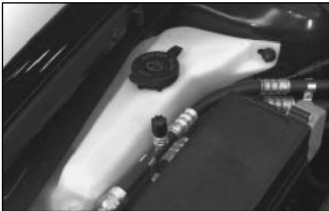
The windshield washer fluid reservoir is located next to the fuse relay center on the passenger's side of the engine. See "Engine Compartment Overview" in the Index for more information on location.
