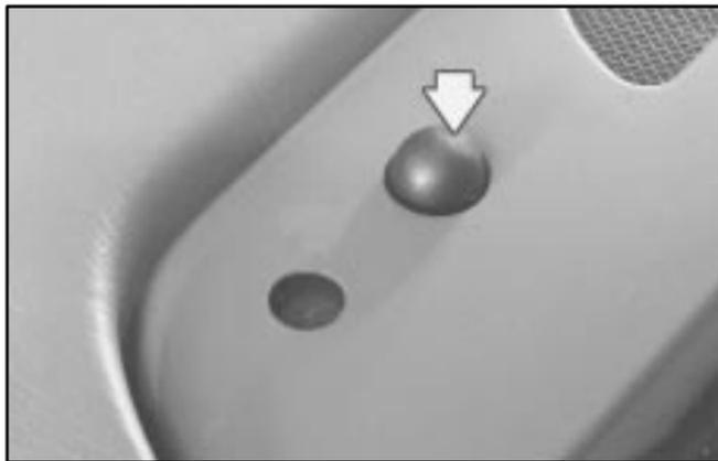
The sensor monitors the sun's solar radiation and is located near the end of the instrument panel near the windshield.
