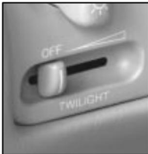
This lever is located below the exterior lamps control knob. It automatically turns the lamps on and off by sensing how dark it is outside.
