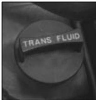
The transaxle fluid cap is located next to the radiator hose and below the engine air cleaner/filter assembly on the driver's side of the engine. See "Engine Compartment Overview" in the Index for more information on location.
