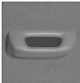
The URPA display is located inside the vehicle, above the rear window. It has three color-coded lights that can be seen through the rearview mirror or by turning around.
