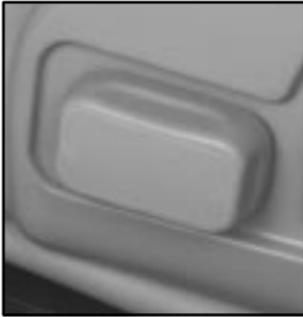
The power seat controls are located on the outboard side of the front seat cushions.
