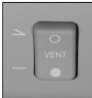
To vent the sunroof, press and hold the upper part of the VENT switch. The sunshade must be opened by hand. To close, press and hold the lower part of the VENT switch.
