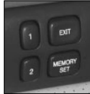
The controls for these features are located on the driver's door panel, and are used to program and recall memory settings for the driver's seating positions.
