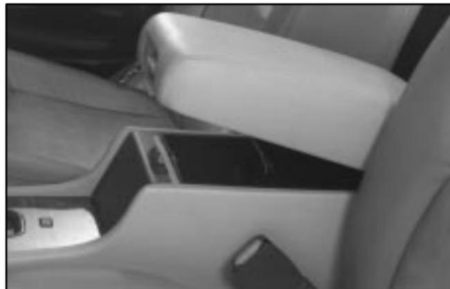
The center console comes with a storage tray, a storage compartment for CDs or tapes, a dual cupholder that unfolds, a coinholder, an optional phone and an armrest. The cupholder can be opened by pressing on the surface panel located in front of the armrest and unfolding it. Close the lid to secure it.
