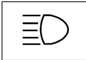
This light on the instrument panel cluster will be on, indicating high-beam usage.
