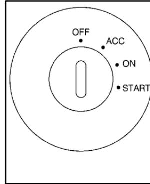
With the key in the ignition switch located on the instrument panel, you can turn the key to four different positions:
