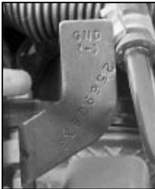
Your vehicle has a remote negative (-) terminal, marked "GND (-)" located near the power steering fluid reservoir. Attach the cable to the remote negative terminal provided.
