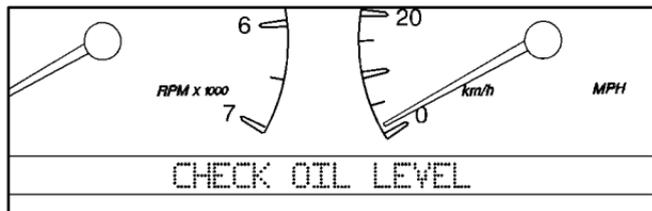
If the CHECK OIL LEVEL Message appears on the instrument panel, it means you need to check your engine oil level right away. For more information, see “CHECK OIL LEVEL message” in the Index.
