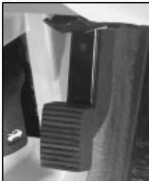
Hold the regular brake pedal down with your right foot and push the parking brake pedal down with your left foot to set the parking brake. If the ignition is on, the BRAKE indicator light should come on. If it doesn't, you need to have your vehicle serviced.
