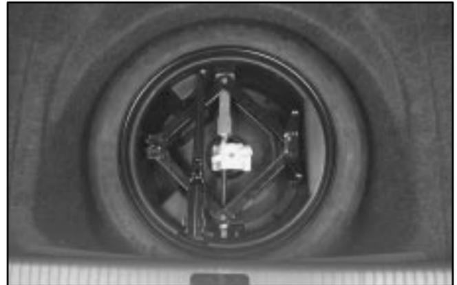
2. Unscrew the wing nuts to remove the container that holds the wrench and jack.
