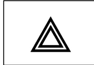
This light located on the instrument panel cluster will flash, indicating that the hazard warning flashers are on.
