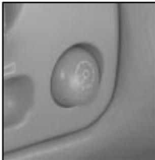
The button is located to the right of the Twilight Sentinel control. Push the button in to release it to the outward position.
