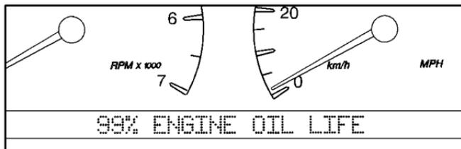
This feature lets you know when to change the engine oil. It's based on the engine oil temperatures and your driving patterns. To see the display, press the INFO button several times until ENGINE OIL LIFE appears.
