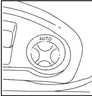
The adaptive seat control is located on the outboard side of the driver's seat. Use the power seat control first to get the proper position.
