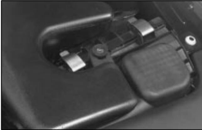
The air cleaner is located next to the coolant surge tank on the driver's side of the engine. See "Engine Compartment Overview" in the Index for more information on location. Be sure the engine has cooled before following these steps to replace the air cleaner filter:
