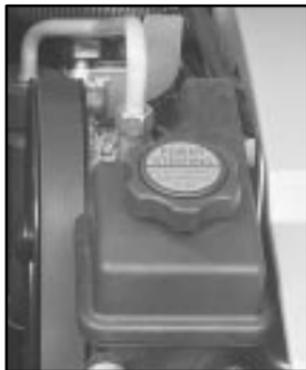
The power steering fluid reservoir is located next to the fuse relay center on the passenger's side of the engine.
