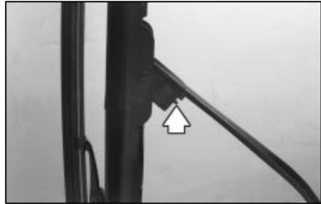
2. Press the tab that holds the wiper blade to the arm.
