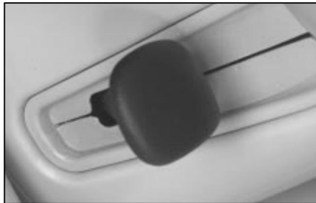
The tilt wheel control is located on the outboard side of the steering column.
