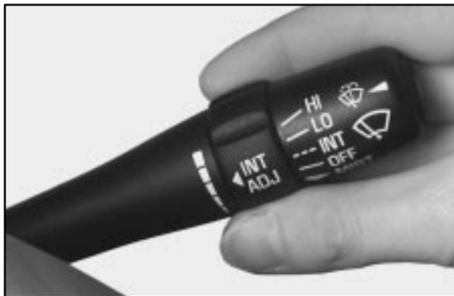
You can control the windshield wipers by moving the lever with the wiper symbol on it. This lever is located on the right side of your steering column. For information on wiper-activated headlamp operation, refer to “Wiper-Activated Headlamps” in the Index.
