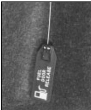
An alternate fuel door release is located inside of the trunk on the driver's side. Pull it to release the fuel door.
