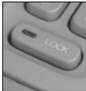
Press the LOCK button down to disable the rear passenger's window switches. A light on the button will illuminate to indicate that the rear window switches are disabled.
