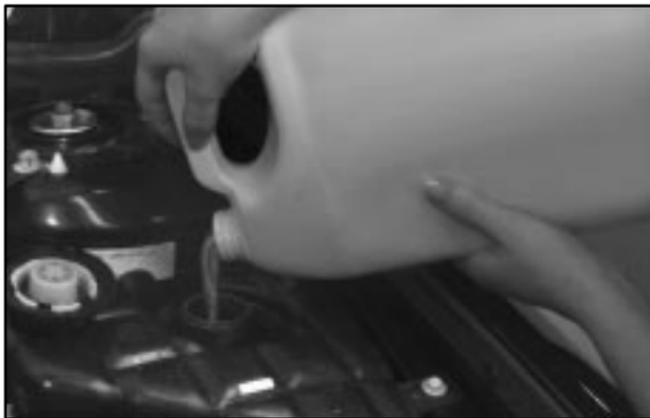
The engine coolant surge tank is located on the driver's side of the engine. See "Engine Compartment Overview" in the Index for more information on location.
