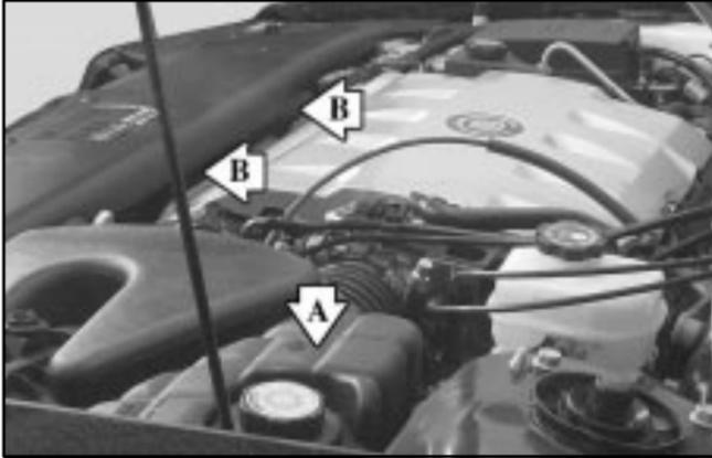
A. Coolant Surge Tank with Pressure Cap
