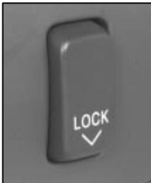
Press the down arrow (LOCK) on the power door lock switch located on either front door to lock all of the doors at once. Press the top of the switch to unlock all of the doors at once.
