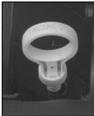
The engine oil dipstick is located directly behind the radiator. The yellow handle says ENGINE OIL on it. See “Engine Compartment Overview” in the Index for more information on location.
