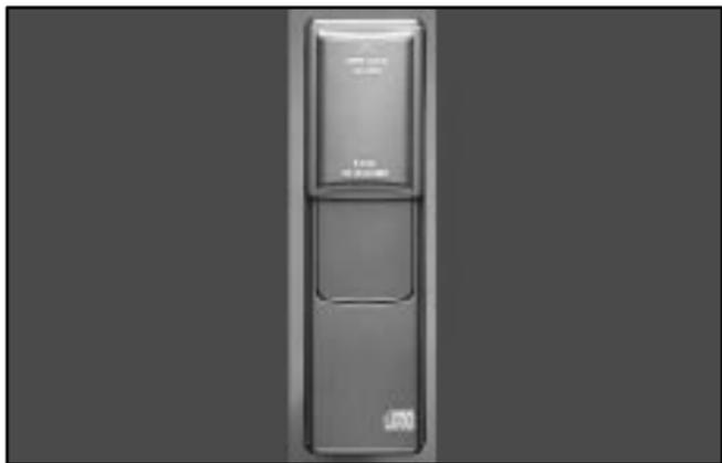
With the compact disc changer, you can play up to six discs continuously. Normal size discs may be played using the slots supplied in the magazine.
