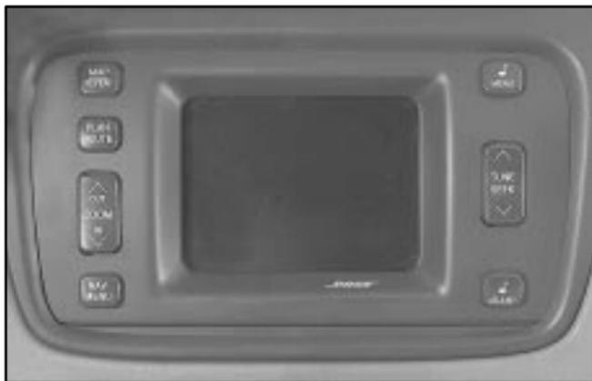
This display screen is located in the center of the instrument panel. There are seven “hard” buttons and a touch sensitive screen.
