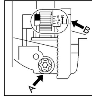
Once the horizontal aim is adjusted, then adjust the vertical aim.
