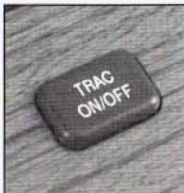
To turn the system off, press the TRAC ON/OFF button located on the center console.
