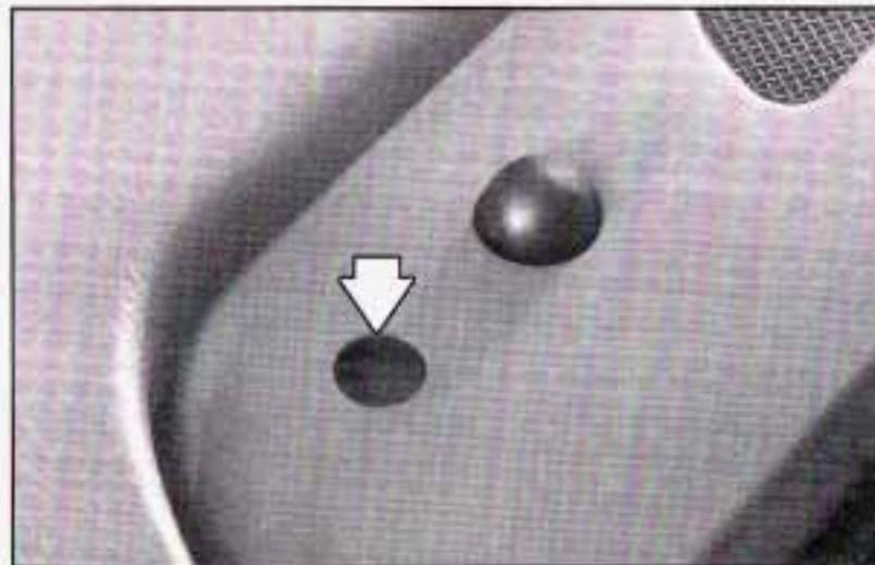
The light sensor for the Daytime Running Lamps (DRL) and the Twilight Sentinel® is located on the driver's side of the front defogger grille.
