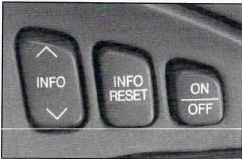
The Driver Information Center (DIC) buttons are located to the right of the steering wheel on the instrument panel, near the air outlets.
