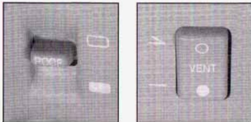
The two switches that operate the optional sunroof are located on the overhead console and include VENT, ROOF, open and close.
