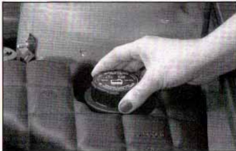
1. Park the vehicle on a level surface. You can remove the coolant surge tank pressure cap when the cooling system, including the coolant surge tank pressure cap and upper radiator hose, is no longer hot. Turn the pressure cap slowly counterclockwise (left) about one-quarter turn and then stop.
