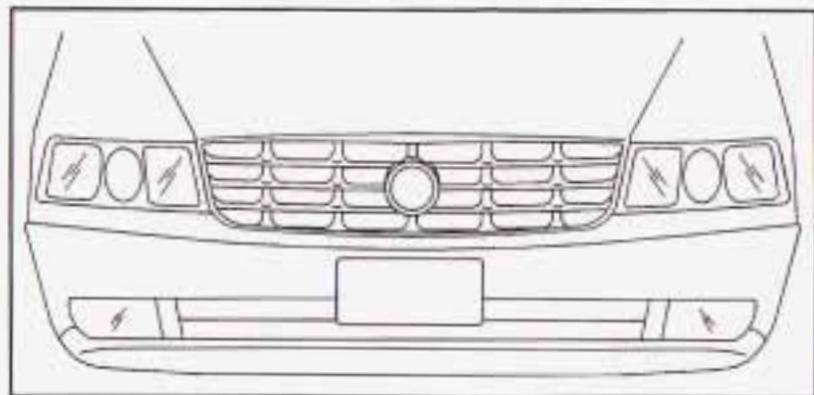
Your vehicle has a visual optical headlamp aiming system equipped with horizontal aim indicators. The aim has been preset at the factory and should need no further adjustment. This is true even though your horizontal aim indicators may not fall exactly on the "0" (zero) marks on their scales.
