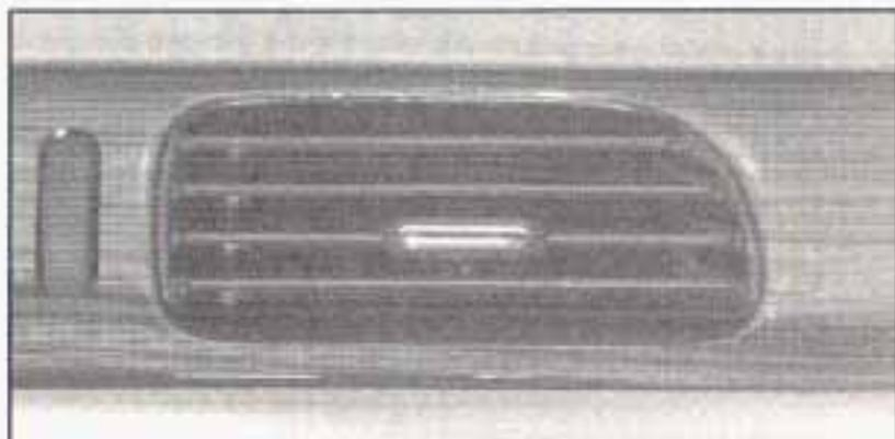
Use the levers located in the center of each outlet to change the direction of the airflow. Use the thumbwheels to open or close the outlets.
