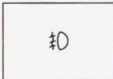
This light will come on when the fog lamps are in use. It will go out when the fog lamps are turned off.
