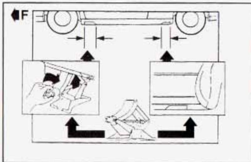
2. Find the jacking location from the diagram above and corresponding hoisting notches located in the plastic molding. The front location is 9.0 inches (23 cm) from the rear edge of the front wheel well, and the rear location is 2.5 inches (7 cm) from the front edge of the rear wheel well.
