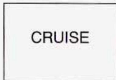
This light comes on whenever the cruise control system is in use. It will go out when the system is turned off.
