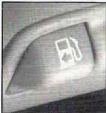
The fuel door release button is located on the left side of the instrument panel below the exterior lamp control.
