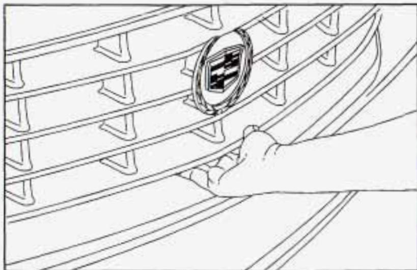
2. Then go to the front of the vehicle and find the secondary hood release which is located below the front grille.
