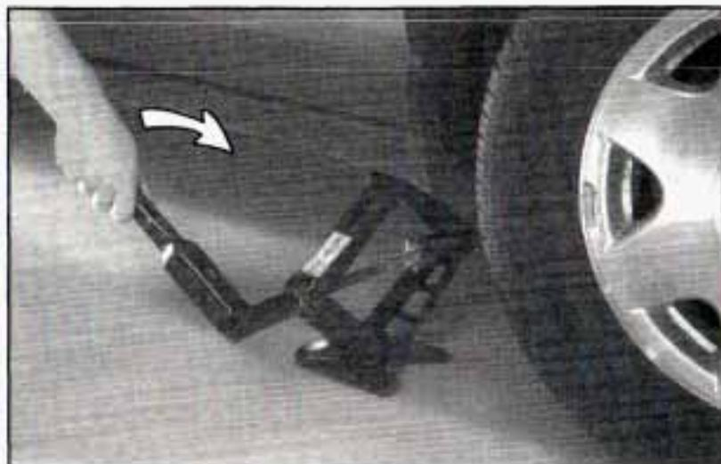
6. Raise the vehicle by turning the jack handle clockwise. Raise the vehicle far enough off the ground for the compact spare tire to fit under the vehicle.
