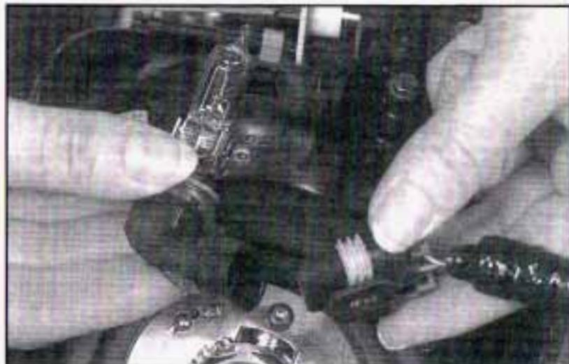
8. After removing the wiring harness connector from the headlamp bulb socket, replace the bulb assembly. Reconnect it to the wiring harness and reinstall the headlamp bulb assembly back into the headlamp housing.
