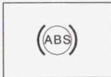
With the anti-lock brake system, the light(s) will come on when your engine is started and may stay on for several seconds. That's normal.
