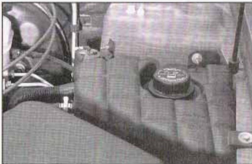
A low coolant level should be indicated by a CHECK COOLANT LEVEL message on the Driver Information Center. If it is, you may have a leak at the pressure cap or in the radiator hoses, heater hoses, radiator, water pump or somewhere else in the cooling system.
