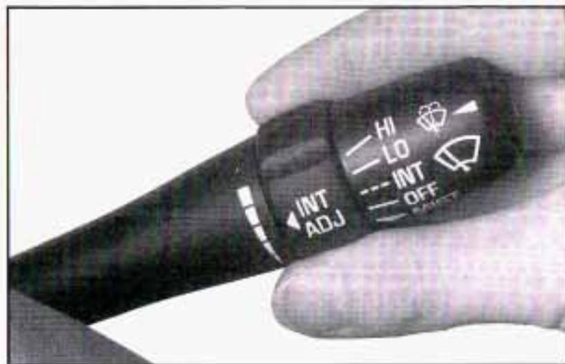
You can control the windshield wipers by moving the lever with the wiper symbol on it. This lever is located on the right side of your steering column. For information on wiper-activated headlamp operation, refer to *Exterior Lamps* on page 3-15.
