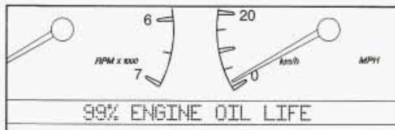
This feature lets you know when to change the engine oil. It's based on the engine oil temperatures and your driving patterns.
