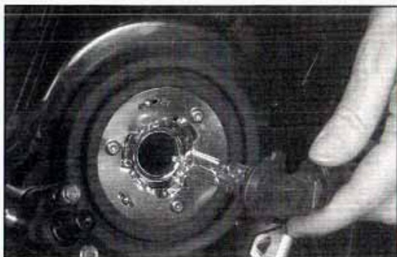
7. Remove the headlamp bulb socket.
