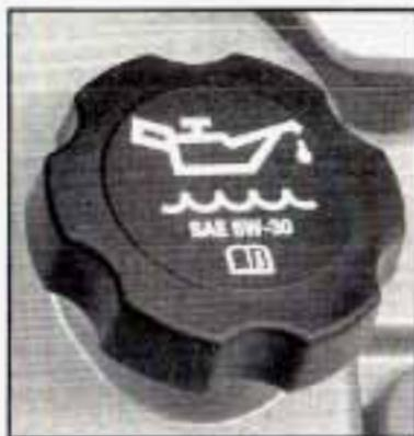
The engine oil fill cap is located behind the radiator on the passenger's side of the vehicle. For more information on location, see *Engine Compartment Overview on page 5-14*.
