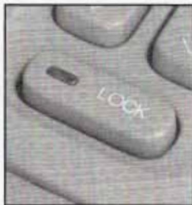
The rear window lockout button is located on the driver's door armrest next to the window switches.
