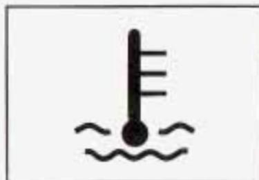
This light tells you that your engine has overheated. As a check, the light should come on for a few seconds when you start your engine.
