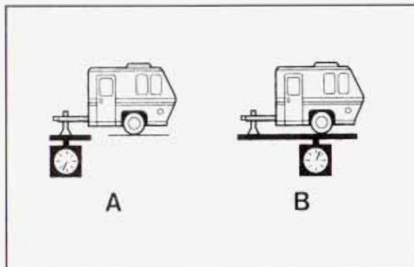
If you're using a weight-carrying hitch or a weight-distributing hitch, the trailer tongue (A) should weigh 10–15 percent of the total loaded trailer weight (B). After you've loaded your trailer, weigh the trailer and then the tongue, separately, to see if the weights are proper. If they aren't, you may be able to get them right simply by moving some items around in the trailer.
