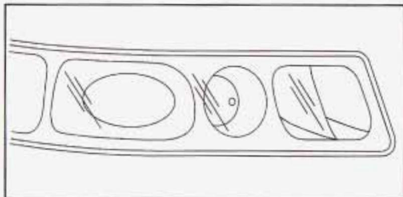
2. Measure the distance from the ground to the aim dot on each low beam lamp. Record this distance.
