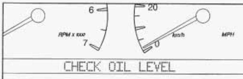
If the CHECK OIL LEVEL message appears on the instrument cluster, it means you need to check your engine oil level right away. For more information, see "CHECK OIL LEVEL" under *DIC Warnings and Messages* on page 3-52.
