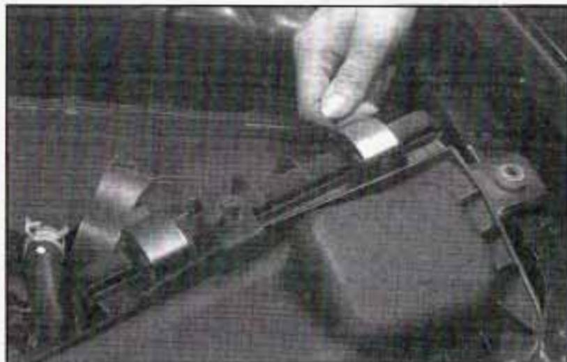
3. Unhook both of the engine air cleaner/filter cover latches.
