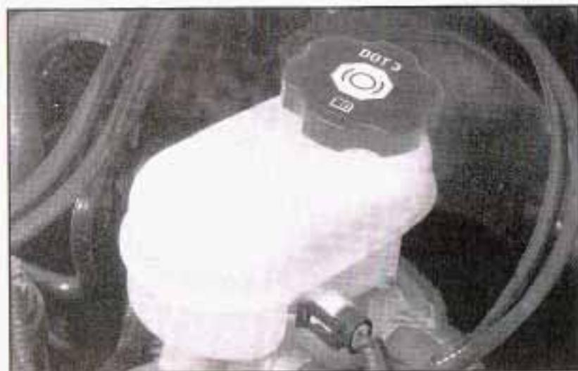
Your brake master cylinder reservoir is on the driver's side of the engine compartment. It is filled with DOT-3 brake fluid. See *Engine Compartment Overview* on page 5-14.
