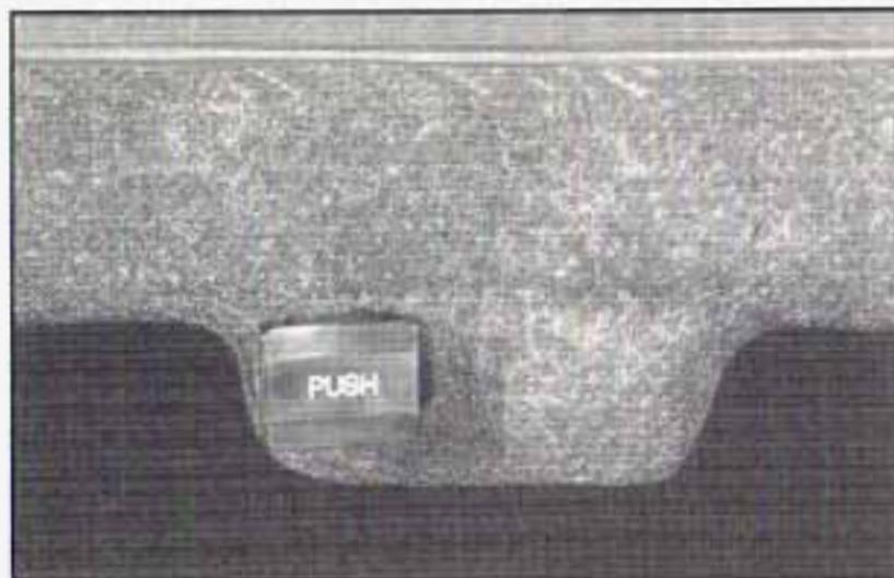
Your vehicle may be equipped with a rear seat pass-through door. The button for this feature is located in the trunk.
