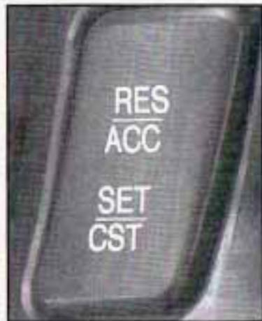
The buttons to operate cruise control are located on the steering wheel.
