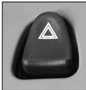
The hazard warning flasher button is located on the top of the steering column.
