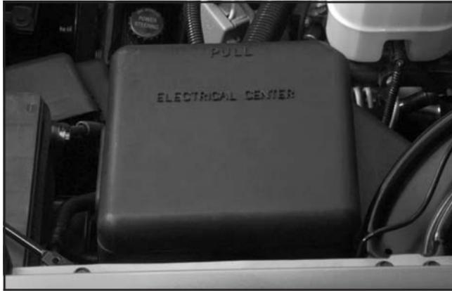
The underhood fuse block in the engine compartment on the driver's side of the vehicle near the battery. Lift the cover for access to the fuse/relay block.
