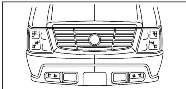
Your vehicle has a visual optical headlamp aiming system equipped with horizontal aim indicators. The aim has been preset at the factory and should need no further adjustment. This is true even though your horizontal aim indicators may not fall exactly on the "0" (zero) marks on their scales.
