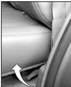
2. Pull the seatback release lever upward and pull the seatback up and fold it down until it is flat. Escalade lever shown, Escalade ESV lever similar. On the Escalade ESV models, first remove the headrest and store it on the top of the seat cushion as shown next.
