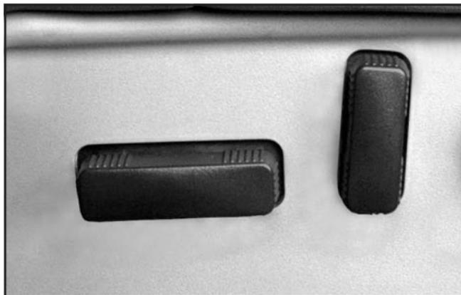
The power seat controls are located on the outboard edge of the front seats.
