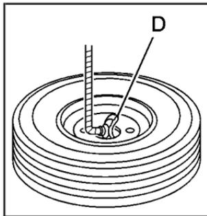
2. Tilt the retainer (D) downward and through the wheel opening. Make sure the retainer is fully seated across the underside of the wheel.
