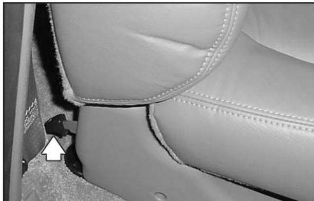
1. Lift the release lever on the back of the seat, upward.
