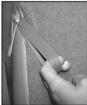
1. Pull up on the release lever labeled 1 and then pull up on the assist strap located on the outboard side of the seat until the seatback locks into the upright position.
