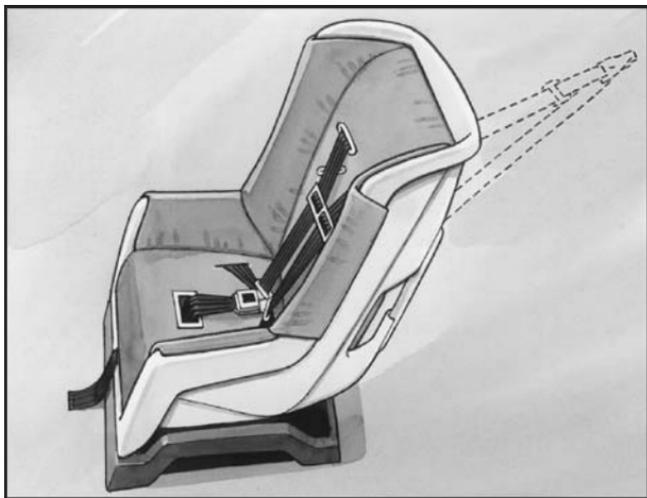
In Canada, the law requires that forward-facing child restraints have a top strap, and that the strap be anchored. In the United States, some child restraints also have a top strap. If your child restraint has a top strap, it should be anchored.
