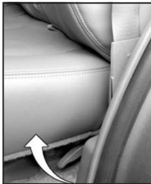
1. Pull up the lever located under the seat cushion. Escalade lever shown, Escalade ESV lever similar.
