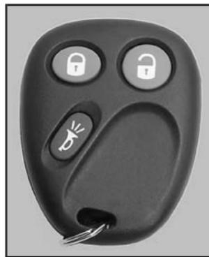
**U (Unlock):** Pressing this button once will unlock the driver's door. The interior lamps will come on. Pressing unlock again within three seconds will cause the remaining doors to unlock.
