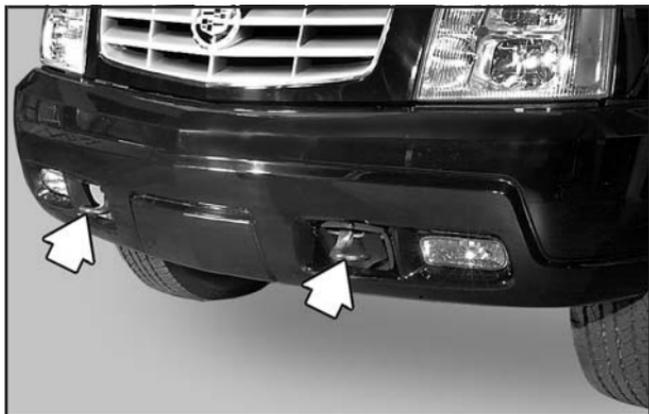
Your vehicle may be equipped with recovery hooks. The recovery hooks are provided at the front of your vehicle. You may need to use them if you are stuck off-road and need to be pulled to some place where you can continue driving.
