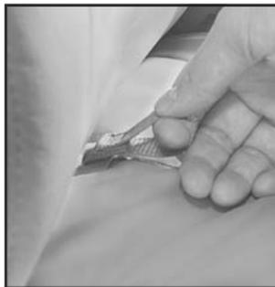
2. Pull up on the strap loop located at the rear of the seat cushion and flip the seat cushion forward.
