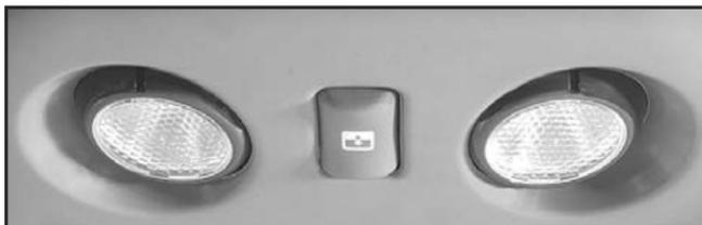
Your vehicle may be equipped with a power sliding sunroof. To open or close your sunroof, the ignition needs to be on or RAP needs to be active. See “Retained Accessory Power” under *Ignition Positions* on page 2-18.
