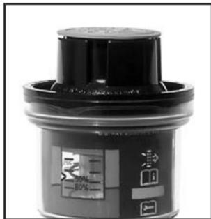
See *Engine Compartment Overview* on page 5-10 for location of engine air cleaner/filter and air filter restriction indicator (if equipped).
