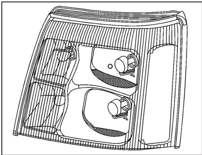
2. Measure the distance from the ground to the aim dot on each low beam lamp. Record this distance.
