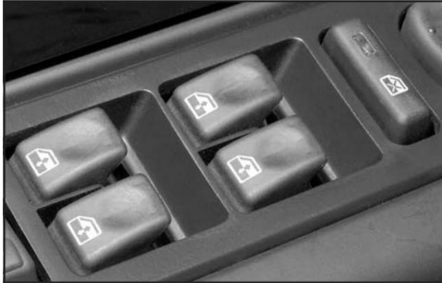
The controls for the power windows are located on the armrest on each of the side doors. The switches operate the windows when the ignition is in RUN, ACCESSORY or when Retained Accessory Power (RAP) is active. See “Retained Accessory Power” under *Ignition Positions* on page 2-18.
