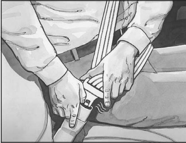
To unclash the belt, just push the button on the buckle. The belt should go back out of the way.
