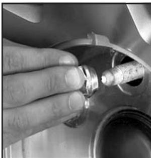
6. After mounting the spare, put the wheel nuts back on with the rounded end of the nuts toward the wheel. Tighten each wheel nut by hand.
