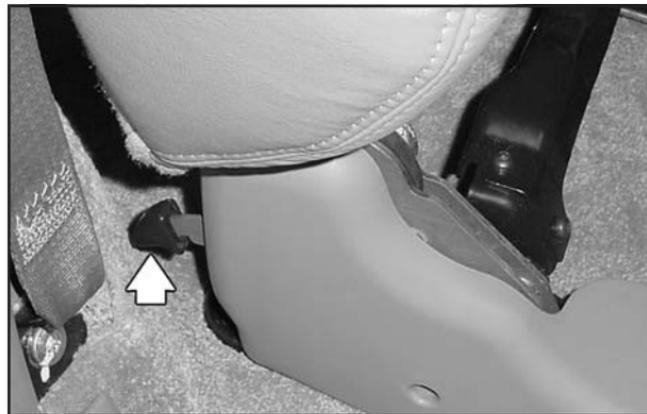
**Escalade ESV:** On the passenger side of Escalade ESV models, the lever at the base of the seat must be pulled up to release the seatback. Pull the seatback forward and fold it down until it is flat.
