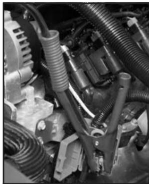
The remote positive (+) terminal is located near the engine accessory drive bracket. On some vehicles, the terminal may be covered under a red plastic cover. To access the remote positive (+) terminal, open the red plastic cover.
