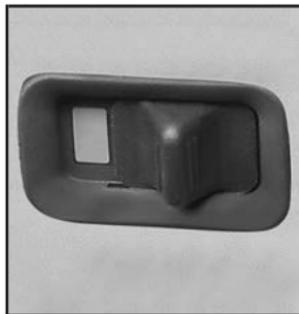
To unlock the door from the inside, slide the manual lever forward. To lock the door, slide the manual lever rearward.
