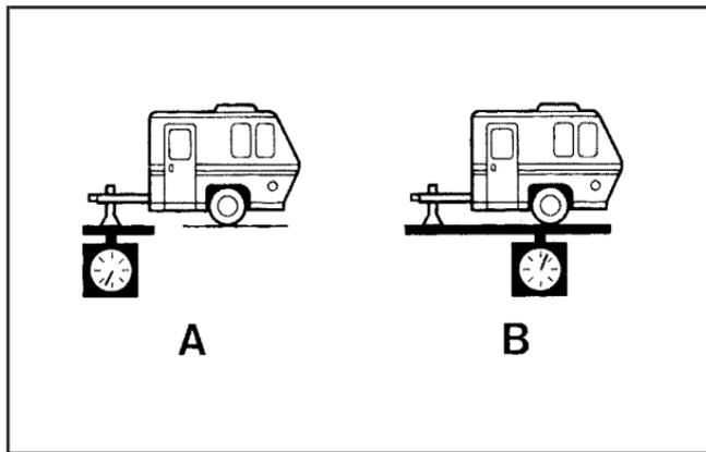
The trailer tongue weight (A) should be 10 percent to 15 percent of the total loaded trailer weight (B), up to a maximum of 600 lbs (272 kg) with a weight carrying hitch. The trailer tongue weight (A) should be 10 percent to 15 percent of the total loaded trailer weight (B), up to the maximum of 1,000 lbs (454 kg) with a weight distributing hitch.
