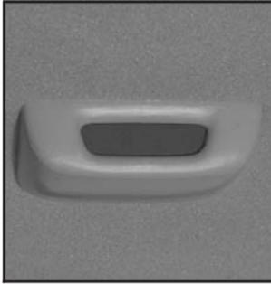
The URPA display is located inside the vehicle, near the rear window. It has three color-coded lights used to provide distance and system information to the driver.
