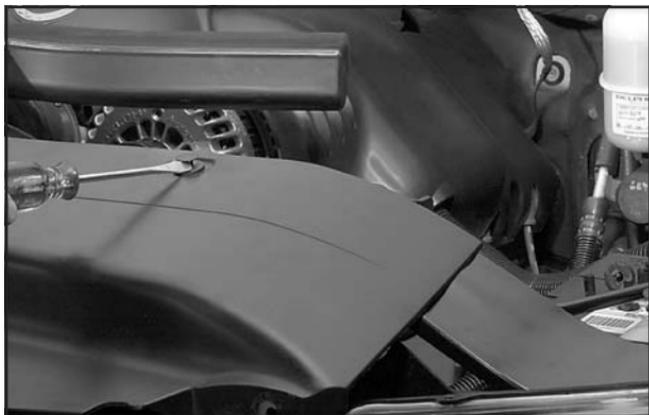
2. Pry up the eight fastener plugs on the radiator cover and pull the fasteners out.
