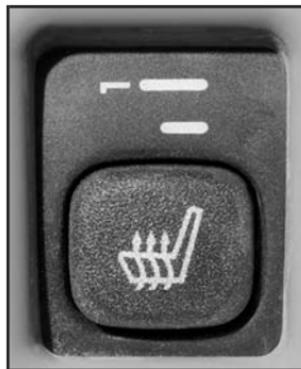
If your vehicle has this feature, the buttons used to control this feature are located on the back of the center console. The engine must be running for the heated seat feature to work.
