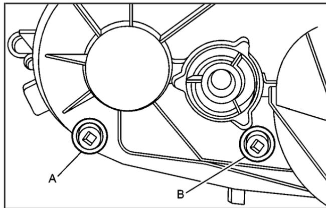
(A) Drain Plug (B) Filler Plug
