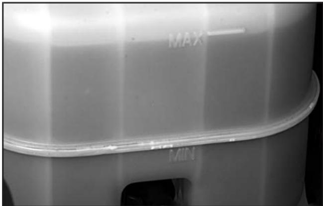
Just look at the brake fluid reservoir. The fluid level should be above MIN. If it is not, have your brake system checked to see if there is a leak.
