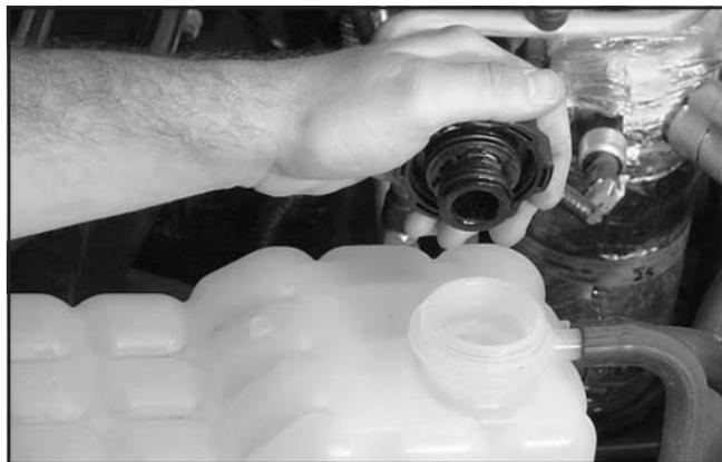
1. Park the vehicle on a level surface. You can remove the coolant surge tank pressure cap when the cooling system, including the coolant surge tank pressure cap and upper radiator hose, is no longer hot. Turn the pressure cap slowly counterclockwise (left) about one full turn. If you hear a hiss, wait for that to stop. A hiss means there is still some pressure left.
