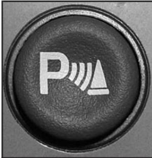
URPA can be turned off by pressing the rear park aid disable switch located near the climate control system and radio. You will not see any lights on the rear display if URPA is turned off.
