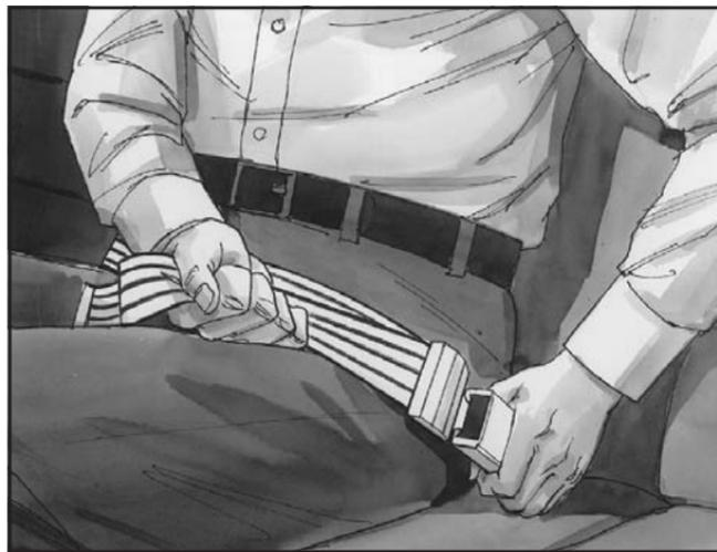
To make the belt shorter, pull its free end as shown until the belt is snug. Buckle, position and release it the same way as the lap part of a lap-shoulder belt. If the belt is not long enough, see *Safety Belt Extender* on page 1-48.
