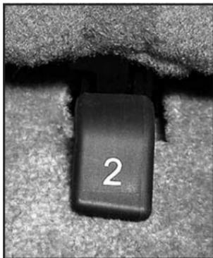
4. Squeeze the release handle while pulling the seat out.
