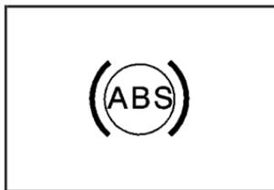
If there is a problem with the anti-lock brake system, this warning light will stay on. See *Anti-Lock Brake System Warning Light* on page 3-38.
