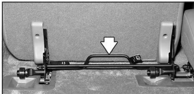
3. To unlatch the rear of the seat from the floor, pull up on the release lever labeled 2 at the rear of the seat, and lift the rear of the seat up from the floor.
