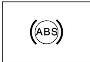
With the anti-lock brake system, the light will come on when your engine is started and may stay on for several seconds. That's normal.
