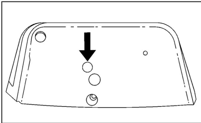
1. Locate the plastic screw head on the underside of the plastic cover for the steering column.
