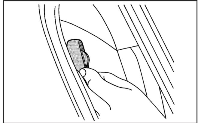
1. Slide the guide off of its storage clip located between the interior body and the seatback.
