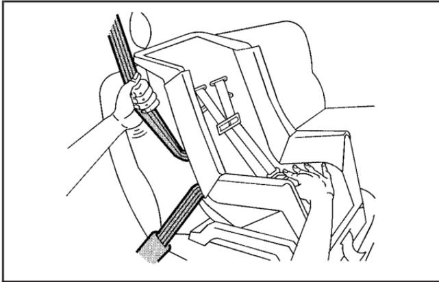
6. To tighten the belt, push down on the child restraint, pull the shoulder portion of the belt to tighten the lap portion of the belt and feed the shoulder belt back into the retractor. You may find it helpful to use your knee to push down on the child restraint as you tighten the belt.
