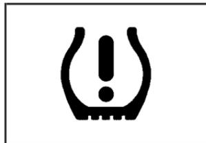
If your vehicle has the Tire Pressure Monitor (TPM) System, this light will come on if the system detects low tire pressure.
