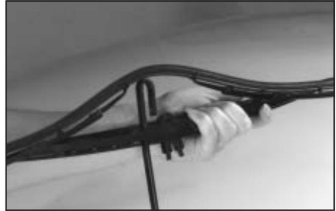
7. Reinstall the wiper blade assembly by sliding it over the wiper arm to engage the J-hooked end. Pull up on the assembly to lock it into place.
