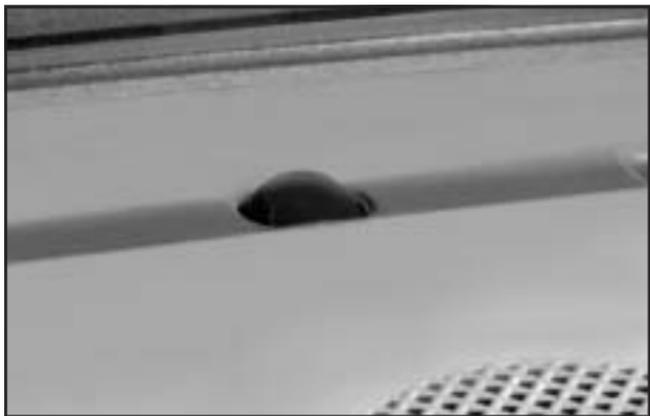
There is a solar sensor located on the instrument panel, near the windshield.
