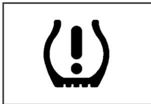
When the tire pressure monitoring system warning light is lit, one or more of your tires is significantly under-inflated.
