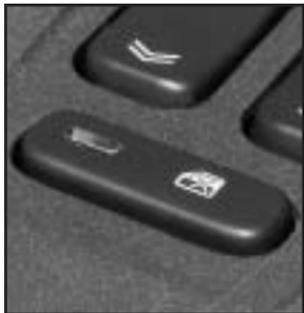
The passenger window lockout button is located below the power window switches on the driver's door armrest.
