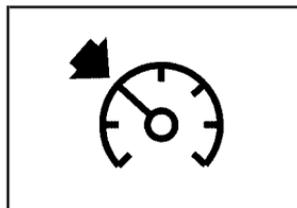
This light on the instrument panel cluster will come on while cruise control is on.
