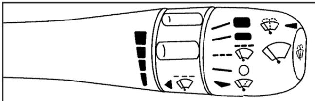
The lever on the right side of the steering column operates the windshield wipers.
