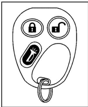
**🔒 (Lock):** Press this symbol on the remote keyless entry transmitter to lock the doors. This also arms the theft-deterrent system.
