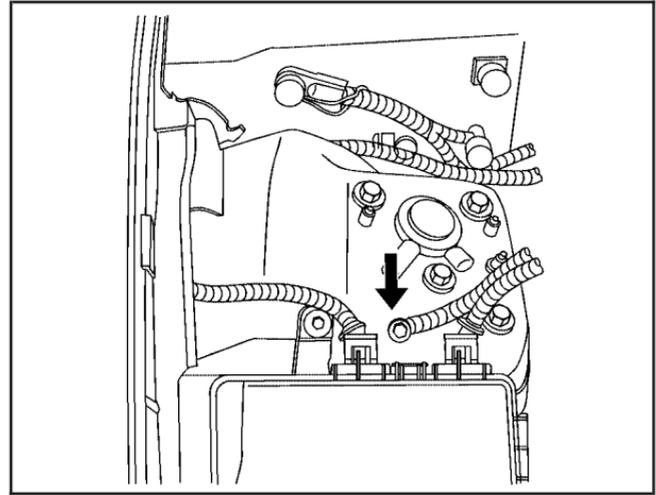
Your vehicle has a remote negative (-) ground location, as shown in the illustration. It is located between the battery and the underhood fuse block. You should always use this remote ground location, instead of the terminal on the battery.
