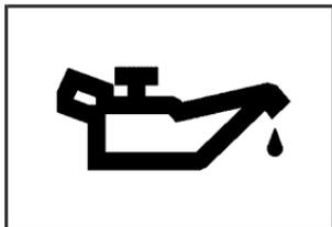
If the oil pressure light and/or the Oil Pressure Low — Stop Engine message on the DIC appears on the instrument cluster, it means you need to check your engine oil level right away.
