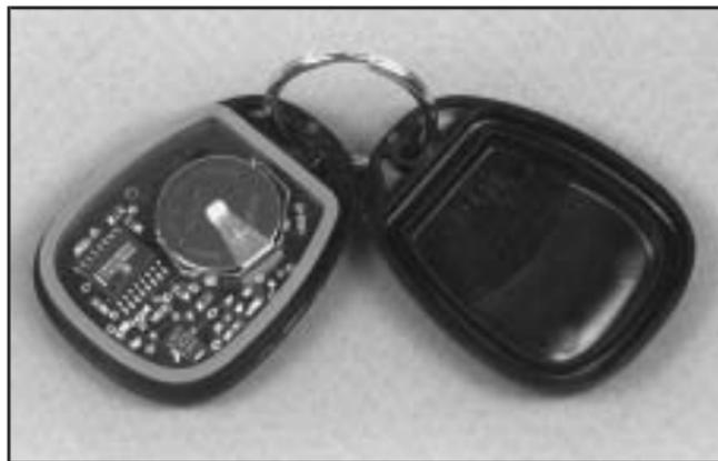
1. Use a flat thin object to pry open the transmitter.
