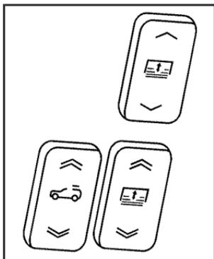
The sunroof/sunshade switches are located in the headliner between the driver and front passenger.
