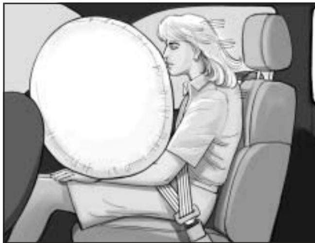
The front passenger's frontal airbag is in the instrument panel on the passenger's side.
