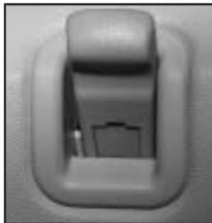
From the inside, use the manual lock levers located on the door panels near the windows.
