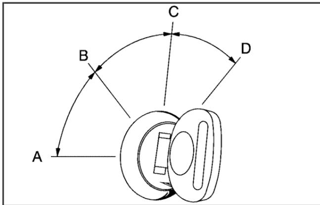
**Notice:** If your key seems stuck in OFF and you can't turn it, be sure you are using the correct key; if so, is it all the way in? If it is, then turn the steering wheel left and right while you turn the key hard. Turn the key only with your hand. Using a tool to force it could break the key or the ignition switch. If none of these works, then your vehicle needs service.
