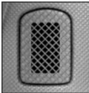
There is also an interior temperature sensor located to the right of the steering wheel on the instrument panel.
