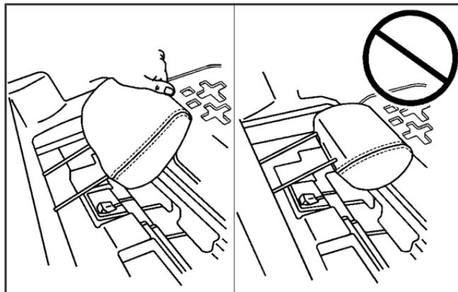
Store the head rests in the storage compartment behind the third row. Open the cover and insert the head rest posts through the slats in the storage area. The head rests must be stored with the front of the rest facing up. Position and snap the head rests in the provided storage tray.
