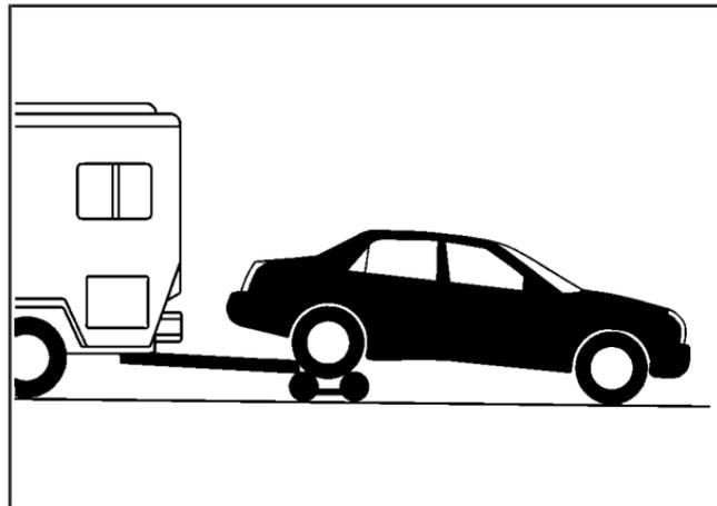
If your vehicle is a rear-wheel drive, it can be towed using a dolly. If you have an All-Wheel-Drive (AWD) vehicle, it can only be towed on a flat-bed trailer. To tow your vehicle using a dolly, follow these steps:
