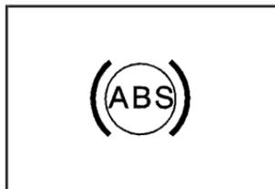
If there is a problem with the anti-lock brake system, this warning light will stay on. See *Anti-Lock Brake System Warning Light* on page 3-39.
