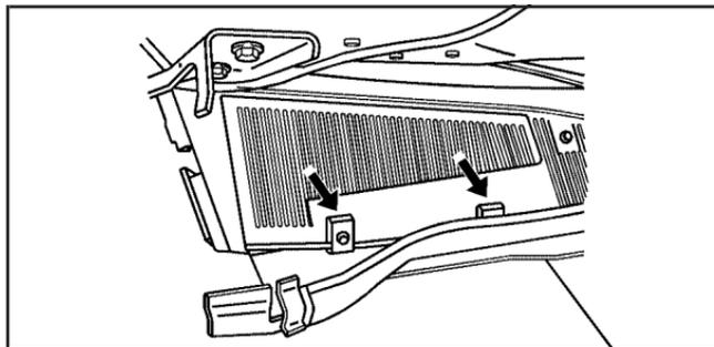
2. Push the two tabs on the access panel door towards the windshield.
