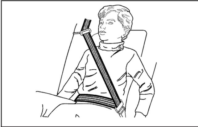
4. Buckle, position and release the safety belt as described in *Rear Seat Passengers* on page 1-22. Make sure that the shoulder belt crosses the shoulder.
