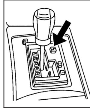
1. Use a tool to remove the cap with the lock symbol located next to the shift lever.
