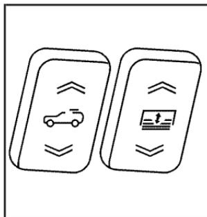
The sunroof/sunshade switches are located in the headliner between the driver and front passenger.
