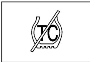
If the TC (traction control) warning light comes on and stays on, there may be a problem with the traction control system.
