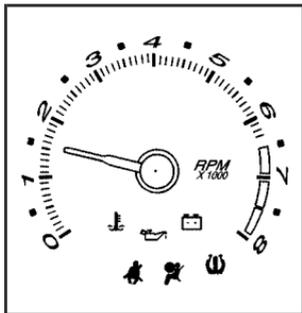
This gage indicates the engine speed in revolutions per minute (rpm).
