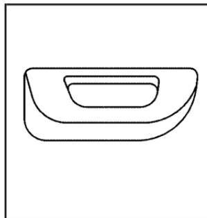
The URPA display is located inside the vehicle, above the liftgate glass. It has three color-coded lights that can be seen through the rearview mirror or by turning around.
