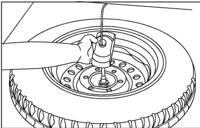
3. Tilt the retainer downward and slip it through the center hole of the spare tire.
