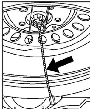
1. Check under the vehicle to see if the cable is visible. If it is not visible, see *Secondary Latch System* on page 5-81.
