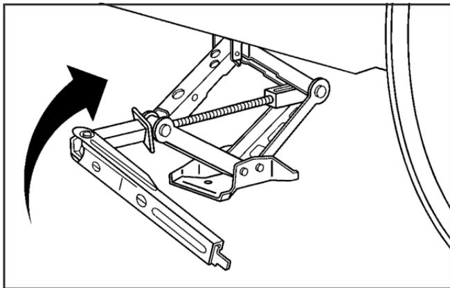
7. Raise the vehicle by turning the wheel wrench clockwise. Raise the vehicle far enough off the ground for the compact spare tire to fit under the vehicle.
