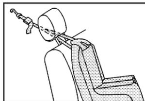
If the position you are using has an adjustable head restraint and you are using a dual tether, route the tether under the head restraint and in between the head restraint posts.
