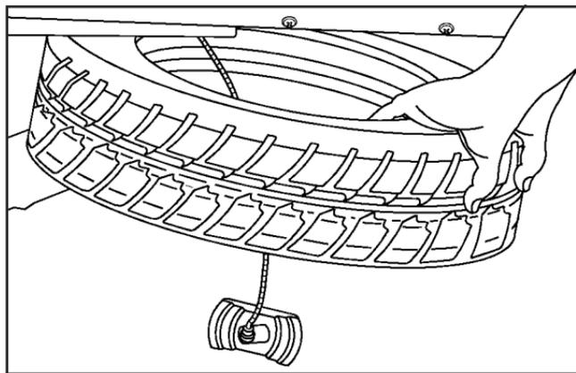
8. Grasp the spare tire with both hands and pull it out from under the vehicle.
