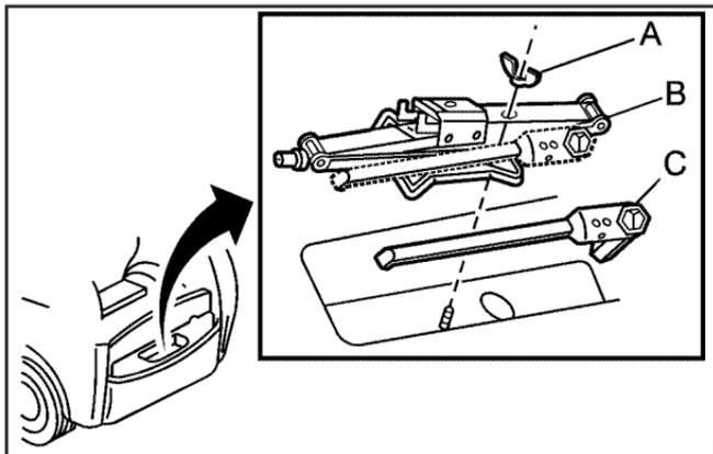
2. Turn the wing nut (A) holding the jack (B) (and storage tray, if applicable) counterclockwise and remove it.
