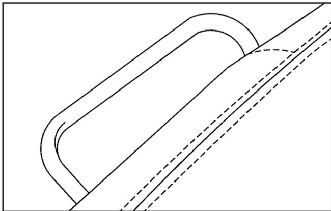
Your vehicle may have a manual passenger seat. To adjust the seat, lift the bar under the front of the seat to unlock it. Slide the seat to where you want it and release the bar. Try to move the seat back and forth with your body to be sure the seat is locked in place.
