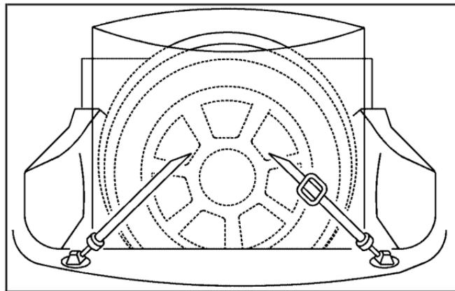
3. Place the flat tire in the tire storage bag and put the tire in an upright position against the third row seat.
