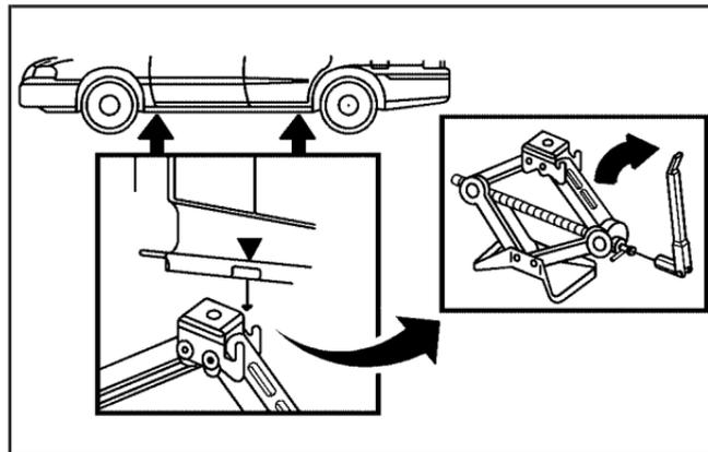
5. Raise the jack by turning the wheel wrench clockwise until the slots in the jack head fit into the metal flange located behind the triangle on the plastic molding as shown.
