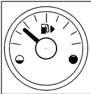
The fuel gage shows approximately how much fuel is in the tank. It works only when the ignition is in ON.
