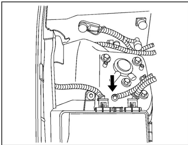
Your vehicle has a remote negative (-) ground location, as shown in the illustration. It is located between the battery and the underhood fuse block. You should always use this remote ground location, instead of the terminal on the battery.
