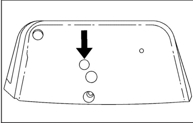
1. Locate the plastic screw head on the underside of the plastic cover for the steering column.
