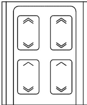
The power window switches are located on the armrest near each window. Press the up or down arrows on the switches to raise or lower the windows.
