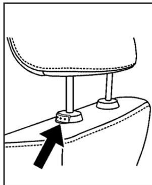
The front seat head restraints can be adjusted up and down. Pull up the head restraint to raise it. Press the button located at the base of the head restraint and push down on the restraint to lower it. The front seat head restraints also tilt forward and rearward.
