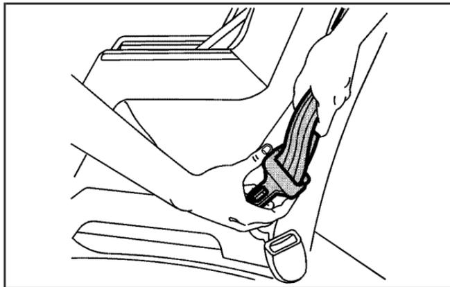
4. Tilt the latch plate to adjust the belt if needed.
