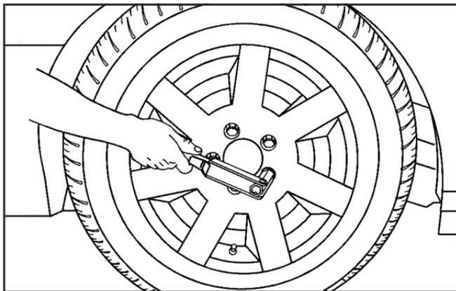
1. Loosen the wheel nuts, but do not remove them yet, using the wheel wrench. Turn the handle about 180 degrees, then flip the handle back to the starting position. This avoids taking the wrench off the lug nut for each turn.
