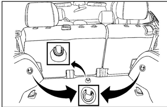
Do not secure a child restraint in the right front passenger's position or any third row position if a national or local law requires that the top tether be attached, or if the instructions that come with the child restraint say that the top tether must be attached. There is no place to attach the top tether in this position.
