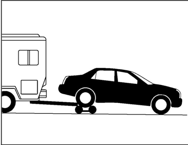
If your vehicle is a rear-wheel drive, it can be towed using a dolly. If you have an All-Wheel-Drive (AWD) vehicle, it can only be towed on a flat-bed trailer. To tow your vehicle using a dolly, follow these steps:
