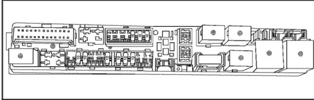
The passenger's side rear fuse block is located under the rear seat on the passenger's side of the vehicle. The carpet must be lifted up to access the rear fuse block.
