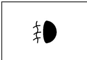
The fog lamps light will come on when the fog lamps are in use.
