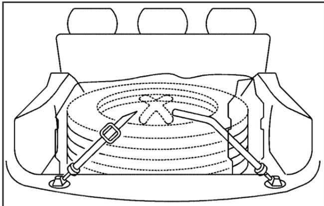
2. Place the flat tire in the tire storage bag and put the tire in a horizontal position on the floor in the rear of the vehicle.
