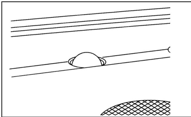
The light sensor for the DRL and AUTO headlamp feature is located on top of the instrument panel. If you cover the sensor, it will read dark, and the exterior lamps or the Headlamps Suggested message will appear on the DIC whenever the ignition is on.
