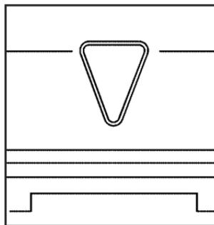
2. Find the jacking location using the hoisting notches located in the plastic molding. The notches in the plastic molding are marked with a triangle shape to help you find them.
