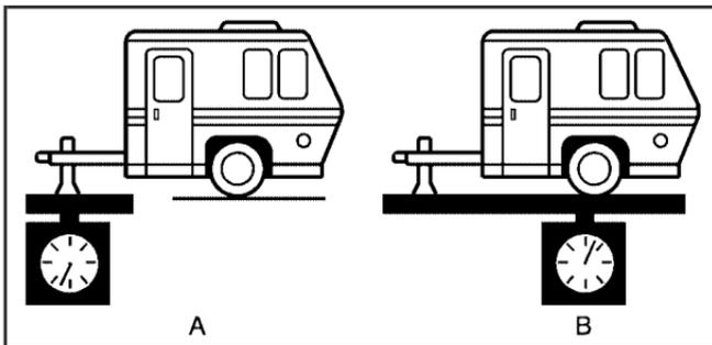
If you're using a weight-carrying hitch or a weight-distributing hitch, the trailer tongue (A) should weigh 10-15 percent of the total loaded trailer weight (B).
