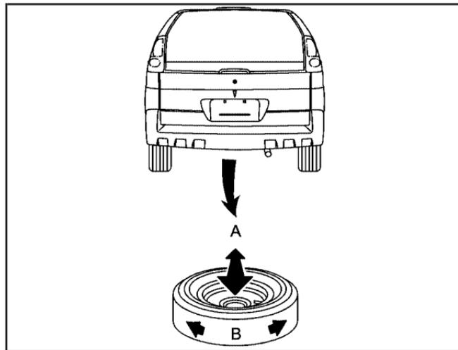
8. Make sure the tire is stored securely. Push, pull (A), and then try to turn the tire (B). If the tire moves, use the wheel wrench to tighten the cable. Put back all tools as they were stored in the rear storage compartment and put the compartment cover back on.
