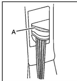
To move it down, press the release button (A) and move the height adjuster to the desired position. You can move the height adjuster up just by pushing up on the shoulder belt guide.
