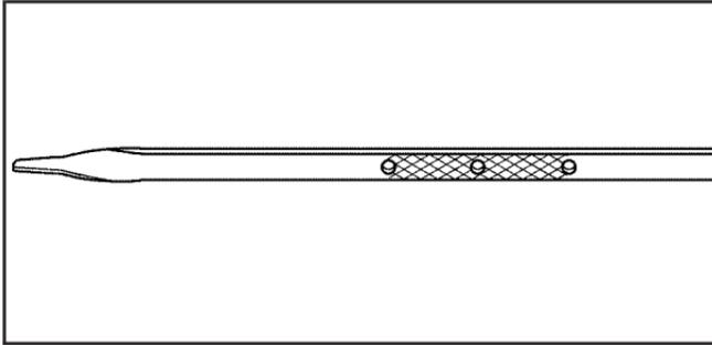
If the oil is below the cross-hatched area at the tip of the dipstick, you will need to add at least one quart/liter of oil. But you must use the right kind. This section explains what kind of oil to use. For engine oil crankcase capacity, see *Capacities and Specifications on page 452*.
