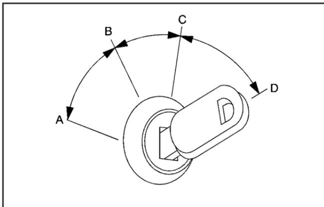
**Notice:** Using a tool to force the key from the ignition switch could cause damage or break the key. Use the correct key and turn the key only with your hand. Make sure the key is in all the way. If none of this works, then your vehicle needs service.
