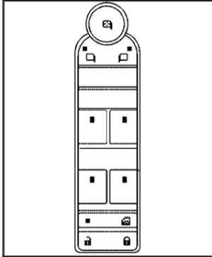
The power window switches are located on the driver's door armrest.
