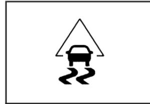
For vehicles that have the StabiliTrak® system, this warning light should come on briefly when the engine is started.
