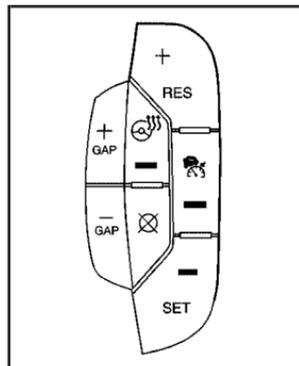
The Adaptive Cruise controls are located on the steering wheel.
