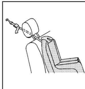
If the position you are using has an adjustable head restraint and you are using a single tether, route the tether under the head restraint and in between the head restraint posts.
