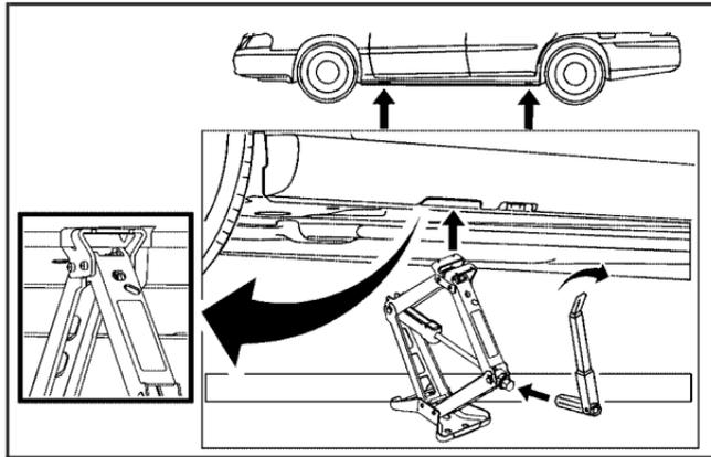
5. Raise the jack until the metal flange fits firmly into the channel of the jack head.
