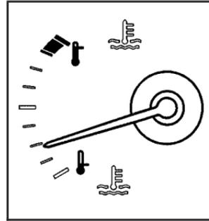
This gage shows the engine coolant temperature.
