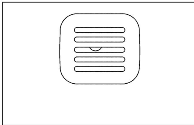
There is also an interior temperature sensor located next to the steering wheel that measures the temperature of the air inside your vehicle.
