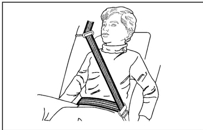
4. Buckle, position, and release the safety belt as described in *Rear Seat Passengers on page 34*. Make sure that the shoulder belt crosses the shoulder.
