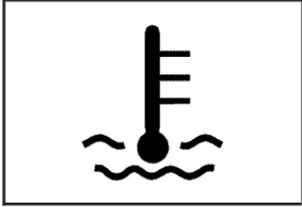
The engine coolant temperature warning light will come on when the engine is very hot.
