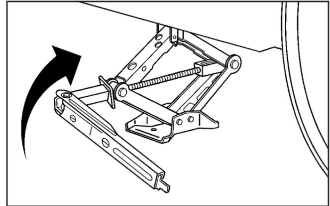
7. Raise the vehicle by turning the jack handle clockwise. Raise the vehicle far enough off the ground for the spare tire to fit under the vehicle.
