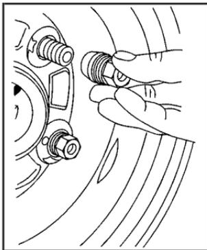
11. Put the wheel nuts back on with the rounded end of the nuts toward the wheel. Tighten each nut by hand until the wheel is held against the hub.
