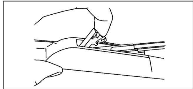
3. Pull the clip up from the blade connecting point, and pull the blade assembly down toward the windshield to remove it from the wiper arm.
