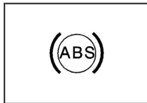
With the anti-lock brake system, the light will come on when your engine is started and may stay on for several seconds. That is normal.
