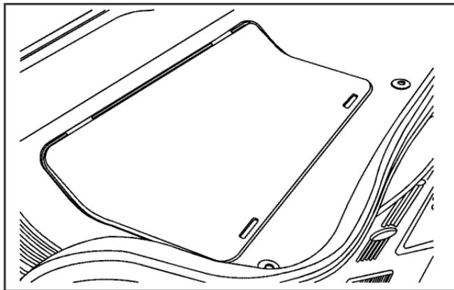
The access panel for the passenger compartment air filter is located under the hood near the windshield, on the passenger's side of the vehicle.
