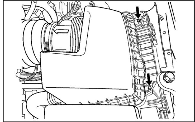
1. Loosen and remove the two screws on the top of the engine air cleaner/filter cover.
