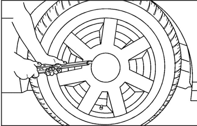
1. For models having aluminum wheels with a center wheel cover, use the flat end of the wheel wrench to gently pry the wheel covers off. Be careful not to scratch the aluminum wheel edge and do not try to remove it with your hands. Then loosen the wheel nuts with the wheel wrench. Do not remove them yet.
