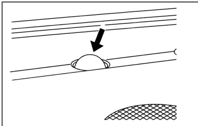
The solar sensor, located in the defrost grille, middle of the instrument panel, monitors the solar radiation. Do not cover the solar sensor or the system will not work properly.
