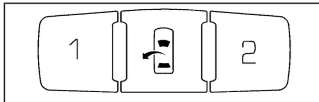
The controls for this feature are located on the driver's door panel, and are used to program and recall memory settings for the driver's seat, outside mirror, and the steering wheel position if the vehicle has the power tilt wheel and telescopic steering feature.
