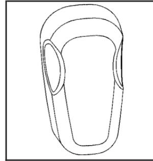
Your seats have power reclining seatbacks. Use the vertical power seat control located on the outboard side of the seat to operate them.
