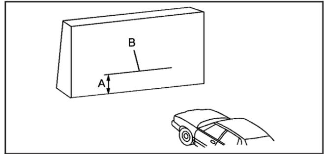
4. At the wall measure from the ground upward (A) to the recorded distance from Step 3 and mark it.
