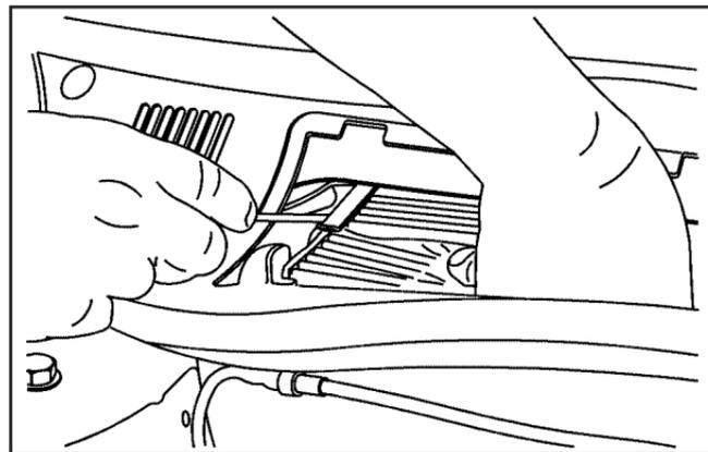
3. To remove the air filter, insert a tool between the air filter and the compartment wall on the outboard side of the vehicle. Then, push in to flatten the pin holding the air filter in place. Gently remove the air filter and any loose debris that may be inside the air filter compartment.
