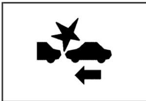
The Adaptive Cruise Control alert symbol is located on the display at the top of the instrument panel to the right of the driver.
