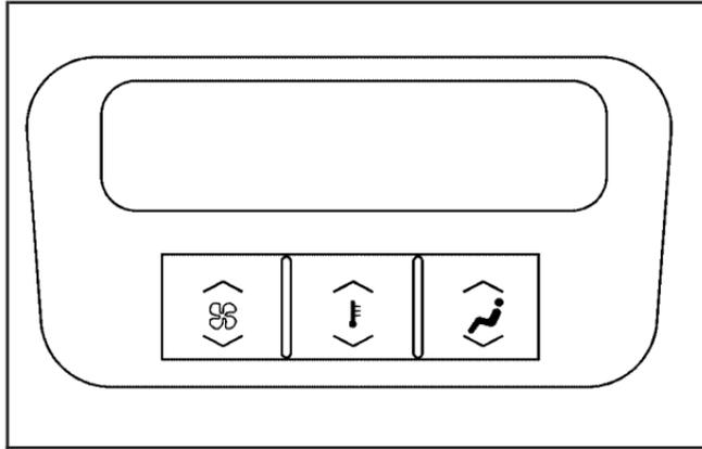
If your vehicle has a rear climate-control system, the rear-seat passengers can use it to adjust the direction of the airflow, the fan speed and the temperature for the rear-seating area. This system also works with the main climate-control system in your vehicle.
