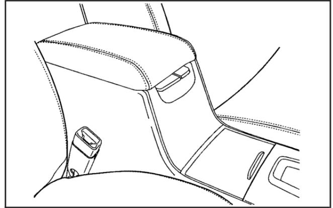
If your vehicle has a full floor console it has two storage areas. To access the upper tray storage, lift the left lever located in the front of the armrest lid. To access the lower storage area, lift the right lever. If your vehicle has a center seat console it will have two storage areas.
