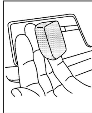
To tilt the wheel, hold the wheel and pull the lever. Then move the wheel to a comfortable position and release the lever to lock the wheel in place.
