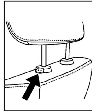
To raise a front seat head restraint, pull up on the restraint. To lower it, press the button, located on the top of the seatback, and push the head restraint down.
