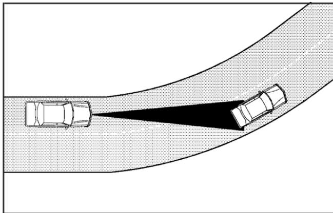
Adaptive Cruise Control may detect a vehicle that is not in your lane and apply the brakes.
