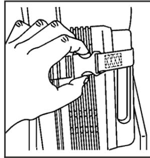
3. Remove the tire inflator kit strap by squeezing the two tabs of the quick release buckle.
