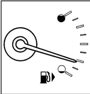
The fuel gage shows approximately how much fuel is in the tank. It works only when the engine is on.
