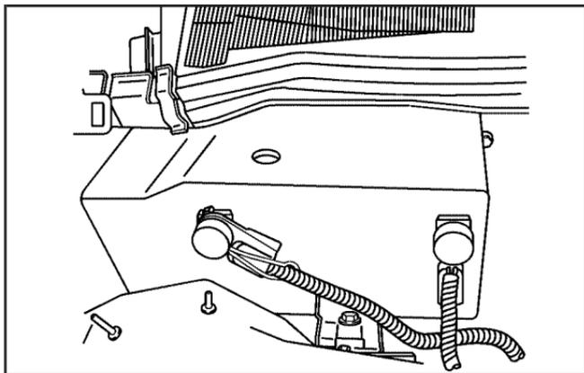
4. Open the hoods and locate the positive (+) and negative (-) terminal locations of the other vehicle, as well as the positive (+) terminal location on your vehicle's battery. See *Engine Compartment Overview* on page 373 for more information on the location of the battery.
