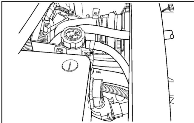
See *Engine Compartment Overview* on page 373 for the location of the intercooler system pressure cap.
