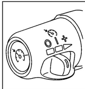
The Forward Collision Alert (FCA) controls are located on the end of the multifunction lever.
