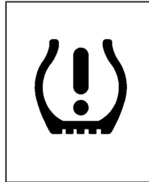
This light will come on briefly as you start the engine, for vehicles equipped with the Tire Pressure Monitor System.
