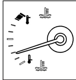
This gage shows the engine coolant temperature.
