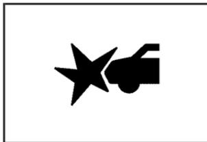
The alert symbol will flash on the HUD and a warning beep will sound when driver action is required.
