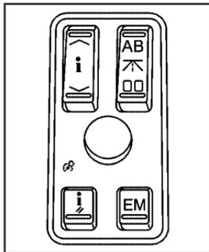
If your vehicle does not have a Head-Up Display (HUD), these are the buttons for the DIC.
