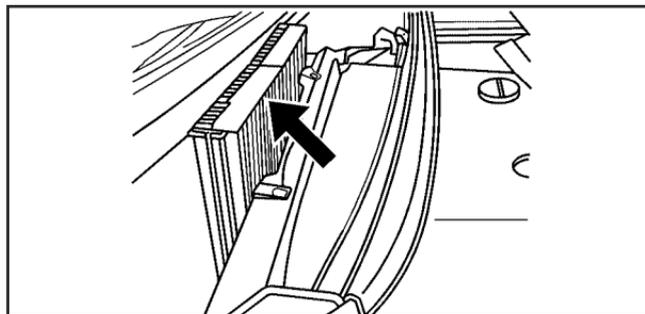
6. The top edge of the filter should be visible. Reach in and lift the filter out, pulling upward and toward the front of the vehicle.
