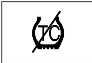
If the Traction Control (TC) warning light comes on and stays on, there may be a problem with the traction control system.
