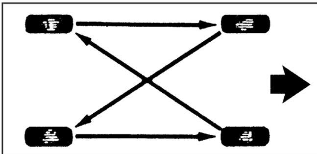
When rotating P235/50R17 size tires or 255/45ZR18 size tires, always use the correct rotation pattern shown here.
