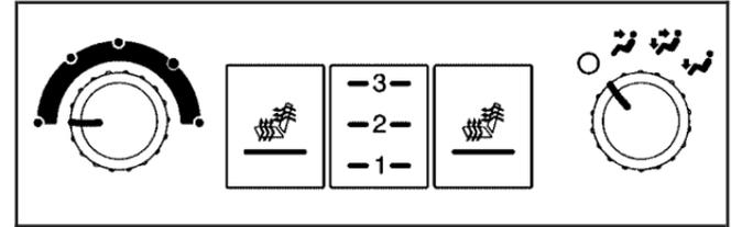
Your vehicle has a rear climate control system. The base model includes air outlets in the rear of the center console for cooling and under-seat air outlets for heating. The temperature, quantity, and air delivery location is controlled automatically by the front climate control system.
