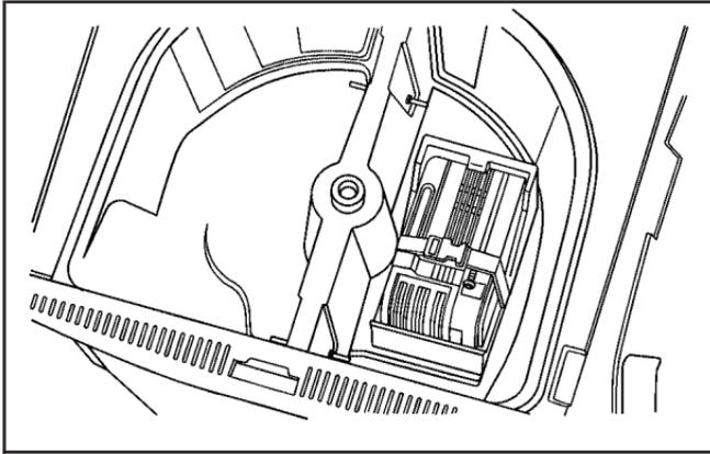
2. Locate the tire inflator kit on the driver's side of the vehicle, near the back corner of the trunk.
