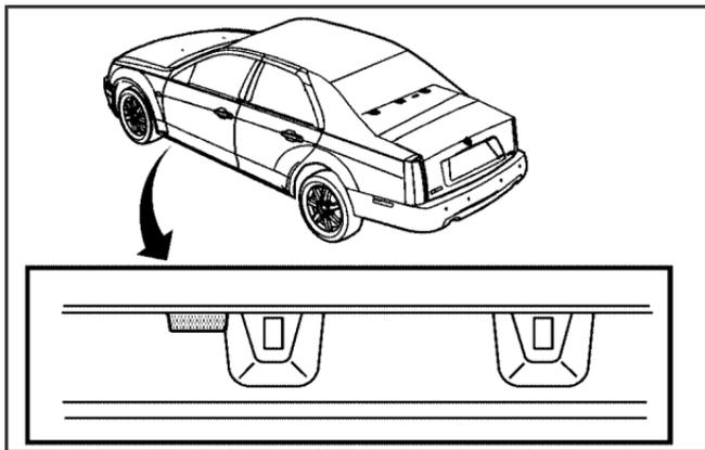
1. Locate the front lifting points using the diagram above. The front lifting location is about 15 inches (37 cm) from the rear edge of the front wheel well.
