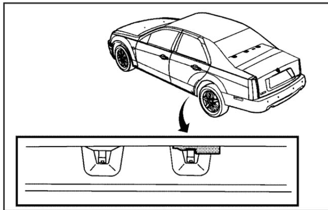
1. Locate the rear lifting points using the diagram above. The rear lifting location is about 7 inches (17 cm) from the front edge of the rear wheel well.
