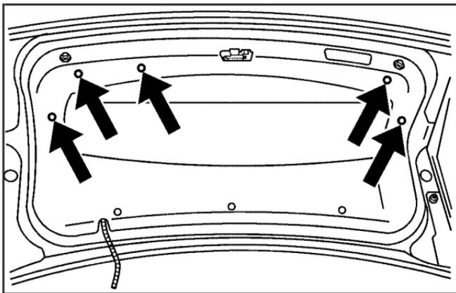
2. Pull out the push pins holding down the top portion of the cloth cover.
