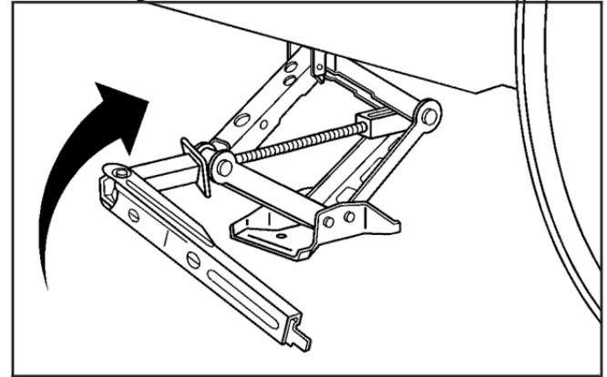
7. Raise the vehicle by turning the wheel wrench clockwise. Raise the vehicle far enough off the ground for the compact spare tire to fit under the vehicle.
