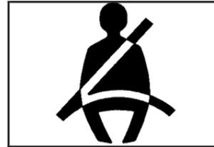
This chime and light will be repeated if the driver remains unbuckled and the vehicle is in motion.
