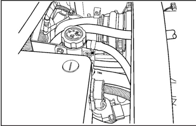
1. Remove the Intercooler System pressure cap when the Intercooler System, including the upper intercooler hoses, are no longer hot. Turn the pressure cap slowly counterclockwise about one-quarter of a turn. If you hear a hiss, wait for that to stop. This allows any pressure still left to be vented.
