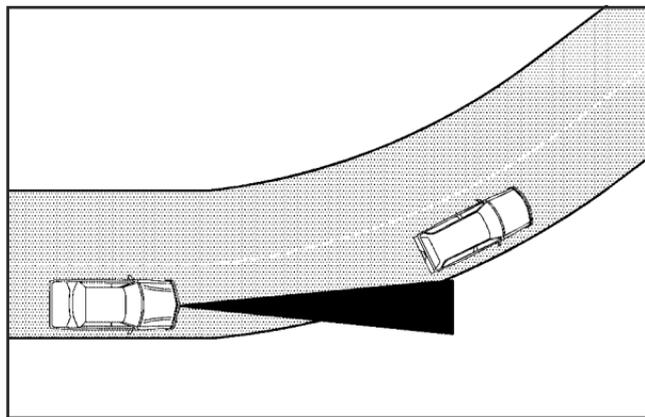
When following a vehicle and entering a curve, Adaptive Cruise Control could lose track of the vehicle in your lane and accelerate your vehicle. When this happens, the vehicle ahead symbol will not appear on the HUD.
