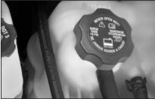
The coolant surge tank and pressure cap are located on the driver's side of the vehicle, toward the rear of the engine compartment. See *Engine Compartment Overview on page 373* for more information on location.
