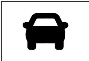
The vehicle ahead symbol will only appear on the HUD when a vehicle ahead is detected in your path.
