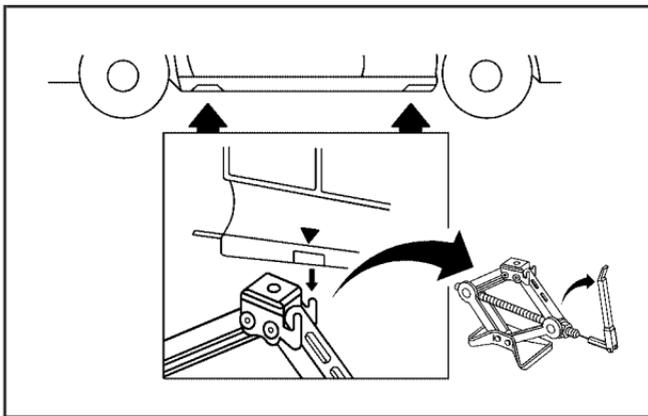
2. Find the vehicle's jacking location using the diagram above and corresponding hoisting notches located in the plastic molding on the vehicle's frame. The notches in the plastic molding are marked with a triangle shape to help you find them.
