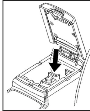
If moving the transmitter to different locations within the vehicle does not help, place the transmitter in the center console transmitter pocket with the buttons facing forward and then press the START button.
