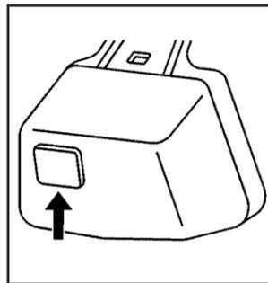
The light sensor is located on the inside of the vehicle at the back of the rearview mirror.
