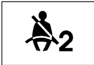
This chime and light will be repeated if the passenger remains unbuckled and the vehicle is in motion.
