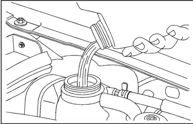
3. Fill the coolant surge tank with the proper DEX-COOL<sup>®</sup> coolant mixture, to slightly above the FULL COLD/FROID line on the side of the coolant surge tank.
