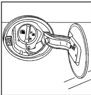
The tethered fuel cap is located behind a hinged fuel door on the passenger's side of the vehicle.
