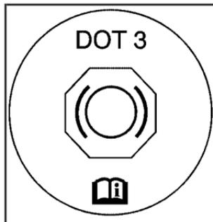
Your brake master cylinder reservoir is filled with DOT-3 brake fluid. See *Engine Compartment Overview* on page 373 for reservoir location and access.
