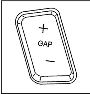
Use the GAP button on the steering wheel to adjust the follow distance.
