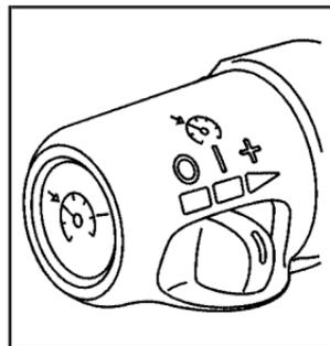
The Adaptive Cruise controls are located on the end of the multifunction lever.
