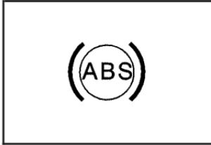
With the Anti-Lock Brake System (ABS), this light will come on when your engine is started and may stay on for several seconds. That is normal.
