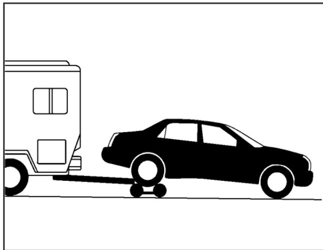
If your vehicle is a rear-wheel drive, it can be towed using a dolly. To tow your vehicle using a dolly, follow these steps:
