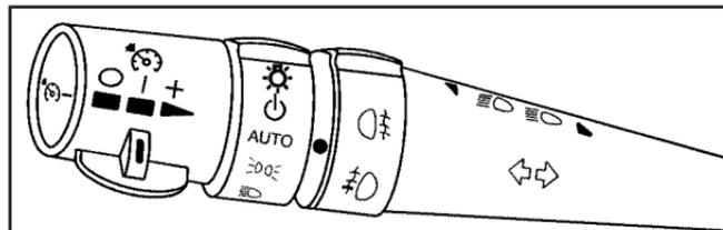
The exterior lamp control is located in the middle of the turn signal/multifunction lever.
