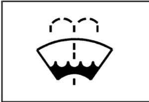
Open the cap with the washer symbol on it. Add washer fluid until the tank is full. See *Engine Compartment Overview on page 373* for reservoir location.
