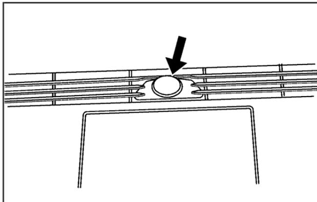
The light sensor for the DRL is located on top of the instrument panel. If you cover the sensor, it will read dark, and the exterior lamps may come on when you do not need them.
