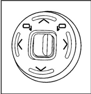
The power mirror control is on the driver's door armrest and controls the driver's side and passenger's side mirrors.
