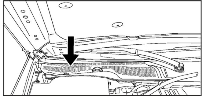
The access panel for the passenger compartment air filter is located under the hood near the windshield, on the passenger's side of the vehicle. See *Engine Compartment Overview on page 373* for more information on location. See *Doing Your Own Service Work on page 364* for information on doing your own service work.
