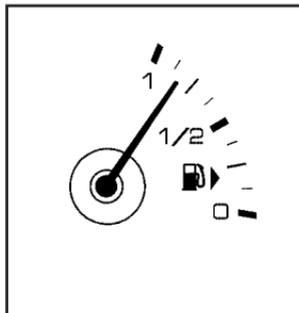
The fuel gage shows approximately how much fuel is in the fuel tank. It works only when the ignition is in the ON/RUN position.
