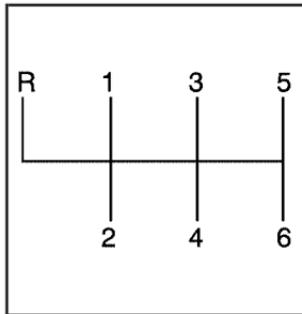
**FIRST (1):** Press the clutch pedal and shift into FIRST (1). Then slowly let up on the clutch pedal as you press the accelerator pedal.
