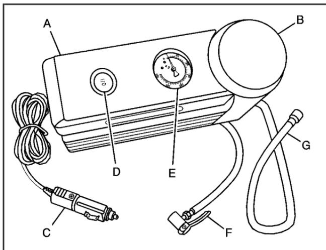
5. Pull the air only hose (F) from the sealant canister (B).
