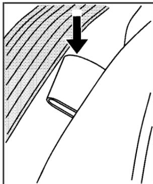
1. Pull forward on the tab, located on the outboard side of the seatback, to unlock the seatback.
