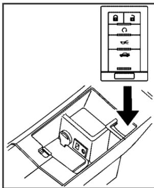
2. Place the new, unrecognized transmitter into the transmitter pocket with the transmitter buttons facing the front of the vehicle. The transmitter pocket is inside the center console storage area located between the driver and front passenger seats.
