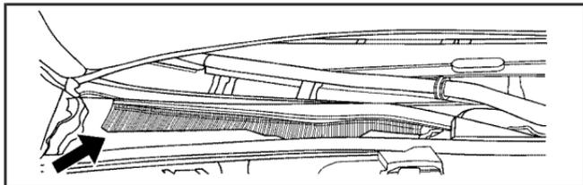
The passenger compartment air filter is located underneath the hood below the windshield wiper arm and the screen on the passenger side of the vehicle. See *Engine Compartment Overview on page 5-14* for more information on location.
