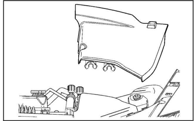
2. Remove side cover by pulling up on front of cover.
