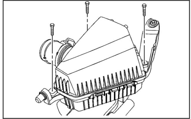
6. Remove the three air cleaner housing cover screws.
