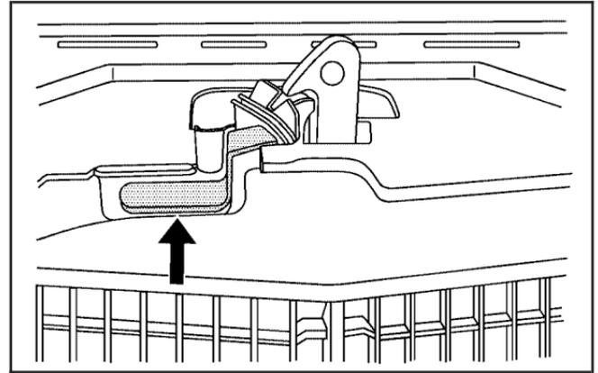
2. Then go to the front of the vehicle and find the secondary hood release lever. The lever is located under the front edge of the grille near the center. Push the release lever up and raise the hood.
