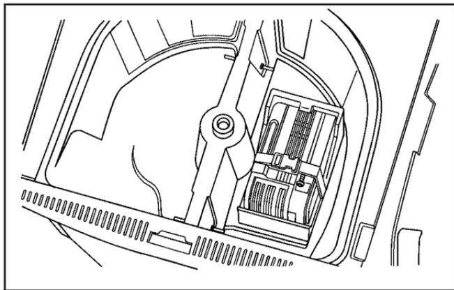
2. Locate the tire sealant and compressor kit on the driver side of the vehicle, near the back corner of the trunk.
