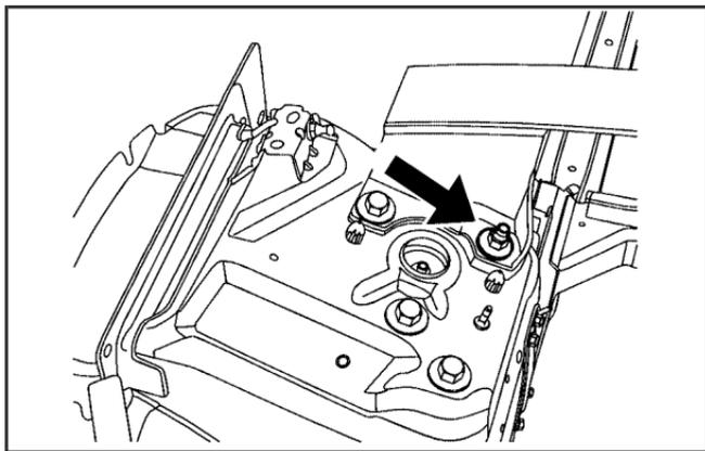
Your vehicle has a remote negative (–) ground location, as shown in the illustration. It is located on the rear passenger side of the vehicle. See *Engine Compartment Overview* on page 5-14. You should always use this remote ground location, instead of the terminal on the battery.
