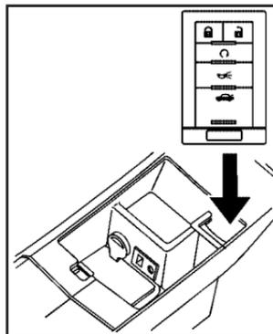
If moving the transmitter to different locations within the vehicle does not help, place the transmitter in the center console transmitter pocket with the buttons facing to the right and then press the START button.
