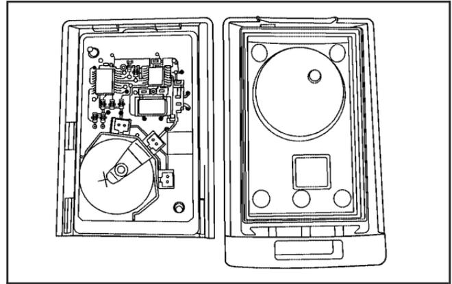
To replace the battery in the RKE transmitter:
