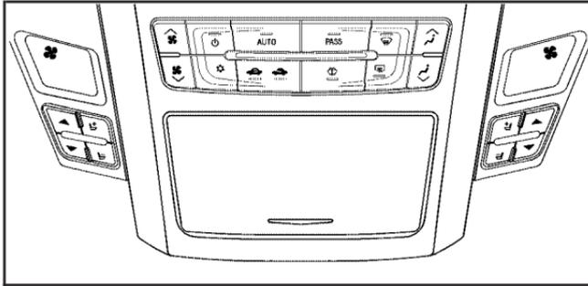
**Power:** Press this button to turn the climate control system on or off. When the climate control system is turned off the air inlet defaults to outside air.
