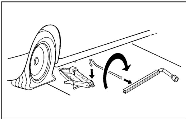
4. Insert the hooked end of the extension handle through the jack and the flat end through the wheel wrench.
