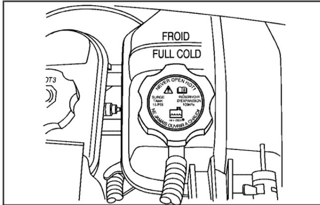
The coolant surge tank and pressure cap are located on the driver's side of the vehicle, toward the rear of the engine compartment. See *Engine Compartment Overview* on page 5-14 for more information on location.
