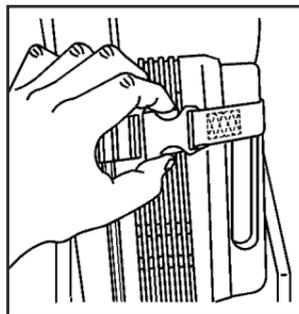
3. Remove the tire sealant and compressor kit strap by squeezing the two tabs of the quick release buckle.
