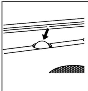
There is a solar sensor, located on the instrument panel, near the windshield.
