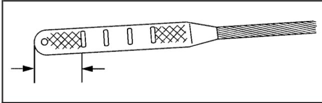
If the oil level is within the add cross-hatched area at the tip of the dipstick, add at least one quart/liter of the recommended oil. This section explains what kind of oil to use. For engine oil crankcase capacity, see *Capacities and Specifications on page 5-128*.
