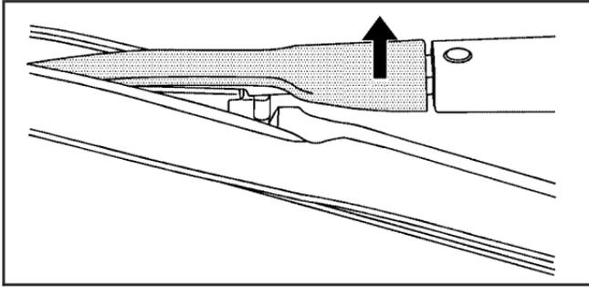
4. Lift up the wiper blade assembly cap.
