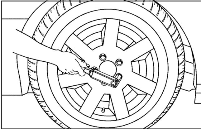
2. Loosen the wheel nuts, but do not remove them yet, using the wheel wrench. Turn the handle about 180 degrees, then return the handle back to the starting position. This avoids taking the wrench off the lug nut for each turn.
