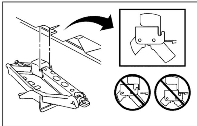
6. Raise the jack by turning the wheel wrench clockwise until the slots in the jack head fit into the metal flange located behind the V-shaped locating notches on the plastic molding as shown.
