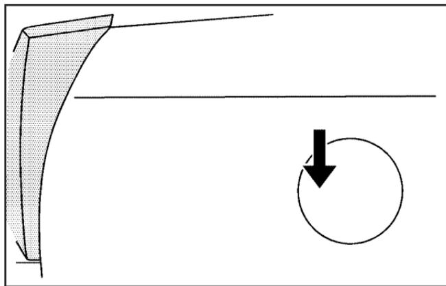
The fuel cap is behind a hinged fuel door on the passenger's side of the vehicle. The fuel door is opened by pushing in on the rear edge until the door pops out.
