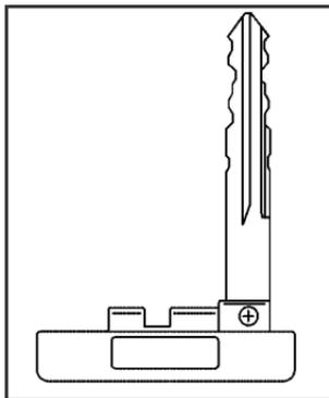
This key, located inside the keyless access transmitter, can be used for the driver's door, glove box, and rear seat pass-through door. See "Rear Seat Pass-Through Door" under *Trunk* on page 2-20 for more information.
