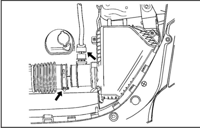
3. Disconnect electrical connector from air box.
