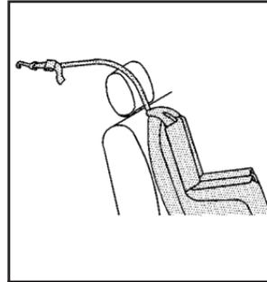
If the position you are using has a fixed head restraint and you are using a single tether, route the tether over the head restraint.
