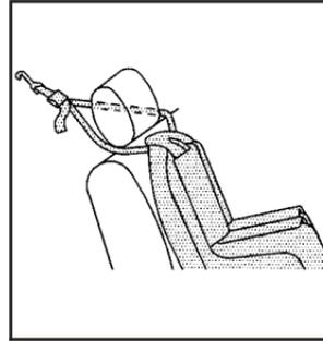
If the position you are using has a fixed head restraint and you are using a dual tether, route the tether around the head restraint.
