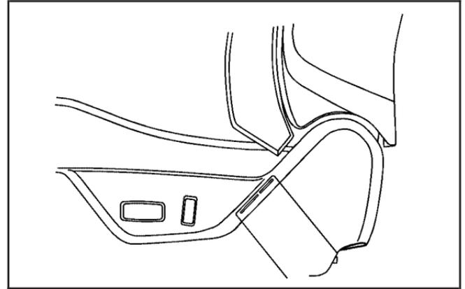
If your seats have power reclining seatbacks, use the vertical power seat control located on the outboard side of each seat.
