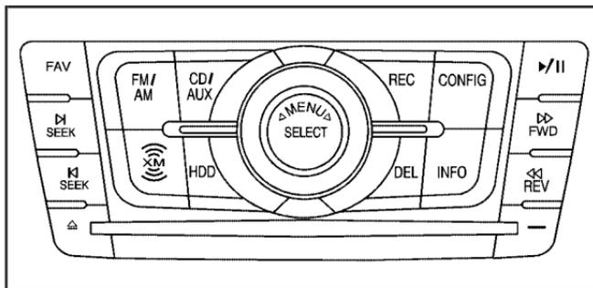
**Partial View of Radio with DVD Audio, Hard Disc Drive (HDD), and USB**
