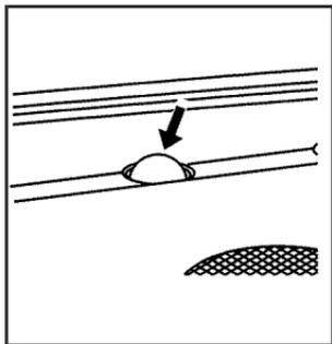
The light sensor for the DRL and AUTO headlamp feature is located on top of the instrument panel. If the sensor is covered, it will prevent it from sensing light, and the exterior lamps or the Headlamps Suggested message will appear on the DIC whenever the ignition is on.
