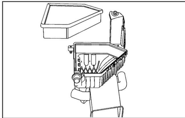
8. Remove the air cleaner element from the air cleaner housing.
