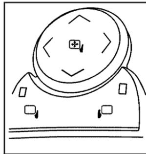
The control on the driver side door operates both outside rearview mirrors.
