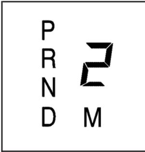
The tachometer display on the instrument panel cluster will show which gear the vehicle is in and a number indicating the requested gear range when moving the shift lever forward or rearward. See *Speedometer and Odometer on page 3-31* for more information on the odometer.
