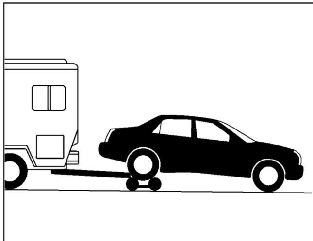
Your vehicle can be towed using a dolly. To tow your vehicle using a dolly:
