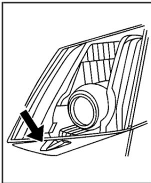
The headlamp washers are located beneath the headlamps.
