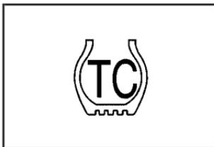
Press the TC (Traction Control) button, located on the instrument panel, to turn the system off.
