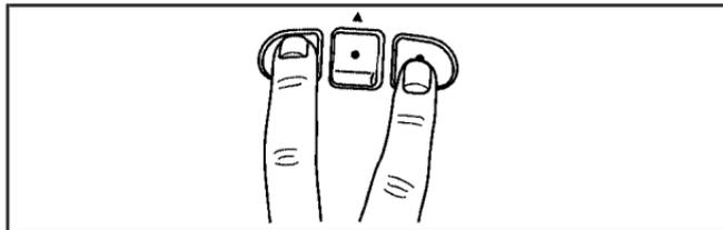
1. Press and hold down the two outside buttons until the indicator light begins to flash, after 20 seconds.
