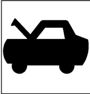
1. Pull the hood release lever with this symbol on it. It is located inside the vehicle on the lower left side of the instrument panel.
