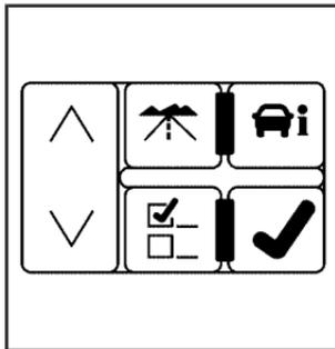
The Driver Information Center (DIC) has different displays which can be accessed by pressing the DIC buttons located on the instrument panel, next to the steering wheel.
