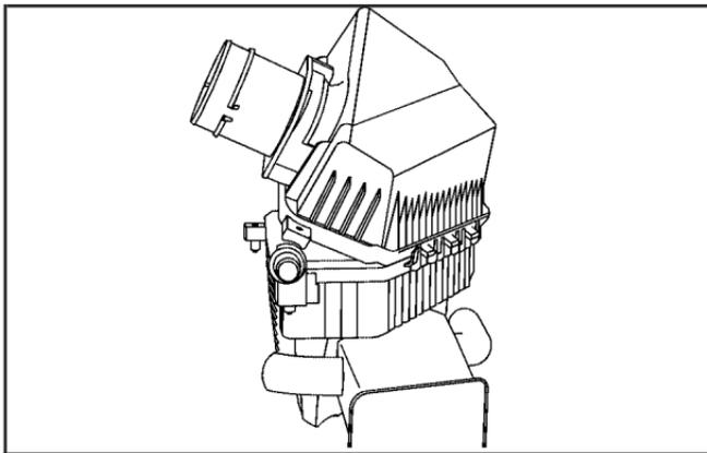
7. Pivot the air cleaner housing cover and remove the cover from the air cleaner housing.
