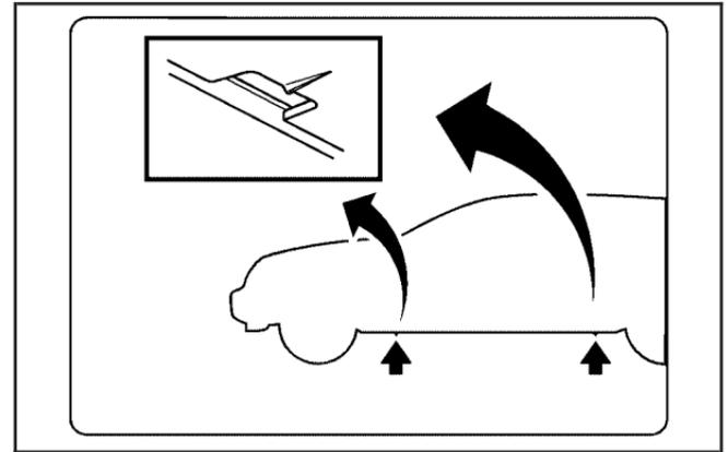
3. Find the jacking location using the diagram above and corresponding V-shaped locating notches located in the plastic molding.
