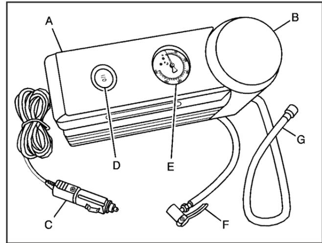
4. Place the sealant and compressor kit on the ground and unwrap the sealant/air hose (G) from the compressor.
