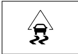
The Traction Control System/StabiliTrak<sup>®</sup> warning light should come on briefly when the engine is started.
