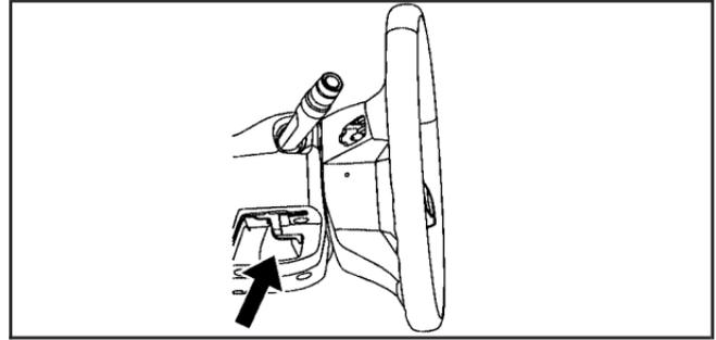
The tilt and telescope lever is located on the left side of the steering column.
