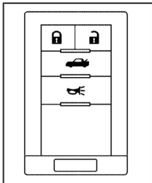
**🔒 (Lock):** Press 🔒 to lock all the doors. If enabled through the Driver Information Center (DIC), the parking lamps may flash once to indicate locking has occurred, or the horn may chirp when 🔒 is pressed again
