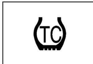
To turn the system off, press the TCS/StabiliTrak<sup>®</sup> button located on the console under the climate controls.
