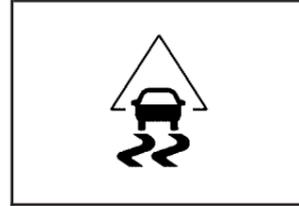
The traction control system warning light comes on briefly while starting the engine.
