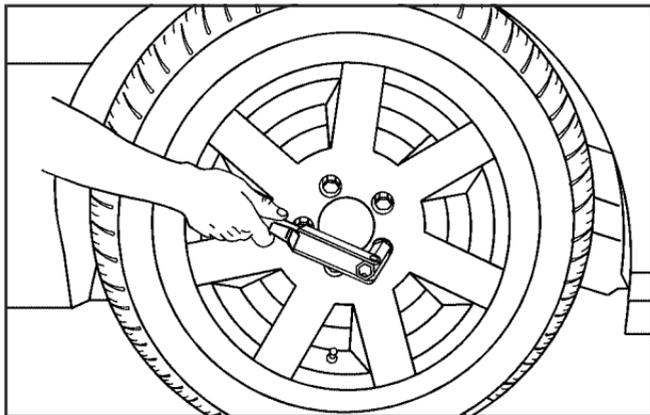
2. Loosen the wheel nuts, but do not remove them yet, using the wheel wrench. Turn the handle about 180 degrees, then flip the handle back to the starting position. This avoids taking the wrench off the lug nut for each turn.
