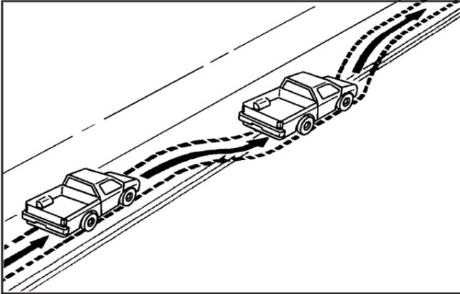
If the level of the shoulder is only slightly below the pavement, recovery should be fairly easy. Ease off the accelerator and then, if there is nothing in the way, steer so that your vehicle straddles the edge of the pavement. Turn the steering wheel 3 to 5 inches, 8 to 13 cm, (about one-eighth turn) until the right front tire contacts the pavement edge. Then turn the steering wheel to go straight down the roadway.
