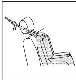
If the position you are using has an adjustable headrest or head restraint and you are using a dual tether, route the tether under the head restraint and in between the head restraint posts.
