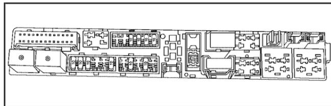
To access the fuse block, push in the two tabs located at each end of the fuse block cover. Then lift the cover off.
