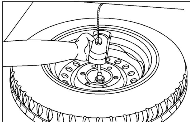
5. Tilt the retainer (C) and slip it through the wheel opening to remove the spare tire from the cable (B).
