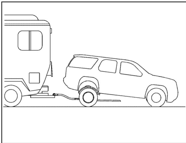
Rear-Wheel Drive (RWD) vehicles, can be towed using a dolly. All-Wheel-Drive (AWD) vehicle, can only be towed on a flat-bed trailer.
