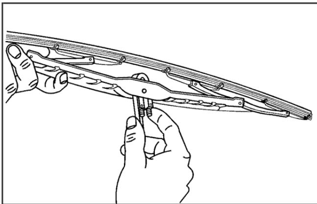
4. Lift the wiper blade assembly up so it is in a T-shaped position. You should be able to see a tab.
