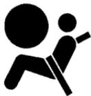
There is an airbag readiness light on the instrument panel cluster, which shows the airbag symbol.
