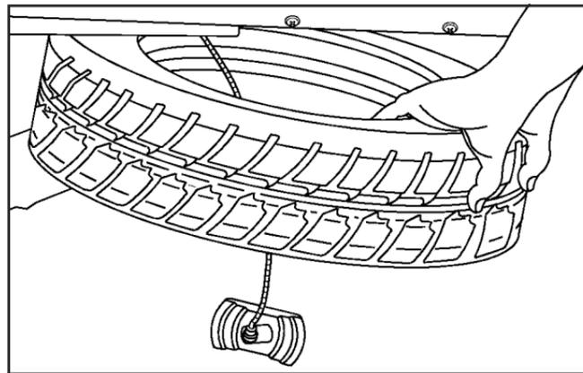
5. Turn the wheel wrench clockwise to raise the jack until it lifts the secondary latch spring.
