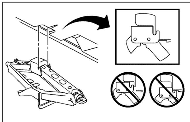
6. Raise the jack by turning the wheel wrench clockwise until the slots in the jack head fit into the metal flange located behind the triangle on the plastic molding as shown.
