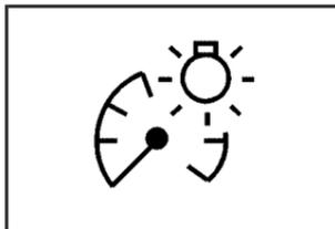
Turn the knob clockwise or counterclockwise to brighten or dim the interior lights.
