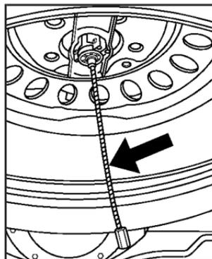
2. If the cable is visible, place the wrench on the hoist drive nut and turn the wrench counterclockwise until approximately 6 inches (15 cm) of cable is exposed.
