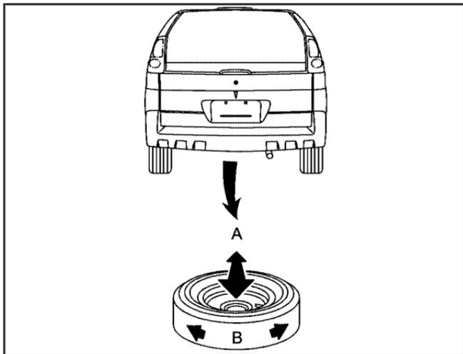
8. Make sure the tire is stored securely. Push, pull (A), and then try to turn the tire (B). If the tire moves, use the wheel wrench to tighten the cable.
