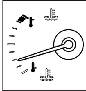
This gage shows the engine coolant temperature.
