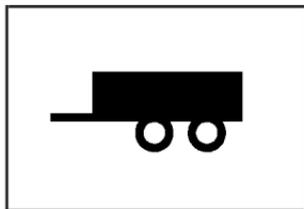
This indicator light on the instrument panel cluster comes on when the tow/haul mode is on.
