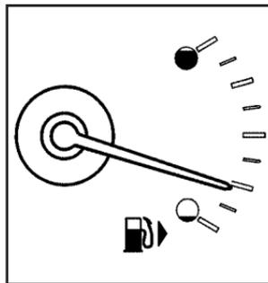
The fuel gage shows approximately how much fuel is in the fuel tank. It works only when the engine is on.
