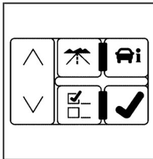
The Driver Information Center (DIC) has different displays which can be accessed by pressing the DIC buttons located on the instrument panel, to the left of the steering wheel.
