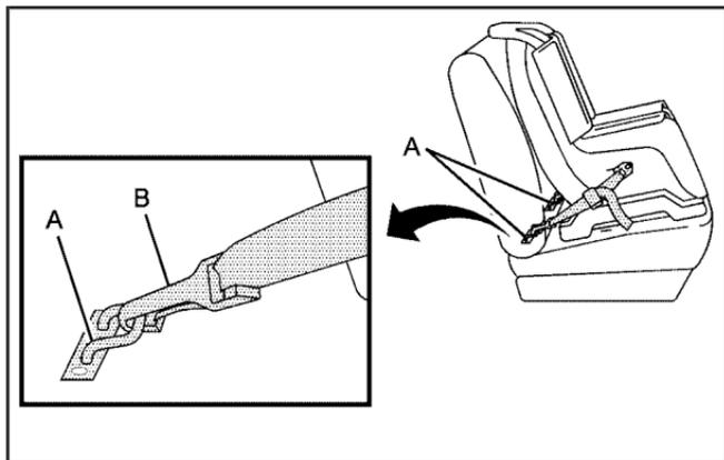
Lower anchors (A) are metal bars built into the vehicle. There are two lower anchors for each LATCH seating position that will accommodate a child restraint with lower attachments (B).
