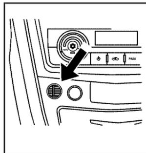
There is an interior temperature sensor located below the climate control system next to the steering wheel.
