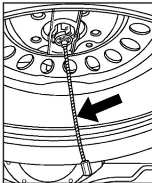
1. Check under the vehicle to see if the cable is visible. If it is not visible, see *Secondary Latch System* on page 5-82.
