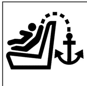
To assist you in locating the top tether anchors, the top tether anchor symbol is located near the top tether anchors.
