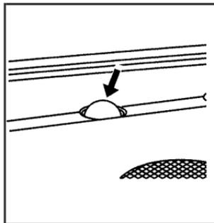
There is a solar sensor located on top of the instrument panel, near the windshield.
