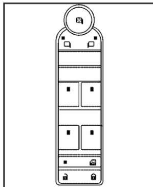
The power window switches are located on the armrest near each window.
