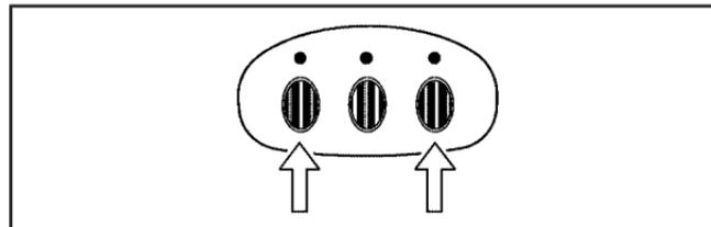
1. From inside the vehicle, press the two outside buttons at the same time for one to two seconds, and immediately release them.
