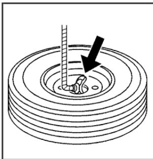
10. Tilt the retainer and slip it through the wheel opening when the spare tire has been completely lowered.
