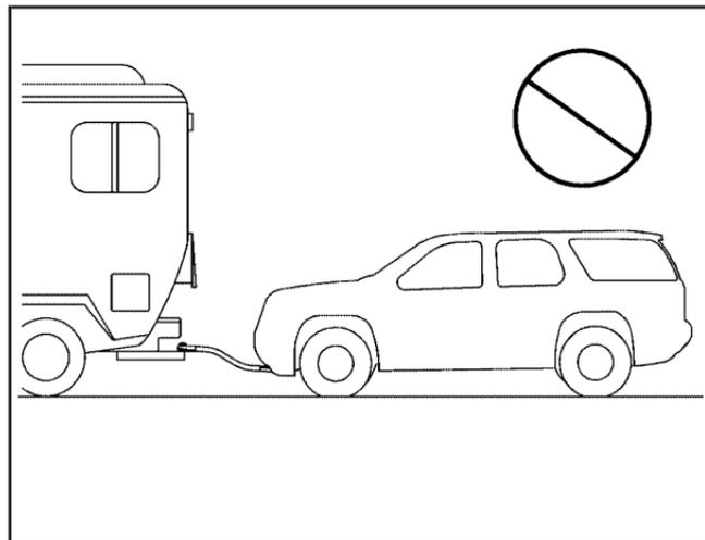
**Notice:** If the vehicle is towed with all four wheels on the ground, the drivetrain components could be damaged. The repairs would not be covered by the vehicle warranty. Do not tow the vehicle with all four wheels on the ground.
