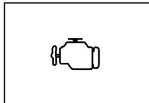
This light should come on when the ignition is on, but the engine is not running, as a check to show it working.
