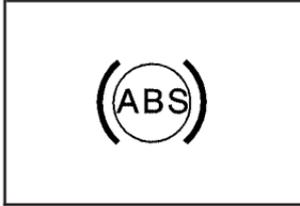
For vehicles with the Antilock Brake System (ABS), this light comes on briefly when the engine is started.
