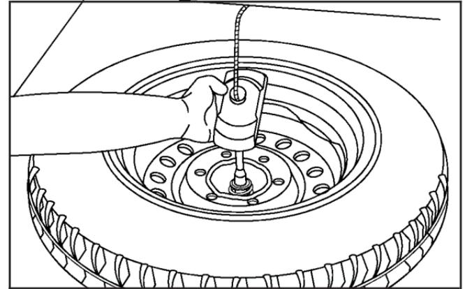
3. Tilt the retainer downward and slip it through the center hole of the spare tire.
