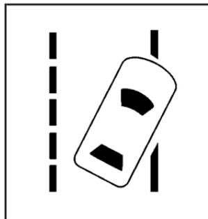
When the vehicle is started, the LDW symbol, located in the instrument panel cluster, will briefly come on to indicate that the light is operational.
