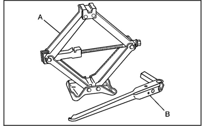
4. Turn the wing nut to remove the retainer that holds the wrench and jack.
