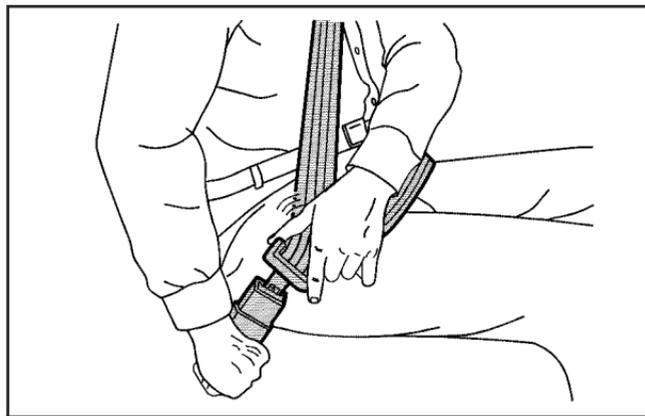
3. Push the latch plate into the buckle until it clicks. If the latch plate will not go fully into the buckle, check if the correct buckle is being used. Pull up on the latch plate to make sure it is secure. If the belt is not long enough, see *Safety Belt Extender on page 2-33*. Position the release button on the buckle so that the safety belt could be quickly unbuckled if necessary.
