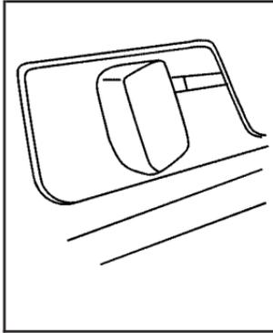
The adjustment lever is located on the left side of the steering column.
