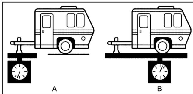
Using a weight-carrying hitch, the trailer tongue (A) should weigh 10 to 15 percent of the total loaded trailer weight (B).
