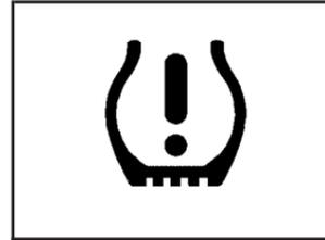
The Tire Pressure Monitor alerts you when a significant reduction in pressure occurs in one or more of the vehicle's tires by illuminating the low tire pressure warning light on the instrument cluster.
