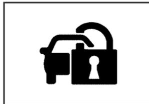
The security light is located on the instrument panel cluster.
