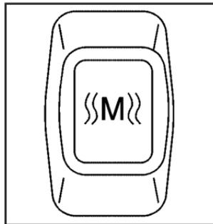
On vehicles with this feature, the switch is located on the outboard side of the front seats behind the lumbar switch.
