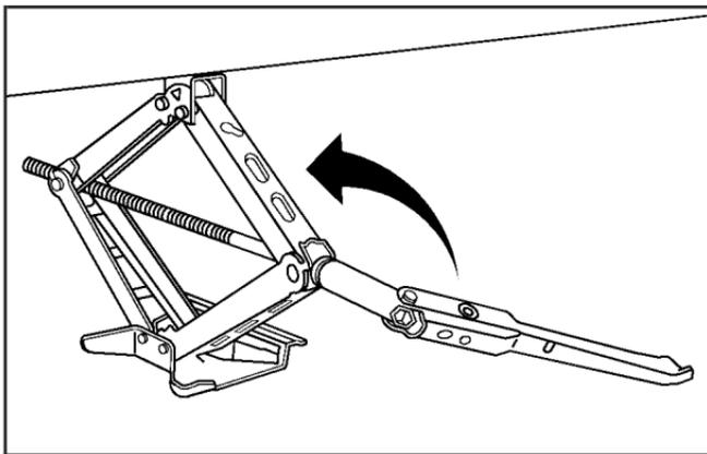
13. Lower the vehicle by turning the jack handle counterclockwise. Lower the jack completely.
