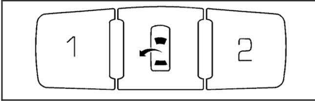
On vehicles with the memory package, the controls are located on the driver door panel. The controls are used to program and recall memory settings for the driver seat, outside mirror, and steering wheel position if the vehicle has the power tilt wheel and telescopic steering feature.
