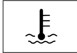
The engine coolant temperature warning light comes on when the engine is very hot.
