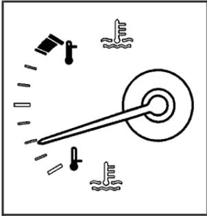
This gage shows the engine coolant temperature.
