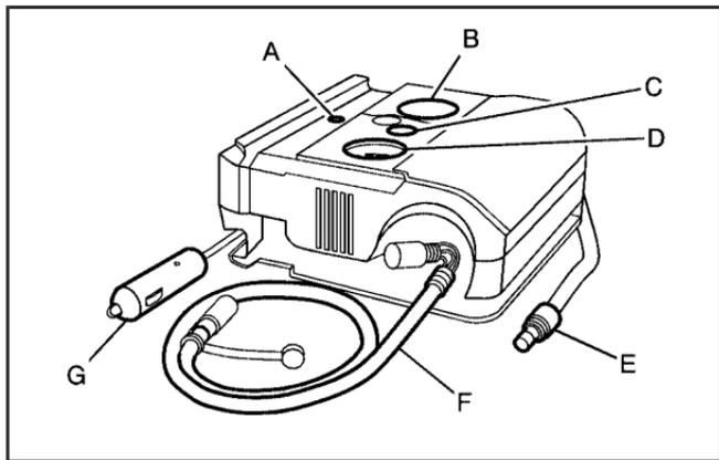
When using the tire sealant and compressor kit during cold temperatures, warm the kit in a heated environment for 5 minutes. This will help to inflate the tire faster.
