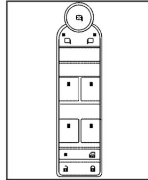
The power window switches are located on the driver door.
