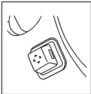
If the vehicle has this feature, the power tilt and telescope wheel control is located on the outboard side of the steering column.
