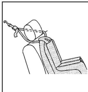
If the position you are using has a fixed or adjustable headrest or head restraint and you are using a dual tether, route the tether around the headrest or head restraint.
