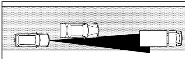
If another vehicle enters the same lane as you, ACC will not detect the vehicle until it is completely in the lane. Be ready to take action and apply the brakes yourself.
