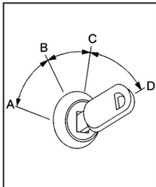
In order to shift out of P (Park), ignition must be in the ON/RUN or ACC/ACCESSORY and the brake pedal must be applied.
