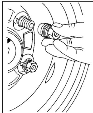
12. Put the wheel nuts back on with the rounded end of the nuts toward the wheel. Tighten each nut by hand until the wheel is held against the hub.
