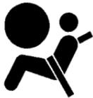
There is an airbag readiness light on the instrument panel, which shows the airbag symbol.
