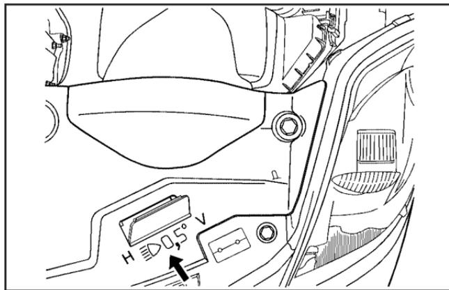
7. Locate the vertical headlamp aiming screws. They are located under the hood near each headlamp assembly. First lift the flap to access either of them. Each one is the top outboard screw by the "V" on the cover panel next to the aiming flap.
