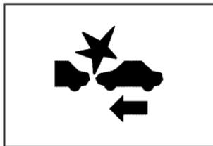
The ACC alert symbol is located on the display at the top of the instrument panel to the right of the driver.
