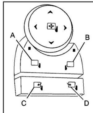
Controls for the outside power mirrors are located on the driver door armrest.
