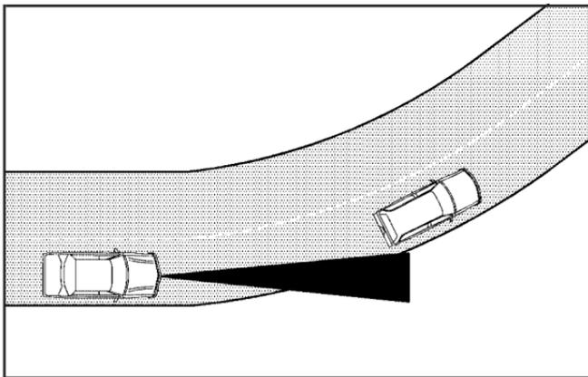
When following a vehicle and entering a curve, ACC could lose track of the vehicle in your lane and accelerate your vehicle. When this happens the Vehicle Ahead symbol will not appear.
