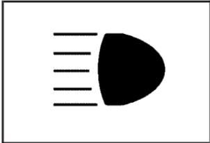
This light on the instrument panel cluster will be on, indicating high-beam usage.
