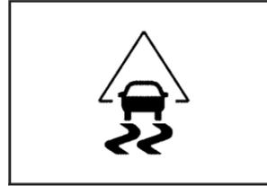
For vehicles with the StabiliTrak<sup>®</sup> system, this light comes on briefly while starting the engine.
