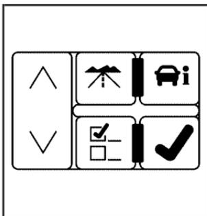
The DIC buttons are located on the instrument panel to the left of the steering wheel.
