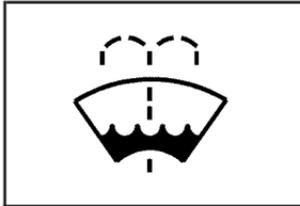
Open the cap with the washer symbol on it. Add washer fluid until the tank is full. See *Engine Compartment Overview* on page 6-12 for reservoir location.
