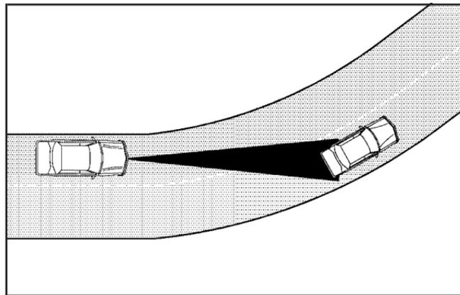
ACC may detect a vehicle that is not in your lane and apply the brakes.
