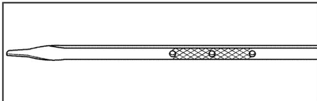
If the oil is below the cross-hatched area at the tip of the dipstick, add at least one quart/liter of the recommended oil. This section explains what kind of oil to use. For engine oil crankcase capacity, see *Capacities and Specifications on page 6-109*.
