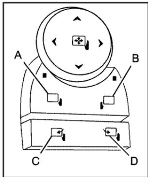
Controls for the outside power folding mirrors are located on the driver door armrest.
