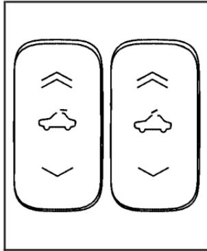
The switches that operate the sunroof are located on the overhead console.
