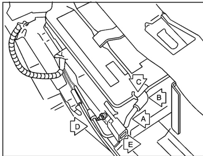
To be sure the vent hose (A) is properly attached, the vent hose connectors (B) must be securely reattached to the vent outlets (C) on each side of the battery and the vent assembly grommet (D) must be secured to the floor pan (E).
