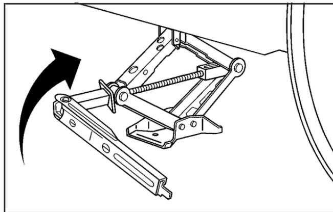
8. Raise the vehicle by turning the jack handle clockwise. Raise the vehicle far enough off the ground for the spare tire to fit under the vehicle.
