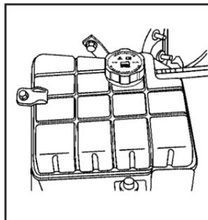
3. Fill the coolant surge tank with the proper mixture to the FULL COLD mark on the side of the coolant surge tank.
