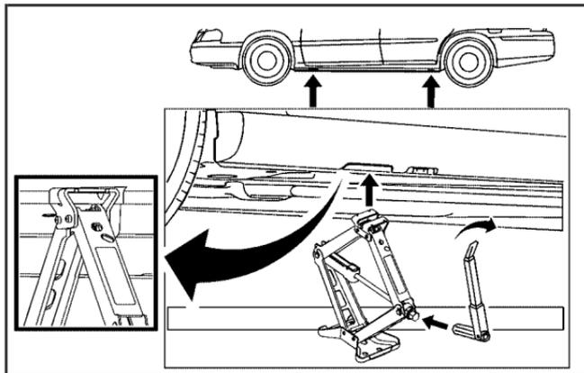
6. Raise the jack until the metal flange fits firmly into the channel of the jack head.
