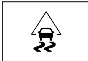
The TCS and StabiliTrak® light will flash when the system is limiting wheel spin.
