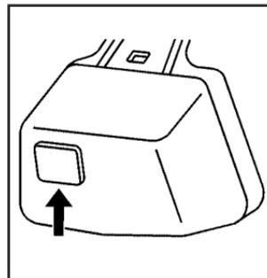
The light sensor is located on the inside of the vehicle in front of the inside rearview mirror.
