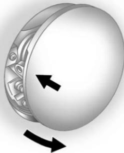
The cap is behind a locking fuel door on the passenger side of the vehicle. The fuel door is locked or unlocked every time the driver's door is locked or unlocked with the power door locks or the transmitter.
