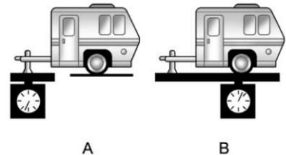
For a weight-carrying hitch, the trailer tongue (A) should weigh 10 to 15 percent of the total loaded trailer weight (B).
