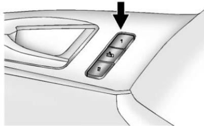
On vehicles with the memory feature, memory buttons 1 and 2 on the driver door are used to save and recall memory settings for the driver seat cushion and seatback, outside
