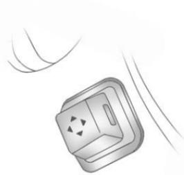
For vehicles with the power tilt wheel, the control is on the left side of the steering column.
