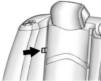
1. Pull forward on the tab, on the outboard side of the seatback, to unlock the seatback.
