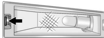
1. Push the tab to remove the license plate lamp.
