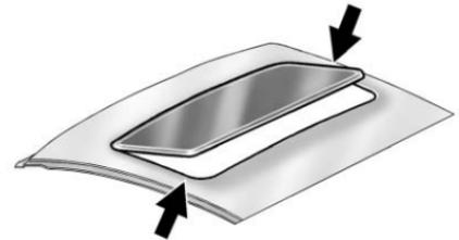
Dirt and debris may collect on the sunroof seal or in the track. This could cause an issue with sunroof operation, noise or plugging the water drainage system. Periodically open the sunroof and remove any obstacles or loose debris. Wipe the sunroof seal and roof sealing area using a clean cloth, mild soap, and water. Do not remove grease from sunroof.
