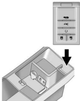
If moving the transmitter to different locations within the vehicle does not help, place the transmitter in the center console transmitter pocket with the buttons facing the front of the vehicle and then start the vehicle.
