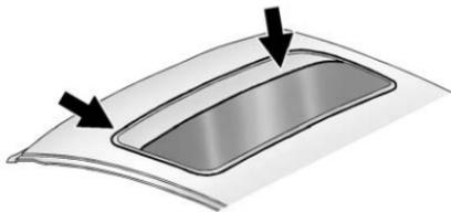
Dirt and debris may collect on the sunroof seal or in the track. This could cause an issue with sunroof
