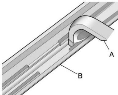
6. Levers must still be in the forward up position. Move the front crossrail forward beyond the cut-out area (B). For the rear crossrail, slide the crossrail assembly (A) rearward until the entire crossrail support is in first position beyond the channel cut-out area (B).
