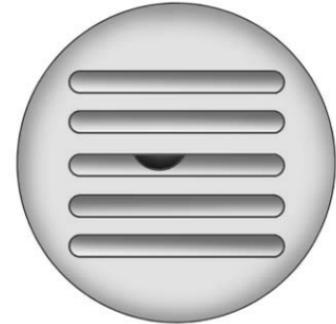
The interior temperature sensor, located on the instrument panel to the right of the steering wheel, measures the temperature of the air inside the vehicle.
