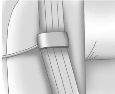
3. Be sure that the belt is not twisted and it lies flat. The elastic cord must be under the belt and the guide on top.
