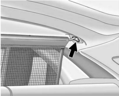
1. There are four installation points in the roof, two located in front of and two behind the rear seats.
