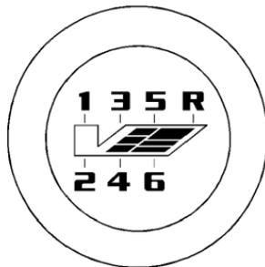
**1 (First):** Press the clutch pedal and shift into 1 (First). Slowly let up on the clutch pedal while pressing on the accelerator pedal.
