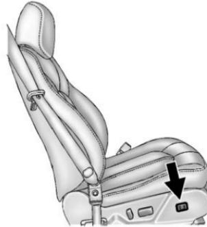
If available, hold the control on the outboard side of the seat forward or rearward to increase or decrease the lumbar support on the driver or front passenger seat.
