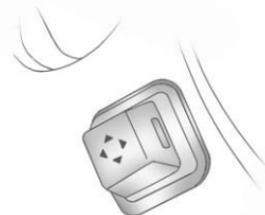
For vehicles with the power tilt wheel, the control is on the left side of the steering column.
