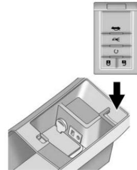
6. Place the new transmitter into the transmitter pocket with the buttons facing the front of the vehicle. The transmitter pocket is inside the center console storage area located between the driver and front passenger seats.
