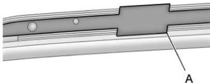
4. Locate the forward or rearward cut-out (A) in the siderail channel.
