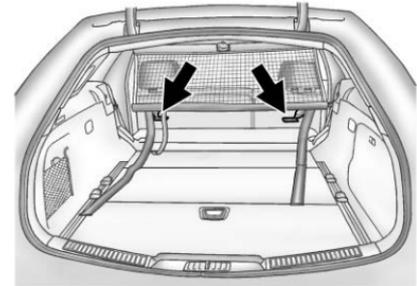
4. The net can also be mounted to the tethers on the back of the rear seats when the seats are upright.
