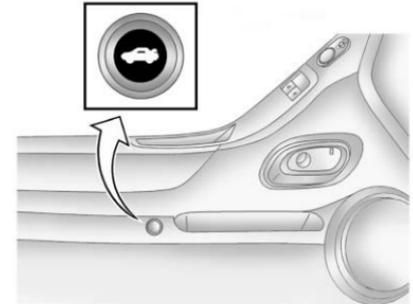
The remote trunk release button is on the driver door.
