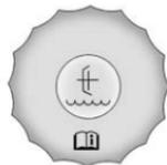
The hydraulic clutch fluid reservoir cap has this symbol on it. See *Engine Compartment Overview on page 10-6* for reservoir location.
