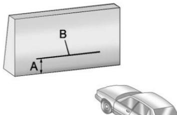
4. At a wall, measure from the ground upward (A) to the recorded distance from Step 3 and mark it.
