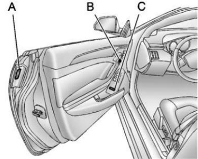
When you have the transmitter with you, you may also unlock and open the door by squeezing the door handle sensor (A). You do not have to press the unlock button on the transmitter. You will be able to open the door when you press the door handle sensor and the vehicle recognizes your keyless access transmitter. When the passenger door is opened first, the driver's door will also unlock.
