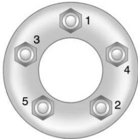
15. Tighten the wheel nuts firmly in a crisscross sequence as shown.
