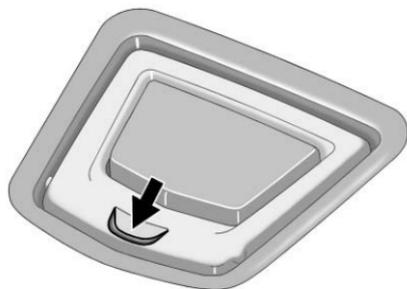
Press the bottom of the load floor handle assembly to lift the top on the handle. Pull up on the handle to open the cargo management system.
