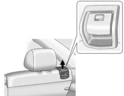
1. Pull on the lever, on the top outboard side of the seatback, to unlock the seatback.
