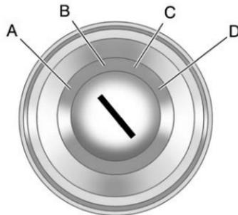
The ignition switch can be turned to four different positions.
