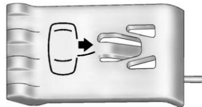
3. Pull the door release tab, located under the package shelf at the top of the trunk, to unlock and unlatch the driver door.
