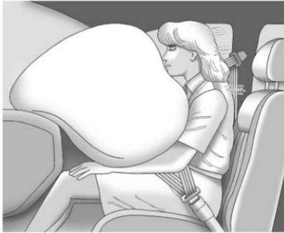
The outboard front passenger frontal airbag is in the instrument panel on the passenger side.
