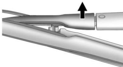
4. Lift up the wiper blade assembly cap.
