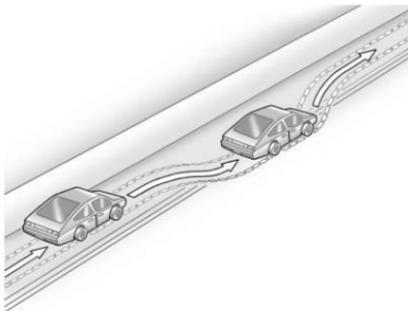
If the level of the shoulder is only slightly below the pavement, recovery should be fairly easy. Ease off the accelerator and then, if there is nothing in the way, steer so that the vehicle straddles the edge of the pavement. Turn the steering wheel 8 to 13 cm (3 to 5 in), about one-eighth turn, until the right front tire contacts the
