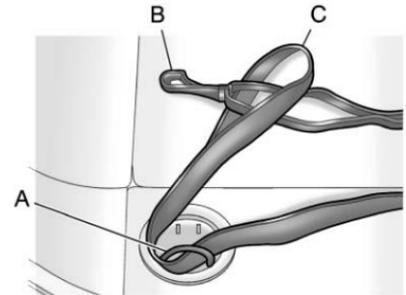
4. Route the loop end of the strap (C) through one of the cargo tie-downs (A) located in the rear of the vehicle.
