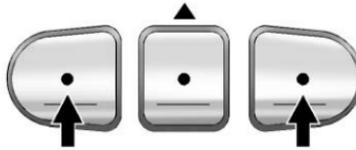
1. From inside the vehicle, press and hold down the two outside buttons at the same time, releasing only when the Universal Home Remote indicator light begins to flash, after 20 seconds. This step will erase the factory settings or all previously programmed buttons.
