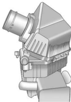
7. Move the air cleaner housing cover and remove the cover from the air cleaner housing.
