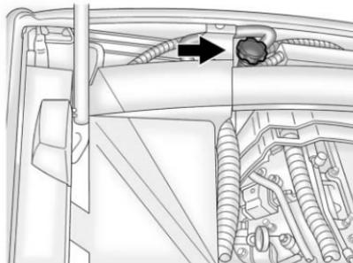
1. Remove the intercooler system pressure cap when the intercooler system hoses are no longer hot. Turn the pressure cap slowly counterclockwise about one-quarter of a turn. If you hear a hiss, wait for that to stop. This allows any pressure still left to be vented.
