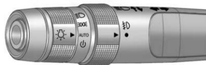
The exterior lamp control is located toward the end of the turn signal/lane change lever.
