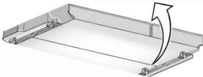
The loop of the D-Ring slider must be facing inward toward the storage area and the ring must be in the up position for proper usage.
