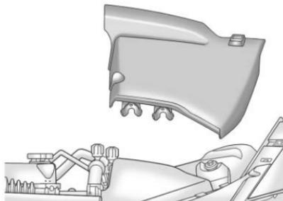
2. Remove the side cover by pulling up on the front of the cover.
