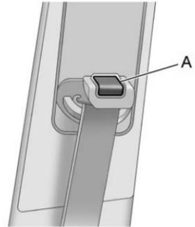
Push down on the release button (A) and move the height adjuster to the desired position. The adjuster can be moved up by pushing up on the shoulder belt guide.
