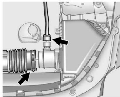
3. Disconnect the electrical connector from the air box.
