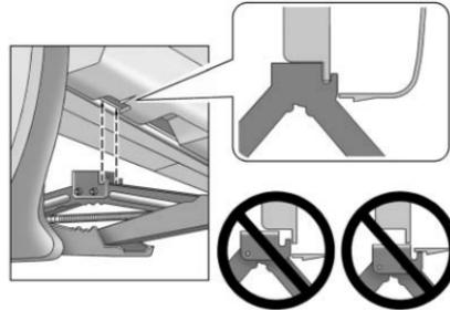
6. Raise the jack by turning the wheel wrench clockwise until the slots in the jack head fit into the metal flange located behind the V-shaped locating notches on the plastic molding as shown.
