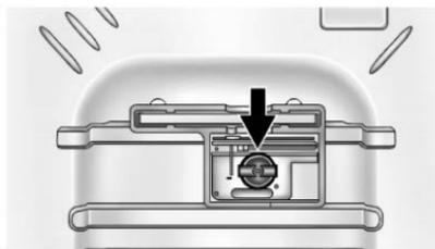
2. Remove the retainer that holds the tire sealant and compressor kit in place.
