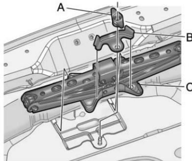
1. Remove the retainer nut (A).
