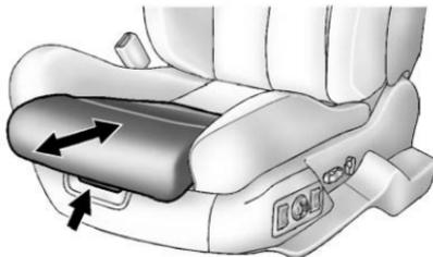
If available, adjust the manual leg extension by reaching under it, in the pocketed area. Press the button and pull or push to lengthen or shorten it. Release the button to lock it in place.
