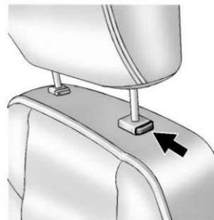
Pull the head restraint up to raise it. To lower the head restraint, press the button, located on the top of the seatback, and push the restraint down.
