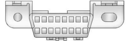
The DLC is under the instrument panel to the left of the steering wheel. See your dealer if assistance is needed.
