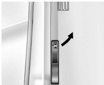
1. From inside the vehicle, use the door release handle located on the floor next to each seat. Pull the handle up to unlock and unlatch the door.
