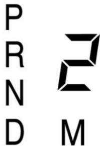
The tachometer display indicates which gear the vehicle is in. The number indicates the requested gear range when moving the shift lever forward or rearward.
