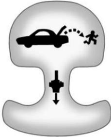
**Notice:** Do not use the emergency trunk release handle as a tie-down or anchor point when securing items in the trunk as it could damage the handle. The emergency trunk release handle is only intended to aid a person trapped in a latched trunk, enabling them to open the trunk from the inside.
