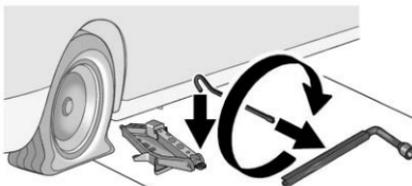
4. Insert the hooked end of the extension handle through the jack and the flat end through the wheel wrench.
