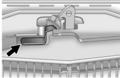
2. Go to the front of the vehicle and find the secondary hood release lever. The lever is located under the front edge of the grille near the center. Push the release lever up and raise the hood.
