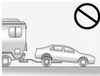
**Notice:** Towing an all-wheel-drive vehicle with all four wheels on the ground, or even with only two of its wheels on the ground, will damage drivetrain components. Do not tow an all-wheel-drive vehicle with any of its wheels on the ground.
