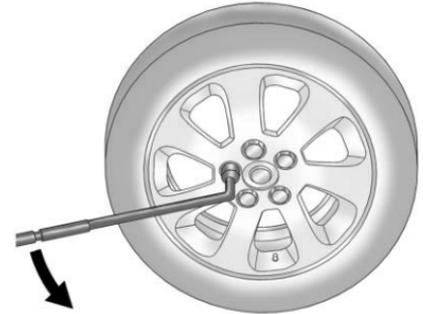
2. Use the wrench to loosen all the wheel nuts. Do not remove them yet.
