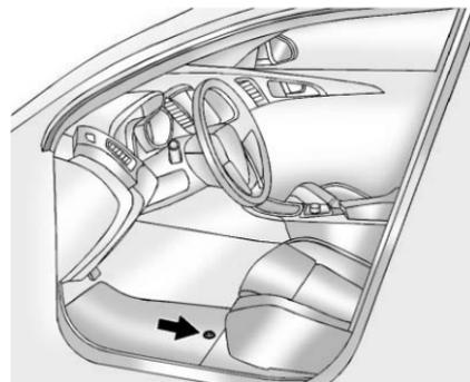
1. Pull up on the rear of the floor mat to unlock the retainer and remove.
