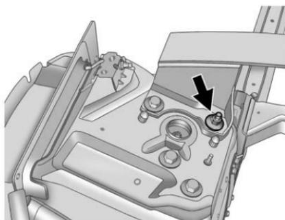
Your vehicle has a remote negative (-) ground location, as shown in the illustration. It is located on the left side of the engine compartment. See *Engine Compartment Overview* on page 10-6. You should always use this remote ground location, instead of the terminal on the battery.
