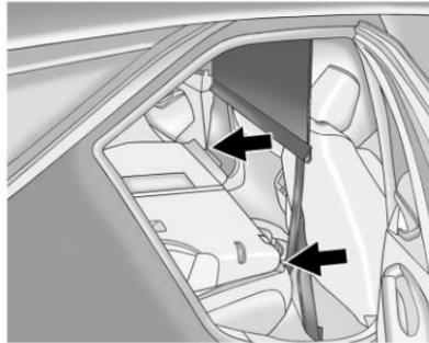
3. Mount the cargo net to the rear seat tethers located on the front of the bottom cushions.
