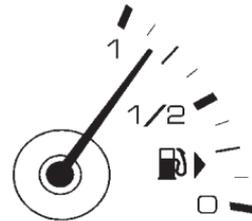
When the ignition is on, the fuel gauge indicates how much fuel is left in the tank.
