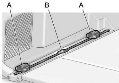
To install the D-Ring slider (A), insert it into the channel (B) located in the middle of each rail.
