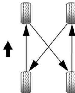
Use the rotation pattern shown here when rotating tires of the same size installed on all four wheel positions.
