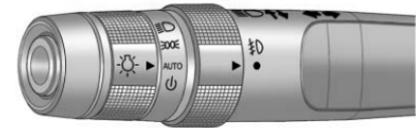
The exterior lamp control is located toward the end of the turn signal/ lane change lever.
