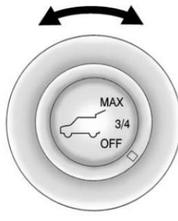
The power liftgate mode selector switch is located on the driver door. The vehicle must be in P (Park) to use the power feature. The taillamps flash when the power liftgate moves.
