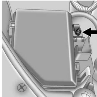
6. Connect the red positive (+) cable to the positive (+) terminal of the dead battery. Use a remote positive (+) terminal if the vehicle has one.
