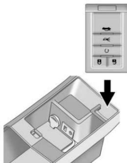
2. Place the new transmitter into the transmitter pocket with the buttons facing the front of the vehicle. The transmitter pocket is inside the center console storage area located between the driver and front passenger seats.
