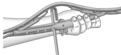
7. Reinstall the wiper blade assembly by sliding it over the wiper arm to engage the J-hooked end. Pull up on the assembly to lock it into place.
