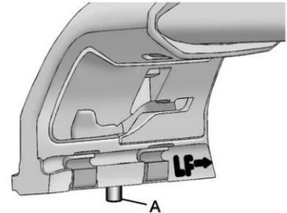
3. The crossrail supports are labeled with an arrow that needs to point toward the front of the vehicle. A pin (A) will be visible on the bottom when the crossrail support lever is down. To install the crossrail support, move the lever into the forward upper position, the pin (A) will not be visible.
