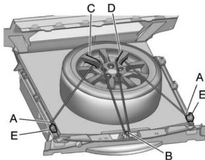
4. Route one of the hooks (A), at the end of the cable provided, through the liftgate striker (B).
