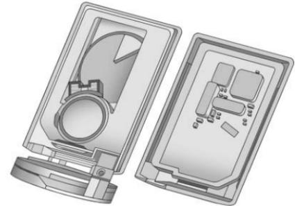
1. Separate the transmitter with a flat, thin object inserted into the slot on the side or back of the transmitter.
