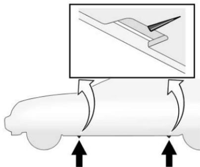
3. Find the jacking location using the diagram above and corresponding V-shaped locating notches located in the plastic molding.
