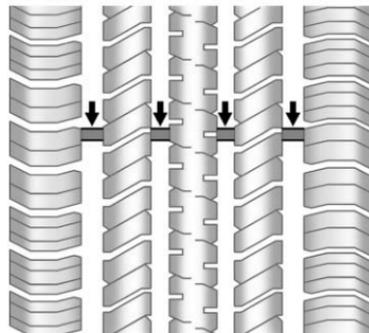
One way to tell when it is time for new tires is to check the treadwear indicators, which appear when the tires have only 1.6 mm (1/16 in) or less of tread remaining. See *Tire*
