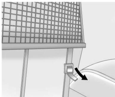
5. Pull on the straps to tighten the net.
