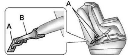
Lower anchors (A) are metal bars built into the vehicle. There are two lower anchors for each LATCH seating position that will accommodate a child restraint with lower attachments (B).
