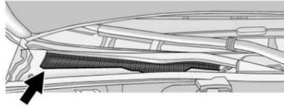
The passenger compartment air filter is located under the hood below the windshield wiper arm and the screen on the passenger side of the vehicle. See *Engine Compartment Overview on page 10-6* for more information on location.
