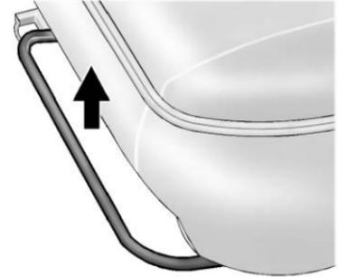
1. Lift the bar to unlock the seat.
