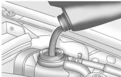
3. Fill the coolant surge tank with the proper mixture, to slightly above the FROID/FULL COLD line on the side of the coolant surge tank.
