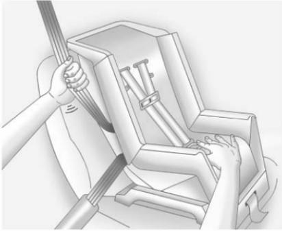
5. To tighten the belt, push down on the child restraint, pull the shoulder portion of the belt to tighten the lap portion of the belt, and feed the shoulder belt back into the retractor. When installing a forward-facing child restraint, it may be helpful to use your knee to push down on the child restraint as you tighten the belt. Try to pull the belt out of the retractor to make sure the retractor is locked. If the retractor is not locked, repeat Steps 4 and 5.
