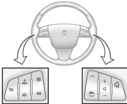
Some audio steering wheel controls could differ depending on the vehicle's options. Controls that can be adjusted at the steering wheel may include:
