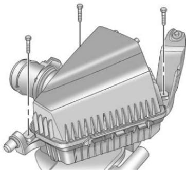
6. Remove the three air cleaner housing cover screws.
