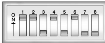
Example of Eight Dip Switches with Two Positions
