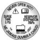
The CAC bottle pressure cap can be removed when the Charged Air Coolant cooling system, including the CAC bottle pressure cap, is no longer hot.
