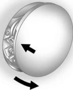
If equipped, the fuel door is locked when the vehicle doors are locked. Press
