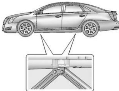
8. Position the jack lift head at the jack location nearest the flat tire, as shown. The jack must not be used in any other position.
