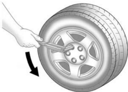
3. Turn the wheel wrench counterclockwise to loosen all the wheel nuts, but do not remove them yet.
