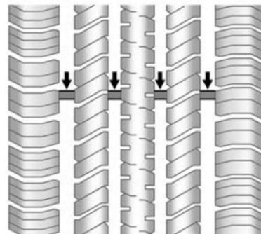
Treadwear indicators are one way to tell when it is time for new tires. Treadwear indicators appear when the tires have only 1.6 mm (1/16 in) or less of tread remaining. See *Tire Inspection* on page 10-52 and *Tire Rotation* on page 10-52.
