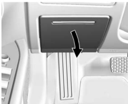
The instrument panel fuse block is in the instrument panel, on the driver side of the vehicle. To access the fuses, open the fuse panel door by pulling down at the top.
