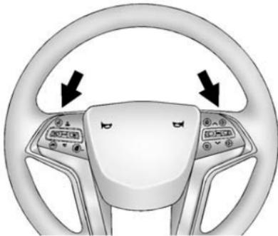
Tap Shift allows the driver to manually control the automatic transmission. To use Tap Shift, the shift lever must be in M (Manual Mode). If equipped, the controls are
