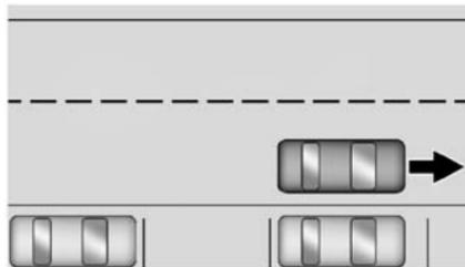
After completely passing a large enough space, an audible beep occurs and a red symbol displays in the DIC.
