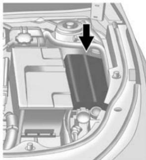
To remove the fuse block cover, squeeze the three retaining clips on the cover and lift it straight up.
