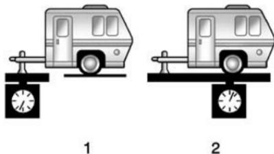
The trailer tongue (1) should weigh 10 % of the total loaded trailer weight (2).
