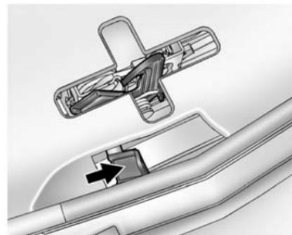
2. Go to the front of the vehicle to find the secondary hood release handle. The handle is under the front edge of the hood near the center. Push the handle to the right and at the same time raise the hood.
