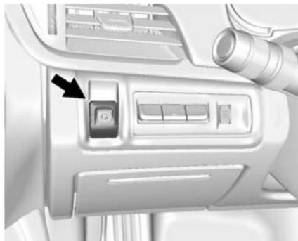
The EPB switch is on the left side of the instrument panel. The EPB can always be activated, even if the ignition is off. To prevent draining the battery, avoid repeated cycles of the EPB when the engine is not running.
