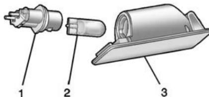
4. Pull the bulb (2) straight out of the bulb socket (1).
