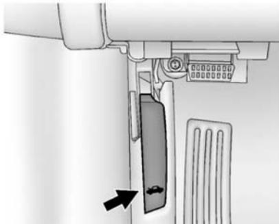
1. Pull the hood release lever with this symbol on it. It is inside the vehicle on the lower side of the instrument panel.
