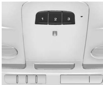
If equipped, this system provides a way to replace up to three remote control transmitters used to activate devices such as garage door openers, security systems, and home automation devices.
