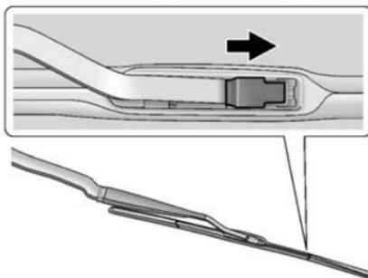
2. Lift up on the latch in the middle of the wiper blade where the wiper arm attaches.
