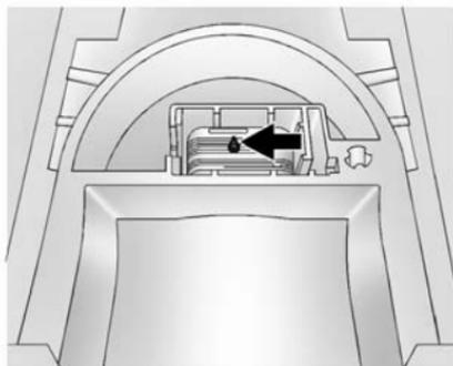
3. Turn the wing nut counterclockwise to remove it.
