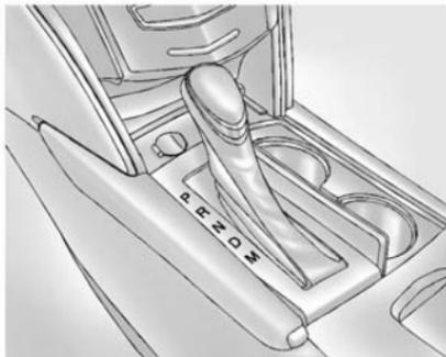
**P (Park):** This position locks the wheels. It is the best position to use when starting the engine because the vehicle cannot move easily.
