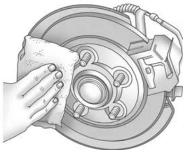
12. Remove any rust or dirt from the wheel bolts, mounting surfaces, and spare wheel.
