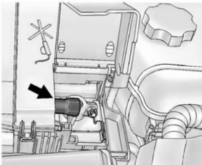
The vehicle has a remote positive (+) terminal under a trim cover. It is under the battery cover
