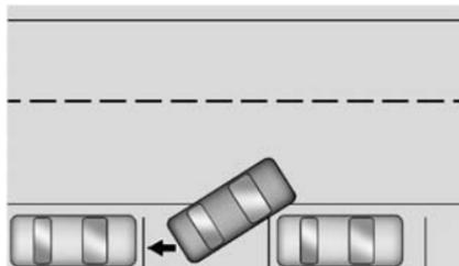
APA will instruct the vehicle to stop once a large enough space is found. Follow the instructions in the DIC. When instructed to drive in reverse, shift to R (Reverse) to engage automatic steering. The steering wheel will vibrate briefly as a reminder to remove hands from the steering wheel. Check surroundings and continue braking or accelerating as needed, and be prepared to stop
