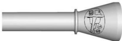
1. Locate the capless funnel adapter from within the vehicle.
