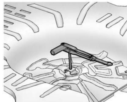
1. Turn the wrench counterclockwise to remove the fastener rod.
