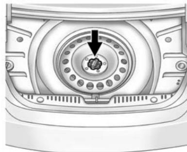
3. Turn the retainer nut counterclockwise and remove the spare tire. Place the spare tire next to the tire being changed.
