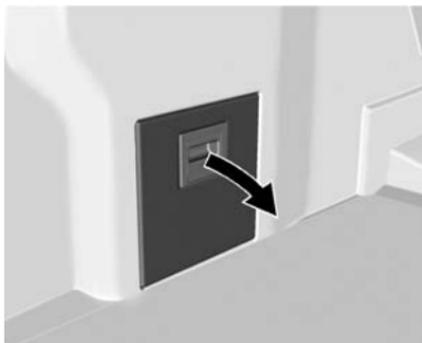
The rear compartment fuse block is on the left side of the trunk behind a cover.
