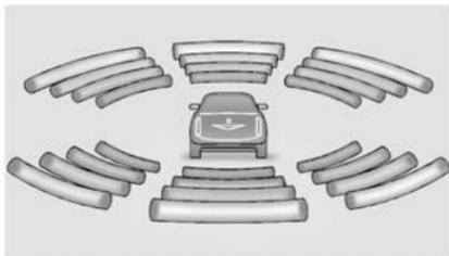
The instrument cluster may have a parking assist display with bars that show “distance to object” and object location information for RPA, and on some vehicles, for the Front Parking Assist system. As the object gets closer, more bars light up and the bars change color from yellow to amber to red.
