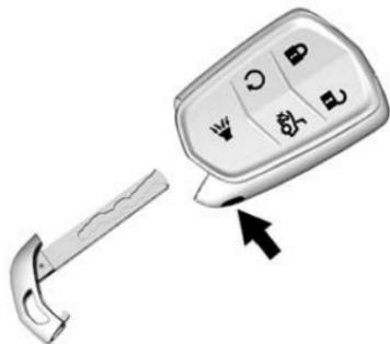
There is a key inside the Remote Keyless Entry (RKE) transmitter that is used for locking/unlocking the
