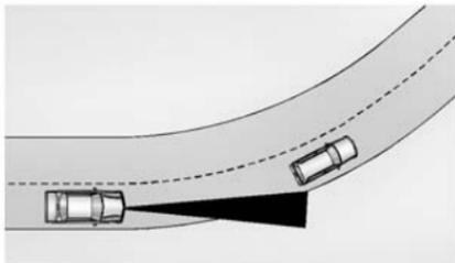
When following a vehicle and entering a curve, ACC may not detect the vehicle ahead and accelerate to the set speed. When this happens, the vehicle ahead symbol will not appear.
