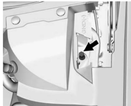
The vehicle has a remote negative (-) ground location. It is located on the driver side of the engine compartment. See *Engine Compartment Overview* on page 10-5. Always use this remote ground location, instead of the terminal on the battery.
