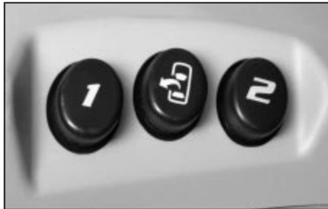
Your vehicle is equipped with the memory package. The controls for these features are located on the driver's seat, and are used to program and recall memory settings for the driver's seating positions.
