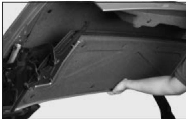
7. Move the rear tonneau rearward and up to the stored position. Pull from the center of the tonneau to keep pressure even. The rubber bumper on each corner will fit against the underside of the trunk decklid.
