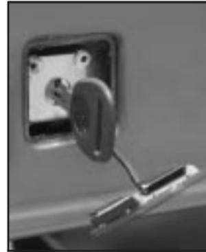
If the vehicle has lost battery power, you can still open the trunk using the key.
