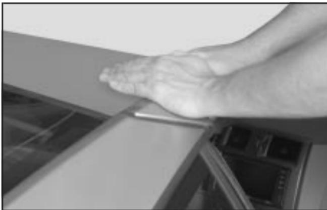
21. From outside the vehicle, push down on both rear corners of the top to make sure it is completely locked into place.
