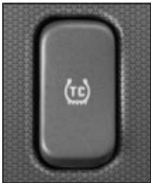
To turn the system off, press the traction control button located on the center console.
