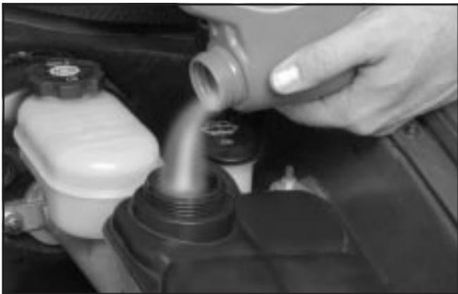
3. Then fill the coolant surge tank with the proper mixture to the full cold fill mark on the front of the coolant surge tank.
