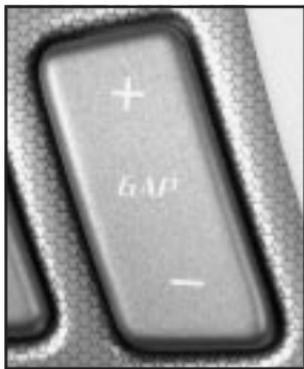
Use the GAP button on the steering wheel to adjust the follow distance.
