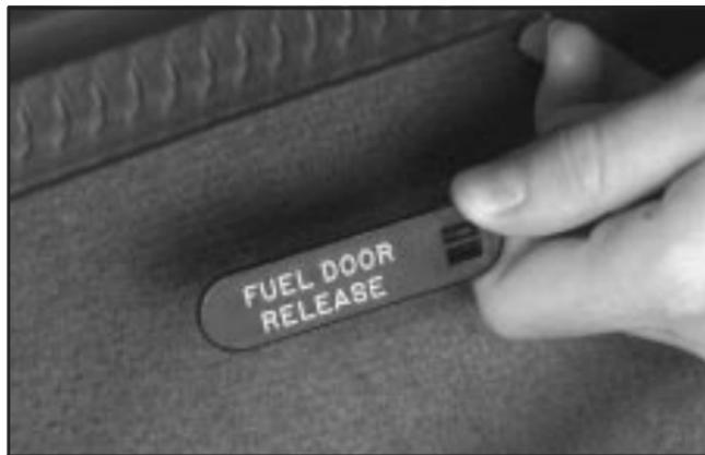
An alternate fuel door release is located inside the trunk behind a panel on the driver's side. Pull the handle to release the fuel door.
