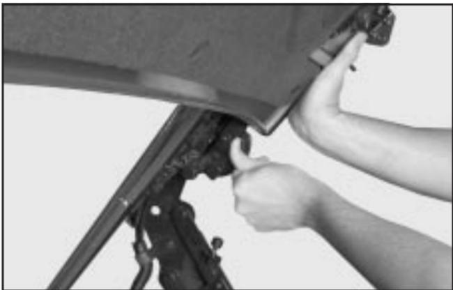
8. Push both sides of the rear tonneau over-center link up until they stop to lock the linkage.
