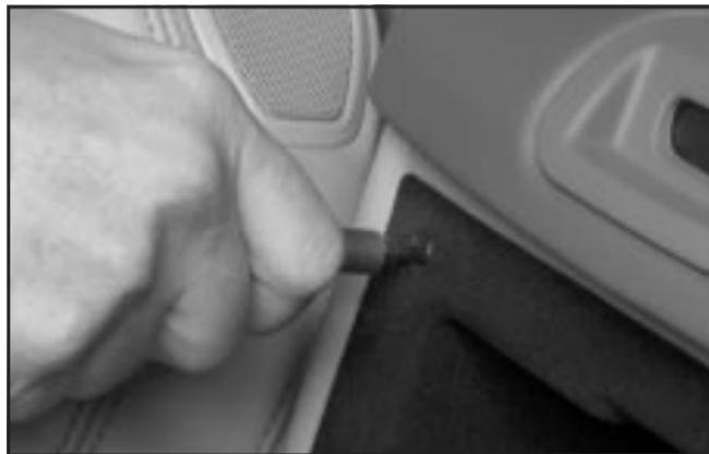
10. Remove the upright center storage compartment. Use the wrench to remove the four screws holding the storage area in place.
