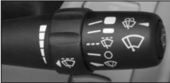
Use the lever located on the right side of the steering column to operate the windshield wipers.
