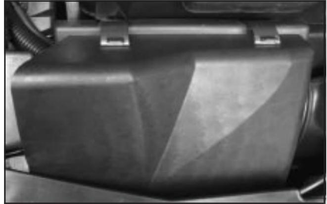
1. Flip the clasps on the top of the engine air cleaner/filter cover forward to unlatch the cover.
