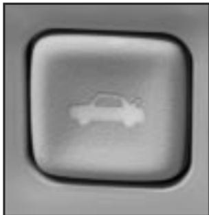
The trunk lock release button is located to the left of the steering wheel on the instrument panel.
