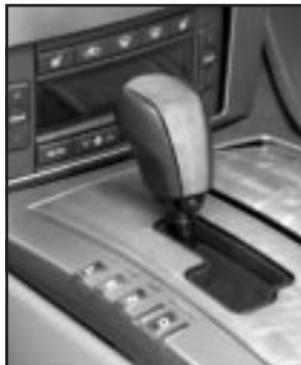
2. Move the shift lever into PARK (P) by pushing the lever all the way toward the front of the vehicle.
