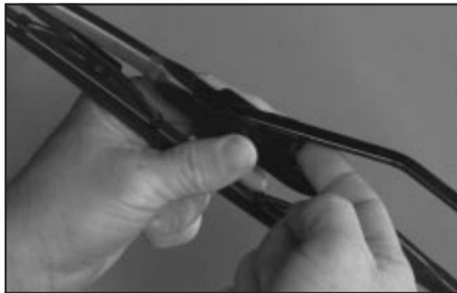
2. Tip the blade up and push down on the tab to release the wiper blade assembly.
