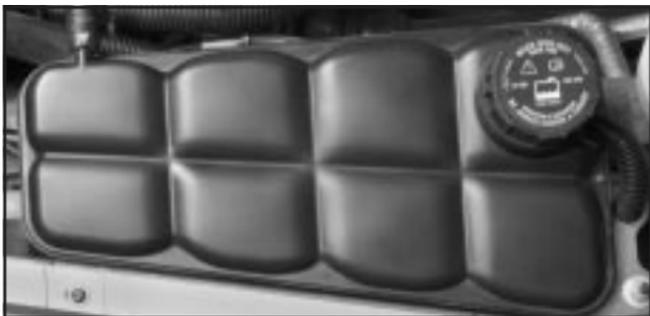
A low coolant level should be indicated by a LOW COOLANT message on the Driver Information Center. If it is, you may have a leak at the pressure cap or in the radiator hoses, heater hoses, radiator, water pump or somewhere else in the cooling system.
