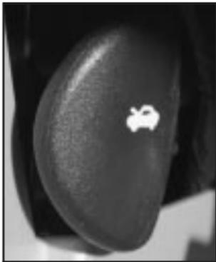
1. Pull the lever inside the vehicle to open the hood. It is located on the lower left side of the instrument panel.
