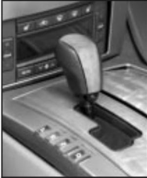
To use this feature, move the shift lever from the AUTOMATIC OVERDRIVE (D) position to the left and into the driver shift control gate.
