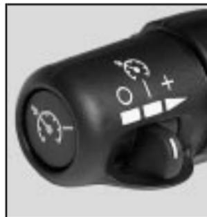
Some of the ACC controls are located on the end of the multifunction lever.
