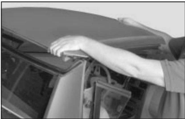
16. Hold the top in the front and the rear and lift the top until it is almost closed. Be careful not to pinch your fingers between the rear of the top and the rear window.
