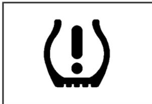
This light should come on briefly as you start the engine. It will then come on only when a low tire pressure condition exists.
