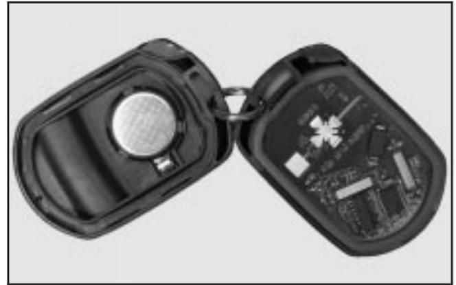
1. Insert a coin or similar object into the slot on the back of the transmitter and gently pry apart the front and back.
