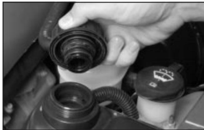
1. Park the vehicle on a level surface. You can remove the coolant surge tank pressure cap when the cooling system, including the coolant surge tank pressure cap and upper radiator hose, is no longer hot. Turn the pressure cap slowly counterclockwise (left).
