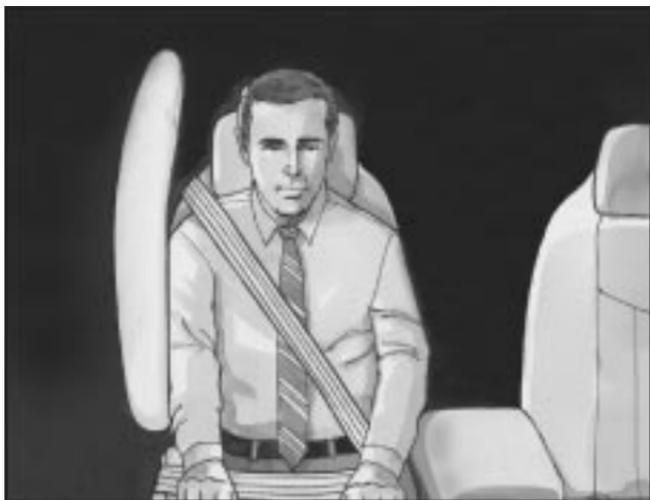
The passenger's side impact air bag is in the side of the passenger's seatback closest to the door.
