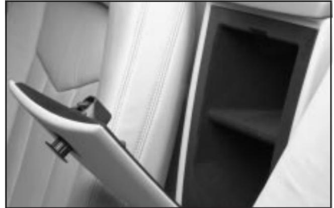
There is also an upright center console storage area between the seatbacks. To open the storage area, press and release the button near the top so it extends out. Then, turn the button in either direction to unlatch the lid and pull the console lid down. After you close the lid, press the release button back in.
