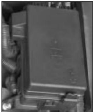
The underhood fuse block is located next to the engine on the passenger's side of the vehicle. For more information on location, see *Engine Compartment Overview* on page 5-12.
