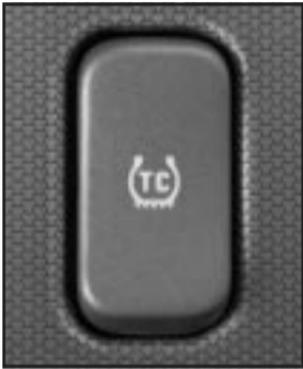
To turn the system off, press and hold the traction control button on the console for five seconds with the vehicle stopped. You can turn the system back on at any time by pressing the button.
