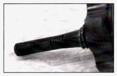
When the engine compartment is hot, the level should be at the HOT mark. If the fluid is at the ADD mark, you should add fluid.
