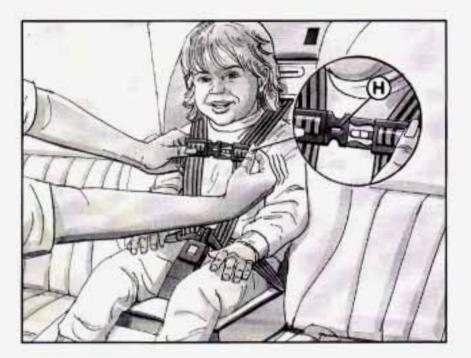
8. Now fasten the left and right halves of the shoulder harness clip together. The indicator window (H) on the clip will show green when the two halves are fastened together. The purpose of this clip is to help keep the harness positioned on the child's shoulders.
