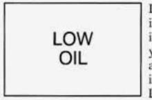
If the LOW OIL light on the instrument panel comes on, it means you need to check your engine oil level right away. For more information, see "Low Oil Level Light" in the Index.
