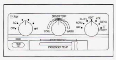
With this system, the driver and passenger can maintain separate temperatures. The system works best if you keep your windows closed while using it.
