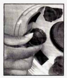
If your vehicle is equipped with wheel covers, be sure to use a wheel wrench to begin the process of loosening the plastic wheel nut caps. Removing the Flat Tire and Installing the Spare Tire
