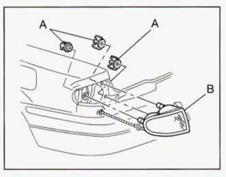
Pull the taillamp housing away from the body of the vehicle (B).
