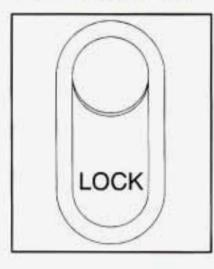
Press the power door lock switch to lock or unlock all doors.
