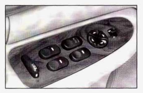
Switches on the driver's door armrest control each of the windows when the ignition is on. In addition, each passenger's door has a switch for its own window. The driver's window switch has an express-down feature. This switch is labeled AUTO. Tap the rear of the switch, and the driver's window will open a small amount. If the rear of the switch is pressed all the way down, the window will go all the way down.
