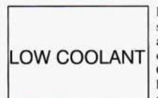
If this light comes on, your system is low on coolant and the engine may overheat. See "Engine Coolant" in the Index and have your vehicle serviced as soon as you can.
