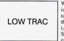
When your anti-lock system is adjusting brake pressure to help avoid a braking skid, this light will come on. (Also see "Anti-Lock Brake System Active Light" earlier in this section.)
