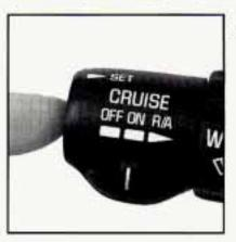
Push in the SET/COAST button at the end of the lever and release it. The CRUISE light on the instrument panel will come on.
