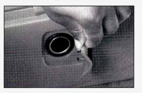
Your vehicle is equipped with a 12-volt outlet. It is located on the console's passenger's side, near the floor. Open the cover to use the outlet. This feature can be used to add aftermarket electrical equipment to your vehicle.
