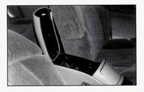
The console has cupholders, a cassette tape storage area and a coinholder. To open the console's storage area, press the latch located toward the front of the console lid on the driver's side of the vehicle and pull up.
