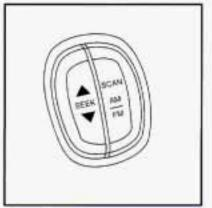
SEEK: Press the up or down arrow to tune to the next or previous radio station.
