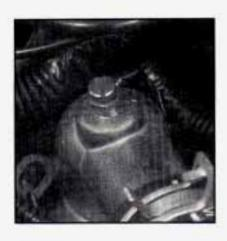
After the engine cools, open the coolant air bleed valve.
