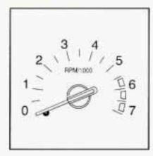
The tachometer displays the engine speed in thousands of revolutions per minute (rpm).
