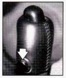
Press the driver selectable shift button to allow the transaxle to shift at higher engine speeds, increasing acceleration performance.
