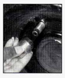
8. Replace the wheel nuts with the rounded end of the nuts toward the wheel. Tighten each nut by hand until the wheel is held against the hub.
