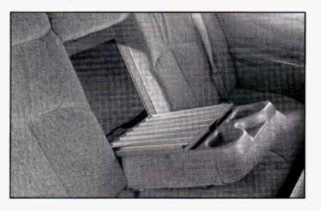
If your vehicle has this feature, you may access your trunk by pulling down the center back seat cushion — this gives you access to the pass-through door. The door can only be unlocked using your door key. Once this door is unlocked, you will then have access to the trunk area.
