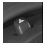
The hazard warning flasher button is located on the top of the steering column.
