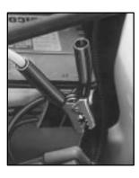
8. Now connect the negative (-) cable to the negative (-) terminal of the good battery. Use a remote negative (-) terminal if the vehicle has one.
