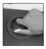
1. Turn the center nut on the compact spare tire cover counterclockwise to remove it. Then lift and remove the cover. (See "Compact Spare Tire" in the Index for more information about the compact spare tire.)
