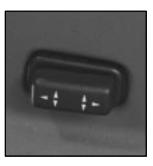
If your vehicle is equipped with this feature, the driver's and passenger's controls are located on the outboard sides of the seat cushions.
