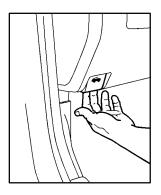
1. Pull the handle inside the vehicle, located just below the instrument panel and to the left of the steering column.
