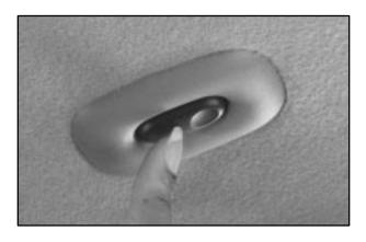
The switch works only when the ignition is on or when retained accessory power is active. See"Retained Accessory Power" in the Index.
