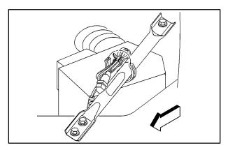
In very cold weather, 0°F (-18°C) or colder, the engine coolant heater can help. You'll get easier starting and better fuel economy during engine warm-up. Usually, the coolant heater should be plugged in a minimum of four hours prior to starting your vehicle. At temperatures above 32°F (0°C), use of the coolant heater is not required.
