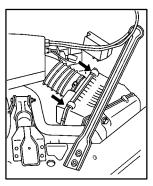
2. Lift up on the two clips located on the top of the filter assembly.
