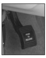
To set the parking brake, hold the regular brake pedal down with your right foot. Push down the parking brake pedal with your left foot.
