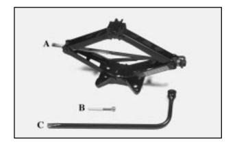
The tools you'll be using include the jack (A), extension and protection guide (B) and wheel wrench (C).
