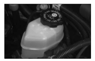
Your brake master cylinder reservoir is on the driver's side of the engine compartment. It is filled with DOT-3 brake fluid. See "Engine Compartment Overview" in the Index.
