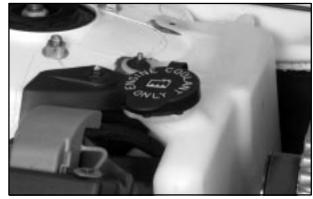
When the engine is cold, the coolant level should be at or above the COLD mark on the coolant recovery tank. If it isn't, you may have a leak at the pressure cap or in the radiator hoses, heater hoses, radiator, water pump or somewhere else in the cooling system.
