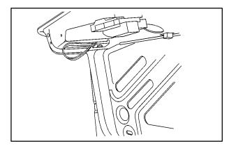
Your vehicle may have an assist handle located on the inside of the trunk lid toward the driver's side of the vehicle. Pull down on the handle to lower the trunk lid. Then close the trunk with your other hand. If the trunk is not properly closed, the DOOR/TRUNK light will appear in the message center of your instrument panel cluster. See "DOOR/TRUNK Light" in the Index for more information.
