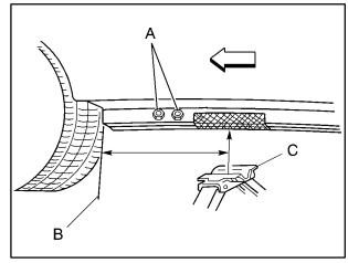
3. For jacking at the vehicle's front location, put the jack lift head (C) about 6 inches (15 cm) from the rear edge of the front wheel opening (B) or just behind the two bolts (A) as shown.
