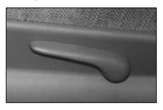
Lift the lever located on the outboard side of the seat to release the seatback, then move the seatback to where you want it. Release the lever to lock the seatback into place. Pull up on the lever without pushing on the seatback and the seatback will move forward.
