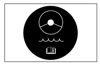
The power steering fluid reservoir is located on the passenger's side of the vehicle at the back of the engine compartment.
