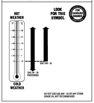
As in the chart shown previously, SAE 5W-30 is best for your vehicle. However, you can use SAE 10W-30 if it's going to be  $0^{\circ}F$  ( $-18^{\circ}C$ ) or above. These numbers on an oil container show its viscosity, or thickness. Do not use other viscosity oils, such as SAE 20W-50.
