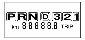
The graphic shown above is displayed on your instrument panel cluster in reference to your steering column shift lever.
