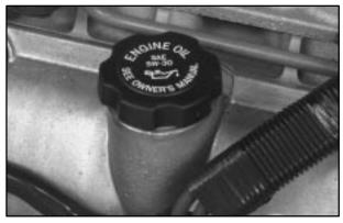
The engine oil fill cap is located toward the front of the engine near the engine oil dipstick handle. See "Engine Compartment Overview" in the Index for more information on location.
