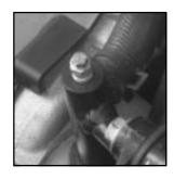
3. After the engine cools, open the coolant air bleed valves. There are two bleed valves. One is located on the thermostat housing. The other is located on the thermostat bypass tube.
