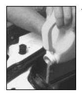
4. Fill the radiator with the proper DEX-COOL ® coolant mixture, up to the base of the filler neck. See "Engine Coolant" in the Index for more information about the proper coolant mixture.
