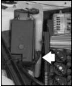
The vehicle must be on a level surface. When your engine is cold, the coolant level should be at the COLD mark or a little higher. When your engine is warm, the level should be up to the HOT mark or a little higher.
