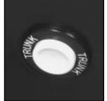
Press the button located inside of the glove box door to unlock the trunk from inside the vehicle. The shift lever must be in PARK (P) for the remote trunk release button to work.
