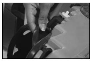
5. Remove the rubber access cover from behind the bulb you are replacing.
