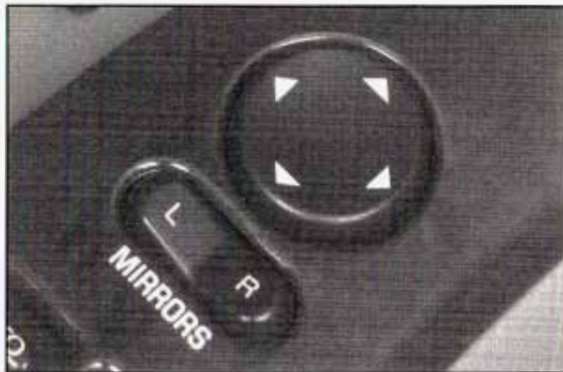
Your vehicle has power mirror controls located on the driver's door armrest.
