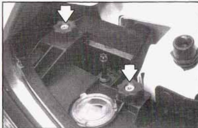
Each headlamp is attached by thumb screws.
