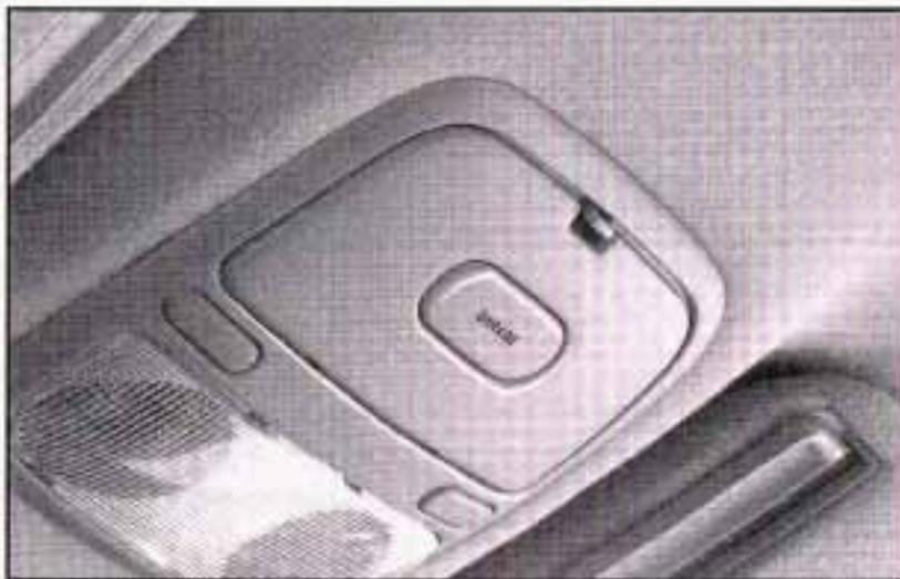
If your vehicle has this feature, the garage door opener storage area is located in the headliner near the front reading lamps.
