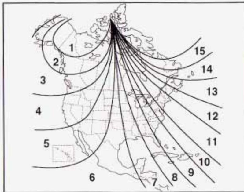
3. Once a zone number appears in the display, press the COMPASS button (or the on/off button for mirrors equipped with OnStar® controls) quickly until the correct zone number appears in the display. Stop pressing the button and the mirror will return to normal operation. If C appears in the compass window, the compass may need calibration. See "Compass Calibration" explained previously.
