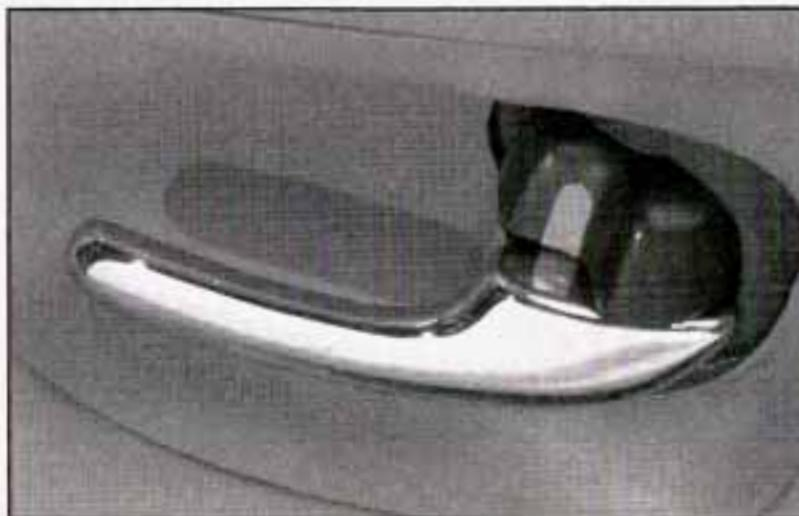
To lock or unlock the doors from the inside, move the manual lock on the door handle forward or rearward.
