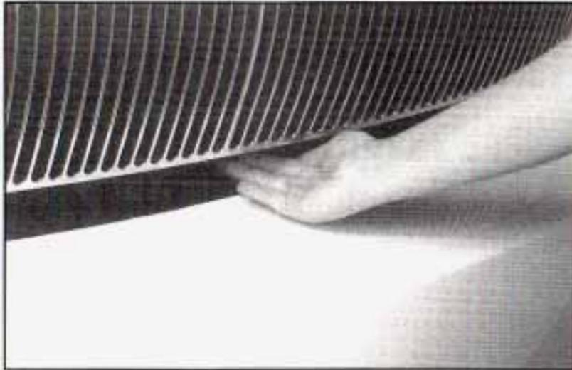
2. Then go to the front of the vehicle and locate the secondary hood release lever under the front edge of the grille.
