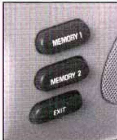
If your vehicle has this feature, the controls are located on the driver's door panel, and are used to program and recall memory settings for the driver's seating, outside mirror positions and climate controls. See *Climate Controls Personalization* on page 3-32 for more information.
