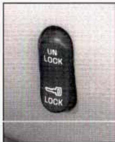
With power door locks, you can lock or unlock all doors on your vehicle using either the driver's or the front passenger's power door lock switch.
