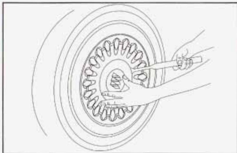
1. Insert the flat end of the wheel wrench in the notch.
