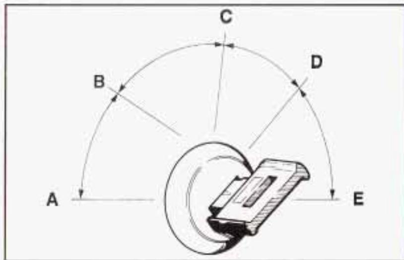
**A (ACCESSORY):** In this position you can operate your electrical accessories. Press in the ignition switch as you turn the top of it toward you.
