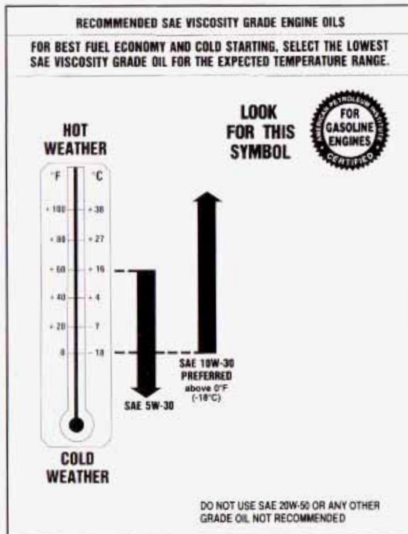
**Notice:** Use only engine oil with the American Petroleum Institute Certified For Gasoline Engines starburst symbol. Failure to use the recommended oil can result in engine damage not covered by your warranty.
