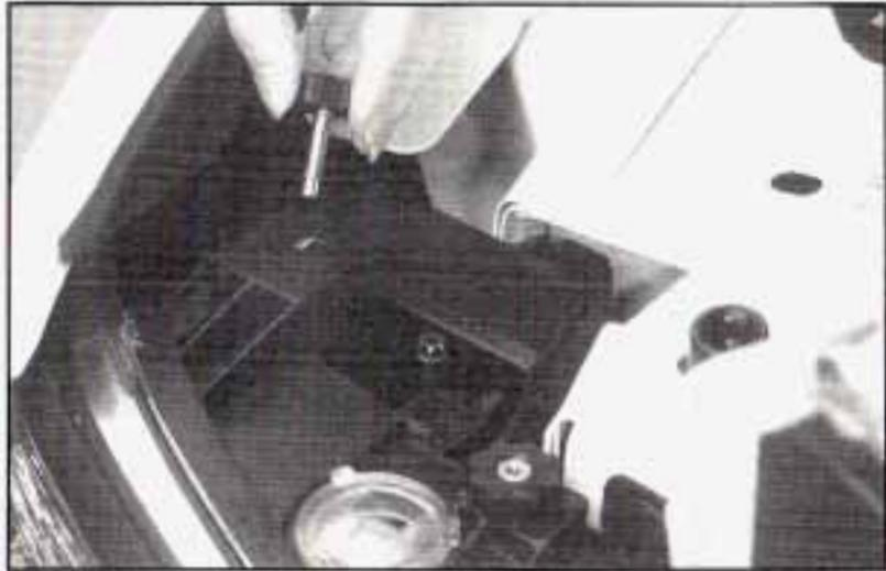
1. Remove the thumb screws by turning them counterclockwise.
