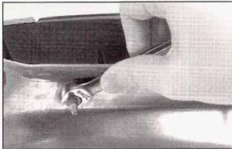
5. From inside the trunk compartment, remove the nuts from the studs.
