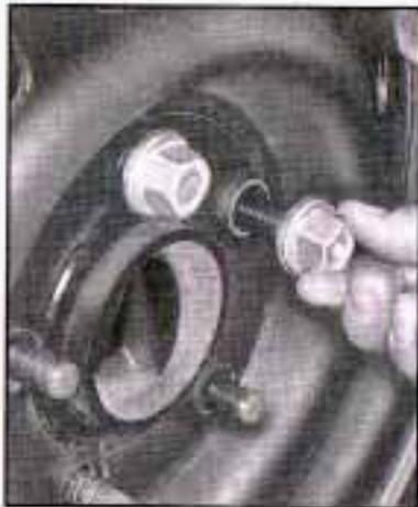
9. Then reinstall the wheel nuts with the rounded end of the nuts toward the wheel. Tighten each nut by hand until the wheel is held against the hub.
