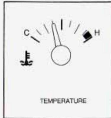
This gage measures the temperature of the vehicle's engine. If the pointer moves into the shaded area, the engine is too hot. A temperature indicator light will turn on and a chime will sound.
