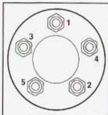
11. Using the wheel wrench, tighten the wheel nuts firmly in a crisscross sequence.
