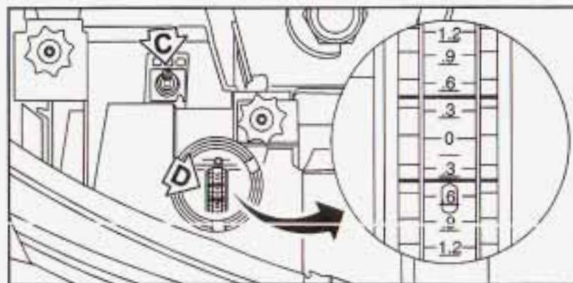
2. Turn the vertical aiming screw (C) until the level bubble (D) is lined up with zero.
