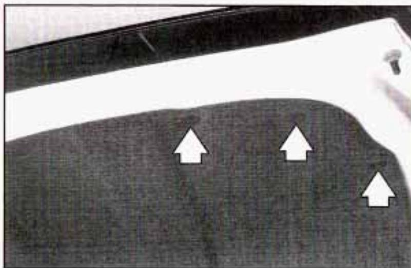
3. Remove the six fasteners along the top of the trunk lid (three on each side), holding the trunk trim in place.
