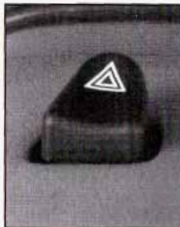
The hazard warning flasher button is located on top of the steering column.
