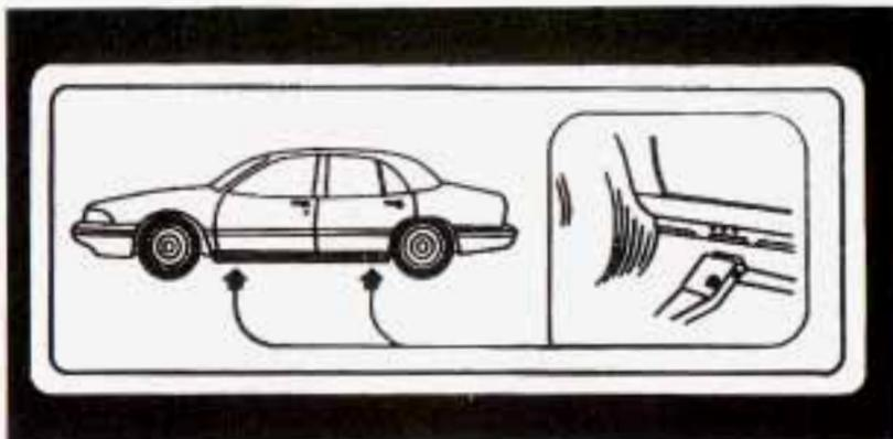
4. Near each wheel well is a notch in the plastic trim panel to position the jack head. You'll find the word JACK and an arrow stamped into the plastic near each notch. Position the jack under the vehicle and raise the jack head until it fits firmly against the sheet metal next to the word JACK. Do not raise the vehicle yet. Put the compact spare tire near you.
