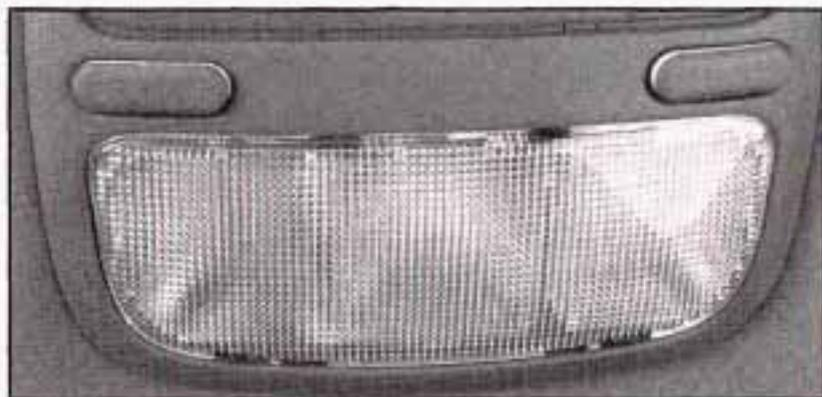
The front reading lamps, located on the headliner, and the interior courtesy lamps will come on when you open a door. They will turn off when you turn on the ignition.
