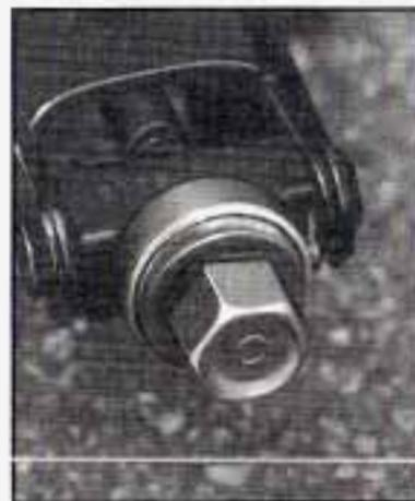
2. The jack has a bolt at the end. Attach the wheel wrench to the bolt to create a jack handle.
