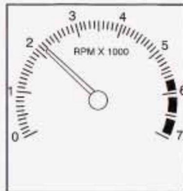
The tachometer tells you how fast the engine is running. It displays engine speed in thousands of revolutions per minute (rpm).
