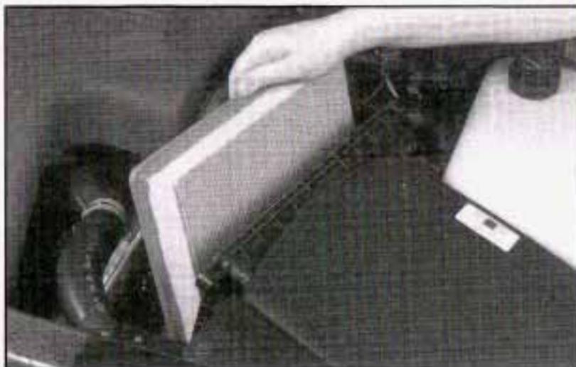
3. Check or replace the engine air cleaner/filter.
