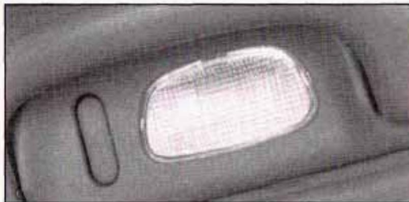
To turn on a rear reading lamp, press the button above that rear door. To turn off the reading lamp, press the button again.
