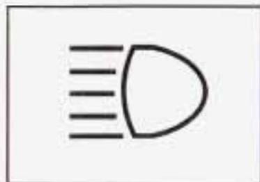
When the high beams are on, a light on the instrument panel cluster will also be on. If your vehicle is equipped with HUD, this light will also appear in the display area.
