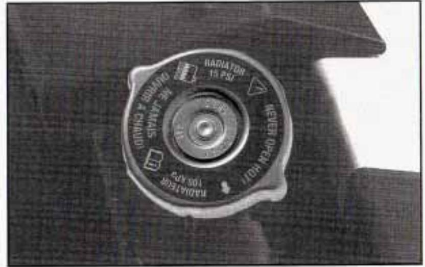
12. Then replace the pressure cap. At any time during this procedure if coolant begins to flow out of the filler neck, reinstall the pressure cap. Be sure the arrow on the pressure cap lines up like this.
