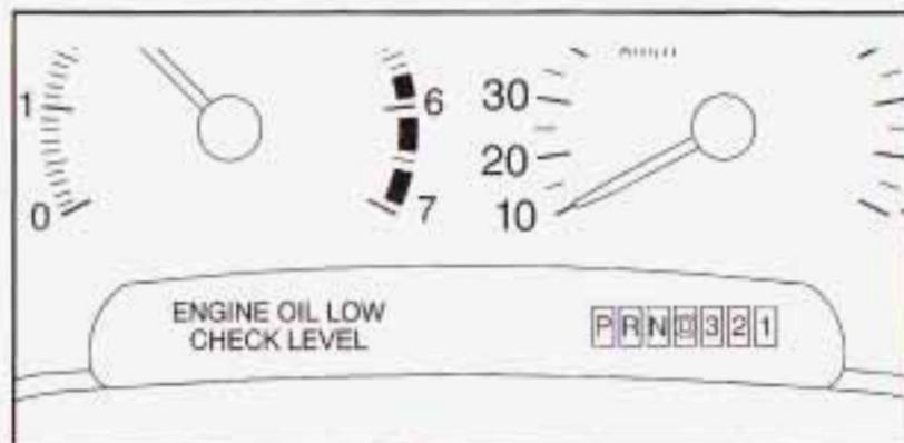
If the DIC message, ENGINE OIL LOW — CHECK LEVEL appears on the instrument cluster, it means you need to check your engine oil level right away. For more information, see *Driver Information Center (DIC)* on page 3-48.
