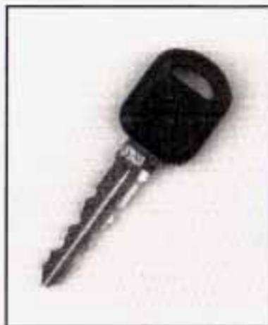
Your vehicle is equipped with the PASS-Key® III (Personalized Automotive Security System) theft-deterrent system. PASS-Key® III is a passive theft-deterrent system. This means you don't have to do anything different to arm or disarm the system. It works when you insert or remove the key from the ignition.
