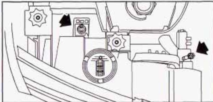
The headlamp aiming device is under the hood, directly behind the headlamps.
