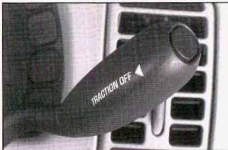
To turn the system off, press the button located at the end of the shift lever.
