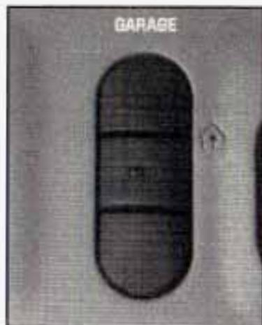
HomeLink<sup>®</sup>, a combined universal transmitter and receiver, provides a way to replace up to three hand-held transmitters used to activate devices such as gate operators, garage door openers, entry door locks, security systems and home lighting.
