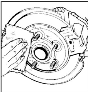
7. Remove any rust or dirt from the wheel bolts, mounting surfaces and spare wheel.
