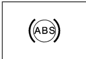
If there is a problem with the anti-lock brake system, this warning light will stay on. See *Anti-Lock Brake System Warning Light* on page 3-34.
