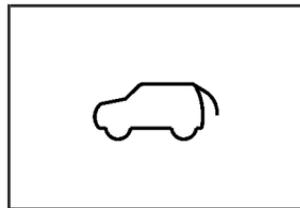
If this light comes on, your liftgate or liftglass is not completely shut.
