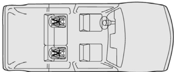
Your vehicle has the LATCH system. You'll find anchors (A) in the rear outside seat positions.
