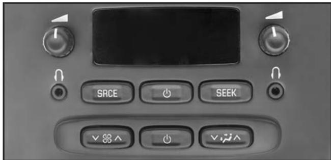
**⏻ (Power):** Press this button to turn the rear seat audio system on or off. The rear speakers will be muted when the power is turned on unless you have a Bose® equipped vehicle. You may operate the rear seat audio functions even when the primary radio power is off.
