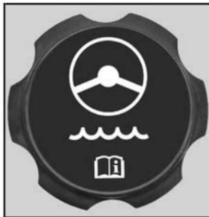
The power steering fluid reservoir is located in the engine compartment. It is on the passenger's side of vehicles with the L6 engine and is on the driver's side of vehicles with the V8 engine. See *Engine Compartment Overview on page 5-14* for reservoir location.
