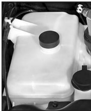
The engine coolant recovery tank is in the engine compartment on the passenger's side of the vehicle. See *Engine Compartment Overview* on page 5-14 for more information on location.
