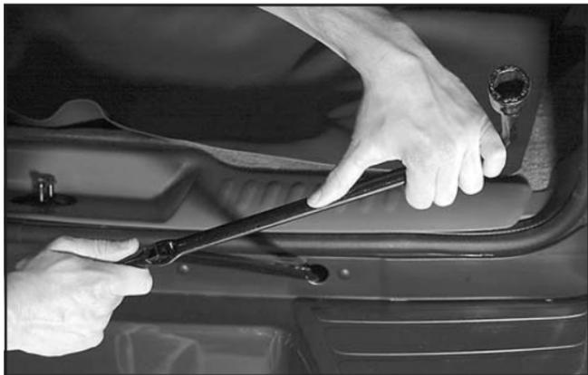
If the spare tire is hanging from the cable, insert the socket end of the extension connected to the wheel wrench into the hoist shaft hole in the bumper, on an angle, and turn the wheel wrench counterclockwise to lower the spare the rest of the way.
