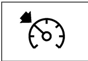
The cruise light on the instrument panel cluster will come on when the cruise control is engaged.
