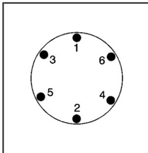
12. Use the wheel wrench to tighten the wheel nuts firmly in a crisscross sequence as shown.
