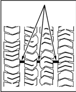
One way to tell when it's time for new tires is to check the treadwear indicators, which will appear when your tires have only 1/16 inch (1.6 mm) or less of tread remaining. Some commercial truck tires may not have treadwear indicators.
