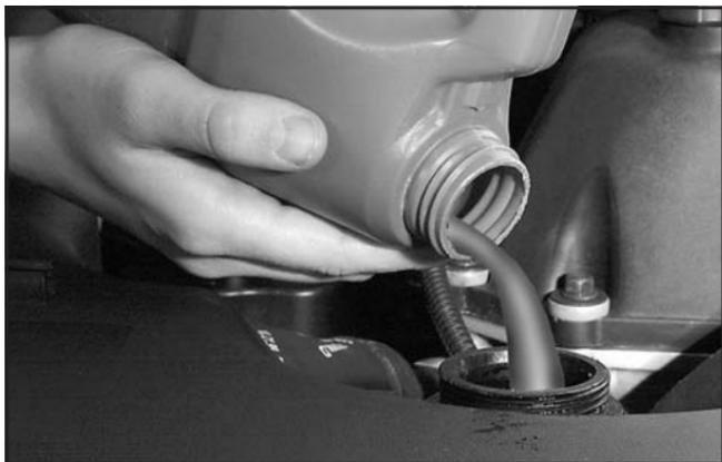
3. Fill the radiator with the proper DEX-COOL<sup>®</sup> coolant mixture, up to the base of the filler neck. See *Engine Coolant* on page 5-27 for more information about the proper coolant mixture.
