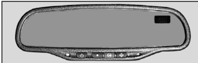
Your vehicle has an automatic-dimming rearview mirror with a compass and the OnStar<sup>®</sup> system.
