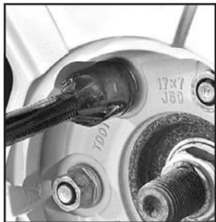
1. Using the wheel wrench, loosen all the wheel nuts. Don't remove them yet.
