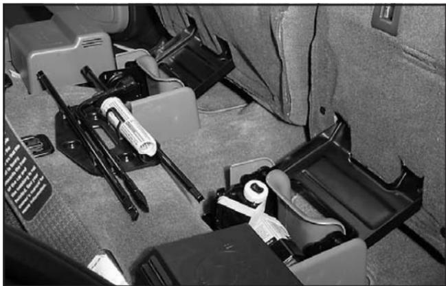
The jacking equipment you will need is stored under the rear seat on the passenger's side of the vehicle. See *Rear Seat Operation* on page 1-5. To release the jack from its holder, turn the knob on the jack counterclockwise to lower the jack head.
