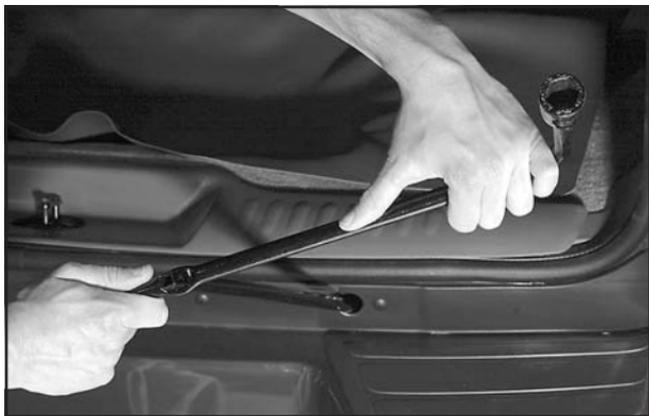
1. To remove the underbody-mounted spare, insert the socket end of the extension on a 45° angle downward into the hoist drive shaft hole. This will be exposed when the rear gate is open and is just above the rear bumper. Be sure the socket end of the extension connects to the hoist shaft.
