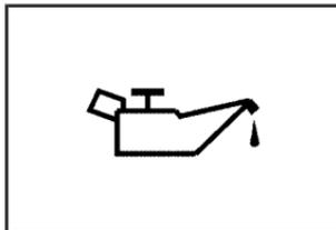
If the vehicle has an oil problem, this light may stay on after the engine is started, or come on while you are driving.
