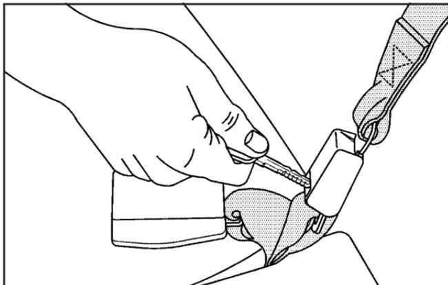
1. Disconnect the rear center lap-shoulder belt latch, if equipped, by using a pointed object to press the release button.
