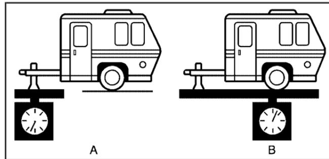
When using a weight-carrying hitch, the trailer tongue (A) should weigh 10 percent to 15 percent of the total loaded trailer weight (B).
