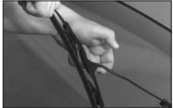
2. Push the release lever under the windshield wiper arm, and slide the wiper assembly off of the wiper arm.
