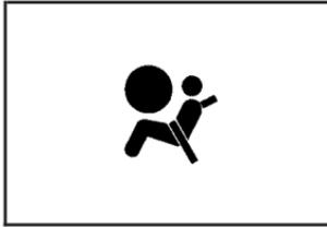
This light will come on when the vehicle is started, and it will flash for a few seconds. Then the light should go out. This means the system is functioning properly.
