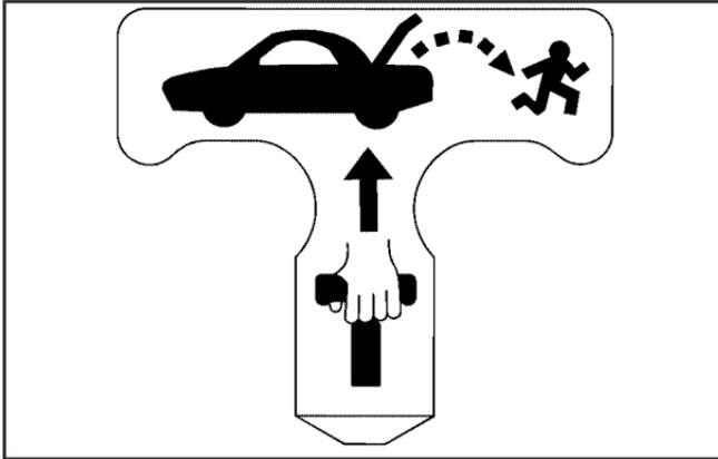
There is a glow-in-the-dark emergency trunk release handle located on the trunk latch of the trunk lid. This handle will glow following exposure to light. If ever needed, pull the emergency trunk release handle to open the trunk from the inside.
