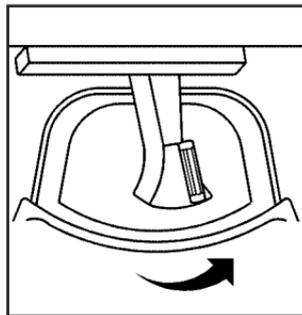
If your vehicle has the five-passenger console, there is a cupholder in front of the center console. The cupholder has an arm that adjusts to two positions to fit either a large cup or two smaller cups.
