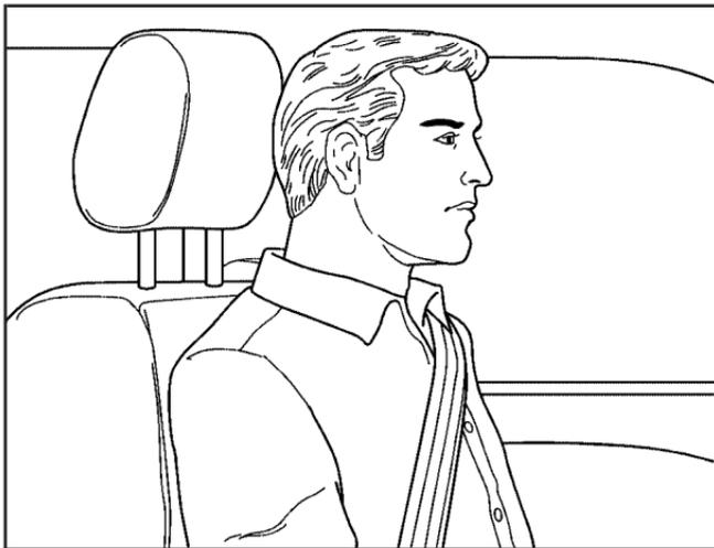
Adjust the head restraint so that the top of the restraint is closest to the top of the occupant's head in each front seat. This position reduces the chance of a neck injury in a crash. Push the release button, located under the head restraint, to lower the head restraint.
