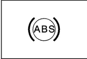
With the anti-lock brake system, the light will come on when your engine is started and may stay on for several seconds. That is normal.
