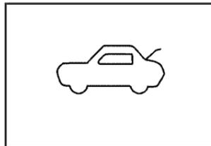
This light will come on and a chime will sound if the trunk is ajar and the vehicle is not in Park (P). Try closing the trunk again. Never drive with the trunk open.
