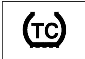
The traction control system active light will come on while the TCS is limiting wheel spin.
