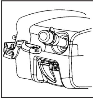
The lever on the steering wheel column that enables telescoping is located on the left side of the steering column and behind the tilt lever.
