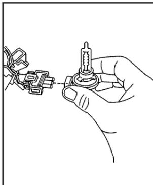
6. Disconnect the wire connector from the bulb by lifting the lock tab and pulling it away from the plastic base.
