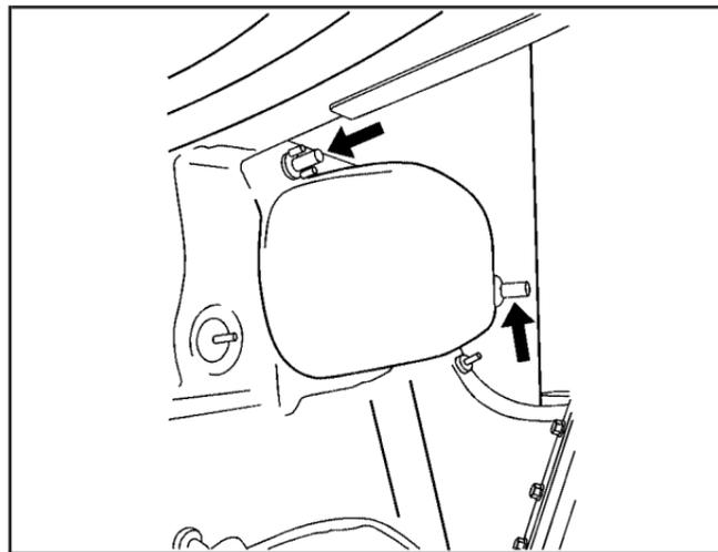
5. Remove the two wing nuts holding the taillamp assembly in place.
