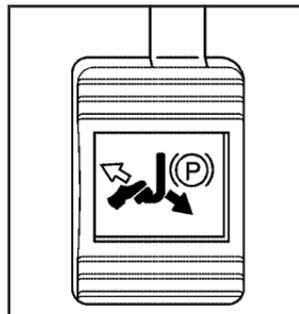
To set the parking brake, hold the regular brake pedal down with your right foot. Push down the parking brake pedal with your left foot.
