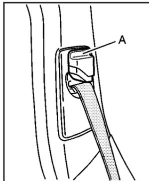
To move it down, push down on the release lever (A) move the height adjuster to the desired position. You can move the adjuster up just by pushing up on the shoulder belt guide.
