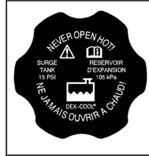
1. You can remove the radiator pressure cap when the cooling system, including the radiator pressure cap and upper radiator hose, is no longer hot. Turn the pressure cap slowly counterclockwise until it first stops.
