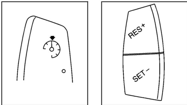
The buttons for the cruise control are located on the steering wheel.
