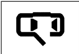
When the ignition is on, this light will stay on until all doors are closed and completely latched.
