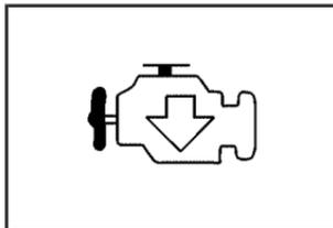
If the reduced engine power light is on, a chime will sound and a noticeable reduction in the vehicle's performance may occur.
