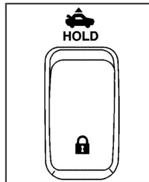
Press and hold the top of the driver's or front passenger's power door lock switch for one and one-half seconds to unlock the trunk.
