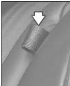
2. Pull forward on the seatback tab located on the outboard side of the rear seat cushion to fold the seatback down.
