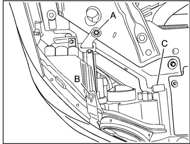
3. Pull up on the plastic retaining clip (C) while pushing rearward on the headlamp. Align the square cut-out on the retaining clip with the notch on the headlamp.
