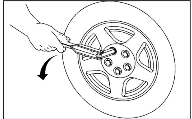
1. Place the wheel wrench securely over the wheel nut. Turn the wheel wrench counterclockwise to loosen all the wheel nuts, but do not remove them yet.
