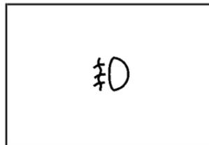
Press the fog lamps button, located in the center of the exterior lamps control on the left side of the steering column, to turn the fog lamps on or off.
