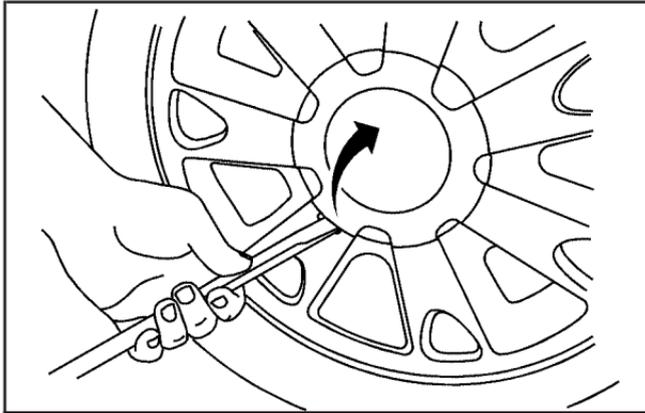
To remove a center cap, use the wrench to pry gently at the notch on the cap. Do not use a tool that is narrower than the wrench to pry at this notch. Then pry off the cap.
