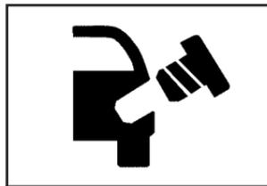
If equipped, this light will come on and a chime will sound if your gas cap is not securely fastened.
