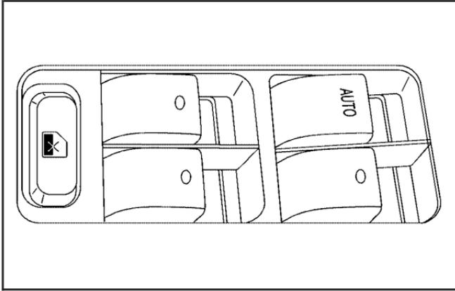
The switches on the driver's door armrest are used to control each of the windows. The power window switches work while the ignition is on, in ACCESSORY, or while Retained Accessory Power (RAP) is active. See *Retained Accessory Power (RAP)* on page 2-22. Each passenger door has its own window switch.
