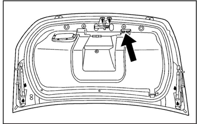
Your vehicle has a tie-down feature inside the trunk lid that can be used to secure the trunk lid when large items are stored in the trunk.
