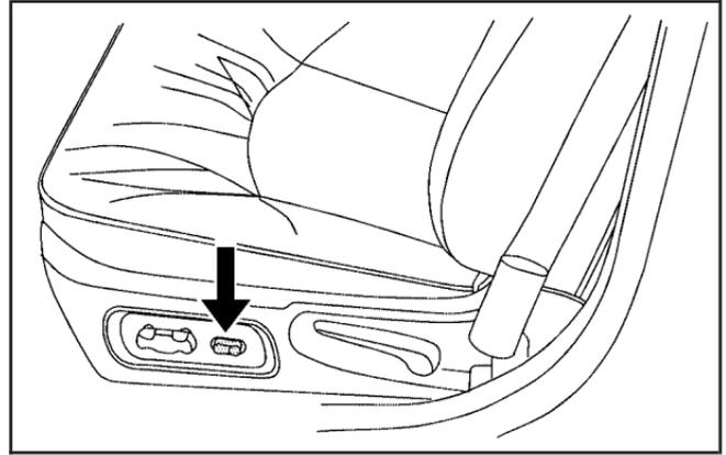
Your vehicle may have power lumbar. The control is located on the outboard side of the driver's seat cushion.
