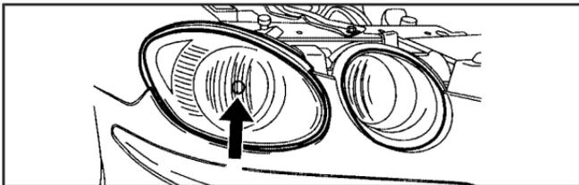
1. Find the aim dot on the lens of the low-beam lamp.
