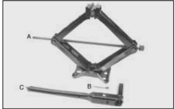
The tools needed to change a tire include the jack (A), extension and protection guide (B), and wheel wrench (C).
