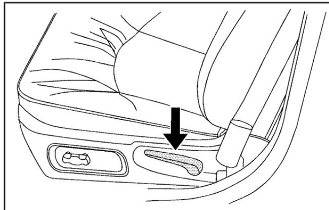
Lift the lever located on the outboard side of the seat to release the seatback, then move the seatback to the desired position. Release the lever to lock the seatback in place.
