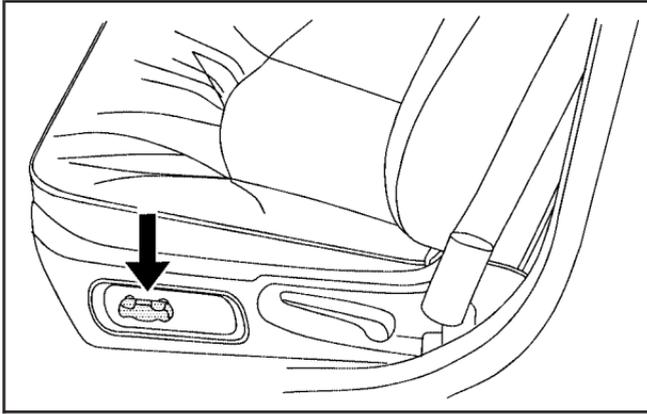
If your vehicle has power seats, the controls are located on the outboard sides of the seat cushions.
