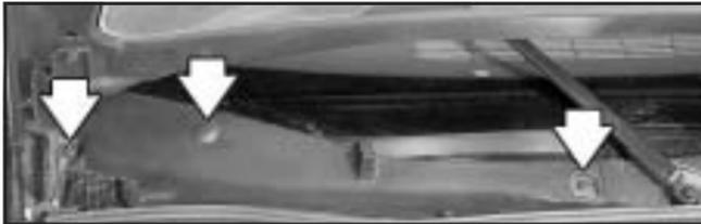
6. Remove the three air inlet grille retainers.
