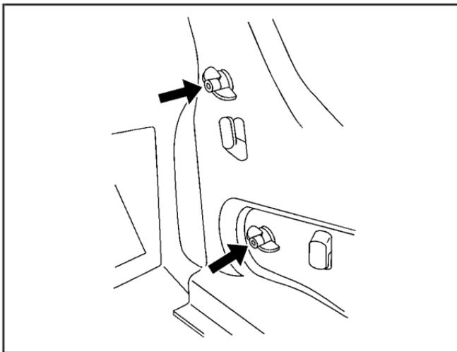
3. Remove the four plastic wing nuts retaining the trunk trim. There are two wing nuts located on the driver's side (shown) and two located on the passenger's side of the vehicle.
