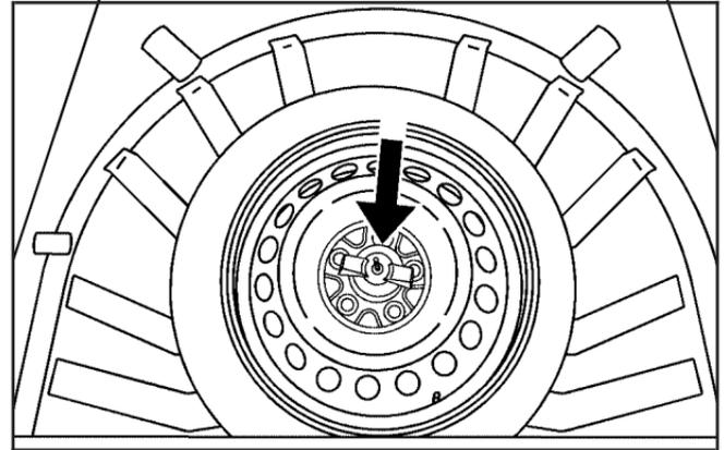
4. Turn the wing nut counterclockwise and remove it.
