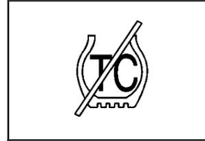
If the TC (traction control) warning light comes on and stays on, there may be a problem with the traction control system and, if equipped, the StabiliTrak<sup>®</sup> system.
