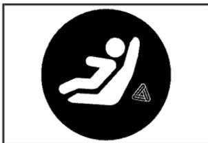
To assist you in locating the lower anchors for this child restraint system, each seating position with the LATCH system has a label on the seatback at each lower anchor position.
