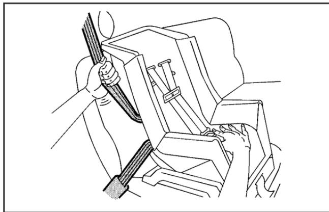
5. To tighten the belt, push down on the child restraint, pull the shoulder portion of the belt to tighten the lap portion of the belt and feed the shoulder belt back into the retractor. If you are using a forward-facing child restraint, you may find it helpful to use your knee to push down on the child restraint as you tighten the belt. You should not be able to pull more of the belt from the retractor once the lock has been set.
