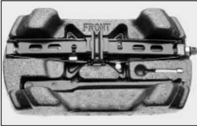
6. Turn the nut holding the jack counterclockwise and remove it. Then remove the jack and wrench.
