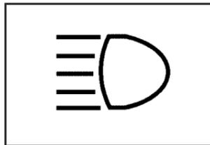
When the high beams are on, a light on the instrument panel cluster also will be on if the ignition is in ON.
