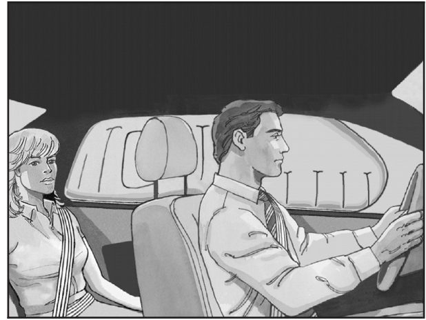
The roof-mounted side impact airbag for the driver and the person seated directly behind the driver is in the ceiling above the side windows.
