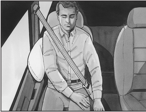
The seat-mounted side impact airbag for the right front passenger is in the side of the passenger's seatback closest to the door.
