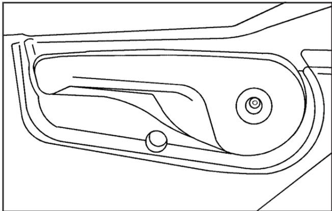
To adjust a seatback, pull up on the lever located on the outboard side of the driver's or front passenger's seats. Release the lever to lock the seatback where you want it. Push and pull on the seat to make sure it is locked into position.
