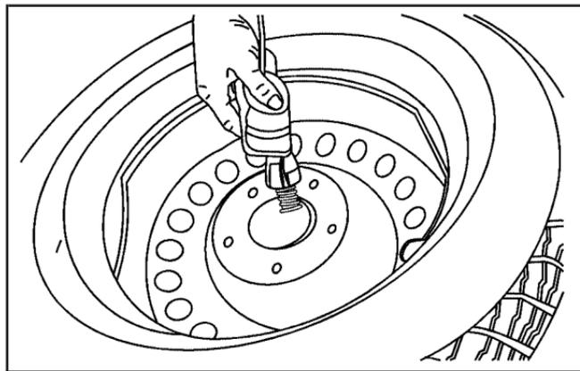
4. Tilt the retainer and slip it through the wheel opening to remove the spare tire from the cable.
