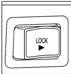
The power door lock switch is located on the driver's and front passenger's doors next to the door handle.
