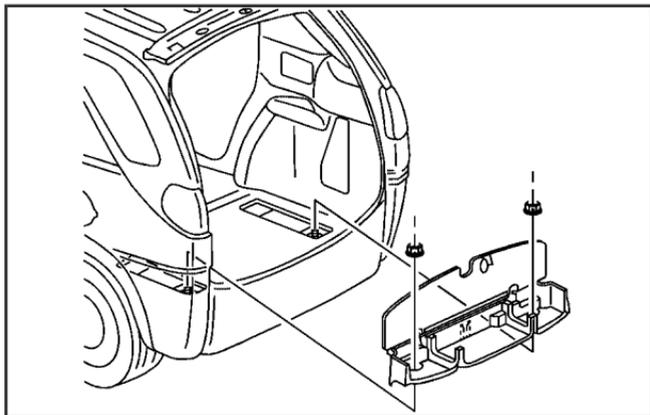
2. Lift the bin into the back of the vehicle. Align the bin over the rear mounting bolts.
