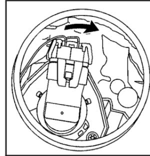
6. Turn the bulb socket one-quarter of a turn clockwise.
