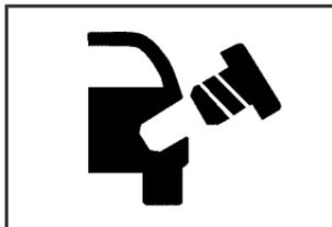
If your vehicle is equipped with this message, it will come on when the ignition is turned to ON or START and the gas cap is open.
