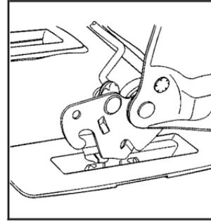
2. Make sure that the bench seat is angled so that the front hooks clear the floor pins. If the front legs are not attached correctly, the rear legs will not attach to the rear set of floor pins.
