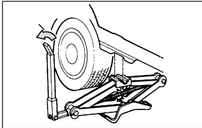
8. Lower the vehicle by attaching the folding wrench to the jack and turning the wrench counterclockwise. Lower the jack completely.
