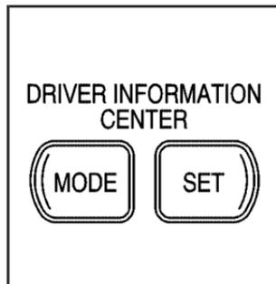
The DIC controls are located to the left of the steering column on the instrument panel.
