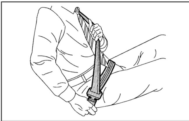
6. To make the lap part tight, pull down on the buckle end of the belt as you pull up on the shoulder belt.
