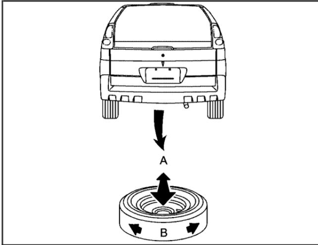
9. Make sure the tire is stored securely. Push, pull (A), and then try to turn (B) the tire. If the tire moves, use the folding wrench to tighten the cable.
