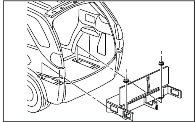
3. Lift the forward bin into the back of the vehicle. Place the mounting brackets onto the forward mounting bolts on the floor of the vehicle.
