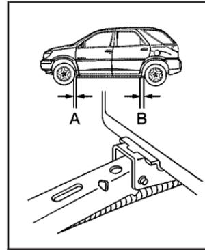
3. Locate the notch (A is 3.0 inches (7.5 cm) from the front tire or B is 5.5 inches (14.0 cm) from the rear tire). The notch is located near each wheel in the vehicle's body.
