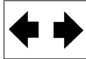
An arrow on the instrument panel cluster and the HUD display will flash in the direction of the turn or lane change.
