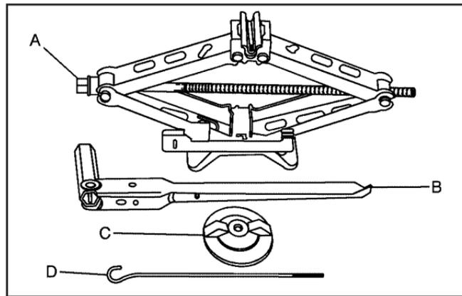
The tools you will be using include the jack (A), folding wrench (B), wing nut (C), and J-hook (D).
