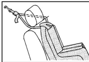
If the position you are using has an adjustable head restraint and you are using a dual tether, route the tether around the head restraint.
