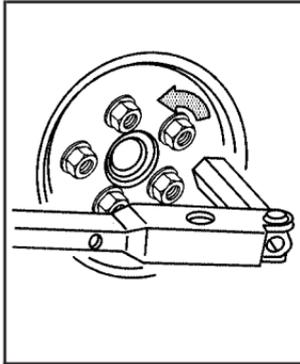
For wheels with a wheel lock key, use the wheel lock key between the lock nut and folding wrench. The key is supplied in the front passenger door pocket.
