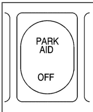
URPA can be turned off by pressing the rear park aid disable switch located in the instrument panel switchbank. When the system is disabled, an indicator light will glow on the switch. You will not see any lights on the rear display if the switch is in the off position.
