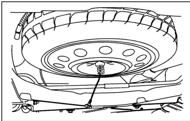
If the spare tire will not lower, the secondary latch may be engaged causing the tire not to lower.
