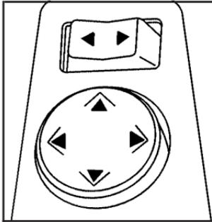
The power mirror controls are located on the driver's door armrest.
