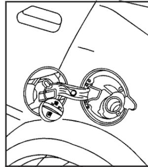
While refueling, hang the tethered fuel cap from the hook on the fuel door.
