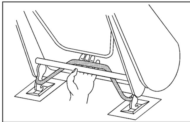
5. To release the front latches, squeeze the angled latch release bar toward the straight crossbar.
