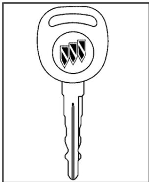
Your vehicle is equipped with the PASS-Key<sup>®</sup> III (Personalized Automotive Security System) theft-deterrent system. PASS-Key<sup>®</sup> III is a passive theft deterrent system. This means you do not have to do anything different to arm or disarm the system. It works when you insert or remove the key from the ignition.
