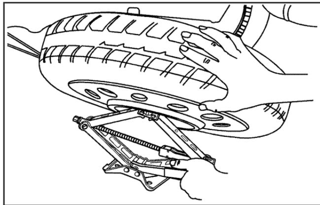
8. Disconnect the folding wrench from the jack and carefully remove the jack. Use one hand to push against the spare tire while firmly pulling the jack out from under the spare tire with the other hand.
