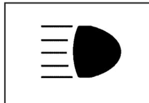
When the high beams are on, this light on the instrument panel cluster and the HUD display (if equipped), will also be on.
