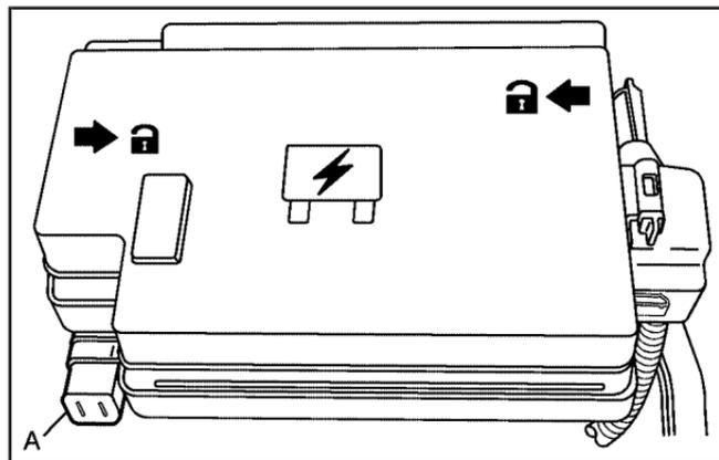
This fuse block is located in the engine compartment, on the passenger's side of the vehicle. See *Engine Compartment Overview* on page 5-10 for more information on location.
