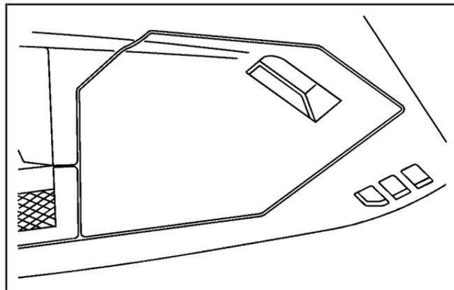
The floor console fuse block is located to the left of the glove box near the floor. Pull the door open to access the fuse block.
