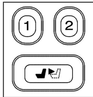
If your vehicle has this feature, the controls are located on the driver's door panel and are used to store and recall the driver's seat position and the outside rearview mirror position.
