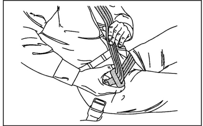
If the belt stops before it reaches the buckle, tilt the latch plate and keep pulling until you can buckle it. Pull up on the latch plate to make sure it is secure. If the belt is not long enough, see *Safety Belt Extender on page 1-45*.
