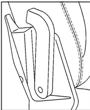
For up-level split bench seats, continue pushing forward on the recliner lever to release the rear latches from the floor pins and flip the seat forward.
