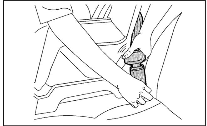
1. Make the belt as long as possible by tilting the latch plate and pulling it along the belt.
