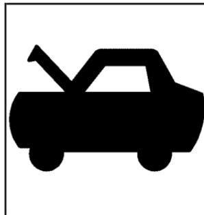
1. Pull the hood release handle with this symbol on it. It is located under the instrument panel on the driver's side of the vehicle.
