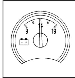
When your engine is not running, but the ignition is in RUN, this gage shows your battery's state of charge in DC volts.
