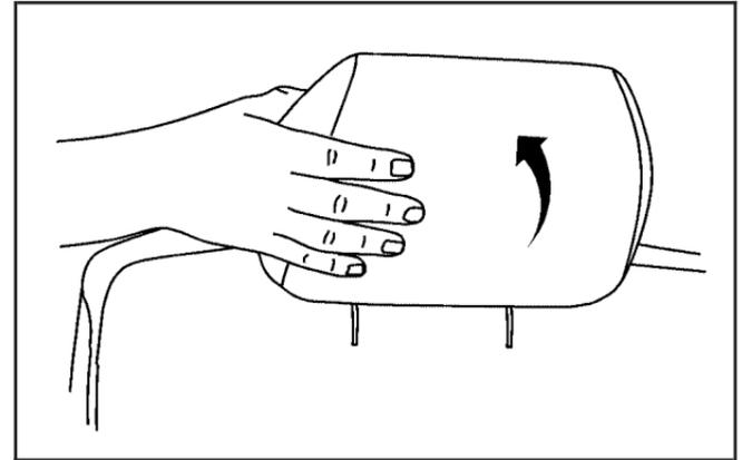
2. Return the head restraints to the upright position by reaching behind the seat and pulling it forward until it locks into place. Push and pull on the head restraint to make sure that it is locked.
