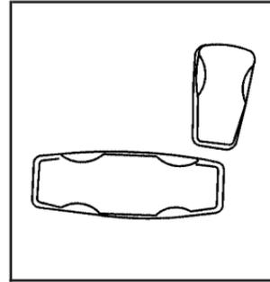
The front seats have power reclining seatbacks. Use the vertical power seat control located on the outboard side of the seat to operate them.
