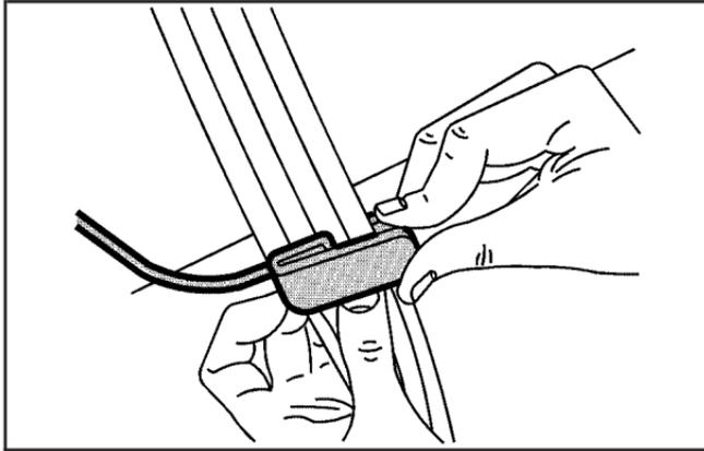
2. Slide the guide under and past the belt. The elastic cord must be under the belt. Then, place the guide over the belt and insert the two edges of the belt into the slots of the guide.
