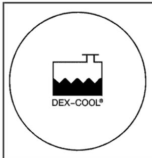
The engine coolant recovery tank is in the engine compartment on the passenger's side of the vehicle. The cap has this symbol on it. See *Engine Compartment Overview on page 366* for more information on location.
