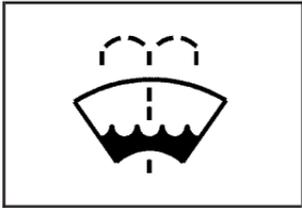
Open the cap with the washer symbol on it. Add washer fluid until the tank is full. See *Engine Compartment Overview on page 366* for reservoir location.
