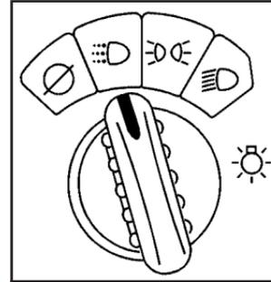
The exterior lamps knob is located on your instrument panel to the left of the steering wheel.
