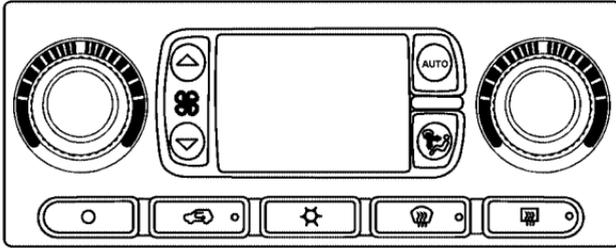
With this system you can control the heating, cooling and ventilation for your vehicle. When your vehicle is first started and the climate control system is on, or if the climate control system has been turned on, the display will show the driver's temperature setting for five seconds. Then it will show the outside temperature.
