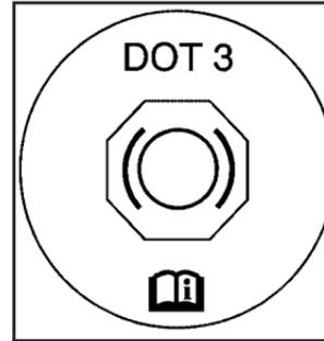
Your brake master cylinder reservoir is filled with DOT-3 brake fluid. See *Engine Compartment Overview on page 366* for the location of the reservoir.
