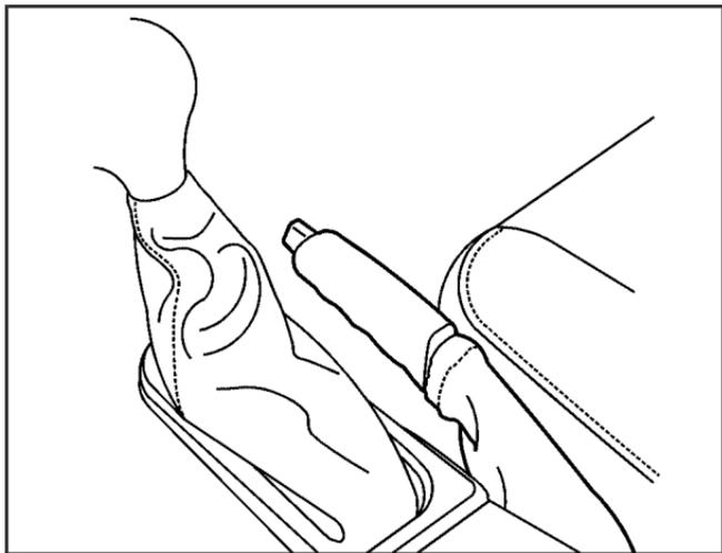
To release the parking brake, hold the regular brake pedal down. Pull the parking brake lever up until you can press in the button at the end of the lever. Hold the button in as you move the parking brake lever all the way down.
