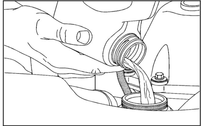
3. Fill the radiator with the proper DEX-COOL® coolant mixture, up to the base of the filler neck. See *Engine Coolant* on page 379 for more information about the proper coolant mixture.
