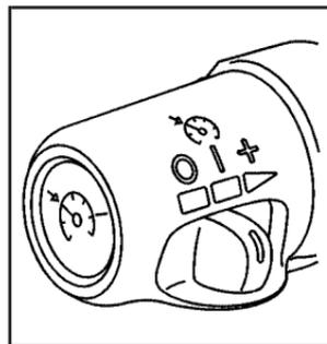
Your vehicle has cruise control. The controls are located on the end of the turn signal/multifunction lever.
