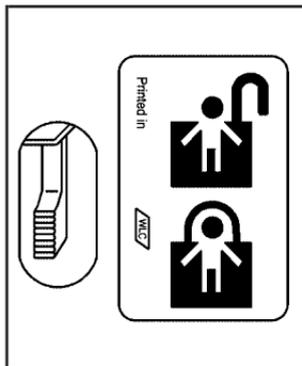
2. Move the lever down to engage the security lock. Move the lever up to disengage the security lock.
