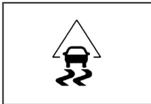
When the StabiliTrak<sup>®</sup> system is both on and actively controlling the stability of the vehicle, the StabiliTrak<sup>®</sup> light will blink for the duration of the event.
