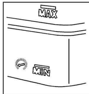
Look at the brake fluid reservoir. The fluid level should be above MIN. If it is not, have your brake system checked to see if there is a leak.
