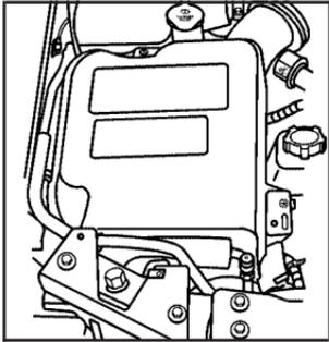
See *Engine Compartment Overview* on page 366 for the location of the engine air cleaner/filter.
