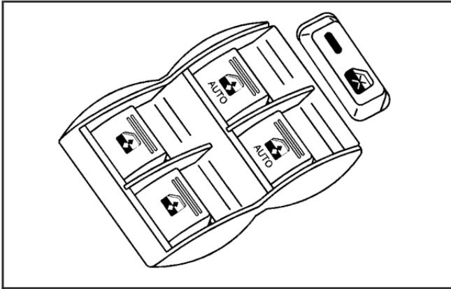
The controls for the power windows are located on the armrest on each of the side doors. With power windows, the switches operate the windows when the ignition is in RUN, ACCESSORY or when Retained Accessory Power (RAP) is active. See *Retained Accessory Power (RAP)* on page 110. The driver's door also has a switch for each of the passenger's windows.
