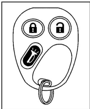
**U (Unlock):** When you press unlock, the driver's door will unlock automatically, the parking lamps may flash and the interior lights will go on.
