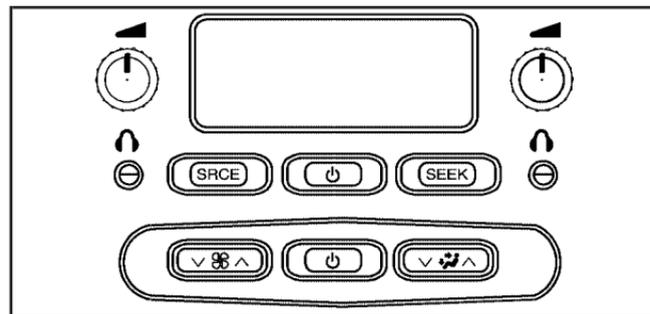
**⏻ (Power):** Press this button to turn the system on or off. The rear speakers will be muted when the power is turned on.
