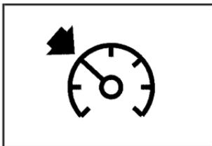
Some vehicles have a cruise light on the instrument panel cluster that will come on when the cruise control is engaged.
