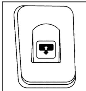
Press and release the back of the control in the overhead console to open the sunroof. Press the front of the control to close the sunroof.
