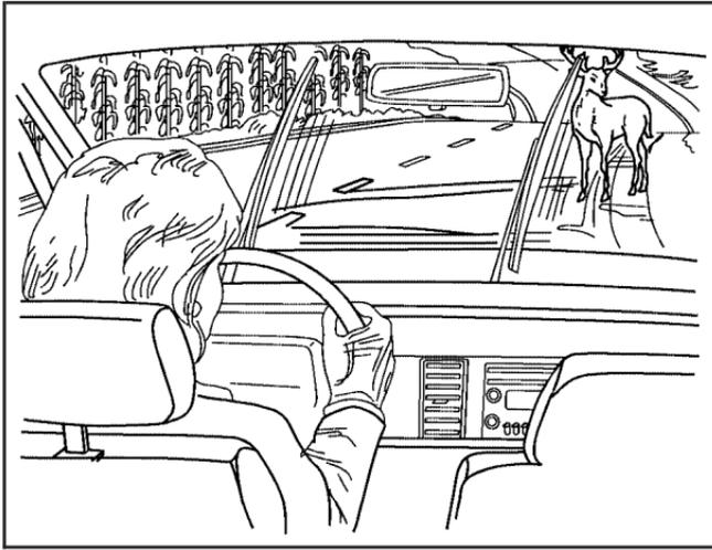
ABS can change the brake pressure faster than any driver could. The computer is programmed to make the most of available tire and road conditions. This can help you steer around the obstacle while braking hard.
