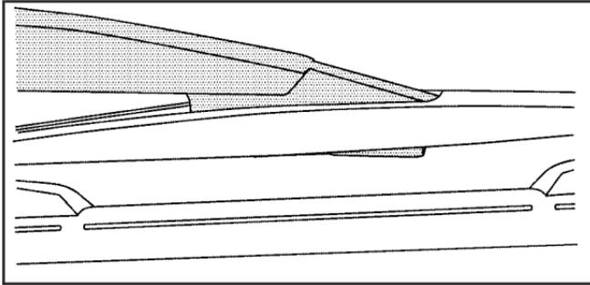
1. Lift the wiper blade assembly up and out of the park rest position.
