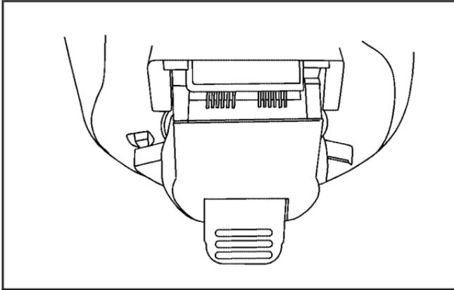
Your vehicle is equipped with a seven-wire trailer towing harness. This harness has a seven-pin universal heavy-duty trailer connector (if equipped with the trailering package) that is attached to a bracket on the hitch platform. If your vehicle is not equipped with the heavy-duty trailer connector, you may purchase one from your dealer.
