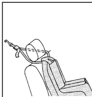
Fold down the head restraint and route the dual tether around the head restraint. See *Rear Seat Operation* on page 16.
