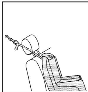
Fold down the head restraint and route the single tether under the head restraint and in between the head restraint posts. See *Rear Seat Operation* on page 16.
