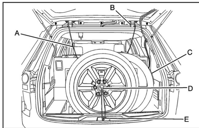
4. Pull the cable (A) through the door striker (E), the center of the wheel (D), and the plastic spare tire heat shield (C), as shown.
