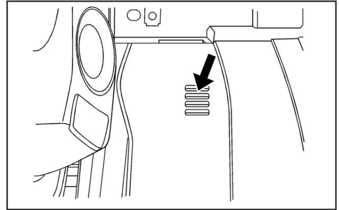
The interior temperature sensor located on the instrument panel to the right of the steering column, measures the temperature of the air inside the vehicle.
