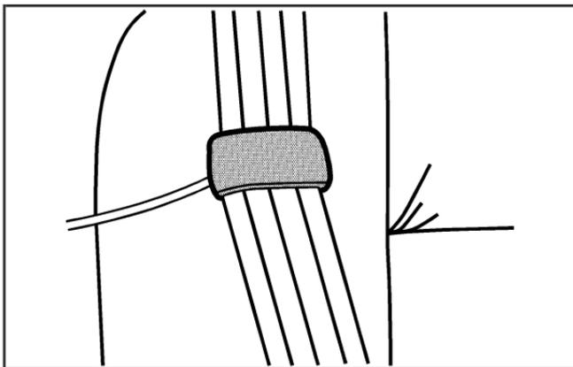
3. Be sure that the belt is not twisted and it lies flat. The elastic cord must be under the belt and the guide on top.
