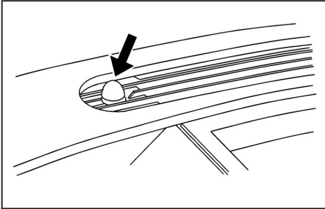
The solar sensor, located in the defrost grille in the middle of the instrument panel, monitors the solar radiation. Do not cover the solar sensor or the system will not work properly.
