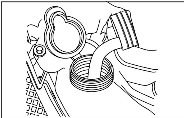
5. Fill the coolant recovery tank to the FULL COLD mark.
