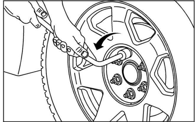
3. Loosen the wheel nuts — but do not remove them — using the lug wrench. For wheels with a wheel lock key, use the wheel lock key between the lock nut and lug wrench. The key is supplied in the front passenger door pocket.
