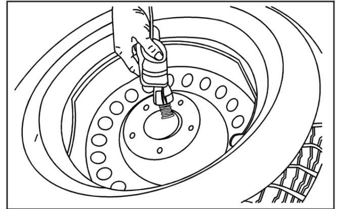
5. Tilt the retainer and slip it through the wheel opening to remove the spare tire from the cable.
