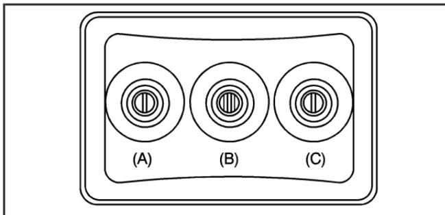
The A/V jacks, located on the rear of the floor console, allow audio or video signals to be connected from an auxiliary device such as a camcorder or a video game unit to the RSE system. Adapter connectors or cables might be required to connect the auxiliary device to the A/V jacks. Refer to the manufacturer's instructions for proper usage.
