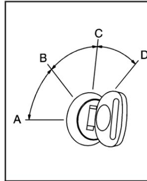
With the key in the ignition, you can turn it to four different positions.
