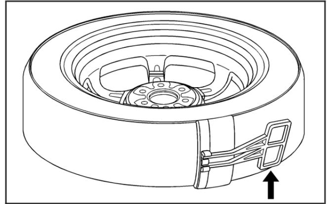
9. Remove the plastic spare tire heat shield by pulling the rubber latch. Store the plastic spare tire heat shield. See *Storing a Flat or Spare Tire and Tools* on page 5-85 for more information.
