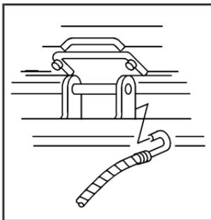
5. Hook the cable onto the outside portion of the liftgate hinges (B).
