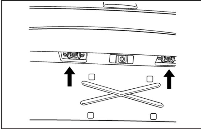
2. Turn and pull the license plate lamp forward through the lift gate trim opening.
