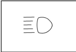
This light on the instrument panel cluster comes on if the high beam lamps are turned on while the ignition is on.
