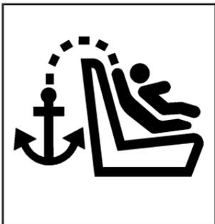
To assist you in locating the top tether anchors, the top tether anchor symbol is located on the cover or near the anchor.
