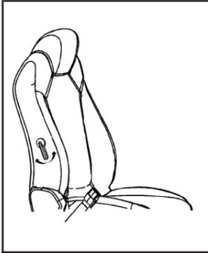
If your vehicle has this feature, the handle is located on the inboard side of the seatback.
