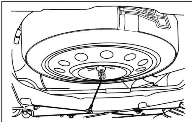
If the spare tire will not lower, the secondary latch could be engaged.
