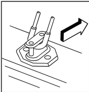
8. Make sure the metal tube is centered at the striker. Push the tube towards the front of the vehicle.
