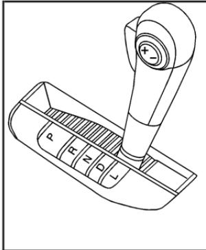
2. Press the plus/minus button located on the shift lever, to increase or decrease the gear range available based upon your current driving conditions and needs.
