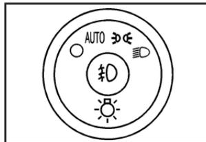
The exterior lamps control is located on the instrument panel to the left of the steering wheel.
