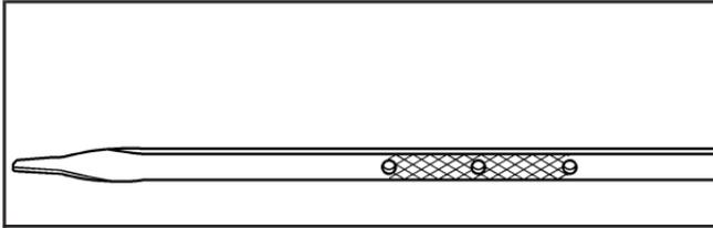
If the oil is below the cross-hatched area at the tip of the dipstick, you need to add at least one quart/liter of oil. But you must use the right kind. This section explains what kind of oil to use. For engine oil crankcase capacity, see *Capacities and Specifications on page 5-108*.
