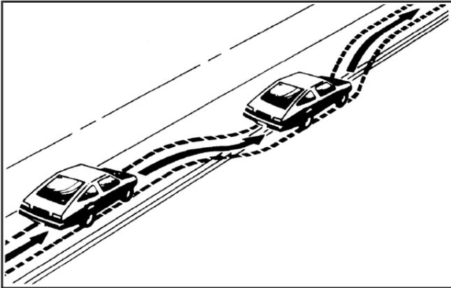
If the level of the shoulder is only slightly below the pavement, recovery should be fairly easy. Ease off the accelerator and then, if there is nothing in the way, steer so that your vehicle straddles the edge of the pavement. You can turn the steering wheel up to one-quarter turn until the right front tire contacts the pavement edge. Then turn the steering wheel to go straight down the roadway.
