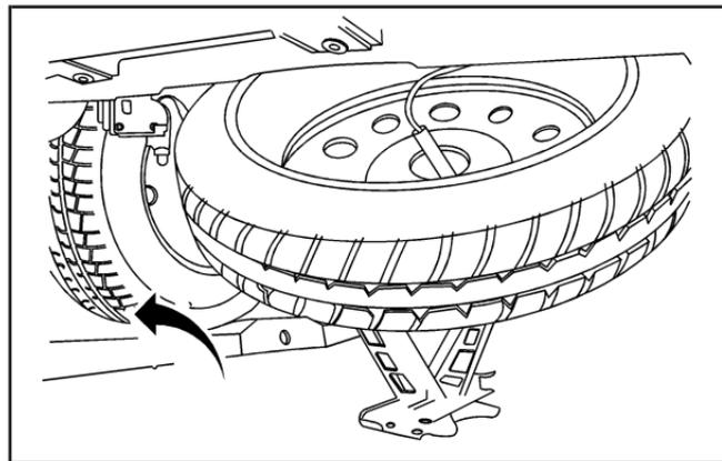
7. Lower the jack by turning the lug wrench counterclockwise. Keep lowering the jack until the spare tire slides off the jack.
