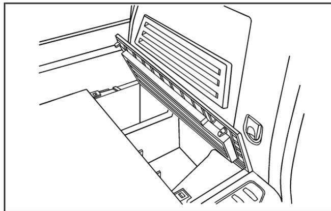
There is an additional storage compartment on each side of the system. To open, unlatch and lift the panel up.
