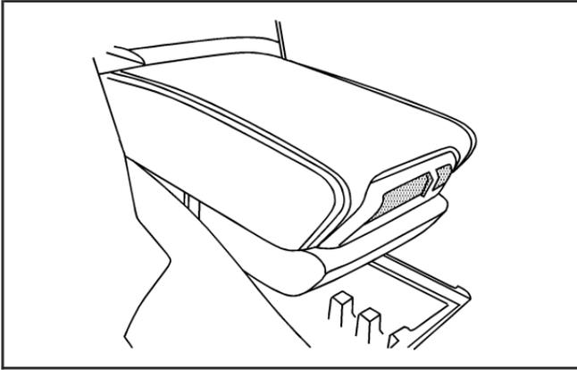
The center console armrest can slide forward and backward by pulling up the lever located on the front of it. To open the armrest storage area, press the button located on the front of the armrest. There is additional storage under the armrest. Move the armrest all the way to the rear position. Slide the cover back and remove the tray for additional storage.
