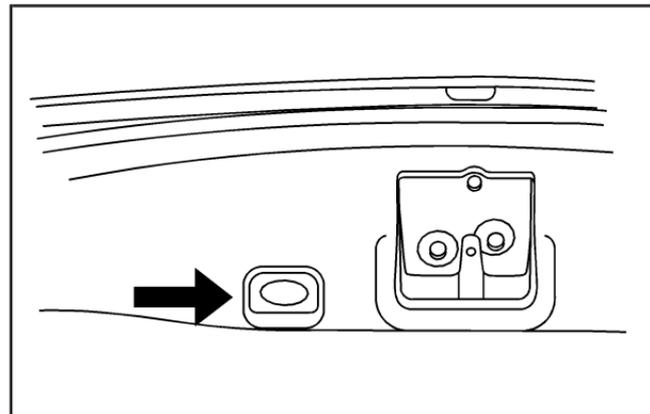
**Power Liftgate Button Near Liftgate Latch**
