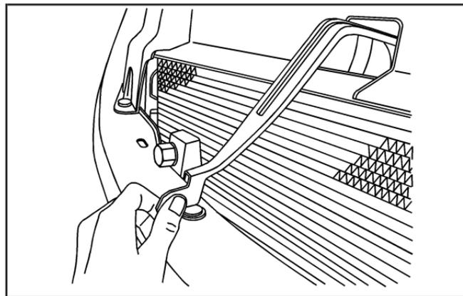
2. At the front of the vehicle, pull up on the bottom center of the grille, and push the secondary hood release to the left.
