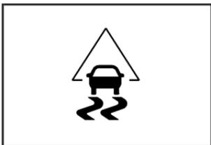
The StabiliTrak® light will flash on the instrument panel cluster when the system is both on and activated.
