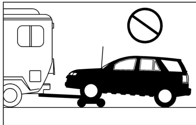
All-wheel-drive vehicles must not be towed with two wheels on the ground. To properly tow these vehicles, they should be placed on a platform trailer with all four wheels off of the ground or dinghy towed from the front.
