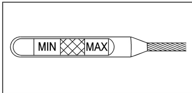
3. Check both sides of the dipstick, and read the lower level. The fluid level must be in the crosshatched area.
