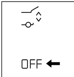
To change the liftgate to manual operation, press the switch on the center console to the OFF position.
