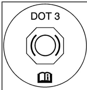
The brake master cylinder reservoir is filled with DOT-3 brake fluid. See *Engine Compartment Overview* on page 5-12 for the location of the reservoir.
