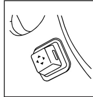
The power tilt and telescope wheel control is located on the outboard side of the steering column.
