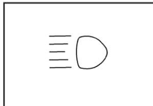
This light comes on when the high-beam headlamps are in use.
