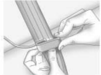
2. Place the guide over the belt and insert the two edges of the belt into the slots of the guide.
