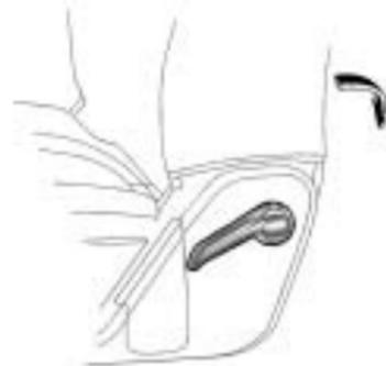
On vehicles with seats that have manual reclining seatbacks, the lever used to operate them is located on the outboard side of the seat.
