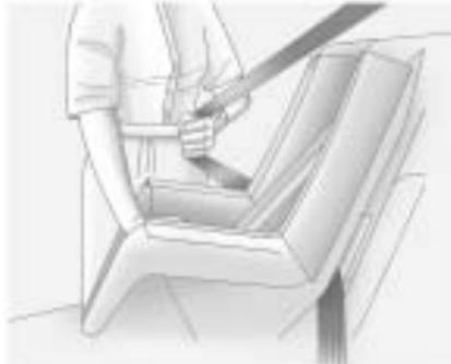
4. Pull the rest of the shoulder belt all the way out of the retractor to set the lock.
