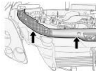
1. Detach fasteners and lift off the panel that covers the radiator cap.
