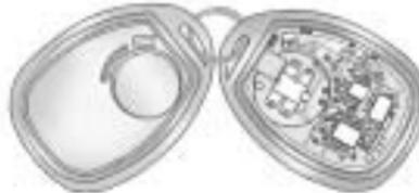
1. Separate the transmitter with a flat, thin object inserted into the notch on the side.
