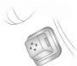
The power tilt and telescope wheel control is located on the outboard side of the steering column.
