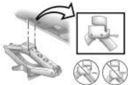
7. Place the jack under the vehicle as identified in Step 3. Raise the vehicle by turning the lug wrench clockwise in the jack. Raise the vehicle far enough off the ground so that there is enough room for the spare tire to fit under the wheel well.
