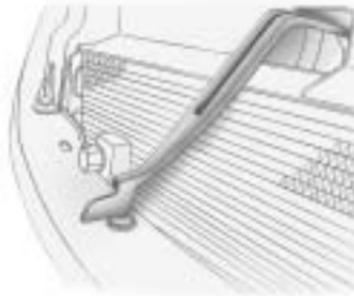
2. At the front of the vehicle, pull up on the bottom center of the grille, and push the secondary hood release to the left.
