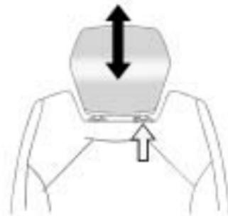
Pull the head restraint up to raise it. To lower the head restraint, press the release button, located on the head restraint post on the top of the seatback, while you push the head restraint down.
