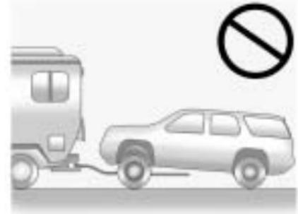
All-wheel-drive vehicles must not be towed with two wheels on the ground. To properly tow these vehicles, they should be placed on a platform trailer with all four wheels off of the ground or dinghy towed from the front.
