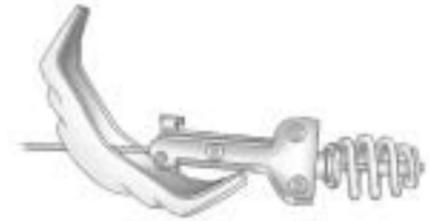
5. Tilt the retainer and slip it through the wheel opening to remove the spare tire from the cable.
