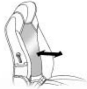
If the vehicle has this feature, the handle is located on the inboard side of the seatback.
