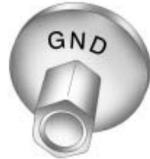
9. Connect the other end of the negative (-) cable at least 18 inches (45 cm) away from the dead battery, but not near engine parts that move.
