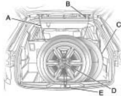
4. Pull the cable (A) through the door striker (E), the center of the wheel (D), and the plastic spare tire heat shield (C), as shown.
