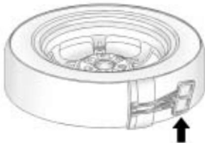
9. Remove the plastic spare tire heat shield by pulling the rubber latch. Store the plastic spare tire heat shield. See *Storing a Flat or Spare Tire and Tools* on page 5-76 for more information.
