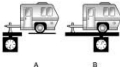
If a weight-carrying hitch or a weight-distributing hitch is being used, the trailer tongue (A) should weigh 10-15 percent of the total loaded trailer weight (B).
