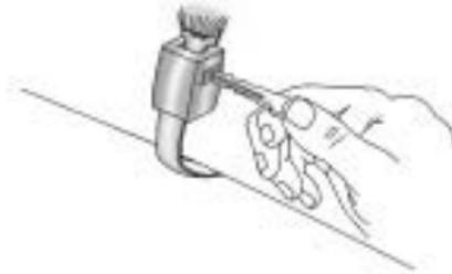
2. Disconnect the rear safety belt mini-latch, using a key in the slot on the mini-buckle, let the belt retract into the headliner. Stow the mini-latch in the holder located in the headliner.
