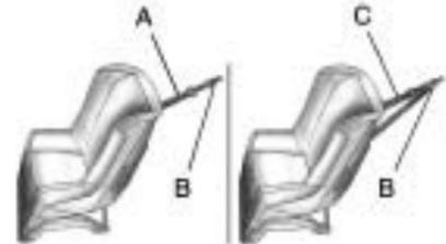
A top tether (A, C) anchors the top of the child restraint to the vehicle. A top tether anchor is built into the vehicle. The top tether attachment (B) on the child restraint connects to the top tether anchor in the vehicle in order to reduce the forward movement and rotation of the child restraint during driving or in a crash.
