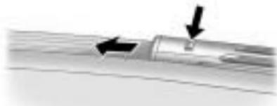
2. Press the button in the middle of the wiper arm connector and pull the wiper blade away from the arm connector.
