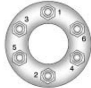
14. Tighten the wheel nuts firmly in a crisscross sequence, as shown.
