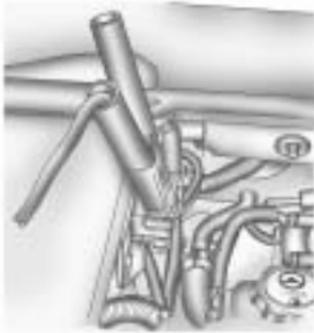
6. Connect the red positive (+) cable to the positive (+) terminal of the dead battery.
