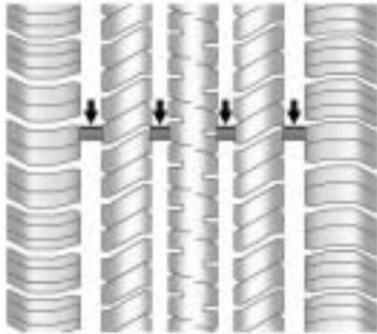
One way to tell when it is time for new tires is to check the treadwear indicators, which will appear when the tires have only 1/16 inch (1.6 mm) or less of tread remaining.
