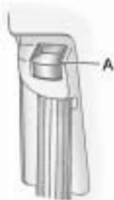
To move it down, push down on the button (A) and move the height adjuster to the desired position.
