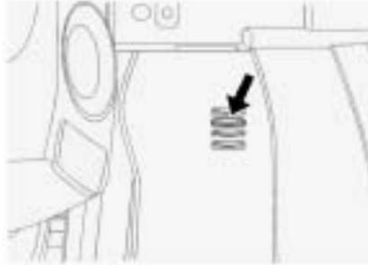
The interior temperature sensor located on the instrument panel to the right of the steering column, measures the temperature of the air inside the vehicle.
