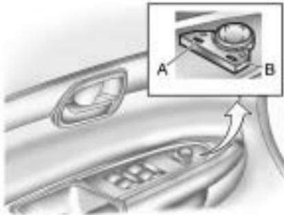
Controls for the outside power mirrors are located on the driver door armrest.
