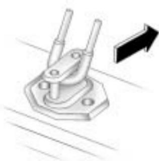
8. Make sure the metal tube is centered at the striker. Push the tube toward the front of the vehicle.
