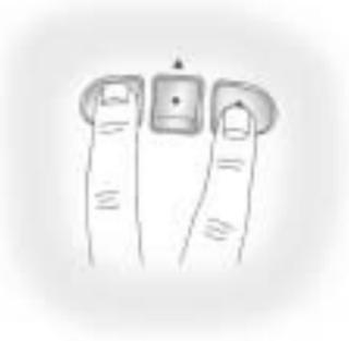
1. Press and hold down the two outside buttons until the indicator light begins to flash, after 20 seconds.
