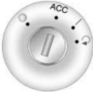
The ignition switch has four different positions.
