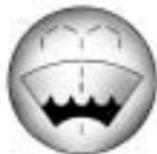
Open the cap with the washer symbol on it. Add washer fluid until the tank is full. See *Engine Compartment Overview on page 5-10* for reservoir location.
