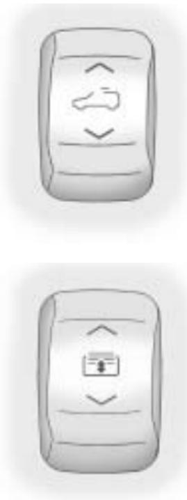
**Vent:** From the closed position, press and hold the front of the driver side switch to vent the sunroof.
