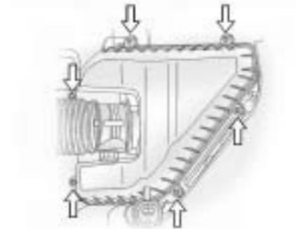
1. Loosen the screws that hold the cover on.
