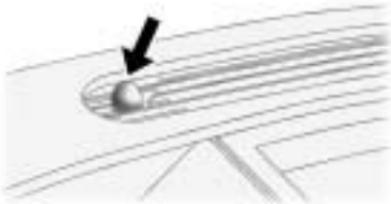
The solar sensor, located in the defrost grille in the middle of the instrument panel, monitors the solar heat. Do not cover the solar sensor or the system will not work properly.
