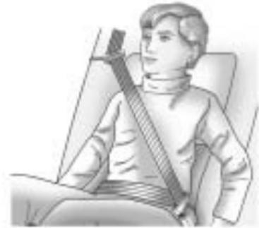
4. Buckle, position, and release the safety belt as described previously in this section. Make sure that the shoulder belt crosses the shoulder.
