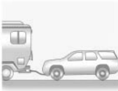
If the vehicle is front-wheel-drive, it can be dinghy towed from the front.
