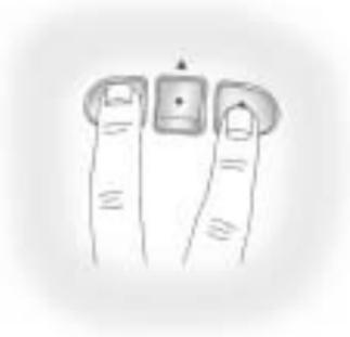
1. From inside the vehicle, press and hold down the two outside buttons at the same time, releasing only when the Universal Home Remote indicator light begins to flash, after 20 seconds. This step will erase the factory settings or all previously programmed buttons.
