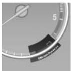
The energy of motion of the vehicle is converted to electrical energy while coasting. The vehicle battery is partially charged and fuel consumption can be lowered.
