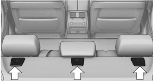
Depending on the vehicle equipment, there are two outer or three mounting points for child restraint fixing systems with a tether strap.
