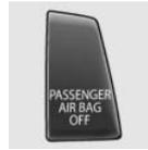
▷ The indicator lamp lights up when a child who is properly seated in a child restraint fixing system intended for that purpose is detected on the seat or the seat is empty. The airbags on the front passenger side are not activated.
