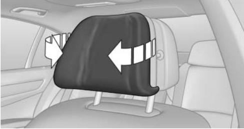
Fold forward for increased lateral support in the resting position.
