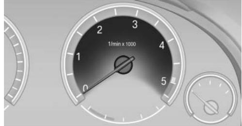
Always avoid engine speeds in the red warning field. In this range, the fuel supply is interrupted to protect the engine.
