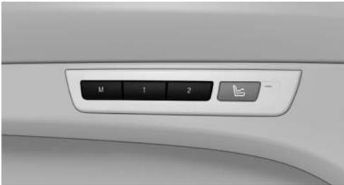
Two different driver's seat, exterior mirror, and steering wheel positions can be stored and retrieved for each remote control. The adjustment of the lumbar support is not stored.
