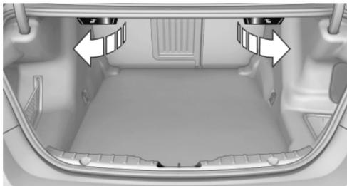
5. The unlocked rear seat backrest moves forward slightly. Fold the backrest forward by the head restraint.
