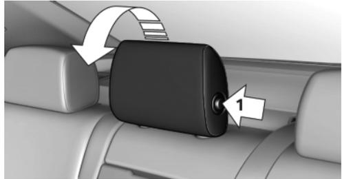
Press the button, arrow 1, and fold the head restraint forward.
