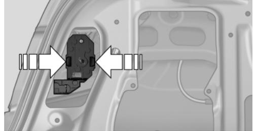
Squeeze the clips together and remove the bulb holder.
