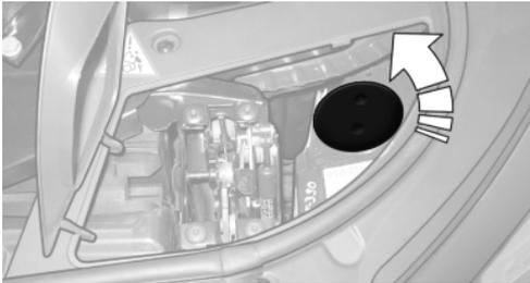
3. Unscrew the bulb holder counterclockwise.
