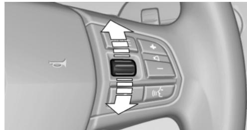
Press a button on the right side of the steering wheel or turn the thumbwheel to activate the required list.
