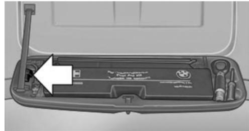
The lug bolt lock is in the tool kit or in a storage compartment close to the tool kit.
