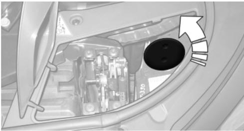
3. Unscrew the bulb holder counterclockwise.
