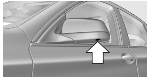
The objectives of the Top View cameras are located at the bottom of the exterior mirror housings. The image quality may be impaired by dirt. Clean the lens, refer to page 276.
