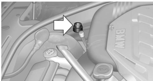
The so-called starting aid terminal in the engine compartment acts as the battery's positive terminal.
