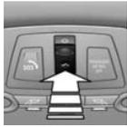
Press the switch up and hold it until the initialization is complete:
