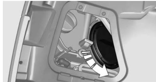
Unscrew the cap, remove it, and change the bulb.
