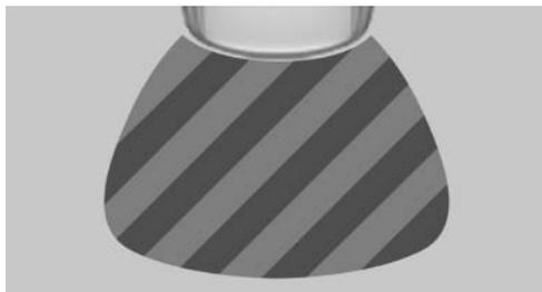
On the Control Display, the areas in front of and behind the vehicle are shaded. PDC has failed. Have the system checked.
