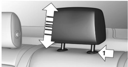
1. Pull the head restraint upward as far as possible.
