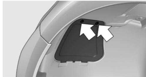
Remove the screws and fold down the cap.
