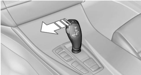
Push the selector lever to the left out of transmission position D.
