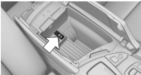
The USB audio interface is in the center armrest. Connect using a flexible adapter cable to protect the USB audio interface and the USB device against physical damage.
