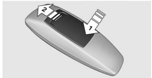
1. Remove the cover. Press on the cover, arrow 1, and push forward, arrow 2.
