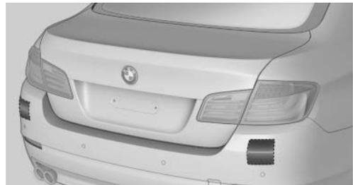
The radar sensors are located under the rear bumper.
