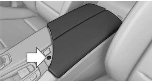
The storage compartment in the armrest can be locked with an integrated key to separately secure the trunk lid, refer to page 37, for example.
