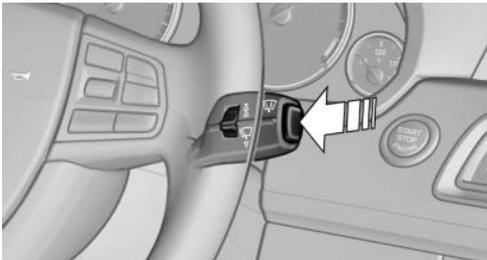
Press the button on the wiper lever.
