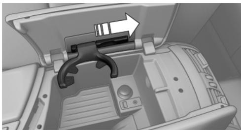
Before closing the center armrest, fold the cupholder back up. Push the lever in the direction of the arrow to do this.
