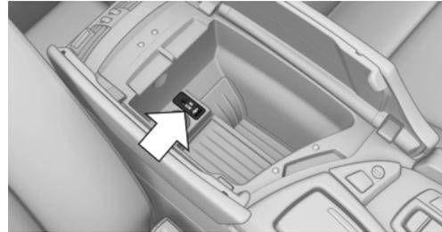
This can be used to connect an external audio device, such as a CD or MP3 player.
