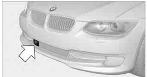
The sensor's ability to detect vehicles ahead may be restricted as a result of heavy rain, dirt,
