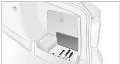
The onboard vehicle tool kit is stored in a compartment on the right-hand side of the cargo area. Remove the cover.
