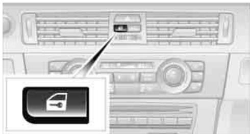
This button serves to unlock or lock doors and the trunk lid, but does not activate the anti-theft system. Depending on the equipment package, the fuel filler flap can be unlocked as needed.
