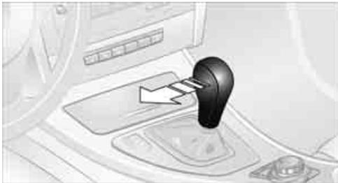
Move selector lever from position D toward the left into the M/S shifting slot; the Sport program is activated. This position is recommended for a performance-oriented driving style.
