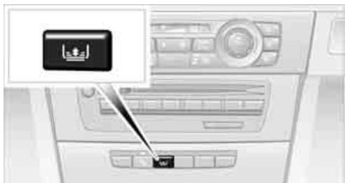
Briefly press the button in the center console to raise or lower the roller sunblind.
