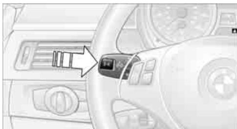
Press the button on the turn signal/high beam lever.
