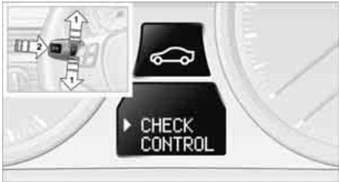
1. Push button **1** in the turn signal/high beam lever up or down repeatedly until the appropriate symbol appears in the display, accompanied by the words "CHECK CONTROL".
