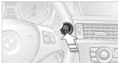
Pressing the Start/Stop button switches radio readiness or the ignition on or off.
