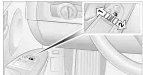
2. Shift into reverse or engage the selector lever- or transmission position R. The glass of the mirror on the passenger side tilts slightly down. This allows the driver to see the area immediately adjacent to the vehicle, e.g. a curb, when backing into a parking space.
