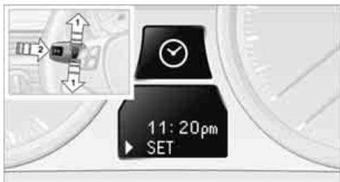
1. Push button **1** in the turn signal/high beam lever up or down repeatedly until the appropriate symbol appears in the display, accompanied by the time and the word "SET".
