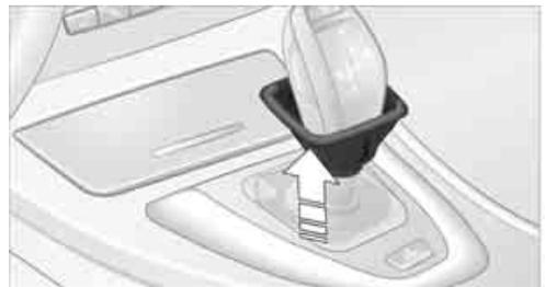
3. Using the allen wrench from the tool kit, refer to page 270, rotate the cover until it reaches the stop, arrow 1, and remove, arrow 2.
