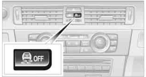
Press the button; the indicator lamp for DSC OFF lights up and TRACTION is displayed in the instrument cluster.
