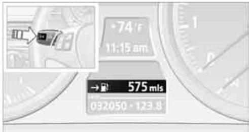
Press the button in the turn signal/high beam lever.
