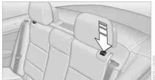
You can fold down the rear seat backrest to transport light objects in the rear without damaging the seats. Depending on the vehicle equipment, the mounting points for the cargo area net are found on the rear panel of the backrest. To unlock the rear seat backrest: press the button on the driver's or the opposite side.
