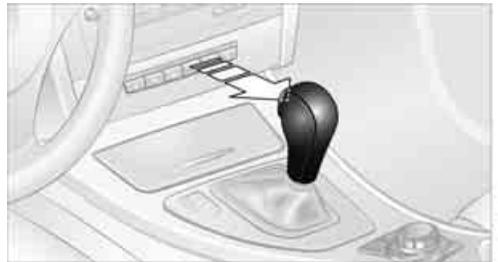
A lock prevents you from inadvertently engaging selector lever positions R and P. To cancel the lock, press the button on the front of the selector lever, see arrow.
