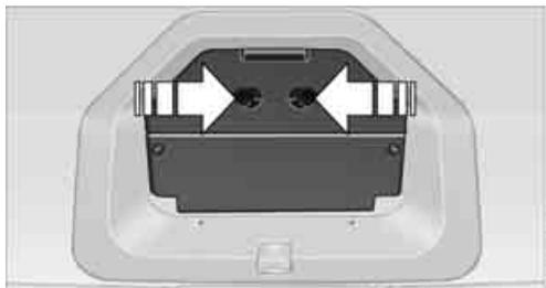
3. In the cargo area: press the two recesses together and fold down the cover.
