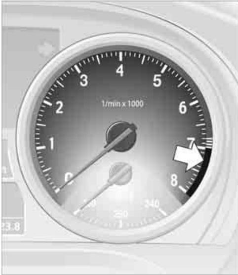
Never force the engine speed up into the red warning field, see arrow. In this range, the fuel supply is interrupted to protect the engine.
