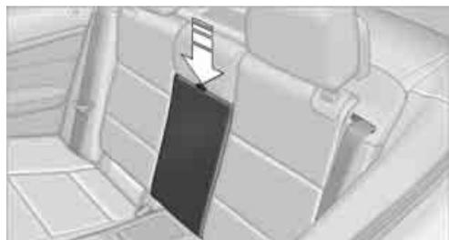
2. Front cover: press the two recesses together and fold the cover down until it engages.
