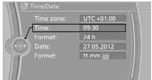
6. Turn the controller to set the hours and press the controller.
