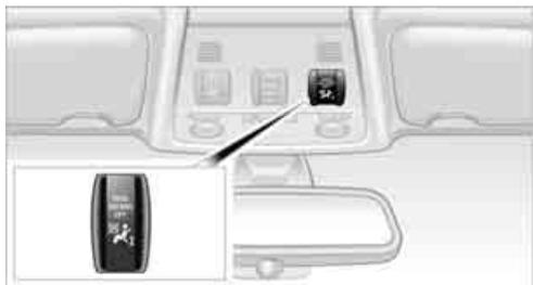
The indicator lamp for the front passenger airbags shows the functional status of the front passenger front and side airbags in accordance with whether and how the front passenger seat is occupied. The indicator lamp shows whether the front passenger airbags are activated or deactivated.
