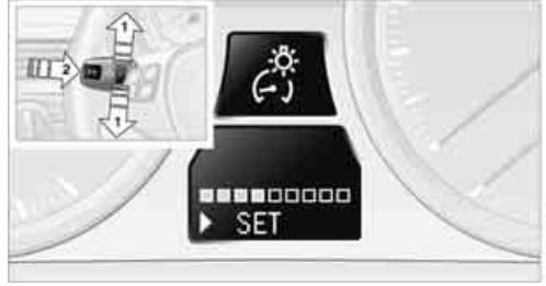
1. Push button 1 up or down repeatedly until the appropriate symbol appears in the display, accompanied by the brightness setting and scale the word "SET".
