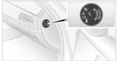
The passenger safety belt can be locked with a key switch so that it is prevented from being pulled out.
