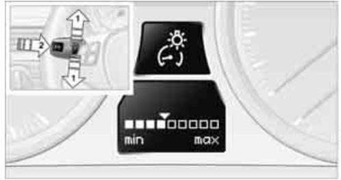
3. Push button 1 up or down to select the desired brightness level.
