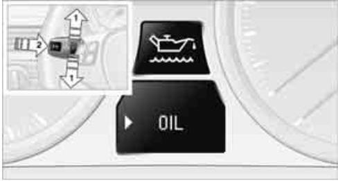
1. Push button **1** in the turn signal/high beam lever up or down repeatedly until the appropriate symbol is shown in the display, accompanied by the word "OIL".
