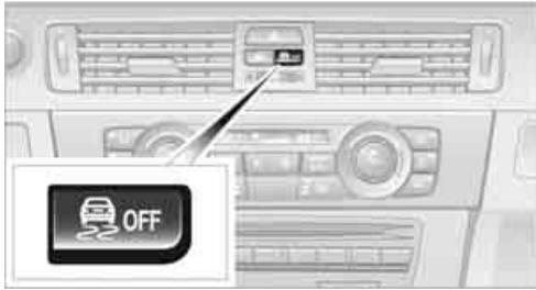
Press the button for at least 3 seconds until the indicator lamp for DSC OFF lights up and DSC OFF is displayed in the instrument cluster. Dynamic Traction Control DTC and DSC have been simultaneously deactivated. Stabilizing and drive-output promoting actions are no longer executed.
