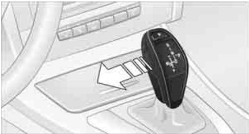
Push selector lever toward the left from the selector lever position D, the Sport program is activated. This position is recommended for a performance-oriented driving style. The engaged gear, e.g. S1, is displayed in the instrument cluster.
