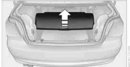
When the hardtop is closed you can enlarge the cargo area:
