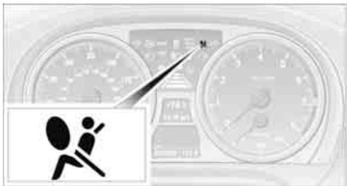
As of radio readiness, refer to page 61, the warning lamp lights up briefly to indicate that the entire airbag system and the belt tensioners are operational.
