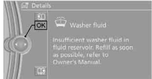
You can call up more information on the Control Display, e.g. on the cause of a malfunction and on how to respond, via Check Control, refer to page 92.
