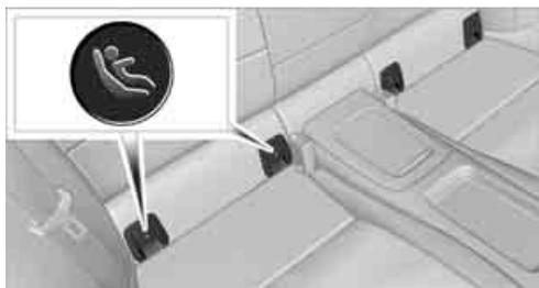
The mounts for the lower LATCH anchors are located behind the labeled protective caps.
