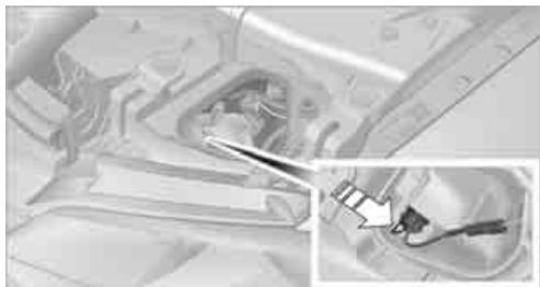
4. Disconnect the plug, change the bulb and reconnect the plug.
