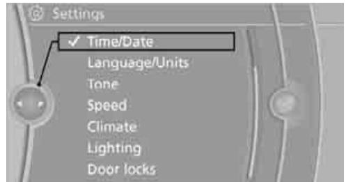
5. Turn the controller until "Time:" is highlighted, and then press the controller.
