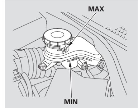
The fluid level should be between the MIN and MAX marks on the side of the reservoir. If the level is at or below the MIN mark, your brake system needs attention. Have the brake system inspected for leaks or worn brake pads.
