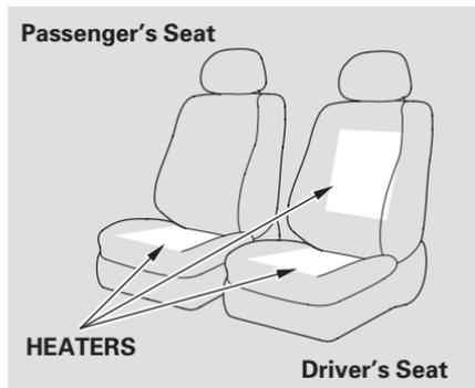
Both front seats are equipped with seat heaters. The passenger seat is only heated in the seat bottom because of the side airbag cutoff system.
