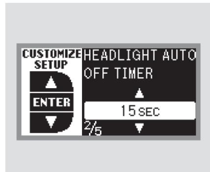
Press the SEL/RESET button. The screen changes as shown above. Select how long you want the lights to stay on before they go off (0, 15, 30, or 60 seconds) by pressing the INFO (▲/▼) button, then press the SEL/RESET button to enter your selection.
