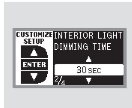
Press the SEL/RESET button. The screen changes as shown above. Select how long you want the lights to stay on before they fade out (15, 30, or 60 seconds) by pressing the INFO ( $\blacktriangle/\blacktriangledown$ ) button, then press the SEL/RESET button to enter your selection.
