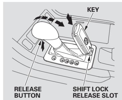
6. Remove the key from the shift lock release slot, then install the cover. Make sure the notch on the cover is on the rear. Return the key to the ignition switch, press the brake pedal, and restart the engine.
