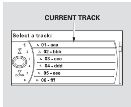
To select a track, rotate the interface dial or push up and down the selector on the interface dial. Then press ENTER on the selector to enter your selection.
