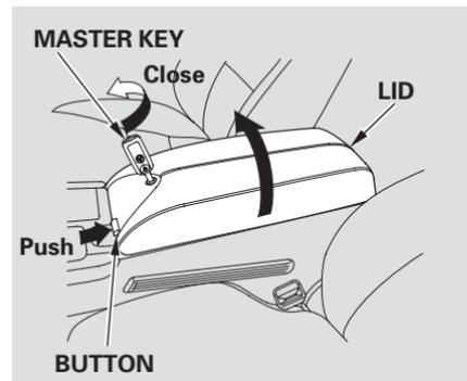
To open the console compartment, push the button and lift the lid.
