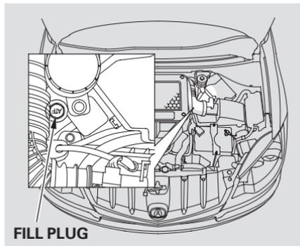
5. If the level is below the lower mark, remove the fill plug, then add the fluid into the fill hole to bring it to the level between the upper and lower marks on the dipstick.
