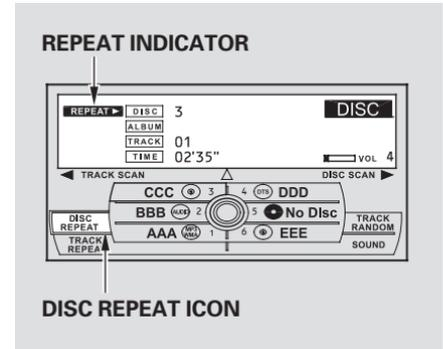
**DISC REPEAT** – This feature, when activated, continuously replays the current CD. Press the AUDIO button to view the audio control display, then push down the selector on the interface dial. Rotate the interface dial to select the disc repeat. Press ENTER on the selector to enter your selection. You will see “REPEAT” next to the DISC icon on the audio control display. To turn off this feature, select the disc repeat, then press ENTER again.
