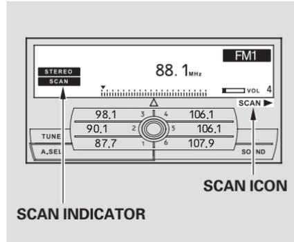
**SCAN** – The SCAN function samples all stations with strong signals on the selected band. To activate it, press the SCAN button, then release it. You will see “SCAN” on the upper display.
