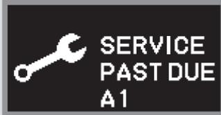
If the indicated maintenance service is not done and the remaining engine oil life reaches 0%, the multi-information display will show the message “SERVICE PAST DUE” and the maintenance item code(s). This message is displayed when the total mileage is less than 10 miles (for U.S. models) or 10 km (for Canadian models) after the engine oil life became 0%.
