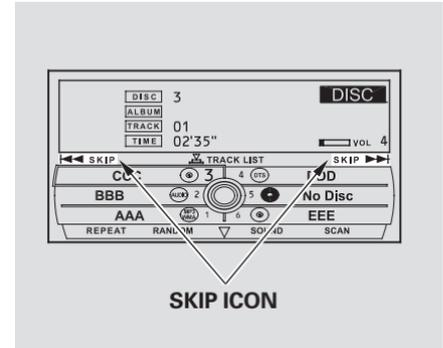
You can also change tracks/files on the audio control display. Press the AUDIO button to view the display, then push the selector on the interface dial to the right to skip forward to the beginning of the next track/file. Push the selector left to skip backward to the beginning of the current track/file. Press it again to skip to the beginning of the previous track/file.
