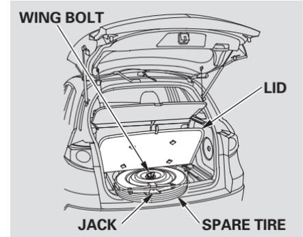
3. Open the tailgate. Raise the cargo area floor lid by lifting it up with the strap, then remove the lid. The spare tire, jack, and tools are under the cargo area floor.
