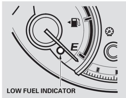
This indicator comes on as a reminder that you must refuel soon. When the indicator comes on, there is about 2.5 U.S. gal (9.5 ℓ) of fuel remaining in the tank.
