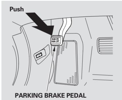
To apply the parking brake, push the pedal down with your foot. To release it, push on the pedal again. The parking brake indicator on the instrument panel should go out when the parking brake is fully released (see page [65](#)).
