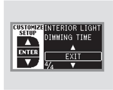
To exit INTERIOR LIGHT DIMMING TIME without changing the current setting, select EXIT by pressing the INFO (▲/▼) button, then press the SEL/RESET button. The screen goes back to CUSTOMIZE MENU.
