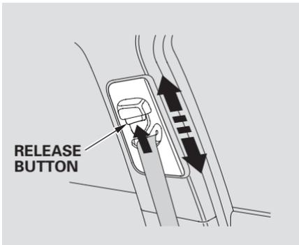
The front seats have adjustable seat belt anchors. To adjust the height of an anchor, press and hold the release button and slide the anchor up or down as needed (it has four positions).
