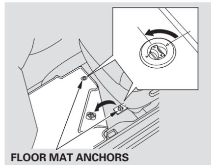
The driver's and front passenger's floor mats that came with your vehicle hook over the floor mat anchors. To lock each anchor, turn the knob clockwise. This keeps the floor mats from sliding forward (possibly interfering with the pedals), or backwards (making the front passenger's weight sensors ineffective). If you remove a floor mat, make sure to re-anchor it when you put it back in your vehicle.
