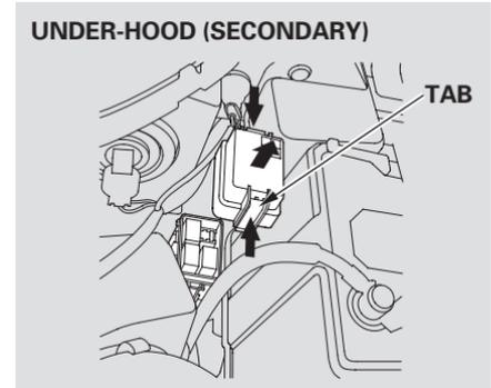
The secondary under-hood fuse box is next to the battery. To open it, push the tabs as shown.
