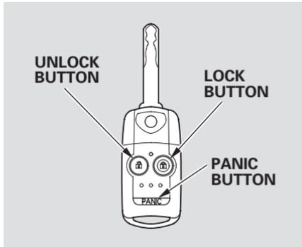
**LOCK** — Press this button once to lock all doors and the tailgate. Some exterior lights will flash. When you push LOCK twice within 5 seconds, you will hear a beep to verify that the doors and tailgate are locked and the security system has set. This button does not work if any door or tailgate is not fully closed.
