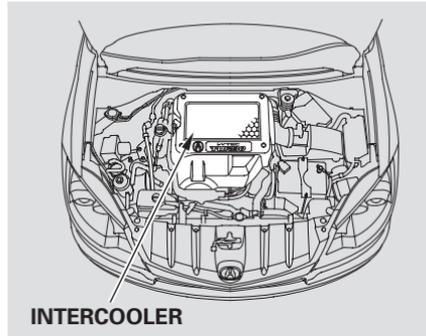
Your vehicle is equipped with a intercooler on the engine to cool the air flow from a turbo charger into the engine. The intercooler fins bend easily. Do not push them with your finger.
