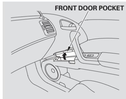
The interior of each front door has an extendable pocket for maps and other small, lightweight items. For safety, be sure both front door pockets are closed while driving.
