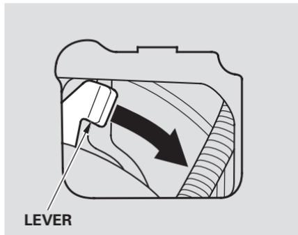
Push and hold the release lever to the right as shown, then push the tailgate to open it.
