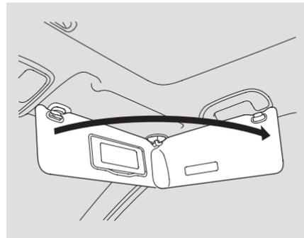
To use the sun visor, pull it down. You can also use the sun visor at the side window. Remove the support rod from the clip and swing the sun visor toward the side window.
