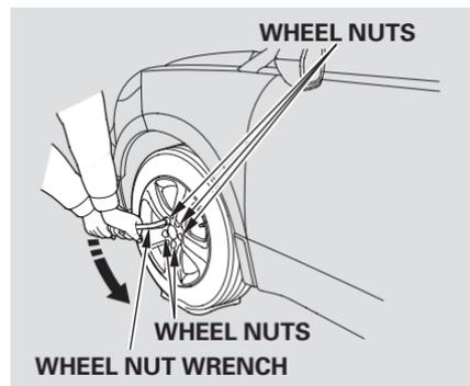
6. Loosen the five wheel nuts 1/2 turn with the wheel nut wrench.
