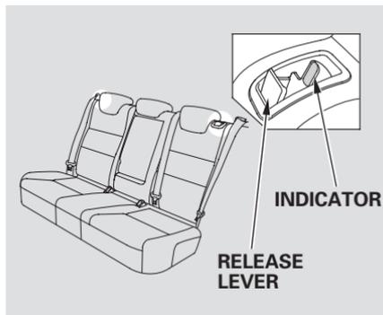
After returning the seat-back to the upright position, tug on the seat-back to make sure it is latched. If the seat-back is not latched fully, the seat belt will not work properly and you will see the red indicator behind the release lever as shown.
