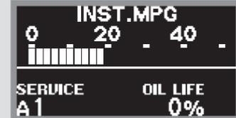
Press the SEL/RESET button on the steering wheel repeatedly to select the engine oil life. The message “SERVICE”, along with “0%”, and the maintenance item code are displayed on the lower part of the multi-information display when the calculated engine oil life is 0–1%.
