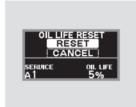
3. Press and hold the SEL/RESET button on the steering wheel for more than 10 seconds. The remaining engine oil life reset mode will be shown on the multi-information display.
