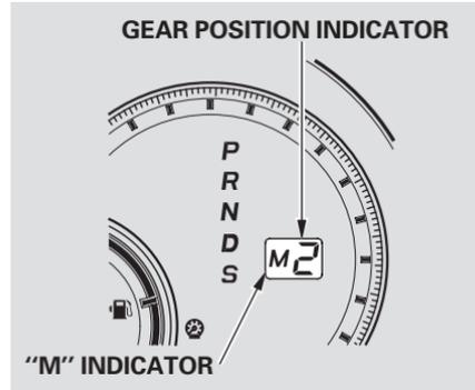
When you move the shift lever from “D” to “S” position and pull either paddle shifter, the gear position indicator displays “M” along with the selected gear number.
