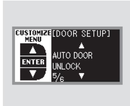
While DOOR SETUP is shown in the CUSTOMIZE GROUP of the multi-information display, press the SEL/RESET button. The screen changes to CUSTOMIZE MENU. Press the INFO (▲/▼) button until you see the above display.
