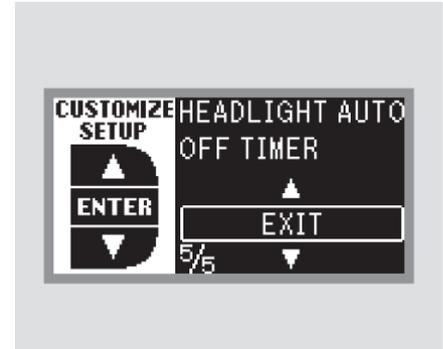
To exit HEADLIGHT AUTO OFF TIMER without changing the current setting, select EXIT by pressing the INFO (▲/▼) button, then press the SEL/RESET button. The screen goes back to CUSTOMIZE MENU.
