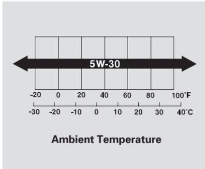
The oil viscosity or weight is provided on the container's label. 5W-30 oil is formulated for year-round protection of your vehicle to improve cold weather starting and fuel economy.
