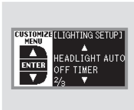
While LIGHTING SETUP is shown in the CUSTOMIZE GROUP of the multi-information display, press the SEL/RESET button. The screen changes to CUSTOMIZE MENU. Press the INFO (▲/▼) button until you see the above display.
