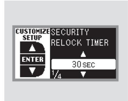
Press the SEL/RESET button. The screen changes as shown above. Select the relock time you want (30, 60, or 90 seconds) by pressing the INFO (▲/▼) button, then press the SEL/RESET button to enter your selection.
