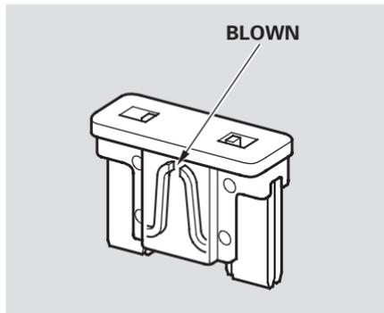
5. Look for a blown wire inside the fuse. If it is blown, replace it with one of the spare fuses of the same rating or lower. The spare fuses are provided on the back of the under-hood fuse cover.
