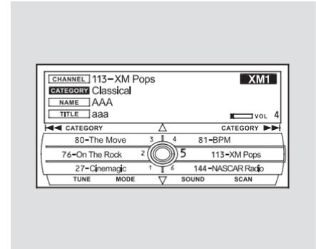
**MODE** — To switch between the category mode and channel mode, press and hold the DISP/MODE button until the mode changes. A “CH” (channel) or “CAT” (category) mode indicator appears on the upper display.
