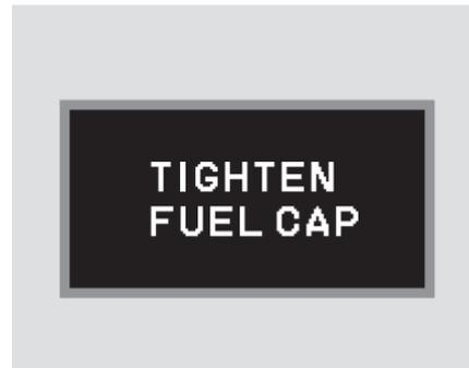
If your fuel fill cap is loose or missing, a “TIGHTEN FUEL CAP” message appears on the multi-information display after you start the engine.
