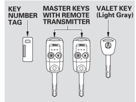
The master key fits all the locks on your vehicle. The valet key works only in the ignition and the door locks. You can keep the glove box and console compartment locked when you leave your vehicle and the valet key at a parking facility.
