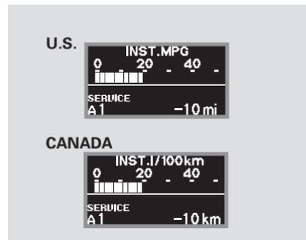
When you press the SEL/RESET button to select the engine oil life, the message “SERVICE”, along with the maintenance item code and the total negative mileage after the oil life became 0 %, will be displayed on the lower part of the multi-information display.
