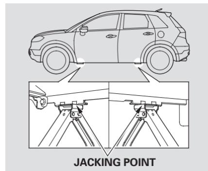
7. Place the jack under the jacking point nearest the tire you need to change. Turn the end bracket clockwise until the top of the jack contacts the jacking point. Make sure the jacking point tab is resting in the jack notch.
