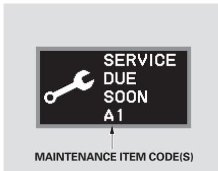
When the remaining engine oil life is 15 to 6 percent, the multi-information display shows a “SERVICE DUE SOON” message along with the maintenance schedule code indicating the main and sub items required at the time of the oil change. Refer to page [334](#) for a complete list of the maintenance main items and sub items.
