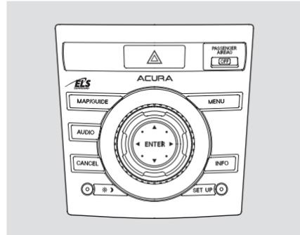
Most AcuraLink functions are controlled by the interface dial. The interface dial has two parts, a knob and a selector.
