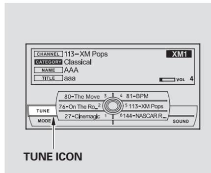
You can also change channel selections on the audio control display. Press the AUDIO button to view the display, then push down the selector on the interface dial. Rotate the interface dial to select the tune. Press ENTER on the selector to enter your selection. Rotate the interface knob to the desired channel. In the category mode, you can only select channels within that category.
