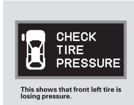
Each tire has its own pressure sensor. If the air pressure of a tire becomes significantly low, the sensor in that tire immediately sends a signal that causes the low tire pressure/TPMS indicator in the instrument panel to come on. If this happens, you will see which tire is losing pressure on the multi-information display along with a "CHECK TIRE PRESSURE" message.
