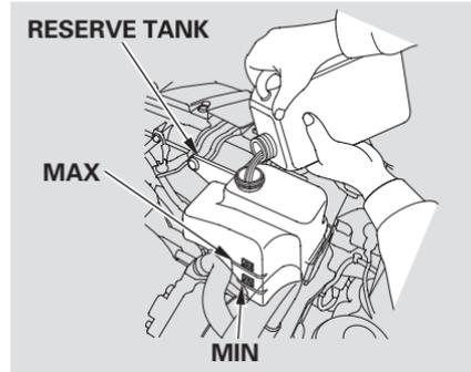
4. The coolant level should be up to the base of the filler neck. Add coolant if it is low.
