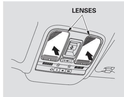
You can use the front ceiling lights whenever the lights are off. To turn a light on or off, push its lens.
