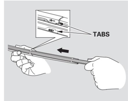
5. Install the new blade onto the blade assembly:
