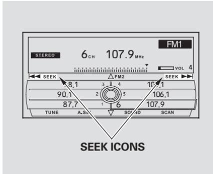
**SEEK** – The SEEK function searches up and down from the current frequency to find a station with a strong signal. To activate it, press the ◀◀ or ▶▶ side of the SEEK/SKIP bar, then release it.
