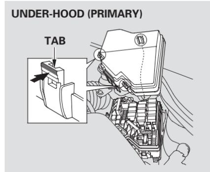
The primary under-hood fuse box is in the engine compartment on the driver's side. To open it, push the tabs as shown.
