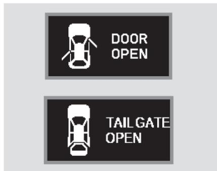
When one or more doors are not tightly closed, the “DOOR OPEN” message will come on. When the tailgate is not tightly closed, the “TAILGATE OPEN” message will come on.
