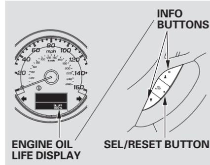
To see the current engine oil life, turn the ignition switch to the ON (II) position, and push and release the INFO ( $\blacktriangle$ / $\blacktriangledown$ ) button on the steering wheel repeatedly, until the engine oil life is displayed (see page [73](#) ).
