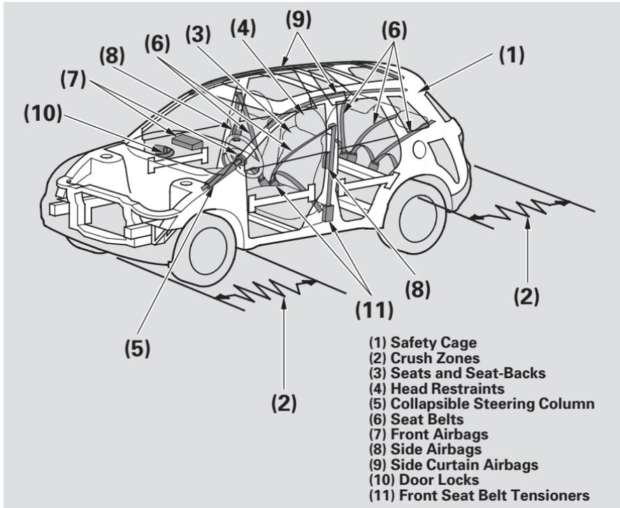
Your vehicle is equipped with many features that work together to protect you and your passengers during a crash.
