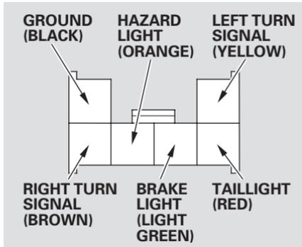
Your vehicle has a trailer lighting connector located under the right side tool case in the cargo area. Refer to the drawing above for the wiring color code and purpose of each pin.
