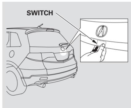
To open the tailgate, press and hold the switch, then lift up.
