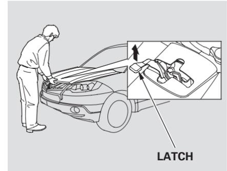
2. Put your fingers under the front edge of the hood near the center. Slide your hand to the left until you feel the hood latch handle. Push this handle up to release it. Lift up the hood.
