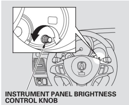
The knob on the instrument panel controls the brightness of the instrument panel lights. Turn the knob to adjust the brightness. Separate adjustments can be made when the headlights are on and off.
