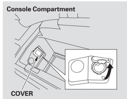
None of the sockets will power an automotive type cigarette lighter element. When both sockets are being used, the combined power rating of the accessories should be 120 watts or less (10 amps).
