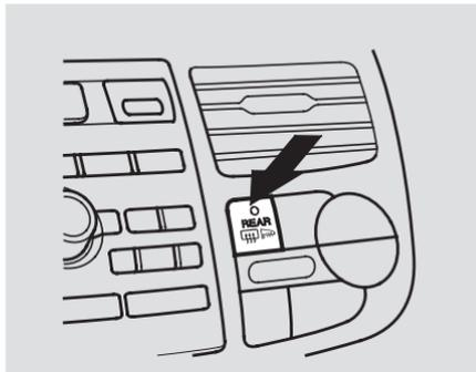
The rear window defogger clears fog, frost, and thin ice from the window. Push the defogger button to turn it on and off. Pushing this button also turns the mirror heaters on and off. The indicator in the button comes on to show the defogger is on.
