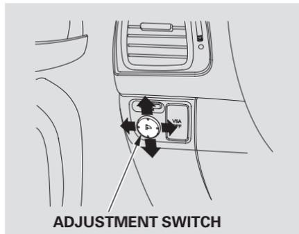
3. Push the appropriate edge of the adjustment switch to move the mirror right, left, up, or down.
