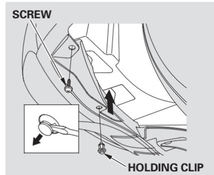
1. Use a Phillips-head screwdriver to remove the screw and use a flat-tipped screwdriver to remove the holding clip located under the front bumper.
