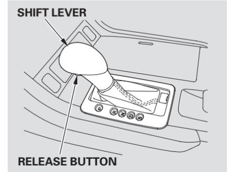
To shift from Park to any position, press firmly on the brake pedal and press the release button on the front of the shift lever, then pull the lever. You cannot shift out of Park when the ignition switch is in the LOCK (0) or the ACCESSORY (I) position.
