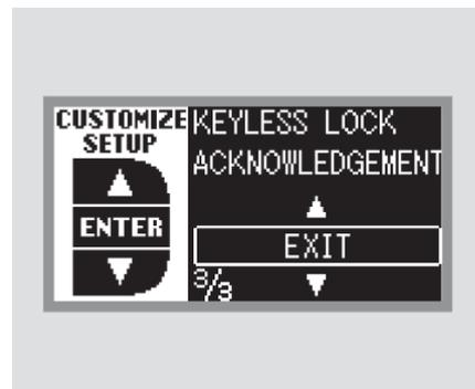
To exit KEYLESS LOCK ACKNOWLEDGEMENT without changing the current setting, select EXIT by pressing the INFO (▲/▼) button, then press the SEL/RESET button. The screen goes back to CUSTOMIZE MENU.
