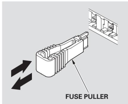
4. Check the smaller fuses in the under-hood fuse box and all the fuses in the interior fuse box by pulling out each one with the fuse puller provided on the back of the primary under-hood fuse box cover.
