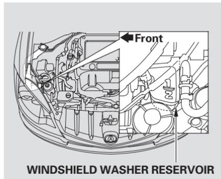
*On U.S. models:* To check the windshield washer fluid level, open the hood and look at the windshield washer reservoir located behind the left headlight. You will see a "1/2" mark on the reservoir.
