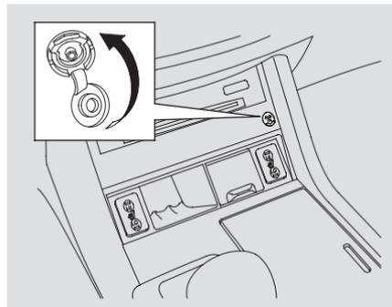
The auxiliary input jack is on the disc changer unit. The system will accept auxiliary input from standard audio accessories.
