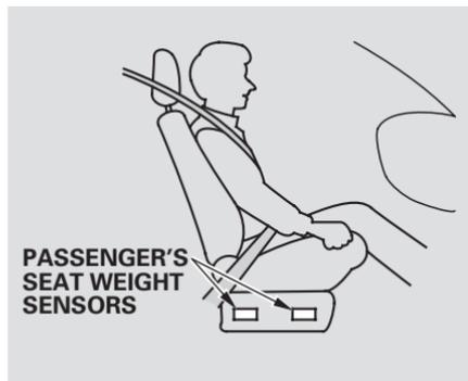
The passenger's advanced front airbag system has weight sensors under the seat. Although Acura does not encourage carrying an infant or small child in front, if the sensors detect the weight of an infant or small child (up to about 65 lbs or 29 kg), the system will automatically turn the passenger's front airbag off.
