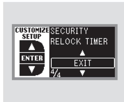
To exit SECURITY RELOCK TIMER without changing the current setting, select EXIT by pressing the INFO (▲/▼) button, then press the SEL/RESET button. The screen goes back to CUSTOMIZE MENU.
