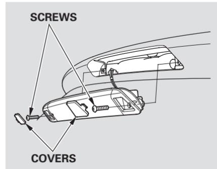
1. Remove the two screw covers on the light assembly by prying on the side edge with a flat-tip screwdriver.
