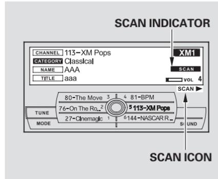
You can also scan the channels on the audio control display. Press the AUDIO button to view the display, then push down the selector on the interface dial. Push the selector to the right to activate scan feature.
