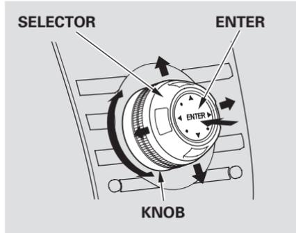
Most audio system functions can still be controlled by standard buttons, bars, and knob, but some functions can only be accessed using the interface dial. The interface dial has two parts, a knob and a selector.
