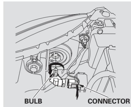
3. Insert the new bulb into the hole, and turn it one-quarter turn clockwise to lock it in place.
