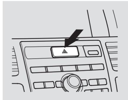
Push the button between the center vents to turn on the hazard warning lights (four-way flashers). This causes all outside turn signals and both indicators in the instrument panel to flash. Use the hazard warning lights if you need to park in a dangerous area near heavy traffic, or if your vehicle is disabled.
