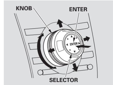
The knob turns left and right. Use it to make selections or adjustments to a list or menu on the screen.
