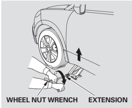
8. Use the extension and the wheel nut wrench as shown to raise the vehicle until the flat tire is off the ground.
