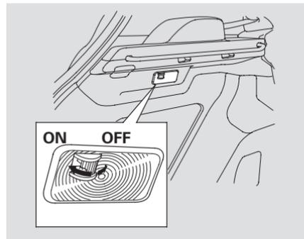
The cargo area light has a two position switch. In the OFF (right) position, the light does not come on. In the ON (left) position, the light comes on when you open the tailgate.
