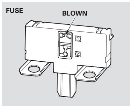
3. Check each of the large fuses in the under-hood fuse box by looking through the side window at the wire inside. Remove the screws with a Phillips-head screwdriver.
