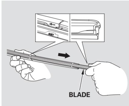
3. Remove the blade from the blade assembly:
