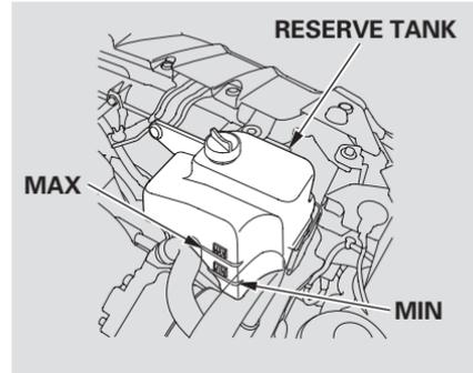
Look at the coolant level in the radiator reserve tank. Make sure it is between the MAX and MIN lines. If it is below the MIN line, see **Adding Engine Coolant** on page [340](#) for information on adding the proper coolant.
