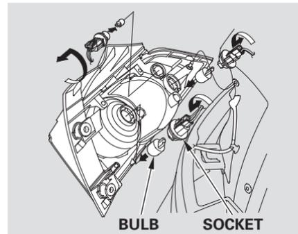
3. Determine which of the three bulbs is burned out: brake/taillight, turn signal or rear side marker.
