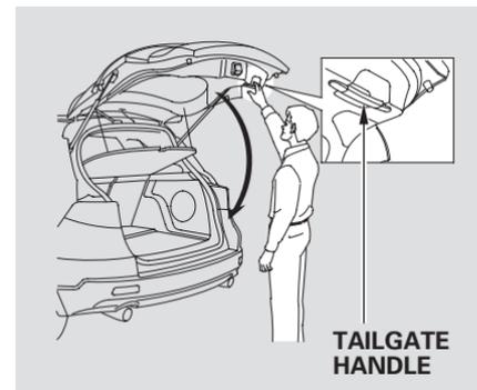
To close the tailgate, hold the tailgate handle, lower the tailgate, then press down on the back edge.
