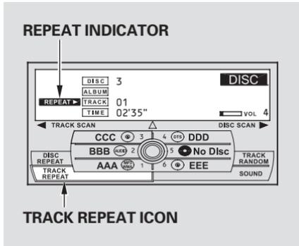
**REPEAT** – This feature, when activated, continuously replays the current track (file in MP3/WMA mode). To activate it, press the AUDIO button to view the display, then push down the selector on the interface dial. Rotate the interface dial to select track repeat. Press ENTER on the selector to enter your selection.
