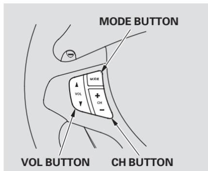
The VOL button adjusts the volume up (▲) or down (▼). Press the top or bottom of the button, hold it until the desired volume is reached, then release it.
