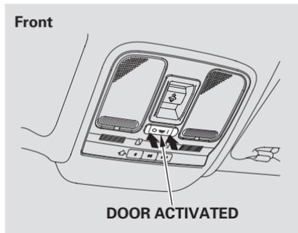
Each front and rear ceiling light has a three-position switch.
