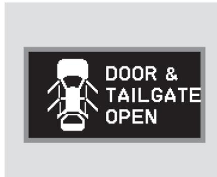
When both tailgate and one or more doors are not tightly closed, the “DOOR & TAILGATE OPEN” message will come on.
