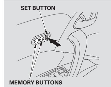
3. Press and release the SET button on the control panel. You will hear a beep. Immediately press and hold one of the memory buttons (1 or 2) until you hear two beeps. The indicator in the memory button will come on. The current positions of the driver's seat and outside mirrors are now stored.
