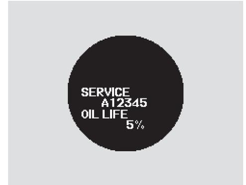
Press the SEL/RESET button on the steering wheel repeatedly to select the engine oil life. The message “SERVICE,” along with “5%,” and the maintenance item code are displayed on the multi-information display when the calculated engine oil life is 1–5 percent (see page 409).
