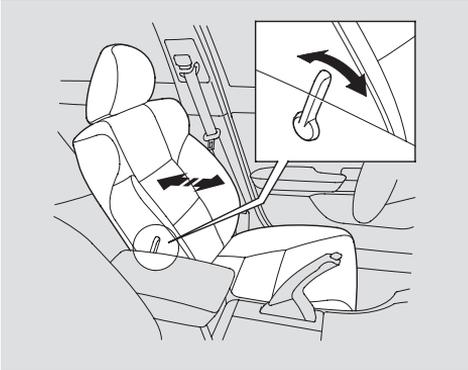
Vary the lumbar support by moving the lever on the side of the seat-back. Move the lever forward or backward to adjust the lumbar support through its full range.
