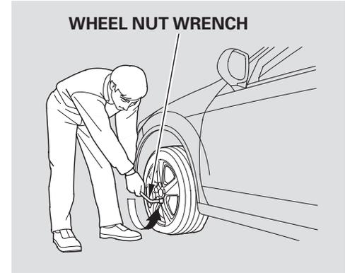
7. Loosen each wheel nut 1/2 turn with the wheel nut wrench.
