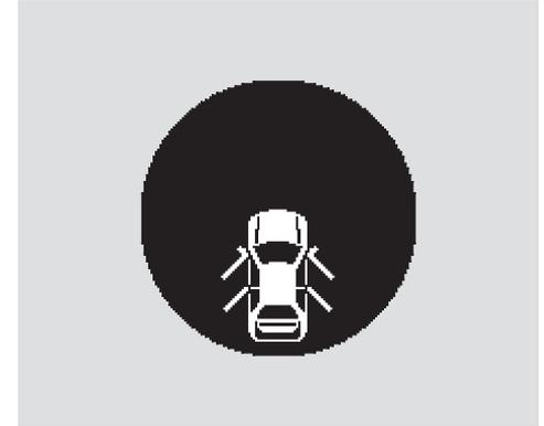
You will also hear a beep when you turn the ignition switch to the ON (II) position, and each time you open any door or the trunk with the key in the ON (II) position.
