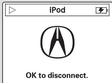
When the iPod is connected and the iPod mode is selected on the audio display, the USB and iPod indicators are shown in the display. After loading, you will see Acura mark\* on the iPod. That means you can only operate your iPod using the vehicle's audio unit.
