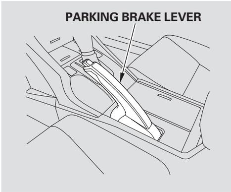
To apply the parking brake, pull the lever up fully. To release it, pull up slightly, push the button, and lower the lever. The parking brake indicator on the instrument panel should go out when the parking brake is fully released (see page [61](#)).
