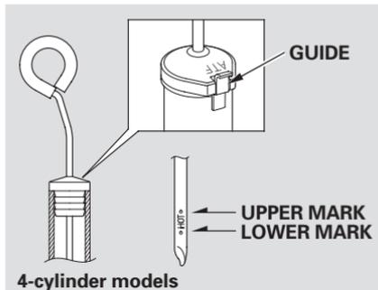
3. Insert the dipstick all the way back into the transmission securely as shown in the illustration.
