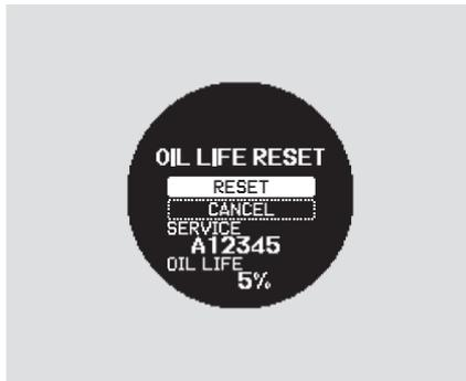
4. Select “RESET” by pressing the INFO (▲/▼) button, then press the SEL/RESET button to reset the engine oil life display. The maintenance item code(s) will disappear, and the engine oil life will reset to “100.” If you want to cancel the oil life reset mode, select “CANCEL.”
