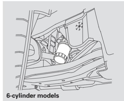
5. Remove the oil filter and let the remaining oil drain. A special wrench (available from your dealer) is required.
