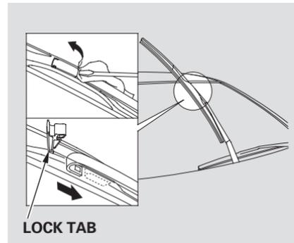
2. Disconnect the blade assembly from the wiper arm:
