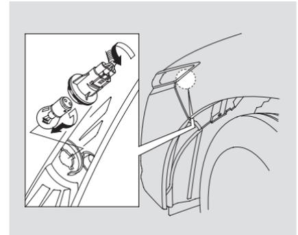
4. Remove the socket from the headlight assembly by turning it one-quarter turn counterclockwise.
