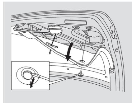
3. Pull back the appropriate corner of the trunk lid lining carefully.
