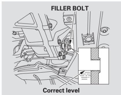
Remove the transmission filler bolt, and carefully feel inside the bolt hole with your finger.
