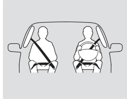
In addition, your vehicle has side curtain airbags to help protect the heads of the driver, front passenger, and passengers in the outer rear seating positions during a moderate to severe side impact (see page [31](#) for more information on how your side curtain airbags work).
