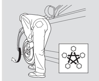
14. Tighten the wheel nuts securely in the same crisscross pattern. Have the wheel nut torque checked at the nearest automotive service facility.
