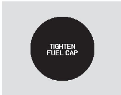
Your vehicle's on board diagnostic system will detect a loose or missing fuel fill cap as an evaporative system leak. The first time a leak is detected a “TIGHTEN FUEL CAP” message appears on the multi-information display.
