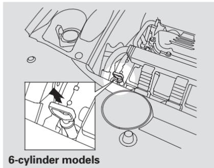
3. Insert the dipstick all the way back into its hole.
