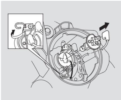
5. Unclip the end of the hold-down wire from its slot. Pivot it out of the way.
