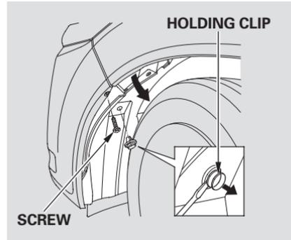
2. Use a flat-tip screwdriver to remove the holding clip from the inner fender, and remove the screw with a Phillips-head screwdriver.
