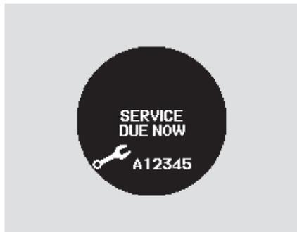
When the remaining oil life is 5 to 1 percent, the multi-information display shows a “SERVICE DUE NOW” message with the same maintenance items “SERVICE DUE SOON” was displayed with. When you see this message, have the indicated maintenance performed as soon as possible.
