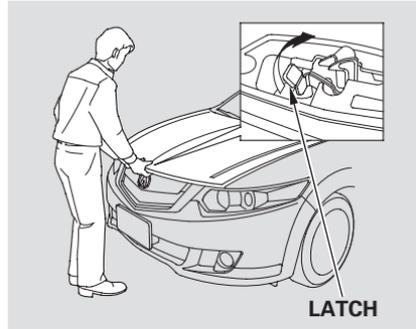
2. Reach in between the hood and the front grille with your fingers. The hood latch handle is above the "A" logo. Push this handle up to the right until it releases the hood. Lift the hood.
