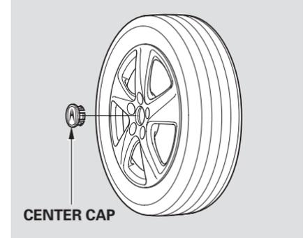
15. Remove the center cap before storing the flat tire in the trunk well.
