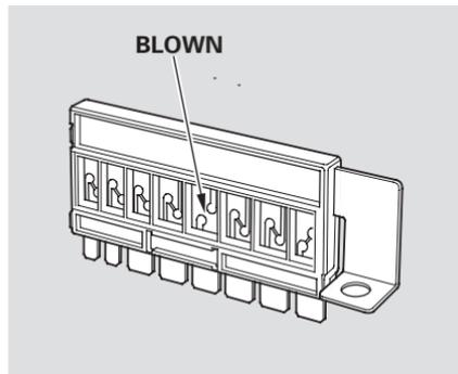
Also check the combined fuse box in the under-hood fuse box.
