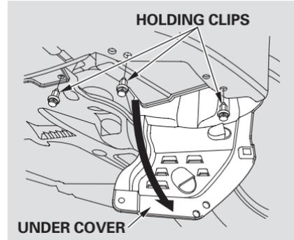
1. Remove the three holding clips with a flat-tip screwdriver.
