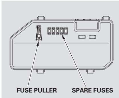
Your vehicle has spare fuses on the back of the under-hood fuse box cover.
