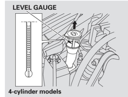
Check the reservoir's fluid level by removing the cap and looking at the level gauge attached to the cap.
