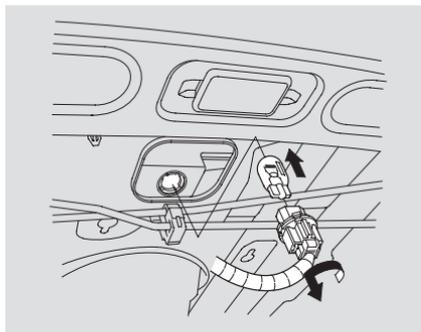
1. Open the trunk, and remove the socket from the light assembly by turning it one-quarter turn counter-clockwise.
