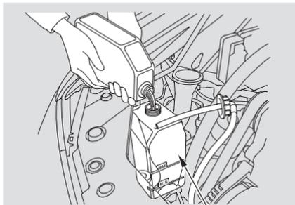
If the coolant level in the reserve tank is at or below the MIN line, add coolant to bring it up to the MAX line. Inspect the cooling system for leaks.
