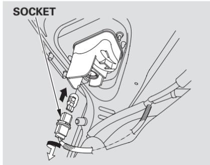
4. Remove the socket by turning it one-quarter turn counterclockwise.
