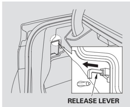
To open the fuel fill door, pull the release lever rearward.
