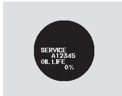
Press the SEL/RESET button on the steering wheel repeatedly to select the engine oil life. The message “SERVICE,” along with “0%,” and the maintenance item code are displayed on the multi-information display when the calculated engine oil life is 0–1 percent.
