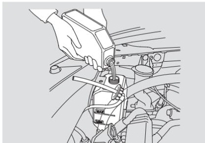
To access the radiator reserve tank, remove the right-side engine compartment cover.
