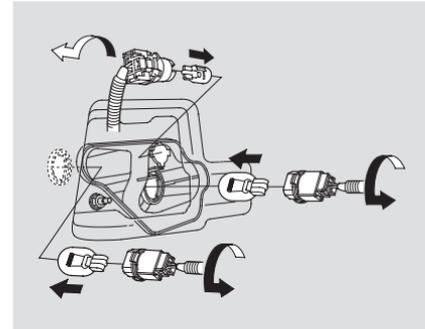
3. Determine which of the three bulbs is burned out: stop/taillight, rear side-marker, or turn signal light.
