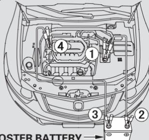
4. Connect one jumper cable to the positive (+) terminal on your battery. Connect the other end to the positive (+) terminal on the booster battery.
