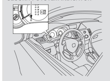
Once the security system is set, opening any door (without using the key or the remote transmitter), the hood, or the trunk will cause the alarm to activate. It will also activate if the audio unit is removed from the dashboard or the wiring is cut.
