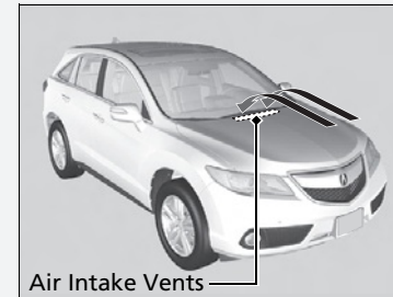
Air Intake Vents
