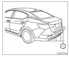
The RAB system detects obstacles behind the vehicle using the parking sensors (1) located on the rear bumper.
