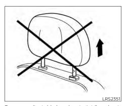
For non-adjustable head restraint/headrest Make sure the head restraint/headrest is positioned so the lock knob is engaged in the notch before riding in that designated
