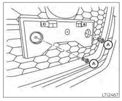
To mount the front license plate, attach the license plate bracket to the grille assembly at the location marks (small dimples) using the two provided screws (A).
