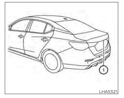
To display the rear view, the Rear View Monitor system uses a camera located just above the vehicle's license plate  $\Omega$ .
