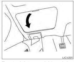
The extended storage switch is used when the vehicle is in transit from the factory. It is located in the fuse panel to the left of the steering wheel on the instrument panel. If any electrical equipment does not operate, ensure the extended storage switch is pushed fully in place, as shown.
