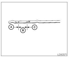
5. Remove the dipstick again and check the oil level. It should be between the H (High) and L (Low) marks (B). This is the normal operating oil level range. If the oil level is below the L (Low) mark (A), remove the oil filler cap and pour recommended oil through the opening. **Do not** overfill (3).
