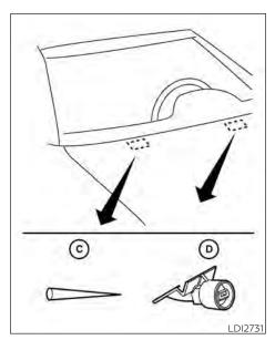
If you wax the surface of the hood, be careful not to let wax get into the washer nozzle (1) This may cause clogging or improper windshield-washer operation. If wax gets into the nozzle, remove it with a needle or small pin @.
