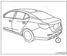
If dirt, rain or snow accumulates on the camera (1), the RearView Monitor may not display objects clearly. Clean the camera by wiping it with a cloth dampened with a diluted mild cleaning agent and then wiping it with a dry cloth.
