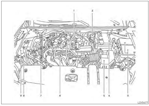
2.0L 4 cylinder (MR20DD engine model)
