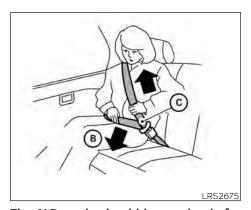
The ALR mode should be used only for child restraint installation. During normal seat belt use by an occupant, the ALR mode should not be activated. If it is activated, it may cause uncomfortable seat belt tension. It can also change the operation of the front passenger air bag. For additional information, see "Front passenger air bag and status light" (P. 1-53).
