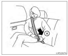
The ELR mode allows the seat belt to extend and retract to allow the driver and passengers some freedom of movement in the seat. The ELR locks the seat belt when the vehicle slows down rapidly or during certain impacts.
