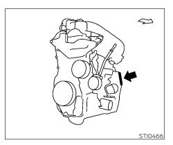
**ENGINE SERIAL NUMBER** The number is stamped on the engine as shown.
