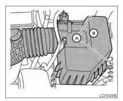
The viscous paper type filter element (if so equipped) should not be cleaned and reused. The dry paper type filter element (if so equipped) may be cleaned and reused. Replace it according to the maintenance log shown in the "Maintenance and schedules" section of this manual.
