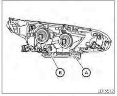
Type A (if so equipped) Replacing the halogen headlight bulb (if so equipped)
