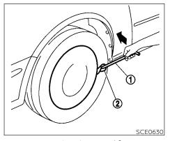
Removing wheel cover (if so equipped)
