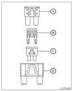
Four types of fuses are used. Type (A) is used exclusively in the passenger compartment fuse box.
