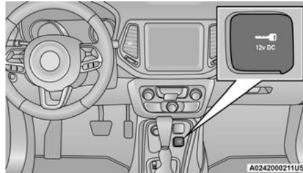
Front Power Outlet
