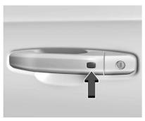
The remote key must be within 1 m (3 ft) of the liftgate or door being opened or locked. Press the button on the door handle to open. See "Keyless Access Operation" in Remote Keyless Entry (RKE) System Operation  $\Rightarrow$  8.
