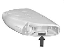
2. With the mechanical key removed, insert a flat, thin object in the center of the remote key to separate and remove the back cover.
