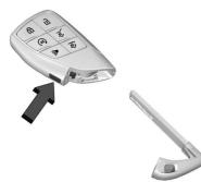
Press the button on the side of the remote key and pull the mechanical key out. Never pull the mechanical key out without pressing the button.
