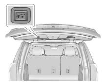
Press any liftgate button, the touch pad, or  $\cancel{3}$  on the remote key while the liftgate is moving to stop it. Pressing any liftgate button or pressing  $\cancel{3}$  twice quickly on the remote key restarts the operation in the reverse direction. Pressing the touch pad on the liftgate handle will restart the motion, but only in the opening direction.
