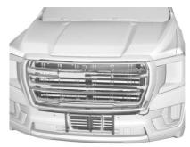
The vehicle may have a shutter system designed to help improve fuel economy. Keep the shutter system clear of debris,
