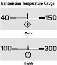
This gauge displays while the vehicle is in the Tow/Haul driver mode, and the lower gauges are configured to display four gauges. The transmission fluid temperature is also selectable as Left/Right side info. To change gauge configurations, see "Options" under *Instrument Cluster* ⇔ 105.
