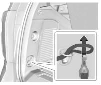
4. Remove the flat tire secure strap from the glove box and place the loop end of the strap through the cargo tie-down. Place the hook end of the strap through the loop and pull it until the strap is fastened securely to the tie-down.
