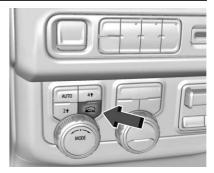
If equipped, select Terrain Mode by pressing the  $\overbrace{}{}$  below the 4  $\uparrow$  transfer case button.
