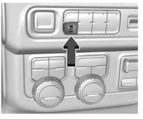
The button for TCS and StabiliTrak/ESC is on the instrument panel to the left of the steering wheel. Caution
