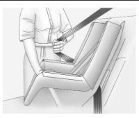
Pull the shoulder belt all the way out of the retractor to set the lock. When the retractor lock is set, the belt can be tightened but not pulled out of the retractor.
