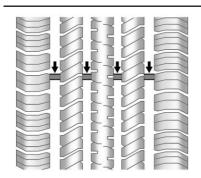
Treadwear indicators are one way to tell when it is time for new tires. Treadwear indicators appear when the tires have only 1.6 mm (1/16 in) or less of tread remaining. See *Tire Inspection*  $\Rightarrow$  339 and *Tire Rotation*  $\Rightarrow$  339 for additional information.
