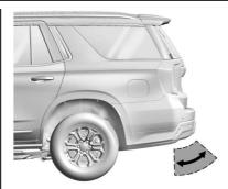
To operate, move your foot in a forward kicking motion under the center of the rear bumper, then pull it back.
