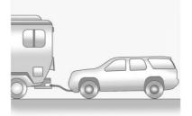
Only dinghy tow four-wheel-drive vehicles with a two speed transfer case that has an N (Neutral) and a 4 $\downarrow$  setting.
