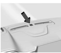
The solar sensor, on top of the instrument panel near the windshield, monitors the solar heat.
