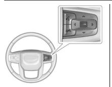
$\triangleleft$  or  $\triangleright$ : Press to move left or right between the interactive display zones in the instrument cluster. Press the thumbwheel to select.
