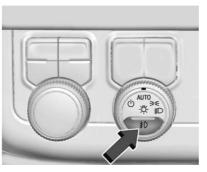
If equipped with fog lamps, the button is on the exterior lamp control, to the left of the steering column. The ignition must be on for the fog lamps to come on.
