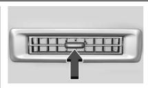
Move the slider knob on rectangular vents and rotate the outlet barrel left to right to change the direction of the air flow and to shut off the air flow.
