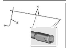
3. Assemble the jack handle extensions (4) and wheel wrench (5), as shown.
