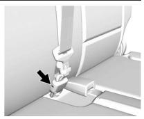
4. Disconnect the rear seat belt mini-latch, using a key in the slot on the mini-buckle, and let the belt retract into the headliner.
