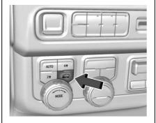
To activate Terrain Mode, press the Terrain Mode button located next to the Mode knob.
