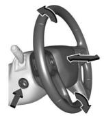
To adjust the steering wheel, if equipped:
