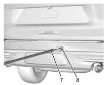
4. Insert the open end of the extension (7) through the hole in the rear bumper (8) (hoist shaft access hole).
