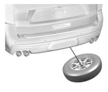
7. Tilt the tire toward the vehicle with some slack in the cable to access the tire/wheel retainer.
