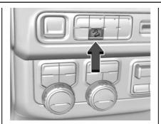
Press  $\overset{o}{\Rightarrow}$  to enable or disable HDC. Vehicle speed must be below 60 km/h (37 mph).
