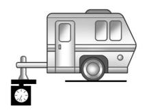
The Maximum Trailer Tongue Weight Rating for a conventional trailer hitch is shown on the Trailering Information Label.
