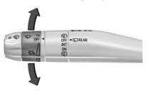
**AUTO :** Move the windshield wiper lever to AUTO. Turn the band on the wiper lever to adjust the sensitivity.
