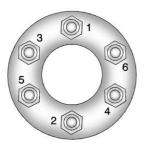
12. Tighten the nuts firmly in a crisscross sequence as shown by turning the wheel wrench clockwise.
