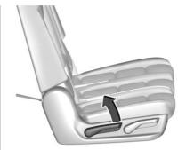
2. Lift the lever on the outboard side of the seat to release the seatback.
