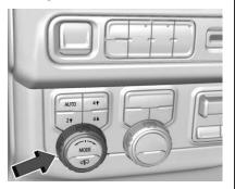
Turn the knob left or right to select the desired ride height in the menu. To finalize the selection, either press the Ride Height button again or wait three seconds for the menu to timeout. Ride Heights that are unavailable for selection will be greyed out in the menu.
