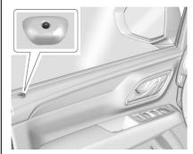
The indicator light, on the driver door near the window, indicates the status of the system. See *Power Door Locks*  $\Leftrightarrow$  15
