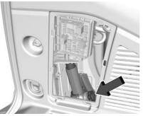
Turn the jack knob counterclockwise to release the jack and wheel blocks from the bracket. If equipped, remove the wheel blocks from the jack and place the wheel blocks on both sides of the tire at the opposite corner of the tire being changed. See *If a Tire Goes Flat* ⇒ 345 for more information on the placement of the wheel blocks. Place the jack and wheel blocks near the tire being changed.
