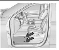
Reinstall by lining up the floor mat retainer openings over the carpet retainers and snapping into position.
