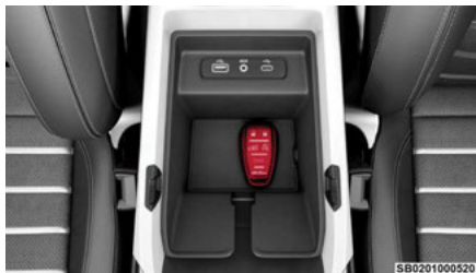
Key Fob Placement Location
