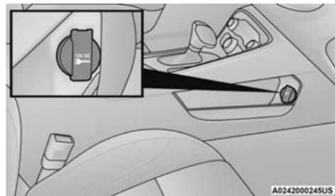
Power Outlet – Integrated Center Stack Front
