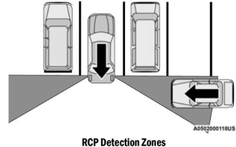
RCP monitors the rear detection zones on both sides of the vehicle, for objects that are moving toward the side of the vehicle with a minimum speed of approximately 3 mph (5 km/h), to objects moving a maximum of approximately 20 mph (32 km/h), such as in parking lot situations.
