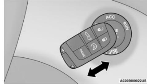
Depleted Key Fob Battery Procedure
