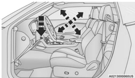
**Power Tilt/Telescoping Steering Column Control**
