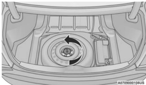
**Removing Tire Fastener**
