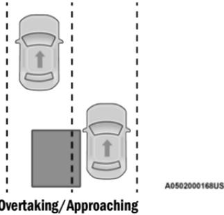
The BSM system is designed not to issue an alert on stationary objects such as guardrails, posts, walls, foliage, berms, etc. However, occasionally the system may alert on such objects. This is normal operation and your vehicle does not require service.
