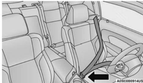
**Inserting Latch Plate Into Buckle**
