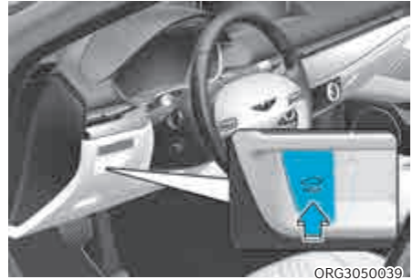
1. Power Trunk Main Control button
