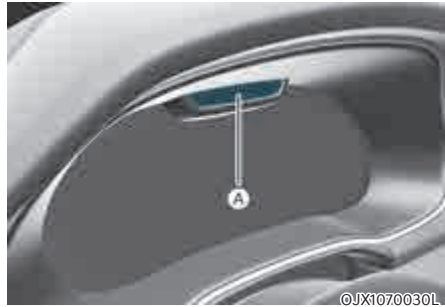
[A] : Interior view camera
