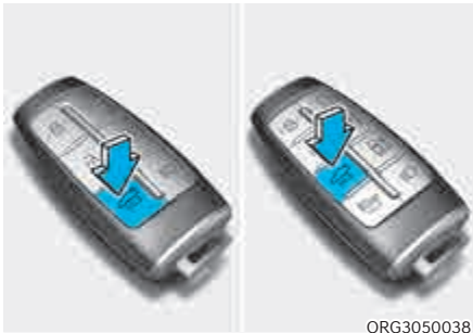
2. Power Trunk Open switch
