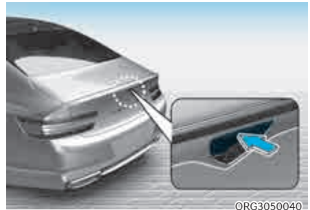
2. Power Trunk Open switch
