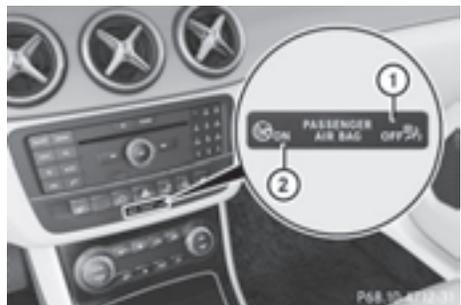
PASSENGER AIR BAG OFF indicator lamp ① and PASSENGER AIR BAG ON indicator lamp ② are part of the Occupant Classification System (OCS).
