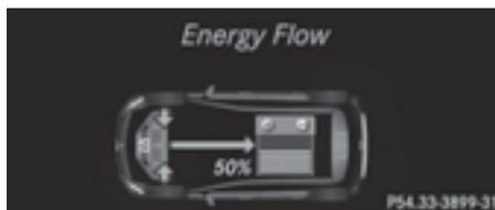
The kinetic energy of the vehicle is converted into electrical energy. The Recuperative Brake System is active. The high-voltage battery is being charged.
