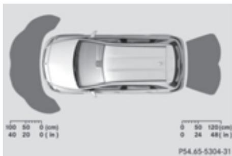
If there is an obstacle within this range, the relevant warning displays light up and a warning tone sounds. If the distance falls below the minimum, the distance may no longer be shown.
