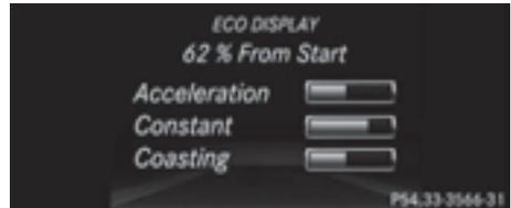
The ECO display provides feedback on how economical your driving characteristics are. The ECO display assists you in achieving the most economical driving style for the selected settings and prevailing conditions. Your driving style can significantly influence the vehicle's consumption.
