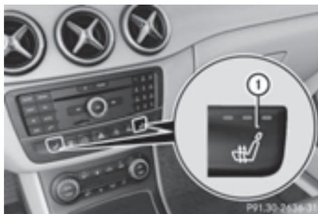
The three red indicator lamps in the button indicate the heating level you have selected. The system automatically switches down from level **3** to level **2** after approximately eight minutes.
