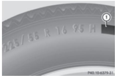
In addition to the load-bearing index, load index **1** may be imprinted after the letters that identify speed rating on the sidewall of the tire. Speed rating (▷ page 315).
