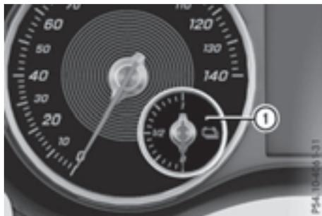
Condition of charge display ① shows the condition of charge of the high-voltage battery.
