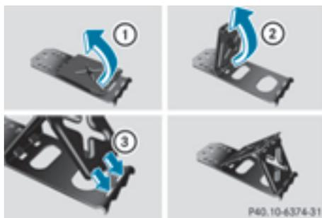
If your vehicle is equipped with a wheel chock, it can be found in the tire-change tool kit (▷ page 280).
