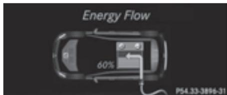
The drive system is switched off. The charging cable is connected and the high-voltage battery is being charged.
