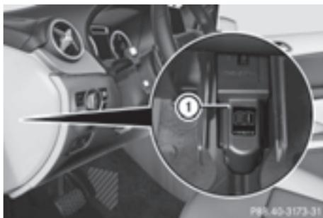
Your vehicle is equipped with a high-voltage switch-off device ① which can be used to switch off the vehicle's high-voltage electrical system.
