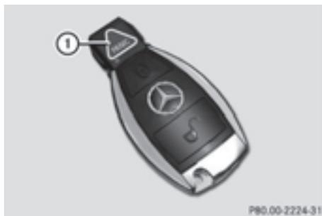
▶ **To activate:** press and hold the **PANIC** button **1** for approx. one second. A visual and audible alarm is triggered if the alarm system is armed.
