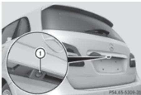
The rear view camera ① is an optical parking and maneuvering aid. It uses guide lines to show the area behind your vehicle in the Audio/COMAND display.
