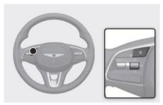
The cluster display modes can be changed by using the control switches.
