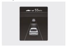
The status of Smart Cruise Control, Lane Following Assist, Highway Driving Assist, etc. appears when Driving Assist view is selected.
