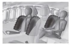
Your vehicle is equipped with a side airbag in each front and outboard second row seat. Additionally, a front center side airbag is provided in the inboard side of the driver seatback. The purpose of the airbag is to provide vehicle occupants with additional protection beyond that offered by the seat belt alone.
