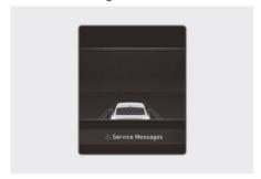
When Service Messages menu is selected, press the **OK** switch on the steering wheel to check vehicle warning messages.
