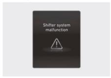
This message appears when the transmission or the shift button does not properly operate in the P (Park) position. Immediately have your vehicle inspected by an authorized retailer of Genesis Branded products.
