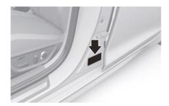
The vehicle certification label attached on the driver's (or front passenger's) side center pillar gives the vehicle identification number (VIN).
