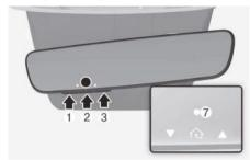
Press and release the HomeLink button (1), (2) or (3), you would like to program. The HomeLink indicator light (7) will flash orange slowly (if not, perform the steps of "Erasing HomeLink Buttons" section, and start over).
