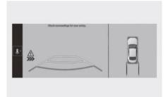
To warn the driver of an approaching vehicle from the rear left/right side of your vehicle, the warning light on the side view mirror will blink and a warning message will appear on the instrument cluster. At the same time, an audible warning will sound. A warning will also appear on the infotainment system.
