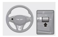
To change the trip mode, toggle the "^, \rightarrow" switch on the steering wheel.
