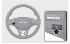
With the engine on, press and hold the Lane Driving Assist button (((a)) located on the steering wheel to turn on Lane Keeping Assist. The gray or green ((a)) indicator light will illuminate on the instrument cluster. Press and hold the button again to turn off the function. If the engine is restarted, Lane Keeping Assist will maintain the last setting.
