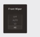
This indicator displays which wiper speed is selected using the wiper control.
