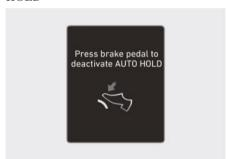
If you did not apply the brake pedal when you release Auto Hold by pressing the AUTO HOLD switch, a warning will sound and a message will appear.
