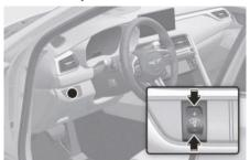
When the vehicle's parking lights or headlights are on, press the illumination control switch to adjust the brightness of the instrument panel illumination.
