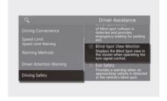
With the engine on, select **Setup** > **Vehicle** > **Driver Assistance** > **Driving Safety** and then enable **Blind-Spot View Monitor** from the Settings menu in the infotainment system to turn on the Blind-Spot View Monitor feature.
