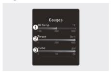
This mode displays information related to your engine such as engine oil temperature (1), current torque (2) and turbo boost pressure (3).
