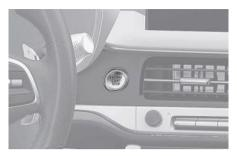
Whenever the front door is opened, the Engine Start/Stop button illuminates and goes off 30 seconds after the door is closed.
