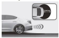
The smart trunk detecting area extends about 20-40 in. (50-100 cm) behind the vehicle. If you are positioned in the detecting area and are carrying the smart key, the hazard warning lights will blink and the chime will sound for about 3 seconds to alert you that the smart trunk will open.
