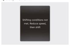
This message appears when engine rpm is too high, or when driving speed is too fast to shift the gear.
