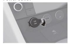
The power outlet is designed to provide power for mobile telephones or other devices designed to operate with vehicle electrical systems. The devices should draw less than 180 W with the engine running.
