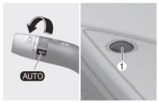
The parking light and headlight will be turned ON or OFF automatically depending on the amount of daylight as measured by the ambient light sensor (1) at the upper end of the windshield glass.
