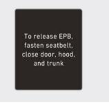
To release EPB, fasten seatbelt, close door, hood and trunk
