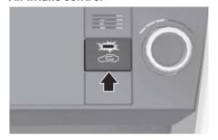
The air intake control button is used to select either Fresh mode (outside air) or Recirculation mode (cabin air).
