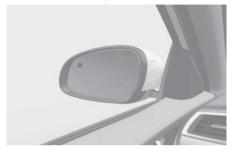
To warn the driver a vehicle is detected, the warning light on the side view mirror illuminates.
