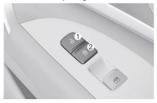
The driver and passenger side door armrest are equipped with a central door lock switch. The lock switch is indicated by a fi symbol. The unlock switch is indicated by a fi symbol.
