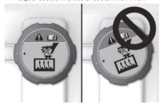
Make sure that the tiny protrusions inside the coolant cap are securely interlocked.
