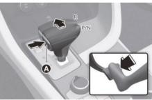
To move the shift lever to R (Reverse), press the **UNLOCK** button [A] while depressing the brake pedal and then move the shift lever forward.
