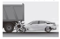
Just before impact, drivers often brake heavily. Such heavy braking lowers the front portion of the vehicle causing it to "nosedive". This is particularly important when the vehicle in front has a higher ground clearance. Airbags may not inflate if your vehicle is in a "nosedive" condition because the collision forces detected by the sensors may have been significantly reduced.
