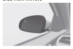
Your vehicle is equipped with both left-hand and right-hand side view mirrors. The mirrors can be adjusted remotely with the mirror adjustment control switch. The side view mirrors can be folded to help prevent damage when going through an automatic car wash or when passing through a narrow street.
