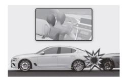
Front airbags are not designed to inflate in rear collisions, because occupants are moved backward by the force of the impact. In this case, inflated airbags would not provide any additional benefit.
