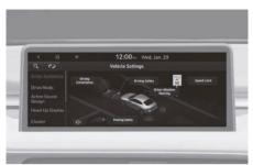
Vehicle Settings in the infotainment system provides user options for a variety of settings including door lock/unlock features, convenience features, driver assistance settings, etc.
