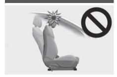
If you recline the seatback towards the front with the head restraints and seat cushion raised, the head restraint may come in contact with the sunvisor or other parts of the vehicle.
