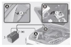
6. Connect the jumper cables in the exact sequence shown in the illustration. First connect one jumper cable to the red, positive (+) jumper terminal of your vehicle (1).
