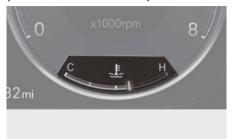
This gauge indicates the temperature of the engine coolant when the Engine Start/Stop button is in the ON position.
