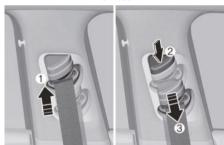
To adjust the height of the seat belt anchor, lower or raise the height adjuster into an appropriate position.
