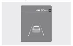
If the vehicle ahead and/or both lane markings are detected and your vehicle speed is below 120 mph (200 km/h), the green indicator light illuminates on the instrument cluster, and Lane Following Assist helps center the vehicle in the lane by assisting the steering wheel.
