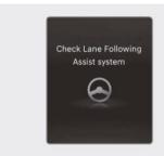
When Lane Following Assist is not working properly, the "Check Lane Following Assist system" warning message will appear for several seconds, and the master (1) warning light will illuminate on the instrument cluster. If this occurs, have your vehicle inspected by an authorized retailer of Genesis Branded products.
