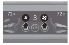
Touch the icon button to increase fan speed and airflow. Touch the left icon to decrease fan speed and airflow.
