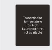
A warning message will pop up on the cluster display if the transmission fluid temperature is above a certain level while using Launch Control. Also, Launch Control will be automatically deactivated.
