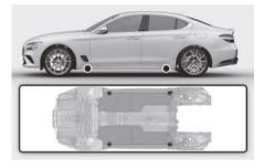
8. Insert the jack handle into the jack and turn it clockwise, raising the vehicle until the tire clears the ground. Make sure the vehicle is stable on the jack.
