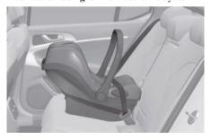
A rearward-facing Child Restraint System provides restraint with the seating surface against the back of the child. The harness system holds the child in place, and in an accident, acts to keep the child positioned in the Child Restraint Systems
