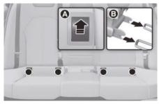
[A] Lower Anchorage Position Indicator [B] Lower Anchorage
