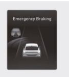
To warn the driver that emergency braking will be assisted, the "Emergency Braking" warning message appears and the warning light blinks on the instrument cluster with a warning sound and the steering wheel vibrates.
