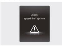
When Intelligent Speed Limit Assist is not working properly, the "Check speed limit system" warning message will appear on the instrument cluster for several seconds, and the master (△) warning light and the speed limit (□) warning light will illuminate on the instrument cluster. If this occurs, have your vehicle inspected by an authorized retailer of Genesis Branded products.
