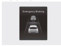
To warn the driver that emergency braking will be assisted, the "Emergency Braking" warning message appears and the warning light blinks on the instrument cluster with a warning sound and the steering wheel vibrates.
