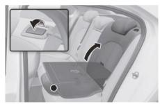
2. Push the seatback firmly until it clicks into place. Make sure the seatback is locked in place.
