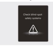
When Safe Exit Warning is not working properly, the "Check Blind-Spot Safety system" warning message will appear on the instrument cluster for several seconds, and the master (A) warning light will illuminate on the instrument cluster. If this occurs, have your vehicle inspected by an authorized retailer of Genesis Branded products.
