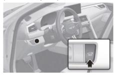
When the trunk is closed, press the power trunk open/close button for 1 second. The power trunk will open with a warning sound.
