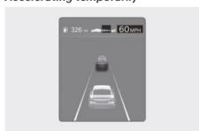
If you want to speed up temporarily without altering the set speed while Smart Cruise Control is operating, depress the accelerator pedal. While the accelerator pedal is depressed, the set speed, distance level and target distance will blink on the instrument cluster.
