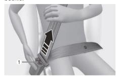
Once it is released, the belt should automatically draw back into the retractor. If this does not happen, check the belt to be sure it is not twisted, then try again.
