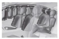
Side and curtain airbags and the front center side airbag are designed to inflate when an impact is detected by side collision sensors depending on the severity of impact resulting from a side impact collision.
