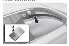
If a window senses any obstacle while it is closing automatically, it will stop and lower about 12 in. (30 cm) to allow the object to be cleared.
