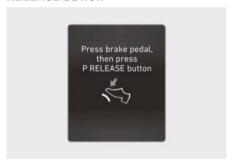
The message appears on the cluster display when the driver presses the **P RELEASE** button without depressing the brake pedal.
