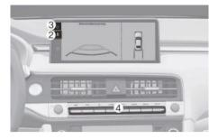
The rear view appears on the screen to assist in parking.
