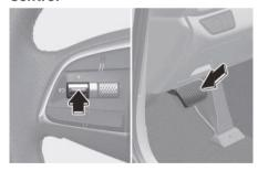
Press the poswitch or depress the brake pedal to temporarily cancel Smart Cruise Control.
