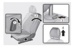
To remove the head restraint:
