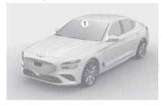
(1) Front view camera See the illustration above for the detailed location of the detecting sensor.
