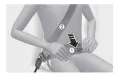
The seat belt automatically adjusts to the proper length after the lap belt portion is adjusted manually so that it fits snugly around your hips. If you lean forward in a slow, easy motion, the belt will extend and move with you.
