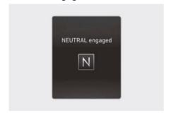
The message appears on the cluster display when the N (Neutral) position is engaged.
