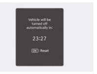
When all the conditions are satisfied, the Vehicle Auto-Shut Off operates and turns the engine off automatically after 60 minutes.
