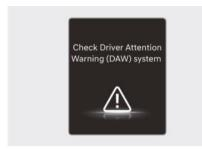
When Driver Attention Warning is not working properly, the "Check Driver Attention Warning (DAW) system" warning message will appear on the instrument cluster for several seconds, and the master ((A)) warning light and the driver's attention ((B)) warning light will illuminate on the instrument cluster. If this occurs, have your vehicle inspected by an authorized retailer of Genesis Branded products.
