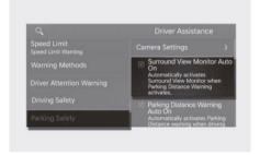
With the engine on, select **Setup** > **Vehicle** > **Driver Assistance** > **Parking Safety** > **Surround View Monitor Auto On** from the Settings menu in the infotainment system to use the function.
