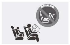
Even though your vehicle is equipped with the OCS, never install a child restraint in the front passenger's seat. An inflating airbag can forcefully strike a child or child restraint resulting in serious or fatal injury.
