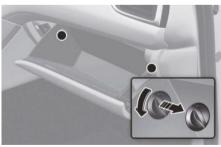
Pull out the cover while Pressing and holding the lock on the left side of the cover.
