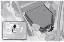
5. Push in a new fuse of the same rating, and make sure it fits tightly in the clips. If it does not fit tightly, consult an authorized retailer of Genesis Branded products.
