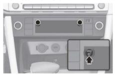
While the engine is running, touch the seat warmer icon to warm the driver's seat or front passenger's seat on the climate control information screen.
