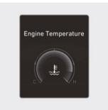
For 8-inch instrument cluster, you can check the engine coolant temperature in the Utility view on the cluster.
