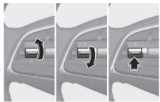
To resume Manual Speed Limit Assist after the function was paused, operate the +, -, || > switch.
