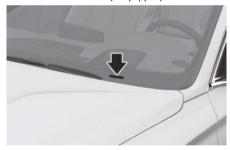
The VIN is also on a plate attached to the top of the left side dashboard. The number on the plate can easily be seen through the windshield from outside.
