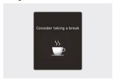
The "Consider taking a break" message will appear and the driver's attention (b) warning light will blink on the instrument cluster with a warning sound to suggest that the driver take a break, when the driver's attention level is below a certain level
