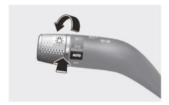
High Beam Assist automatically controls the headlights between high beam and low beam depending on the detected ambient light, such as an oncoming vehicle or leading vehicle.
