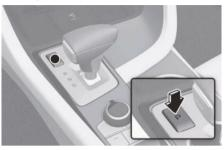
To shift the gear to P (Park), press the **P** button while depressing the brake pedal. If you turn the engine off in R (Reverse) or D (Drive), the gear will automatically shift
