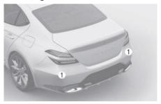
(1) Rear corner radar See the illustration above for the detailed location of the detecting sensors.
