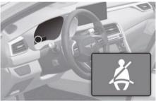
As a reminder to the driver, the seat belt warning light will illuminate for about 6 seconds each time the Engine Start/Stop button is in the ON or START position regardless of seat belt fastening.
