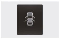
This warning appears if any door or hood or trunk is left open. The warning will indicate which door is open in the display.
