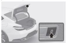
Press the power trunk lock button while carrying the smart key. The power trunk will close and lock with a warning sound. Additionally, all doors will lock.
