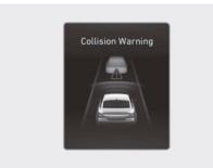
To warn the driver of a collision, the "Collision Warning" warning message appears and the ♣ warning light blinks on the instrument cluster with a warning sound and the steering wheel vibrates.
