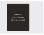
When the front windshield where the front view camera is located is covered with foreign material, such as snow or rain, it can reduce the detecting performance and temporarily limit or disable Intelligent Speed Limit Assist. If this occurs, the "Speed limit system disabled. Camera obscured" warning message and the speed limit (
