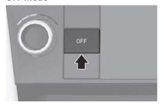
Press the OFF button to turn the climate control system off. You can still operate the air intake buttons as long as the Engine Start/Stop button is in the ON position.
