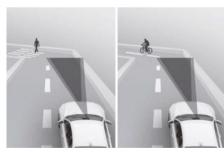
Forward Collision-Avoidance Assist may not detect a vehicle, a powered two-wheeler, and a pedestrian or a cyclist in front of you when driving on curved roads adversely affecting the performance of the sensors. This may result in no warning, braking assist when necessary.
