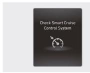
When Smart Cruise Control is not working properly, the "Check Smart Cruise Control system" warning message will appear, and the master (A) warning light will illuminate on the instrument cluster. If this occurs, have your vehicle inspected by an authorized retailer of Genesis Branded products.
