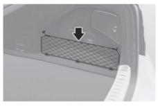
To keep items from shifting in the cargo area, you can use the 4 holders located in the luggage board to attach the luggage net.
