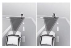
Forward Collision-Avoidance Assist may detect a vehicle, powered two-wheeler, and pedestrian or cyclist in the next lane or outside the lane when driving on a curved road.
