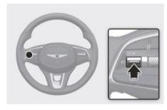
Press the JO switch to temporarily pause the set speed limit. The set speed limit will turn off but the Speed Limit (SLIMIT) indicator will stay on.
