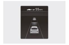
The status of Smart Cruise Control, Lane Following Assist, Highway Driving Assist, etc. appears when Driving Assist view is selected.
