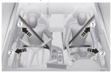
(1) Retractor pretensioner seat belt (Driver and front passenger)(2) Emergency Fastening Device (EFD)
