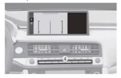
When you touch the icon, the top view appears on the screen and shows the distance from the vehicle in the back of your vehicle while parking.
