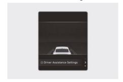
When Driver Assistance Settings menu is selected, press the OK switch on the steering wheel. The "**Driver Assistance**" menu will be displayed on the infotainment system.
