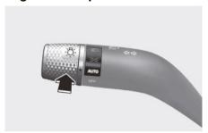
To turn on the high beam headlight, push the lever away from you. The lever will return to its original position.
