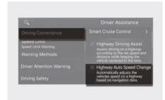
With the engine on, select Setup > Vehicle > Driver Assistance > Driving Convenience > Highway Auto Speed Change from the Settings menu in the infotainment system to turn on Navigation-based Smart Cruise Control and deselect to turn off the function.
