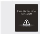
When the side view mirror warning light is not working properly, the "Check side view mirror warning light" warning message will appear on the instrument cluster for several seconds, and the master (A) warning light will illuminate on the instrument cluster. If this occurs, have your vehicle inspected by an authorized retailer of Genesis Branded products.
