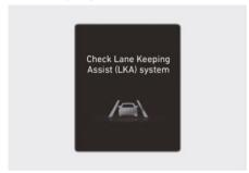
When Lane Keeping Assist is not working properly, the "Check Lane Keeping Assist (LKA) system" warning message will appear and the yellow indicator light will illuminate on the instrument cluster. If this occurs, have your vehicle inspected by an authorized retailer of Genesis Branded products.
