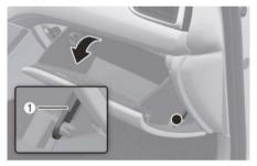
Remove the stoppers on both sides to allow the glove box to hang freely on the hinges.
