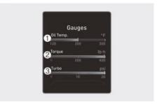
This mode displays information related to your engine such as engine oil temperature(1), current torque(2) and turbo boost pressure(3).
