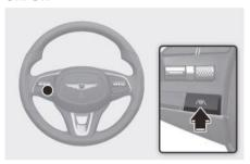
With the engine on, shortly press the Lane Driving Assist ( $_{(\!\varnothing\!)}$ ) button located on the steering wheel to turn on Lane Following Assist. The gray or green  $_{\! \Theta\! }$  indicator light will appear on the instrument cluster.
