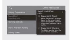
With the engine on, select or deselect **Setup > Vehicle > Driver Assistance > Speed Limit Assist** from the Settings menu in the infotainment system to set whether to use each function.
