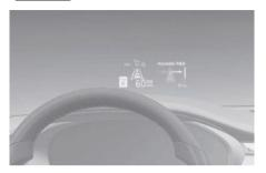
The Head-Up Display is an optional feature that allows the driver to view information projected onto a transparent screen while still keeping your eyes safely on the road ahead while driving.
