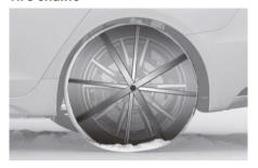
Since the sidewalls on some radial tires are thinner than other types of tires, they may be damaged by mounting certain types of tire chains on them. Do not mount tire chains on vehicles equipped with aluminum wheels; if possible use AutoSock® (fabric snow chain or similar). Install AutoSock® after reviewing the instructions provided with AutoSock®. Damage to your vehicle caused by improper use of fabric snow chains are not covered by your vehicle manufacturer's warranty.
