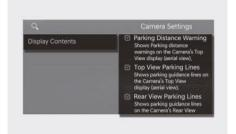
You can change Surround View Monitor Display Contents by touching the setup icon (5) on the screen while Surround View Monitor is operating, or selecting Setup > Vehicle > Driver Assistance > Parking Safety > Camera Settings from the Settings menu in the infotainment system while the engine is on.
