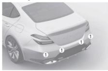
(1) Rear ultrasonic sensors See the illustration above for the detailed location of the detecting sensors.
