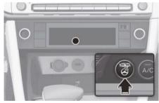
While the engine is running, touch the heated steering wheel icon to warm the steering wheel.
