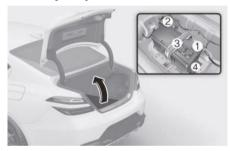
When replacing the battery, disconnect the negative (-) cable (1) and remove the positive (+) battery fuse box (2). Remove the trunk panel and spare wheel. Place the spare wheel on the floor with the finished side up so as not to damage. Then remove the spare wheel bracket (3) followed by the battery hold down mounting bracket (4).
