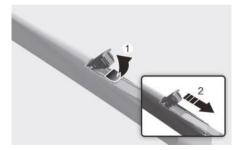
3. Install a new wiper blade assembly in the reverse order of removal (3).
