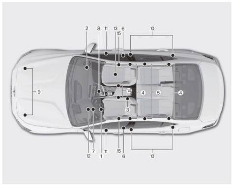
The SRS consists of the following components:
