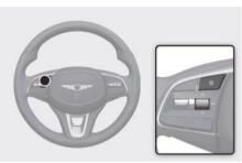
The cluster display modes can be changed by using the control switches.
