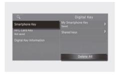
To delete all the registered digital key (smartphone), select **Setup** > **Vehicle** > **Digital Key** > **Smartphone key** > **Delete All** from the Settings menu in the infotainment system.
