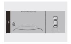
To warn the driver of an approaching vehicle from the rear left/right side of your vehicle, the warning light on the side view mirror will blink and a warning will appear on the instrument cluster. At the same time, an audible warning will sound and the steering wheel will vibrate. Rear View Monitor is operating, a warning will also appear on the infotainment system.
