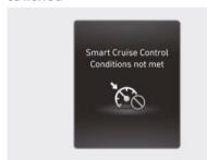
If the Driving Assist button, + switch, - switch or possible switch is operated when Smart Cruise Control operating conditions are not satisfied, the "Smart Cruise Control conditions not met" will appear on the instrument cluster, and an audible warning will sound.
