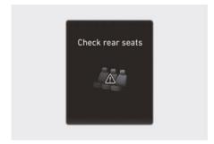
When you turn off the engine and open the driver's door after opening and closing the rear door, the "Check rear seats" warning message appears on the instrument cluster.
