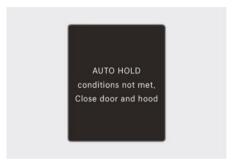
When you press the AUTO HOLD switch, if the driver's door and engine hood are not closed, a warning will sound and a message will appear on the cluster display.
