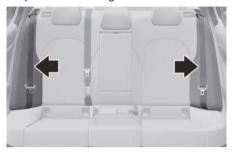
Pull up the seatback folding lever, then fold the seat toward the front of the vehicle.
