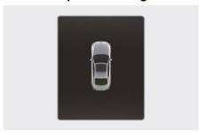
If the driver turns off the engine when the sunroof is not fully closed, the warning chime will sound for several seconds and the sunroof open warning will appear on the cluster display.
