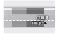
Blind-Spot Collision-Avoidance Assist helps detect and informs the driver that a vehicle is in the blind spot.
