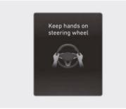
If the driver takes their hands off the steering wheel for several seconds, the "Keep hands on the steering wheel" warning message appears on the instrument cluster, and an audible warning sounds in stages.
