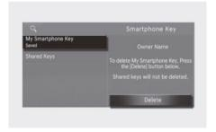
To delete only my registered digital key (smartphone), select **Setup** > **Vehicle** > **Digital Key** > **Smartphone key** > **My Smartphone Key** > **Delete** from the Settings menu in the infotainment system.
