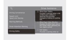
With the engine on, select **Setup** > **Vehicle** > **Driver Assistance** > **Driving Safety** > **Blind-Spot Safety** from the Settings menu in the infotainment system to set whether to use each function.
