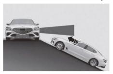
Rear Cross-Traffic Collision-Avoidance Assist may be limited when the vehicle is on a uphill or downhill slope, or near it, and may not detect the vehicle approaching from the left or right. If this occurs, the function may not warn the driver or control the brakes when necessary.
