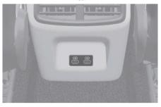
The electrical devices can be recharged when the Engine Start/Stop button is in the ON (or START) position.
