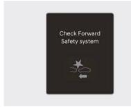
When Forward Collision-Avoidance Assist is not working properly, the "Check Forward Safety system" warning message will appear, and the A and warning lights will illuminate on the instrument cluster. Have your vehicle inspected by an authorized retailer of Genesis Branded products.
