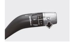
In the OFF position, pull the lever gently toward you to spray washer fluid on the windshield and to run the wipers 1-3 cycles. The spray and wiper operation will continue until you release the lever. If the washer does not work, you may need to add washer fluid to the washer fluid reservoir.
