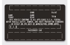
The certification label is located on the driver's door sill at the center pillar and shows the maximum allowable weight of the fully loaded vehicle. This is called the GVWR (Gross Vehicle Weight Rating). The GVWR includes the weight of the vehicle, all occupants, fuel and cargo.
