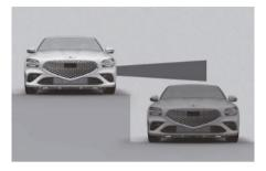
Blind-Spot Collision-Avoidance Assist may not operate properly when driving where the heights of the lanes are different. The function may not detect the vehicle on a road with different lane heights (underpass joining section, grade separated intersections, etc.).
