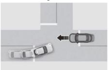
Junction Turning function can help avoid a collision with an oncoming vehicle or powered two-wheeler in an adjacent lane when turning left at a crossroad with the turn signal on by applying emergency braking.
