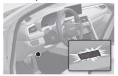
The foot lamp turns on when a door is open and turns off when the door is closed.
