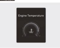
Engine coolant temperature gauge display shows the temperature of the engine coolant when the engine is running.
