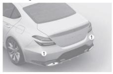
(1) Rear corner radar See the illustration above for the detailed location of the detecting sensors.
