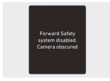
When the front windshield where the front view camera is located, or sensor is covered with foreign material, such as snow or rain, it can reduce the detecting performance and temporarily limit or disable Lane Keeping Assist.
