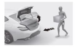
On a vehicle equipped with a smart key, the trunk can be opened with hands-free activation using the smart trunk system.
