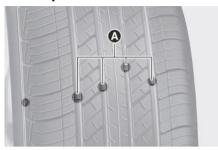
[A]Tread wear indicator If the tire is worn evenly, a tread wear indicator appears as a solid band across the tread. This shows there is less than 1/16 inches (1.6 mm) of tread left on the tire. Replace the tire when this happens.
