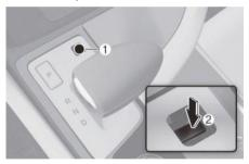
Then, the gear will change to the N (Neutral) position. The button (2) operates only for 20 seconds to change the gear between P (Park) and N (Neutral) from the time when the button (2) is first pressed.
