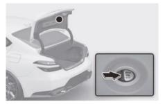
Your vehicle is equipped with an Emergency Trunk Safety Release lever located inside the vehicle. When someone is inadvertently locked in the trunk, the trunk can be opened by moving the lever in the direction of the arrow and pushing the trunk open.
