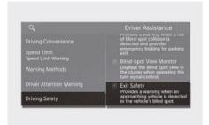
With the engine on, select Setup > Vehicle > Driver Assistance > Driving Safety > Exit Safety from the Settings menu in the infotainment system to set whether to use each function.
