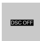
Indicator light illuminates: Dynamic Stability Control is deactivated.
