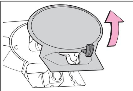
**3** Insert the mechanical key into the key cylinder, and turn it clockwise to open the trunk.
