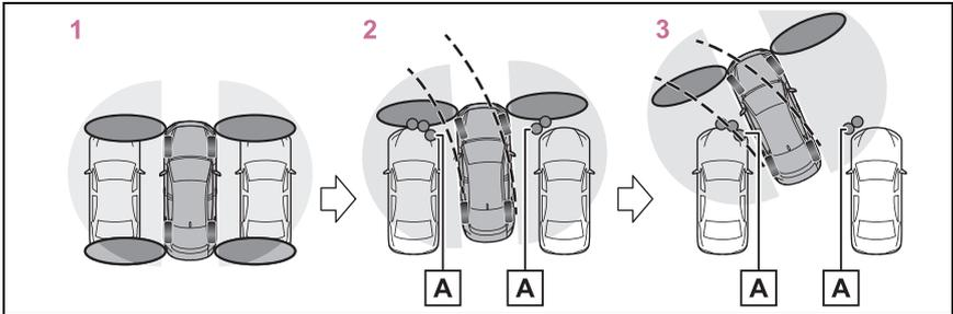
**A** Object detected by side sensors or side cameras
