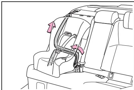
7 If the child restraint has a top tether strap, follow the child restraint manufacturer's operation manual regarding the installation, using the top tether strap to latch onto the top tether strap anchor. (→P.64)
