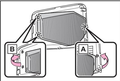
**7** Install the air intake vent cover.
