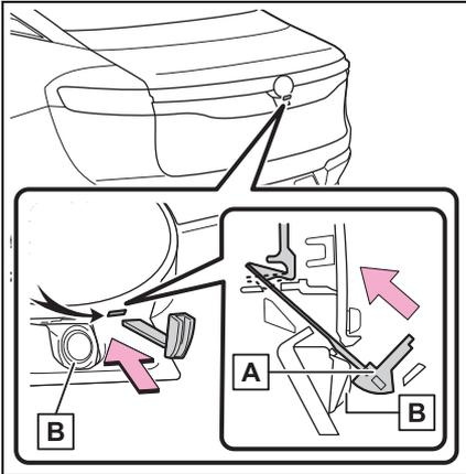
**2** While pushing the mechanical key into the hole, pull the emblem base up to remove it.
