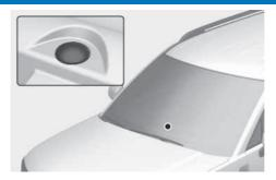
Never place anything near the sensor to ensure better control of the heating and cooling system.
