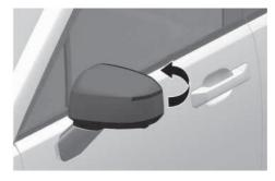
To fold the side view mirror, grasp the housing of the mirror and then fold it toward the rear of the vehicle.
