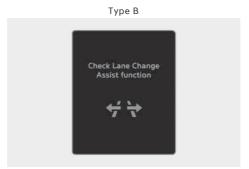
When Highway Driving Assist is not working properly, the "Check Driver Assistance system." or "Check Lane Change Assist function" warning message and Master (A) warning light appears on the instrument cluster. If this occurs, have your vehicle inspected by an authorized HYUNDAI dealer.
