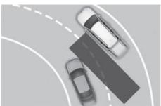
Blind-Spot Collision-Avoidance Assist may not operate properly when driving on a curved road. The function may not detect the vehicle in the next lane. Always pay attention to road and driving conditions while driving.
