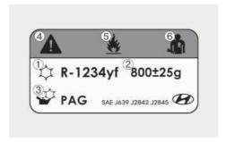
Each symbols and specification on the air conditioning refrigerant label is represented as the following:
