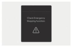
When Emergency Stop is not working properly, the "Check Emergency Stopping function." warning message appears, and the master (A) warning light illuminates on the instrument cluster. If this occurs, have your vehicle inspected by an authorized HYUNDAI dealer.
