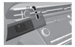
This is the normal driving position. The transmission automatically shifts through a 8 gear sequence, providing the best fuel economy and power.
