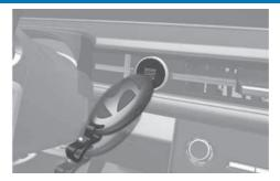
If the smart key battery is weak or the smart key does not work correctly, press the Engine Start/Stop button with the smart key.
