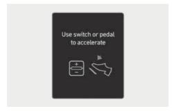
In traffic, your vehicle will stop if the vehicle ahead of you stops. Also, if the vehicle ahead of you starts moving, your vehicle will start as well. In addition, after the vehicle has stopped and a certain time have passed, the "Use switch or pedal to accelerate" message will appear on the instrument cluster. Depress the accelerator pedal or operate the + switch, - switch or || \(\mathbb{O}\) switch to start driving.
