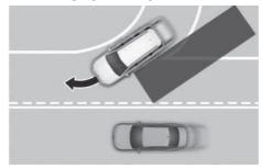
Blind-Spot Collision-Avoidance Assist may not operate properly when driving where the road merges or divides. The function may not detect the vehicle in the next lane.
