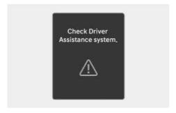
When Blind-Spot Collision-Avoidance Assist is not working properly, the "Check Driver Assistance system." warning message will appear on the instrument cluster for several seconds, and the master (A) warning light will appear on the instrument cluster. If this occurs, have your vehicle inspected by an authorized HYUNDAI dealer.
