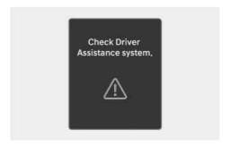
When Smart Cruise Control is not working properly, the "Check Driver Assistance system." warning message will appear, and the "A" warning light will illuminate on the instrument cluster. Have your vehicle inspected by an authorized HYUNDAI dealer.
