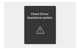
When Rear Cross-Traffic Collision-Avoidance Assist is not working properly, the "Check Driver Assistance system." warning message appears on the instrument cluster for several seconds, and the master (A) warning light illuminates on the instrument cluster. If this occur, have vehicle inspected by an authorized HYUNDAI dealer.
