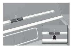
Press the ISG OFF button to turn off the ISG system. The ISG OFF button indicator illuminates. To use the system, press the ISG OFF button again.
