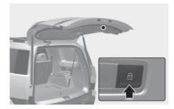
Press the power liftgate lock button while carrying the smart key. The liftgate closes and locks automatically. Additionally, all doors will lock.
