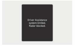
When the rear bumper around the rear corner radar or sensor is covered with foreign material, such as snow or rain, or installing a trailer or carrier, it can reduce the detecting performance and temporarily limit or disable Safe Exit Assist.
