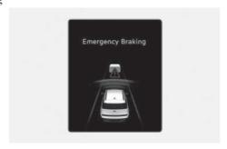
To warn the driver that emergency braking will be assisted, Forward Safety warning light (♣) blinking, the "Emergency Braking" warning message will appear on the instrument cluster, an audible warning will sound and the steering wheel will vibrate.
