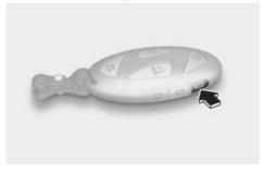
When the liftgate is closed, press the power liftgate open button for 1 second. The liftgate will open with a warning sound.
