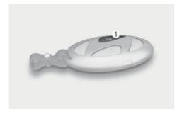
Press and hold the Door Unlock button (1) on the smart key for more than 3 seconds and the windows move down after the doors are unlocked. Window movement stops when you release the door unlock button.
