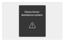
When High Beam Assist is not working properly, the "Check Driver Assistance system" warning message may appear, and the \( \frac{\Lambda}{\text{ warning light may illuminate}} \) on the instrument cluster. Contact an authorized HYUNDAI dealer.
