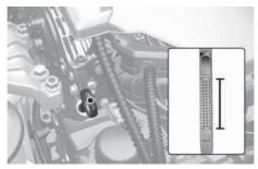
7. If the oil level is below the L, add enough oil to bring the level to F.
