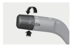
High Beam Assist automatically adjusts the headlights between high beam and low beam depending on the light detected from oncoming vehicles or vehicles in front using the front view camera.
