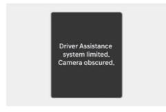
When the front windshield where the front view camera is located is covered with foreign material, such as snow or rain, it can reduce the detecting performance and temporarily limit or disable Intelligent Speed Limit Assist. If this occurs, the "Driver Assistance system limited. Camera obscured." warning message and ( $\square$ ) warning light will appear on the instrument cluster.
