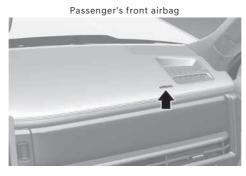
The SRS consists of advanced airbags located in the center of the steering wheel and the passenger's side front panel pad above the glove box.
