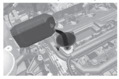
Use only the specified engine oil (Refer to the "Recommended lubricants and capacities" section in chapter 10).
