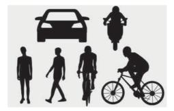
The illustration above shows the image the front view camera and front radar are capable of detecting as a vehicle, pedestrian and cyclist.
