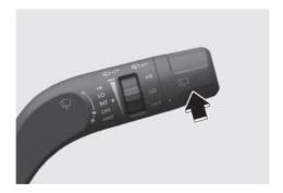
The rear wiper operates while the vehicle is in reverse with the front wiper on. You can select the function from the Settings menu in the infotainment system. Select:
