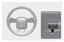
Press the IID switch to temporarily pause the set speed limit. The set speed limit will turn off but the Speed Limit (©LIMIT) indicator will stay on.
