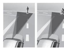
Forward Collision-Avoidance Assist may detect a vehicle, powered twowheeler, pedestrian or cyclist in the next lane or outside the lane when driving on a curved road.
