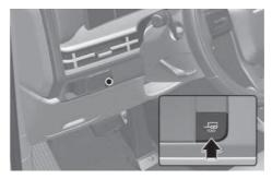
Press the Tow mode button to turn on or off the function.
