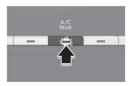
Press the 3rd row air conditioning A/C REAR button located on the front climate control panel.
