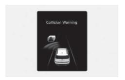
• To warn the driver of a collision, Forward Safety warning light (♣) blinking, the "Collision Warning" warning message will appear on the cluster, an audible warning will sound, and the steering wheel will vibrate.
