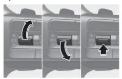
To resume Manual Speed Limit Assist after the function was paused, operate the  $+, -, \mathbb{ID}$  switch.
