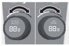
The temperature increases by turning the knob to the right (red side). The temperature decreases by turning the knob to the left (blue side).
