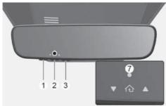
1. Press and release the HomeLink button (1), (2) or (3), you would like to program. The HomeLink indicator light (7) will flash orange slowly (if not, perform the steps of "Erasing HomeLink Buttons" section, and start over).
