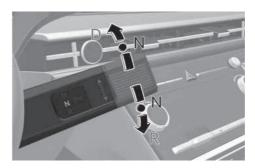
The wheels and transmission are not engaged.
