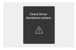
When Lane Keeping Assist is not working properly, the "Check Driver Assistance system." warning message appears and the master (A) warning light and yellow Lane Safety (A) indicator light illuminates on the instrument cluster. If this occurs, have your vehicle inspected by an authorized HYUNDAI dealer.
