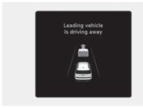
When a detected vehicle in front departs from a stop, Leading Vehicle Departure Alert will inform the driver by displaying the "Leading vehicle is driving away" message on the instrument cluster and an audible warning will sound.
