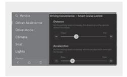
With the engine on, select Setup > Vehicle > Driver Assistance > Driving Convenience > Smart Cruise Control from the Settings menu in the infotainment system, you can change the vehicle distance, the acceleration, and the reaction speed manually.
