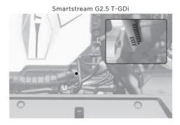
The engine number is stamped on the engine block as shown in the illustration.
