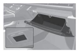
The glove box lamp turns on when the glove box is opened. If the glove box is not closed, the lamp turns off after 20 minutes.
