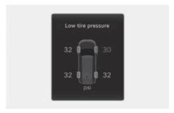
TMPS is not a substitute for manually checking the tire pressure with a tire gauge. Changes in temperature affect tire pressure. Refer to "Check tire inflation pressure" in the Maintenance chapter for proper tire inflation and tire pressure measurement procedure.
