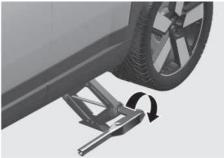
9. Loosen a wheel bolt with the wheel lug wrench and remove it with your fingers.
