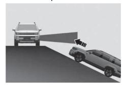
Rear Cross-Traffic Collision-Avoidance Assist may be limited when the vehicle is on a uphill or downhill slope, or near it, and may not detect the vehicle approaching from the left or right. If this occurs, the function may not warn the driver or control the brakes when necessary.
