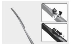
4. Install a new wiper blade assembly in the reverse order of removal.
