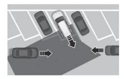
Rear Cross-Traffic Collision-Avoidance Assist may be limited when backing up diagonally, and may not detect the vehicle approaching from the left or right. If this occurs, the function may not warn the driver or control the brakes when necessary.
