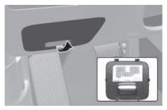
4. Refer to the label on the inside of the fuse panel cover to locate the suspected fuse location.
