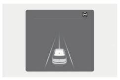
If the vehicle ahead and/or both lane markings are detected and your vehicle speed is below 110 mph (180 km/h), the green  $(\Theta)$  indicator light appears on the cluster, and Lane Following Assist helps center the vehicle in the lane by assisting the steering wheel.
