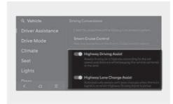
With the engine on, select or deselect **Setup > Vehicle > Driver Assistance > Driving Convenience > Highway Driving Assistance** from the infotainment system to set whether to use each function.
