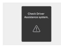
When Reverse Parking Collision-Avoidance Assist or other related functions are not working properly, the "Check Driver Assistance system." warning message appears on the instrument cluster, and Reverse Parking Collision-Avoidance Assist turns off automatically. Have your vehicle inspected by an authorized HYUNDAI dealer.
