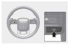
With the engine on, shortly press the Lane Driving Assist button located on the steering wheel to turn on Lane Following Assist. The gray or green  $(\Theta)$  indicator light will illuminate on the instrument cluster.
