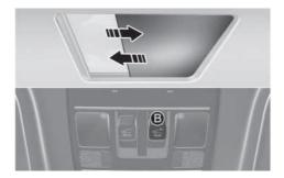
Push the power sunshade open switch (B), the power sunshade automatically slides open.
