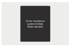
When the front windshield where the front view camera is located, front radar cover, bumper (if equipped) or sensor is covered with foreign material, such as snow or rain, it can reduce the detecting performance and temporarily limit or disable Forward Collision-Avoidance Assist.
