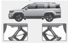
8. Insert the wheel lug wrench into the jack and turn it clockwise, raising the vehicle until the tire clears the ground. Make sure the vehicle is stable on the jack.
