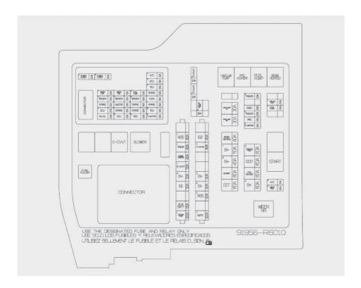
Engine compartment fuse panel
