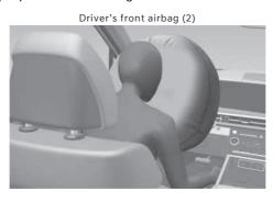
Upon deployment, tear seam in the pad cover separates from the expansion of the airbags.
