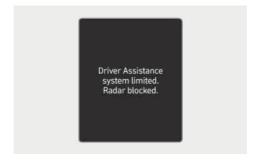
When the front radar cover or sensor is covered with snow, rain, or foreign material, it can reduce the detecting performance and temporarily limit or disable Smart Cruise Control.
