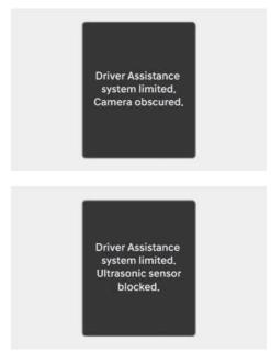
The "Driver Assistance system limited. Camera obscured." or "Driver Assistance system limited. Ultrasonic sensor blocked." warning message appears on the instrument cluster if the following situations occur:
