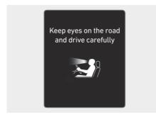
Forward Attention Warning determines whether the driver is focused on the road depending on information, such as the amount of time the driver is looking elsewhere, the amount of time the eyes are closed, how frequently the driver yawns, etc. If Forward Attention Warning judges the driver is not focused, the "Keep eyes on the road and drive carefully" warning message will appear on the cluster, and an audible warning will sound.
