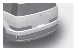
The rear corner radars are mounted near the rear corners of your vehicle above the bumper.
