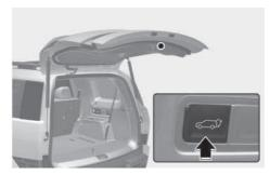
Press the power liftgate open/close button. The liftgate opens or closes automatically.
