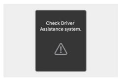
When Lane Following Assist is not working properly, the "Check Driver Assistance system." warning message will appear on the instrument cluster for several seconds, and the master (A) warning light appears on the instrument cluster. If this occur, have your vehicle inspected by an authorized HYUNDAI dealer.
