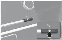
Press and hold the Parking Safety (P<sup>m</sup><u>a</u>) button more than 2 seconds, to turn the Parking Collision-Avoidance Assist on or off.
