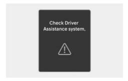
When Forward Collision-Avoidance Assist is not working properly, the **Check Driver Assistance system.** warning message will appear, and the \$\subseteq\$ or \$\noting\$ warning lights will illuminate on the instrument cluster. Have your vehicle inspected by an authorized HYUNDAI dealer.
