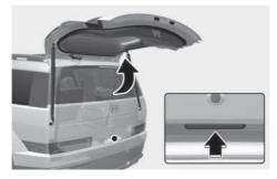
When the liftgate is closed, press the power liftgate open/close button to open the liftgate.
