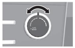
The temperature increases by turning the knob to the right. The temperature decreases by turning the knob to the left.
