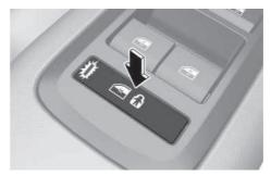
When the electronic child safety lock (a) button is in the LOCK position and an approaching vehicle from the rear area is detected, the electronic child safety lock button will not unlock even if the driver presses the button to prevent the rear doors from opening.
