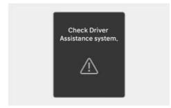
When Safe Exit Assist is not working properly, the "Check Driver Assistance system." warning message appears on the instrument cluster for several
