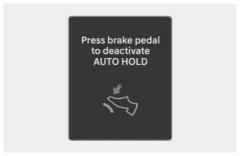
If you did not apply the brake pedal when you release Auto Hold by pressing the AUTO HOLD switch, a warning sounds and a message appears.
