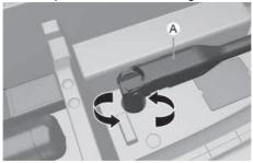
5. After the spare tire reaches the ground, continue to turn the wrench counterclockwise, and draw the spare tire outside. Never rotate the wrench excessively, otherwise the spare tire carrier may be damaged.
