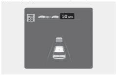
Manual Speed Limit Assist or Smart Cruise Control assists the vehicle to adjust its speed according to the speed limit. When the cruising speed is set as same as the speed limit, the vehicle automatically adjusts its speed if the speed limit changes. The function operates on the road which has a speed limit of 45 mph (70 km/h) or higher. When the function is active, the cruising speed on the instrument cluster appears in green.
