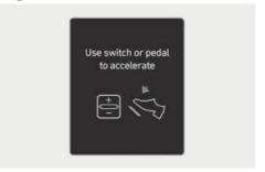
When Highway Driving Assist is operating, your vehicle will stop if the vehicle ahead of you stops. Also, if the vehicle ahead of you starts moving within 30 seconds after the stop, your vehicle will start as well. In addition, after the vehicle has stopped and 30 seconds have passed, the "Use switch or pedal to accelerate" message will appear on the instrument cluster. Depress the accelerator pedal or operate the + switch, - switch or II' which start driving.
