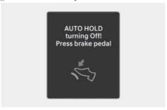
When the conversion from Auto Hold to EPB is not working properly, a warning sounds and a message appears.
