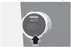
You can control the fan speed in three stages by pressing the **AUTO** button during automatic operation.
