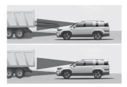
If the vehicle in front of you has cargo that extends rearward from the cab, or when the vehicle in front of you has higher ground clearance, additional special attention is required. Forward Collision-Avoidance Assist may not be
