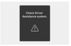
When Intelligent Speed Limit Assist is not working properly, the "Check Driver Assistance system." warning message will appear on the instrument cluster for several seconds, and the master (⚠) warning light and (☐) warning light will illuminate on the instrument cluster. If this occurs, have your vehicle inspected by an authorized HYUNDAI dealer.
