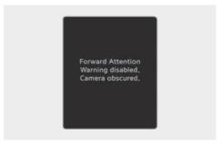
When there is an object right in front of the in-cabin camera or between the driver and the camera for a certain period of time, Forward Attention Warning does not operate properly, and the "Forward Attention Warning disabled. Camera obscured" warning message appears on the instrument cluster, and an audible warning sounds.
