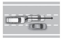
When vehicle speed is above 40 mph (60 km/h), if a vehicle around you is driving at a close distance, your vehicle will control steering in the opposite direction of the vehicle to assist in safe driving.
