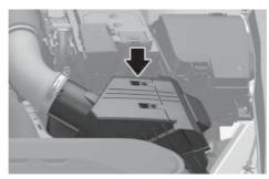
The air cleaner filter can be cleaned for inspection using compressed air. Do not attempt to wash or rinse it, because water can damage the filter. If soiled, replace the air cleaner filter.
