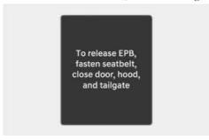
If the driver's seat belt is unfastened, or the hood, liftgate, doors are open, and you try to drive with EPB applied, a warning sounds and a message appears.
