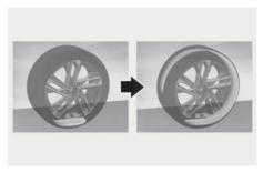
Do not exceed a speed of 50 mph (80 km/h). If possible, do not fall below a speed of 12 mph (20 km/h).
