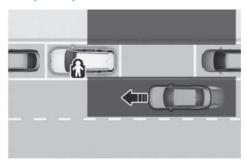
While your vehicle is stopped, if Safe Exit Assist detects a vehicle approaching the rear corner of your vehicle and a passenger opens a door, Safe Exit Assist may warn you with a warning message and a warning sound to help avoid a collision.
