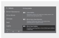
With the engine on, select **Setup > Vehicle > Driver Assistance > Driving Safety** > **Blind-Spot Safety** in the infotainment system to set whether to use each function.
