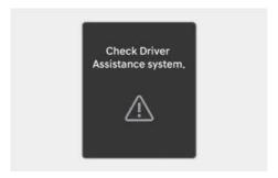
When Driver Attention Warning is not working properly, the "Check Driver Assistance system." warning message will appear on the cluster for several seconds, and the master (A) warning light and the driver's attention (b) warning light will appear on the instrument cluster. If this occurs, have your vehicle inspected by an authorized HYUNDAI dealer.
