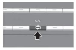
Press the A/C button to turn on the air conditioning system (indicator light ON). Press the button again to turn off the air conditioning system.
