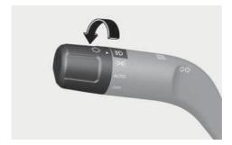
The headlight, parking light, license plate light, and instrument panel light are turned ON.
