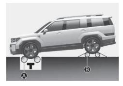
[A]: Roll tester (Speedometer)[B]: Temporary free roller
