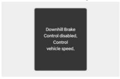
If Downhill Brake Control is not working properly, this warning message appears on the cluster display and you may hear a warning sound. If this occurs, control the vehicle speed by depressing the brake pedal.
