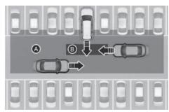
$\hbox{[A] Rear Cross-Traffic Collision Warning operating range}\\$
