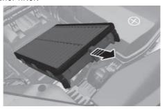
5. Reassemble the air cleaner filter cover in the reverse order.
