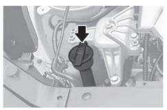
Check the fluid level in the washer fluid reservoir and add fluid if necessary. Plain water can be used during summer months if washer fluid is not available. However, use washer fluid with antifreeze in cold climates to prevent freezing.
