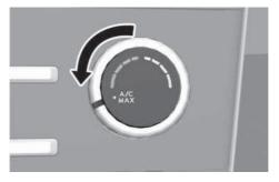
The MAX A/C mode is used to cool the inside of the vehicle faster. Air flow is directed toward the upper body and face.
