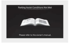
When "Parking Assist Conditions Not Met" message appears when Parking/View (印) button has been pressed and held while Remote Smart Parking Assist is in standby. After a while, press and hold the Parking/View (印) button again to see if Remote Smart Parking Assist works.
