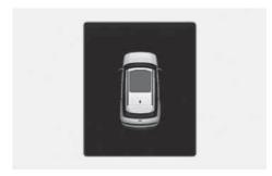
If the driver turns off the engine when the sunroof is not fully closed, the warning chime will sound for several seconds and the sunroof open warning will appear on the cluster display.
