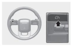
Press the Driving Assist (ਨ) button to turn Manual Speed Limit Assist off. The Speed Limit (ਨੀਂਪੁਸਸ) indicator will go off.
