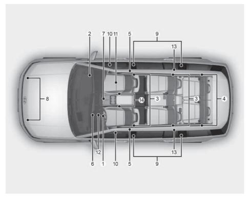
The SRS consists of the following components:
