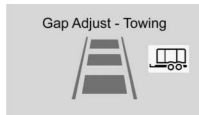
Far Gap Setting with Trailer
