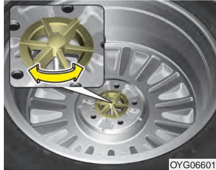
Turn the tire hold-down wing bolt counterclockwise.
