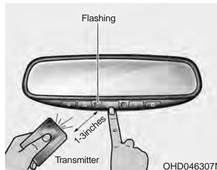
2. Press and hold the button on the HomeLink system you wish to train and the button on the transmitter while the transmitter is approximately 2-8 cm (1 to 3 inches) away from the mirror. Do not release the buttons until step 3 has been completed.
