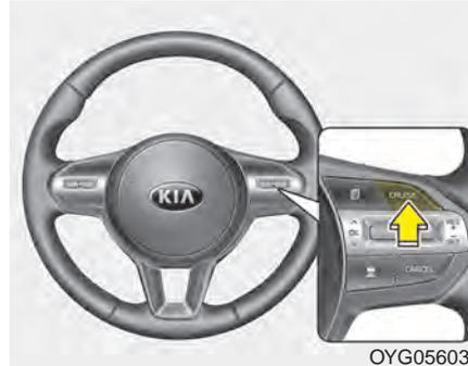
1. Press the CRUISE button, to turn the system on. The CRUISE indicator in the instrument cluster will illuminate.
