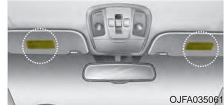
Air bag warning labels, some required by the U.S. National Highway Traffic Safety Administration (NHTSA), are attached to the sunvisors to alert the driver and passengers of potential risks of the air bag system.
