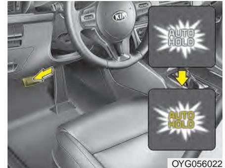
2. When coming to a complete stop by depressing the brake pedal, the AUTO HOLD indicator changes from white to green indicating the AUTO HOLD is engaged. The vehicle will remain at a standstill even if you release the brake pedal.
