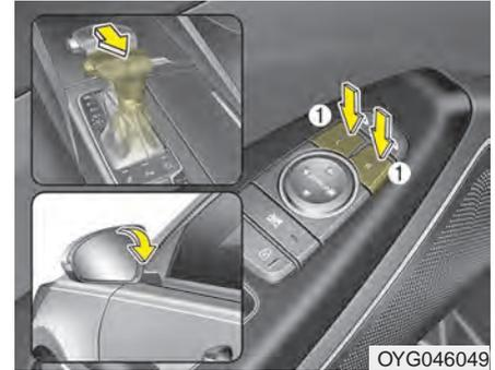
While the vehicle is moving in reverse, the outside rearview mirror(s) will move downward to aid reverse parking. According to the position of the outside rearview mirror switch (1), the outside rearview mirror(s) will operate as follows:
