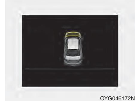
The warning message will appear on the LCD display when hood is open.
