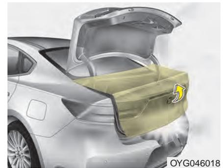
If during power opening or closing, the trunk is blocked by an object or part of someone's body, the power trunk will detect the resistance and it will stop movement or move to the full open position to allow the object to be cleared.
