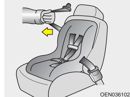
3. Pull the shoulder portion of the seat belt all the way out. When the shoulder portion of the seat belt is fully extended, it will shift the retractor to the "Automatic Locking" (child restraint) mode.
