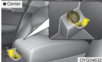
The power outlet is designed to provide power for mobile telephones or other devices designed to operate with vehicle electrical systems. The devices should draw less than 10 amps with the engine running.
