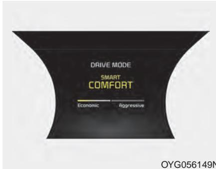
Once the SMART MODE is selected by pressing the DRIVE MODE button, and the DRIVE MODE indicator screen is selected by pressing the trip computer button on the steering wheel, the driving style gauge bar will show up at the bottom of screen and visualize current style of driving.
