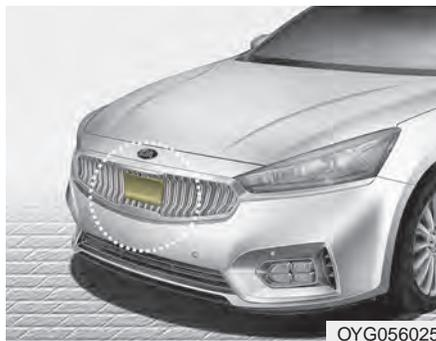
In order for the FCA system to operate properly, always make sure the sensor or sensor cover is clean and free of dirt, snow, and debris. Dirt, snow, or foreign substances on the lens may adversely affect the sensing performance of the sensor.
