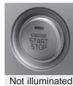
To turn off the engine (START/RUN position) or vehicle power (ON position), press the ENGINE START/STOP button with the shift lever in the P (Park) position. When you press the ENGINE START/STOP button without the shift lever in the P (Park) position, the ENGINE START/STOP button will not change to the OFF position but to the ACC position.
