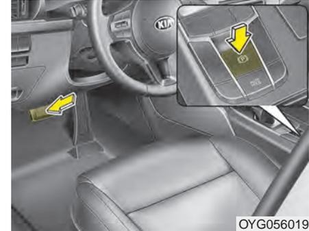
To release the EPB (electronic parking brake), press the EPB switch while doing the following:
