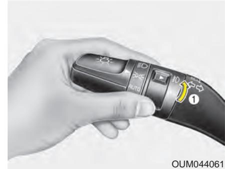
Fog lights are used to provide improved visibility when visibility is poor due to fog, rain or snow, etc. The fog lights will turn on when the fog light switch (1) is turned to the on position after the headlight is turned on.
