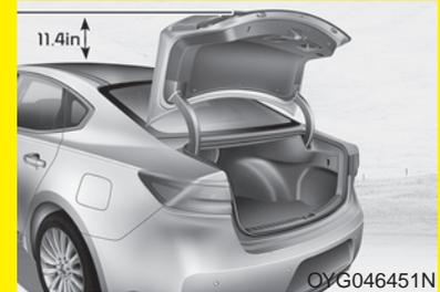
**Make sure that there are no people or objects in the path of the power trunk (or smart trunk) prior to use. Serious injury, damage to the vehicle or damage to surrounding objects may result if contact with the power trunk (or smart trunk) occurs.**
