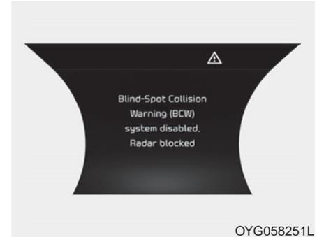
The message will appear to notify the driver if there are foreign substances on the surface or inside the rear bumper or it is hot near the rear bumper. The light on the switch and the system will be turned off automatically.
