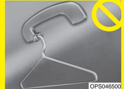
**Do not hang other objects such as hangers or hard objects except clothes. Also, do not put heavy, sharp or breakable objects in the pockets of the clothing. In an accident or when the curtain air bag is inflated, it may cause vehicle damage or personal injury.**
