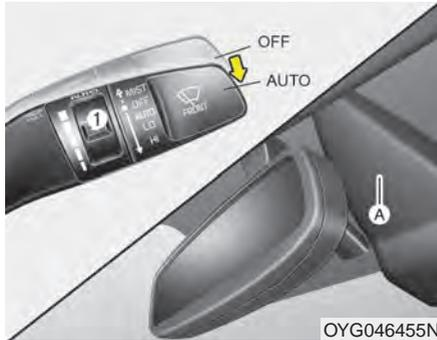
The rain sensor (A) located on the upper end of the windshield glass senses the amount of rainfall and controls the wiping cycle for the proper interval. The more it rains, the faster the wiper operates. When the rain stops, the wiper stops.
