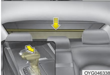
To fold the rear curtain, press the button. To unfold the rear curtain, press the button again.
