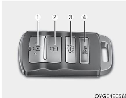
All doors are locked if the lock button is pressed. If all doors (and trunk) are closed, the hazard warning lights will blink once to indicate that all doors (and trunk) are locked.
