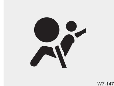
The purpose of air bag warning light in your instrument panel is to alert you of a potential problem with your air bag system, which could include your side and/or curtain air bags used for rollover protection.
