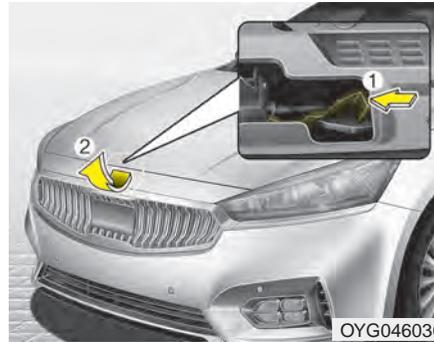
2. Go to the front of the vehicle, raise the hood slightly, push the secondary latch (1) left side of the hood center and lift the hood (2).
