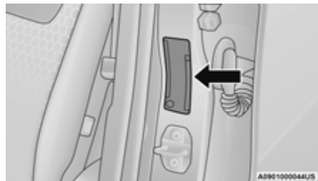
Example Tire Placard Location (B-pillar)
