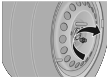
Installing Wheel Bolts
