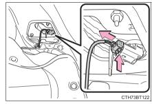
4 Turn the bulb base counter-clockwise.
