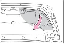
3 Disconnect the connector while depressing the lock release. (When replacing right side bulb only.)
