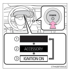
\*: If the shift lever is in a position other than P when turning off the hybrid system, the power switch will be turned to ACCESSORY mode, not to off.
