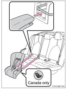
If the child restraint has a top tether strap, follow the child restraint manufacturer's operation manual regarding the installation, using the top tether strap to latch onto the top tether strap anchor. (→P. 70)
