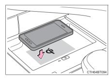
While charging, the operation indicator light (orange) will be illuminated. If charging does not begin, move the portable device as close to the center of the charging area as possible.
