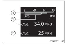
Displays the average vehicle speed since reset or elapsed time since reset, as selected in . (→P. 109)
