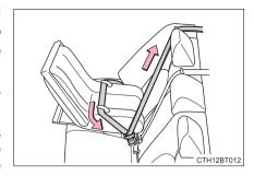
5 After installing the child restraint system, rock it back and forth to ensure that it is installed securely. (→P. 66)
