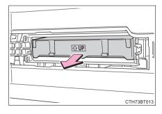
Remove the air conditioning filter from the filter case and replace it with a new one.
