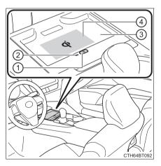
Additionally, if 2 or more portable devices are placed on the charging tray at the same time, each charging coil may not be detected correctly and charging may not be possible.
